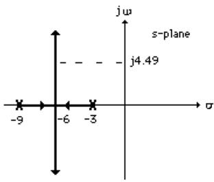
Adding the compensator pole and zero to the system poles, the gain at the design point is found to be 29.16. Summarizing the results:  $G_c(s) = \frac{s+5}{s+9}$  with K = 29.16.
