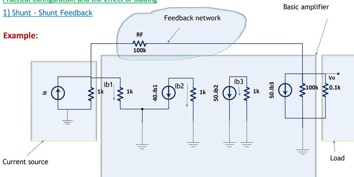
1) Shunt - Shunt Feedback
