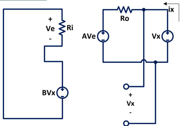
Series Feedback at the input always raises the input impedance by (1+AB)
