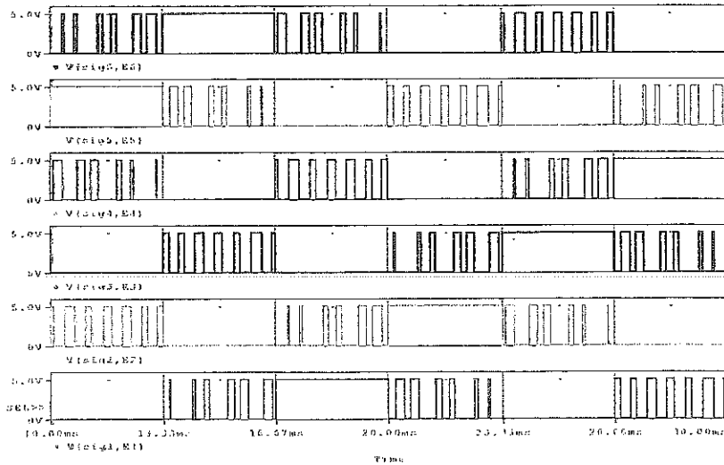
Figure VI.5: The equivalent Sinusoidal PWM signals in a CSI for M = 0.7 and f_c = 900\text{Hz}
