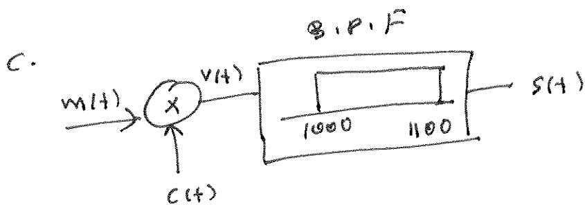
$$\begin{aligned} v(t) &= 4 \cos 2\pi(100)t [2 \cos 2\pi(50)t + 4 \cos 2\pi(100)t] \\ &= 4 \cos 2\pi(1050)t + 4 \cos 2\pi(950)t \\ &\quad + 8 \cos 2\pi 1100t + 8 \cos 2\pi(900)t \end{aligned}$$
