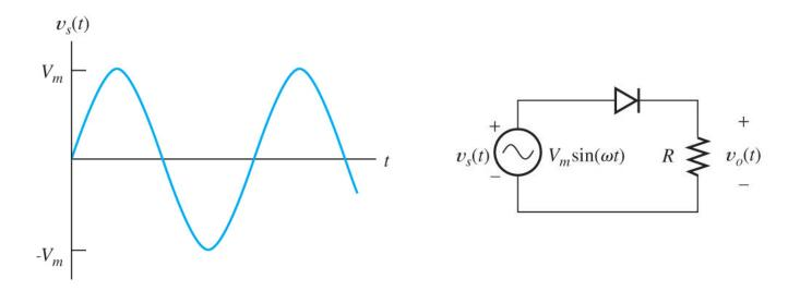
Example Problem 51. Consider the same circuit with an AM input  $v_s(t)$ . Again, assuming an ideal diode, draw the output waveform  $v_o(t)$ .
