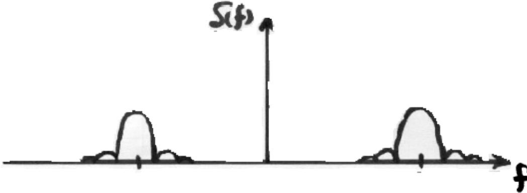
Figure 9.3b. Bandpass spectrum with baseband NRZ line codes.
