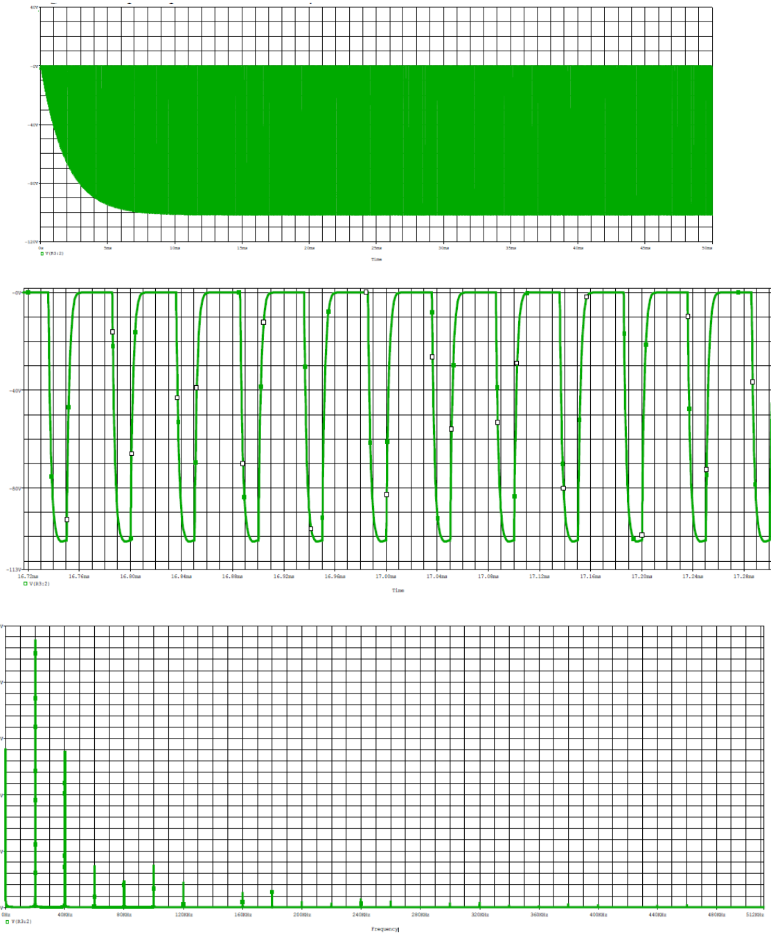
Figure 36: The output voltage, its ripple and FFT of the output voltage from Dc-Dc buck boost convertor at duty cycle 70% and 1uF capacitor
