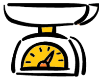
A scale giving a reading when no mass is placed has a zero drift
