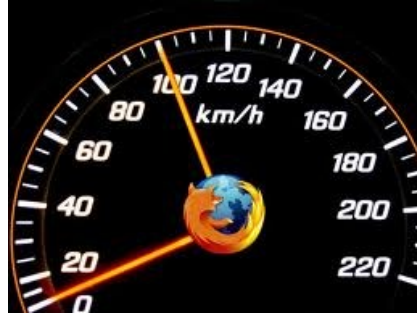
When the needle of a car speedometer is between the scale markings, we cannot estimate speed more accurately than to the nearest 2.5 km/h. This represents the resolution of the instrument.
