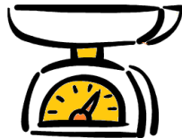
A scale giving a reading when no mass is placed has a zero drift
