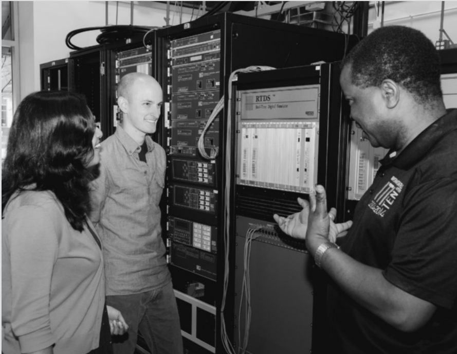
Power engineers with a Real Time Digital Simulator (RTDS) (Courtesy of Tim Yardley, University of Illinois.)
