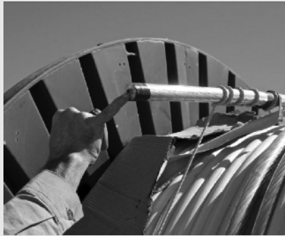
Figure 3 High-capacity low-sag conductor.
