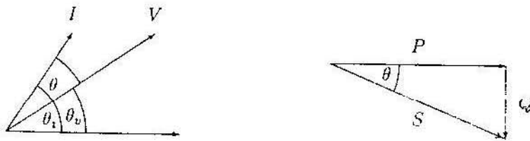
FIGURE 2.4 Phasor diagram and power triangle for a capacitive load (leading PF).
