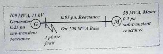
Q4. For the system shown in the figure, the line impedances are as indicated in per unit on 100MVA base.
