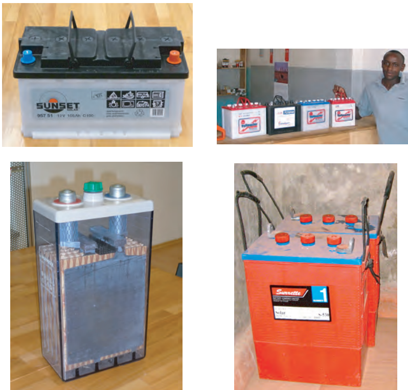
Figure 4.9 Types of battery: Sunset flat plate solar battery (top left); local Kenyan SLI batteries, not generally recommended but often the only option (top right); Hoppecke 2 volt cell, flooded, tubular plates, deep cycle, recommended for larger systems (bottom left); Surrette 6 volt batteries, deep cycle (bottom right)
