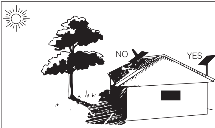
Figure 9.5 Module mounting site
