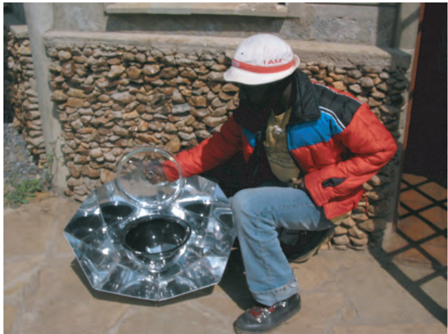
Figure 2.15 Solar cooker in Kenya, combining features of box and concentrator units
