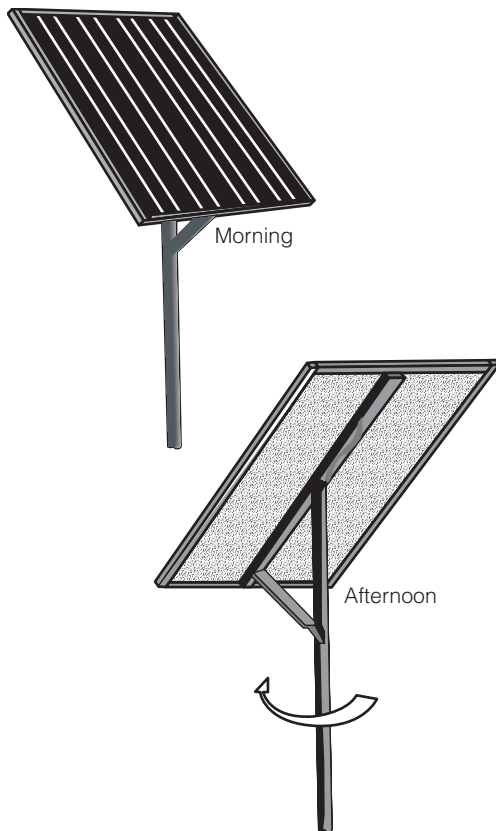
Figure 2.10 Simple manually turned pole-mounted solar tracker
