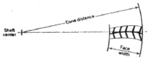
FIGURE 6.8 Diagram showing section through zerol pinion and gear teeth in mesh.
