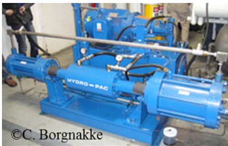
A hydraulic motor driven compressor, intercooler in pipe between the two stages.
