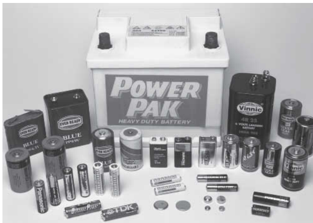
FIGURE 3.33 Examples of different types of batteries.
