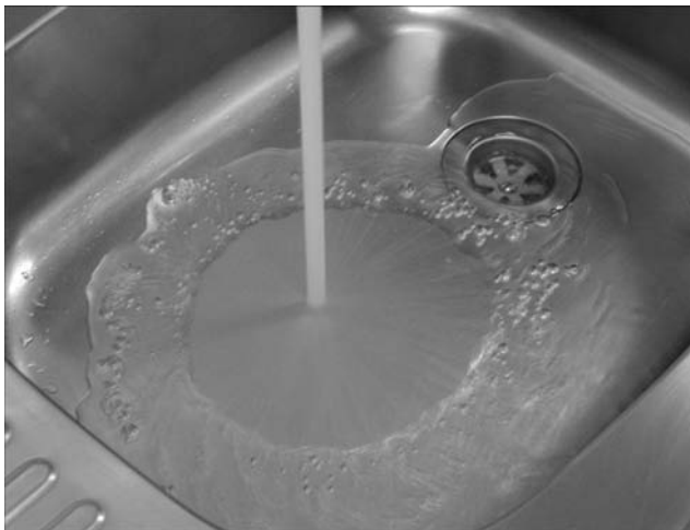
P10.92 A circular hydraulic jump in a kitchen sink. (Courtesy of Prof. Hubert Chanson, University of Queensland.)
