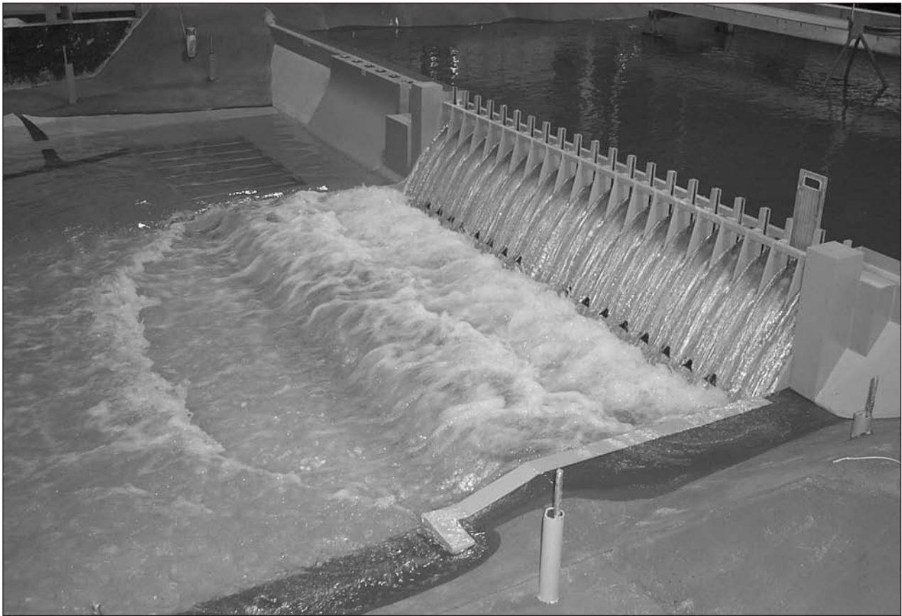
Fig. 5.9 Hydraulic model of the Bluestone Lake Dam on the New River near Hinton, West Virginia. The model scale is 1:65 both vertically and horizontally, and the Reynolds number, though far below the prototype value, is set high enough for the flow to be turbulent. (Courtesy of the U.S. Army Corps of Engineers Waterways Experiment Station.)
