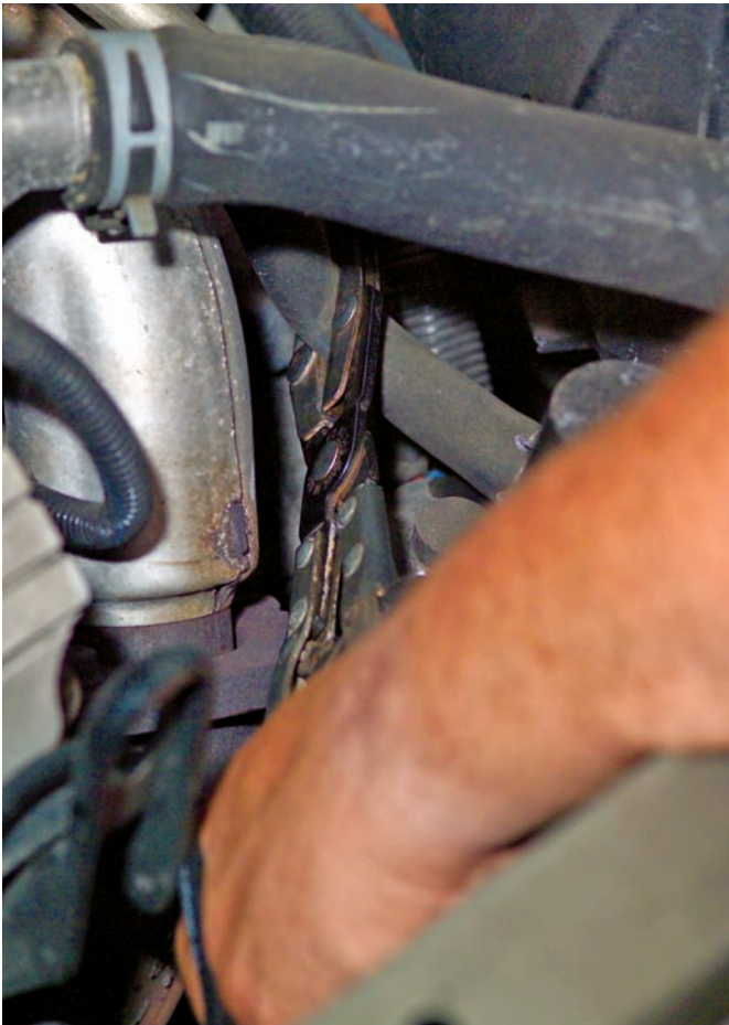
Figure 34-35 Before conducting an oxygen storage test, disable the air injection system.
