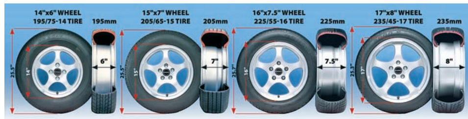
Figure 44-20 The effects of plus sizing. Courtesy of The Tire Rack
