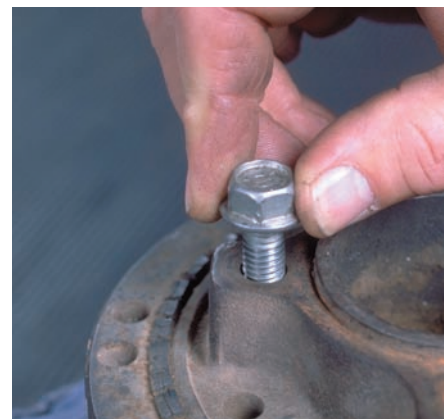
P1-9 Test the threads by threading the correct fastener into the threaded hole.
