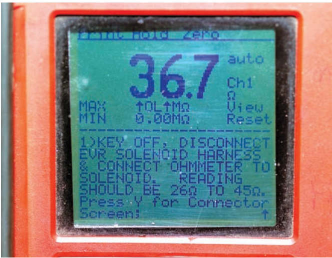
Figure 16-14 Some scan tools can also function as a multimeter and may display sensor specifications and instructions for further testing.
