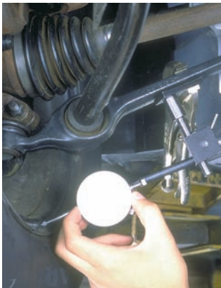
P48-3 Position a dial indicator against the inner edge of the rim at the bottom. Preload and zero the dial indicator.
