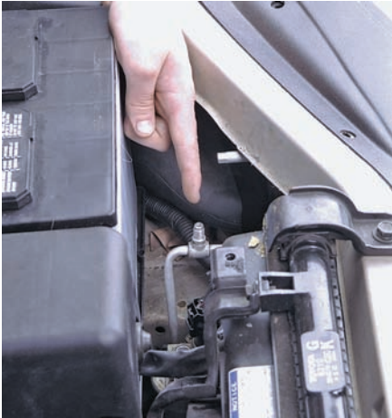
P53-1 Physically locate the pressure fittings of the system you will be working with. Make sure you have the proper adapters for the fittings prior to starting any service work on air-conditioning system.
