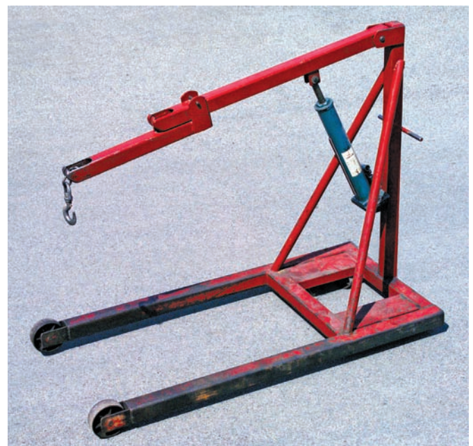
Figure 10-1 To pull an engine out of a vehicle, the chain on the lifting crane is attached to another chain secured to the engine.
