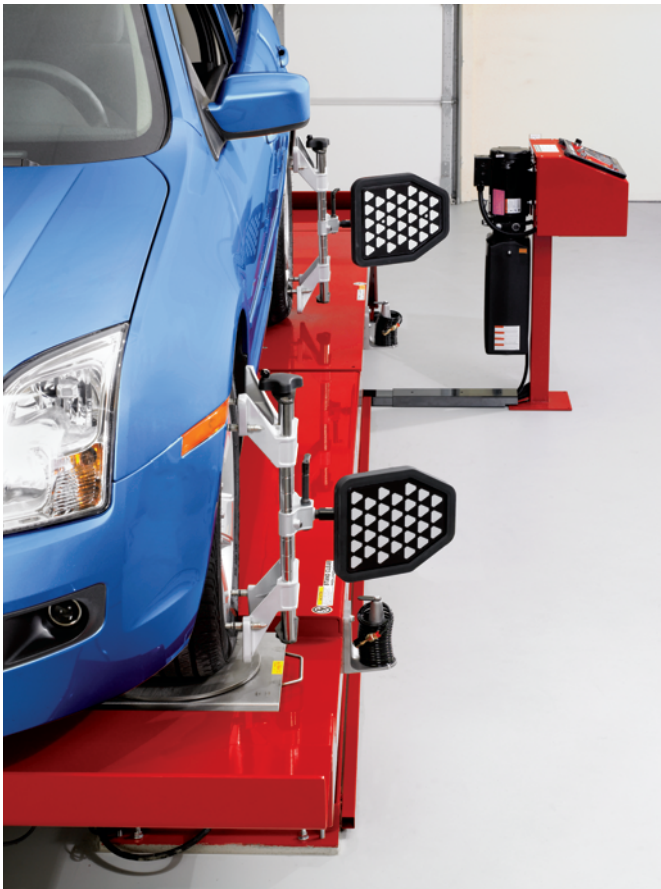
Figure 47-11 The sensors used to measure ride height with a wheel aligner. Courtesy of Hunter Engineering Company
