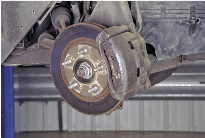
P52-3 Inspect the brake assembly. Look for signs of fluid leaks, broken or cracked lines, or a damaged brake rotor. If any problem is found, correct it before installing the new brake pads.
