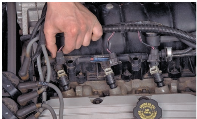
P32-6 Disconnect the wiring harness to the injectors by depressing the center of the attaching wire clip.
