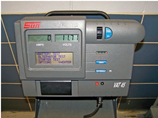
Figure 5-21 The volt/amp tester checks batteries and the starting and charging systems.
