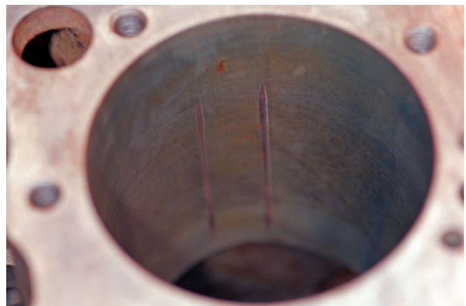
Figure 11-16 A scored cylinder wall.
