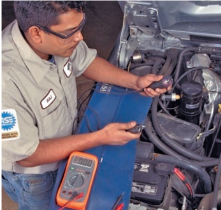
P15-1 The tools required to measure voltage drop at various points within the starter circuit are fender covers, a DMM, and a remote starter switch. Make sure to apply the parking brake and set the transmission into neutral or park.
