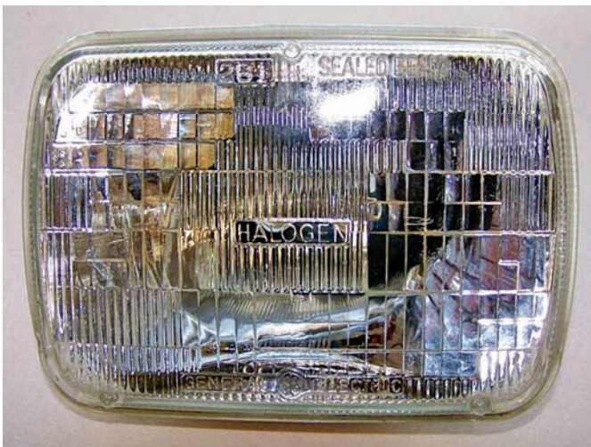
Figure 20-7 A sealed-beam halogen headlamp.
