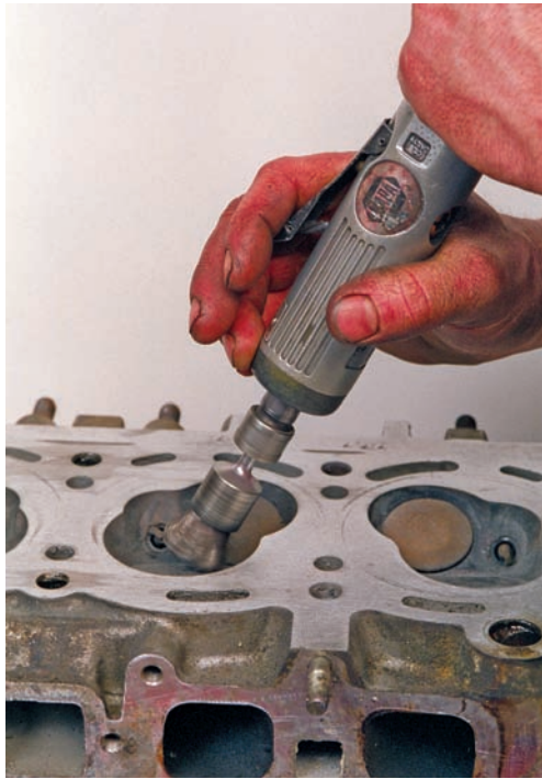
Figure 10-30 Carbon can be removed with a wire wheel driven by an electric or air drill motor.
