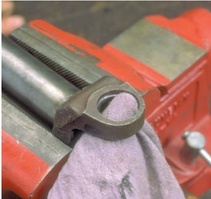
P39-1 Clean any dirt from the yoke and the retaining ring grooves.
