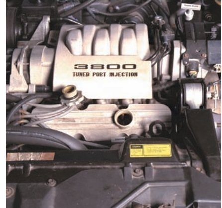
P3-12 With the oil filter and drain plug installed, lower the vehicle and remove the oil filler cap.
