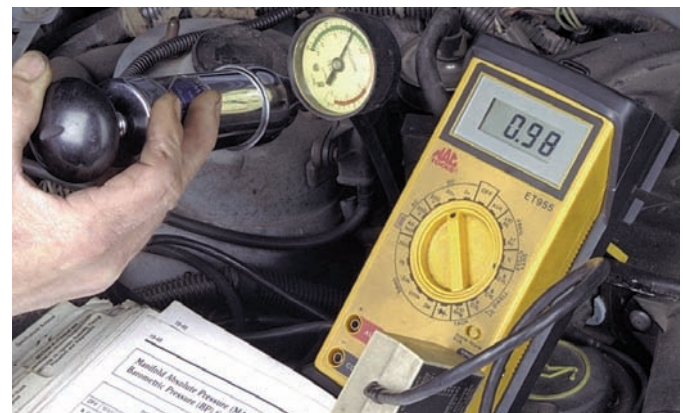
P25-9 Increase the vacuum to 20 in. Hg. Observe the voltage reading now and compare this to specifications. If the voltage signals from any of the tests do not match specifications, the MAP sensor needs to be replaced. Disconnect the tester and reconnect the electrical connector and vacuum hose to the MAP after you have completed your testing.
