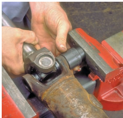
P38-5 Place the large socket against one vise jaw. Position the drive shaft yoke so that the socket is around a bearing cup.
