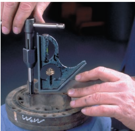
P1-4 Start the tap squarely in the threaded hole using a machinist square as a guide.
