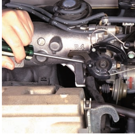
P6-2 Prop the throttle plate into a wide-open position to allow an unrestricted amount of air to enter the cylinders during the test.
