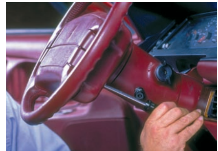
P22-9 Remove the four bolts that secure the module from the rear of the steering wheel.
