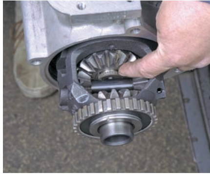
P43-11 Rotate the final drive unit until both ends of the output shaft retaining rings are showing.
