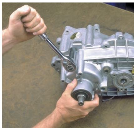
P44-8 Loosen and remove the front case to rear case retaining bolts.
