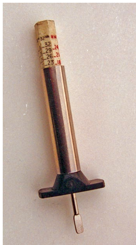
Figure 7-37 A tire tread depth gauge.
