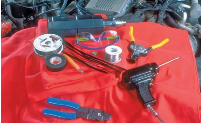
P13-1 Tools required to solder copper wire: 100-watt soldering iron, 60/40 rosin core solder, crimping tool, splice clip, heat shrink tube, heating gun, and safety glasses.
