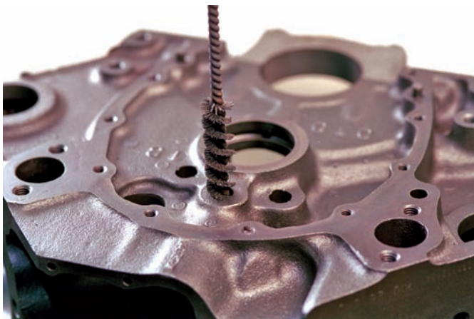
Figure 10-31 It is often necessary to remove the gallery plugs and hand clean the oil galleries.
