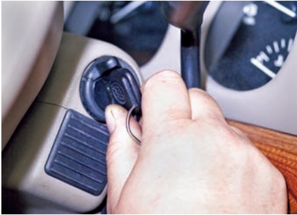
P28-1 Make sure the engine is at normal operating condition and the ignition switch is off.
