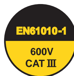
Figure 16-18 Only meters with this symbol should be used on the high-voltage systems in a hybrid vehicle; it is preferable that the equipment is rated at 1,000 V.
