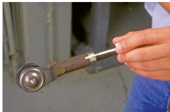
Figure 46-42 Before disassembling the steering gear, make an index mark on the outer tie-rod end, jam nut, and tie-rod.
