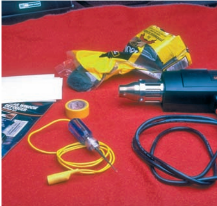
P21-1 The tools required to perform this task include masking tape, repair kit, 500°F heat gun, testlight, steel wool, alcohol, and a clean cloth.
