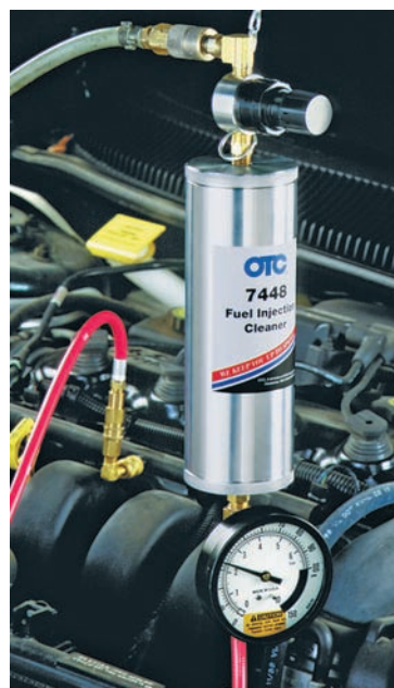
Figure 31-21 An injector cleaner connected to a fuel rail. Courtesy of SPX Service Solutions
