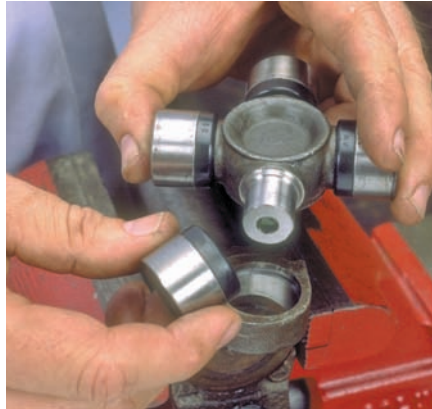
P39-2 Carefully remove the bearing cups from the new U-joint.
