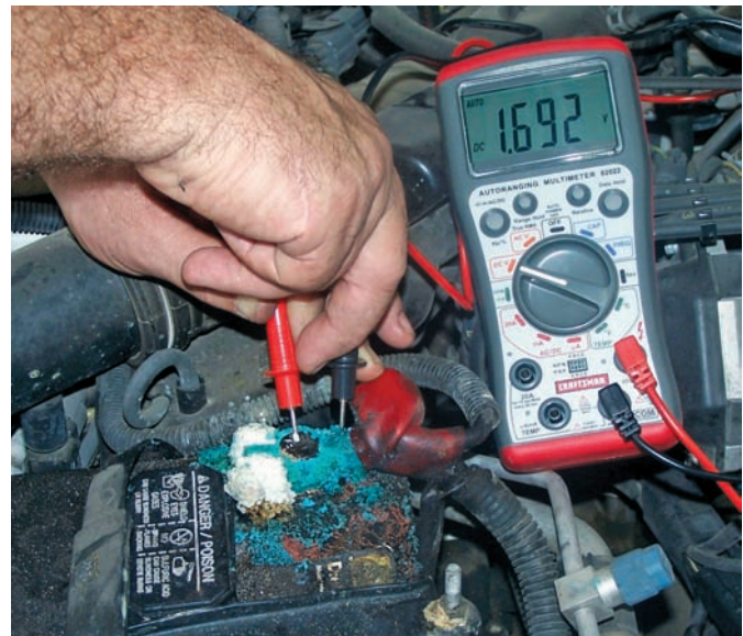
Figure 16-28 Measuring the voltage drop across the battery post and cable. It is easy to see why the voltage drop is high!
