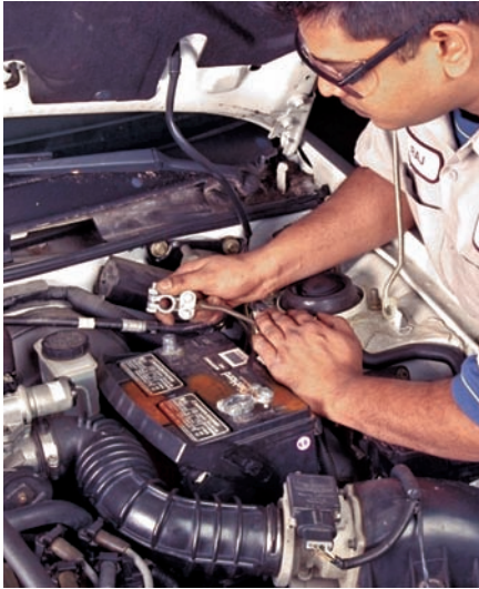
P10-1 Disconnect the negative cable from the battery prior to removing and replacing the timing belt.
