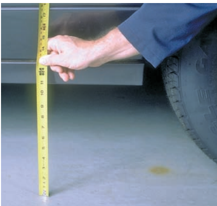
P47-7 Measure and record the right rear curb riding height.
