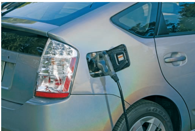
Figure 35–25 A plug-in hybrid being charged with an external power source. Courtesy of Toyota Motor Sales, U.S.A., Inc.
