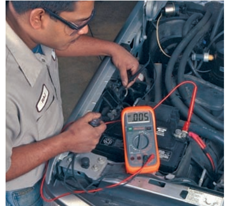
P15-10 Crank the engine and observe the reading on the meter. This is the voltage drop across the cable from the battery to the relay. Notice that hardly any voltage was dropped. This cable is okay.
