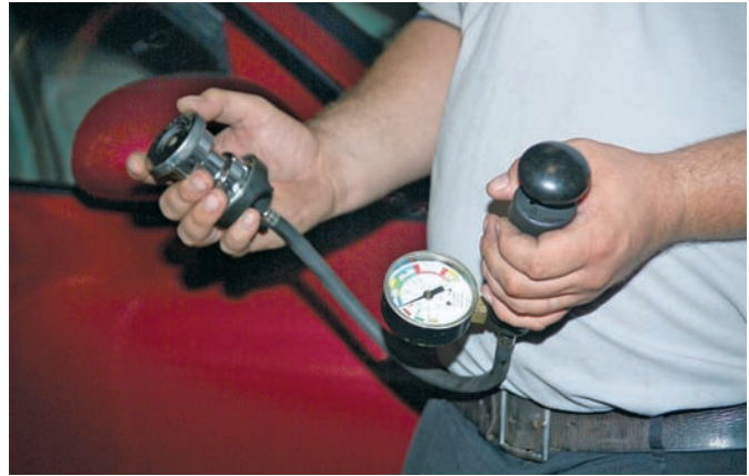
P11-6 Apply pressure to the cap that is equal to the cap's rating. If the cap does not hold that pressure, replace it. Then apply more pressure. If the cap is good, the excess pressure will vent through the cap.
