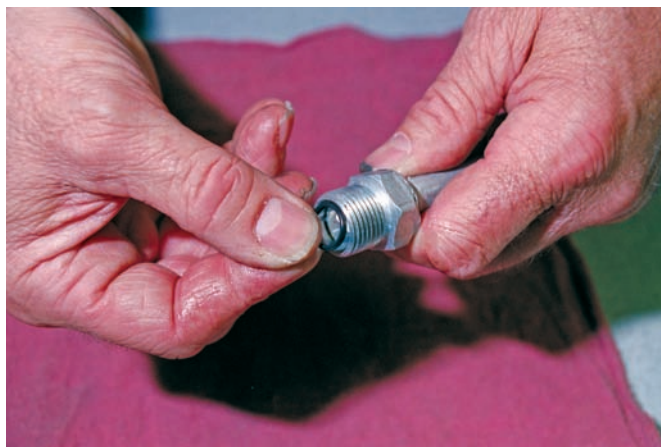
Figure 53-34 Always install a new O-ring when replacing an orifice tube.
