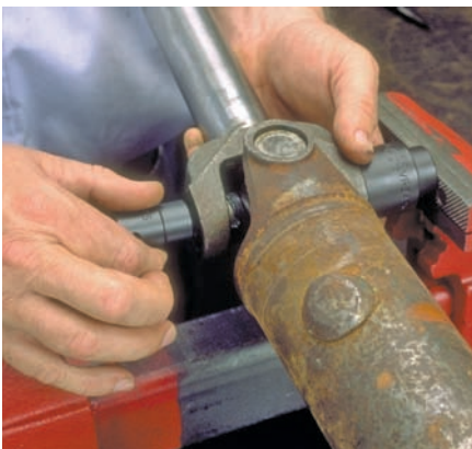
P38-4 Select a second socket that can slide into the shaft's bearing cup bore—usually a 5/16-inch socket.
