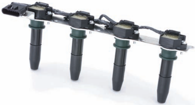
Figure 3-24 An ignition module and coil assembly for four cylinders.
