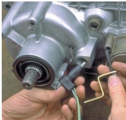
P44-5 Remove the speed sensor retaining bracket screw, bracket, and sensor.
