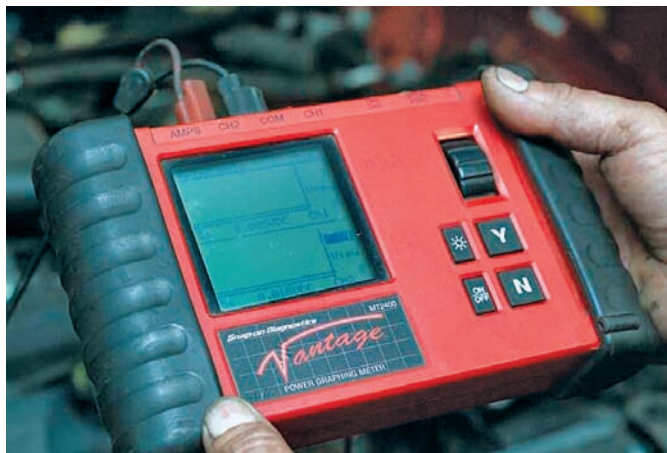
Figure 26-44 A two-channel GMM.
