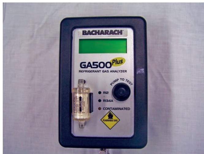
Figure 53-12 A refrigerant identifier.
