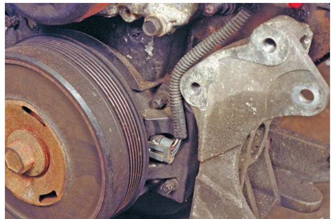
Figure 28-8 The wiring to the crankshaft sensor should be carefully inspected.
