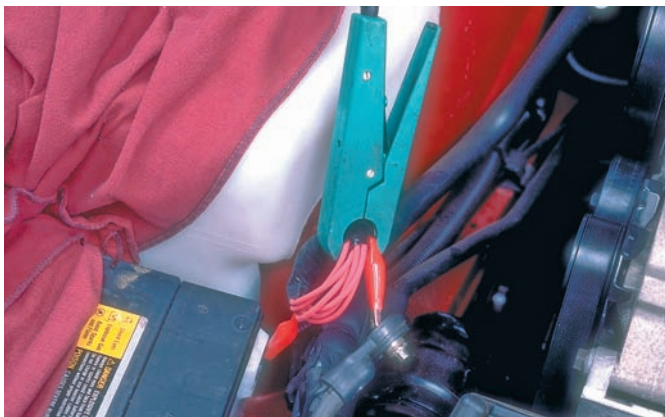
Figure 17-39 Using a multiplying coil to obtain accurate readings when measuring parasitic drains with a VAT-40 or similar tester.
