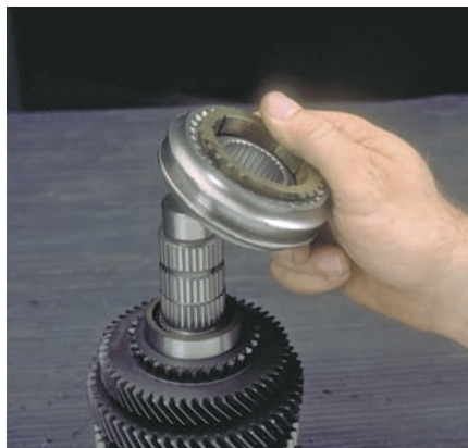
P35-17 Lift the assembly off the shaft. Then remove the remaining gears and synchronizer assembly as a unit.
