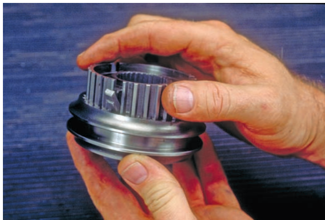
Figure 38-14 The movement of each synchronizer unit should be checked.
