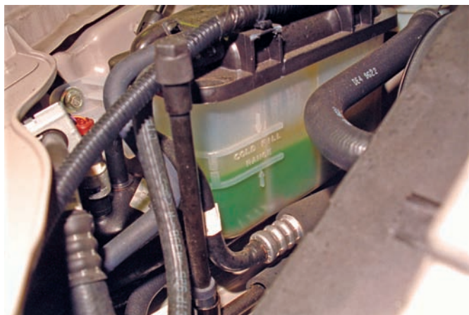
Figure 7-11 The level of coolant in the cooling system should be checked at the coolant recovery tank.
