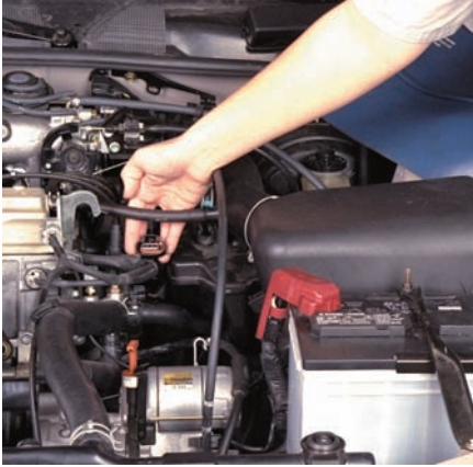
P6-1 Before conducting a compression test, disable the ignition and the fuel injection system. Most manufacturers recommend that the engine be warm when testing.
