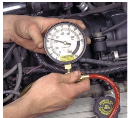
P30-8 To test the fuel pressure regulator, create a vacuum at the regulator with the vacuum pump. Fuel pressure should decrease as vacuum increases. If pressure remains the same, the regulator is faulty.
