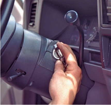
P24-1 Be sure the engine is at normal operating temperature and the ignition switch is off.
