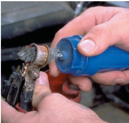
P5-13 Use a terminal cleaner brush to clean the battery cables.
