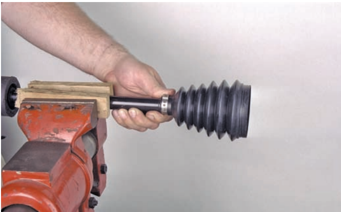
P37-13 Place the boot into its proper location on the shaft and install a new clamp.
