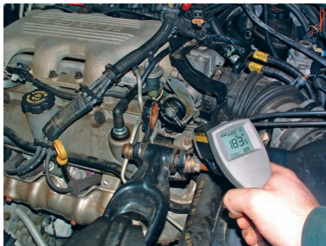
Figure 14-43 The operation of a thermostat can be observed with an infrared thermometer.
