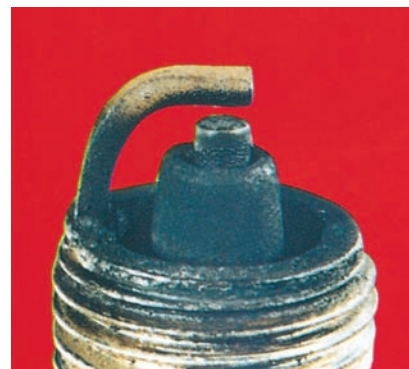
Figure 28-54 A cold- or carbon-fouled spark plug. Courtesy of Federal-Mogul Corporation
