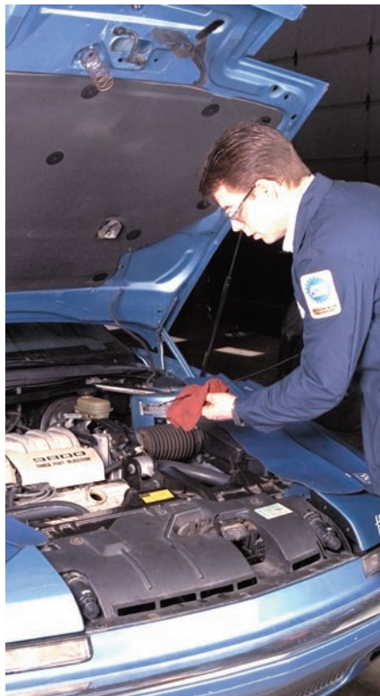
P3-14 After the recommended amount of oil has been put in the engine, check the oil level.
