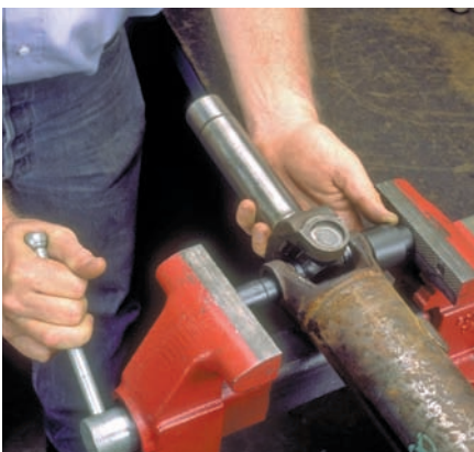
P38-7 Carefully tighten the vise to press the bearing cup out of the yoke and into the large socket.
