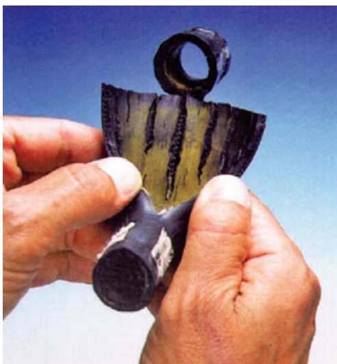
Figure 14-41 An ECD-damaged hose. Courtesy of Gates Corporation
