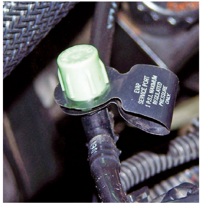
Figure 34-17 An EVAP service port.
