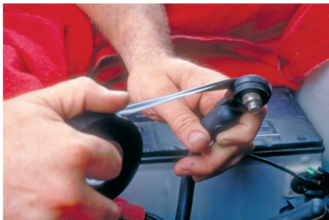
Figure 10-3 After the negative battery cable is disconnected, tape the terminal end to prevent it from accidentally touching the battery.
