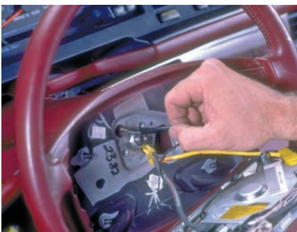
P22-10 Rotate the horn lead \frac{1}{4} turn and disconnect.
