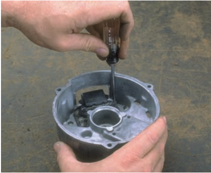
P17-10 Using the torx wrench, remove the four attaching bolts that hold the rectifier bridge.
