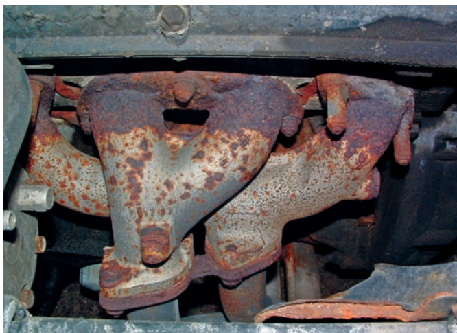
Figure 10-11 The exhaust system must be disconnected to remove the engine. Often this is the condition of the exhaust, so take care not to damage anything.
