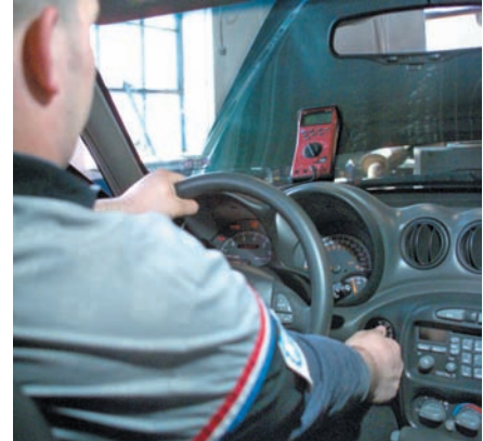
P26-3 Place the meter where you can see it from the driver's seat.
