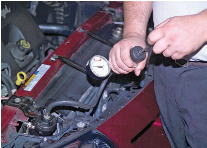
P11-3 Connect the tester to the radiator's filler tube and apply pressure to the system by pumping the handle of the tester.
