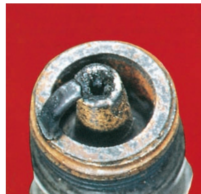
Figure 28-59 A spark plug with preignition damage. Courtesy of Federal-Mogul Corporation
