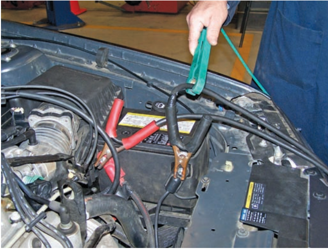
P14-5 Clamp the tester's inductive lead around the tester's negative cable. Normally the arrow on the clamp should face away from the negative post of the battery.
