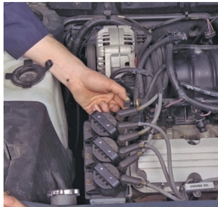
P30-4 Most fuel rails are equipped with a test fitting that can be used to relieve pressure and to test pressure.
