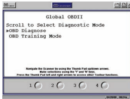
P23-2 After the tool enters into the generic OBD-II mode, select Diagnose to check the system.
