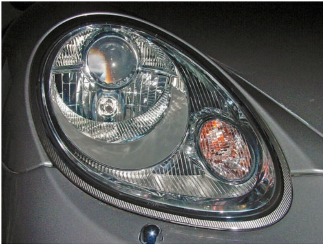
Figure 20-9 A headlamp assembly with cylindrical bulb housings.
