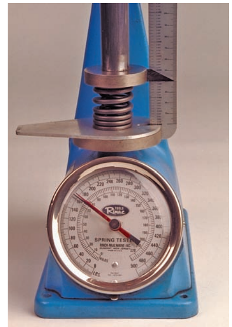
P9-12 Compare this reading to specifications. Any pressure outside the pressure range given in the specifications indicates that the spring should be replaced. After the tension and height have been checked, the spring can be installed on the valve stem.
