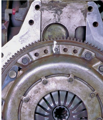
P34-2 Before disassembling the clutch, make sure alignment marks are present on the pressure plate and flywheel.
