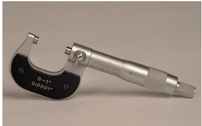
P2-4 The graduations on the thimble assembly define the area between the lines on the sleeve. The number indicated on the thimble is added to the measurement shown on the sleeve.
