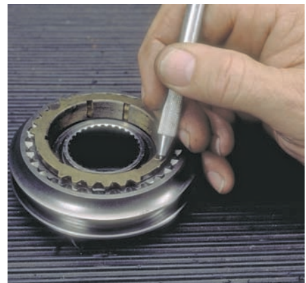
P35-18 Separate the synchronizer's hub, sleeve, and keys, noting their relative positions and scribing their location on the hub and the sleeve prior to separation.
