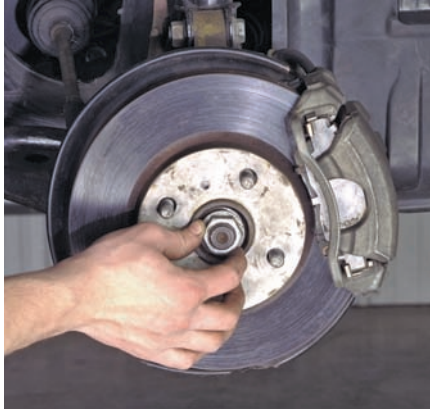
P37-2 After the car is raised and the wheel is removed, the hub nut can be unscrewed from the axle shaft.
