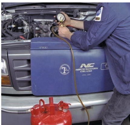
P29-5 Install the free end of the gauge bleed hose into an approved gasoline container, and open the gauge bleed valve to relieve the fuel pressure.
