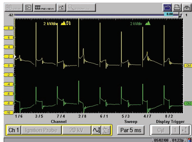
Figure 28-27 Typical parade (display) patterns for the primary and secondary circuits. Reproduced under license from Snap-on Incorporated. All of the marks are marks of their owners.
