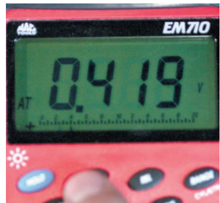
P26-9 Press the Min/Max button again to read the average voltage. This reading should be about 0.45 volt. Repeat this test at different speeds to get a good look at how well the O 2 sensor responds.
