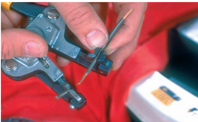
P13-5 Now remove about 1/2 inch of the insulation from both ends of the replacement wire. The length of the replacement wire should be slightly longer than the length of the wire removed.
