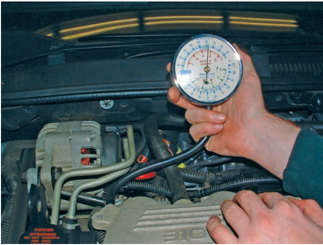
Figure 9-41 The vacuum gauge is connected to the intake manifold where it reads engine vacuum.
