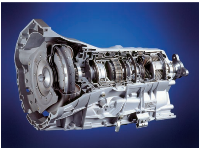
Figure 3-32 A cutaway of a six-speed automatic transmission shown with the torque converter in the housing. Courtesy of BMW of North America, LLC
