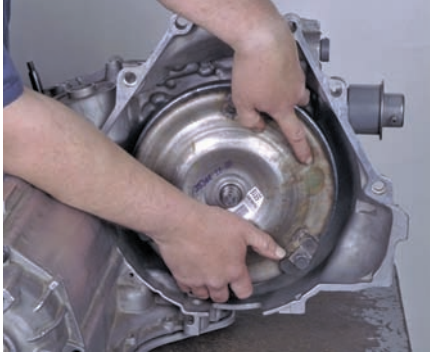
P43-1 Remove the torque converter. Then place the transaxle in a holding fixture. Remove the speedometer sensor and governor assembly.
