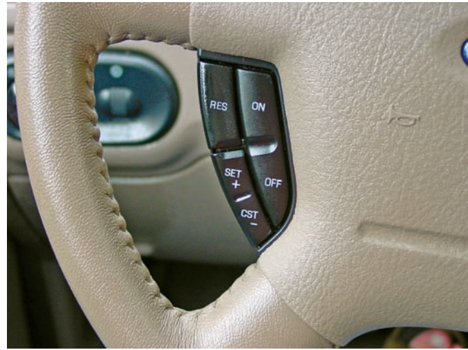
Figure 23-15 The cruise control switch is used to set or increase speed, resume speed, or turn the system off and on.
