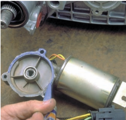
P45-13 Apply a thin bead of sealer to the mating surface of the electric shift motor.
