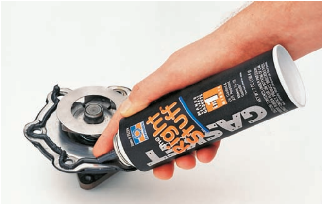
Figure 13-28 Applying a bead of RTV gasket material on a water pump. Courtesy of Loctite Corporation
