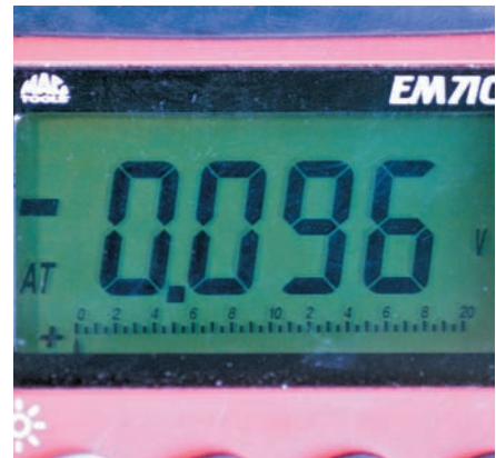
P26-6 Restart the engine and allow it to reach normal operating temperature. Look at the meter to make sure the sensor's signal is toggling from low to high voltage.
