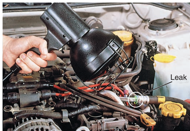
Figure 53-19 A fluorescent dye is added to the system before checking for leaks with the black light. Courtesy of Tracer Products
