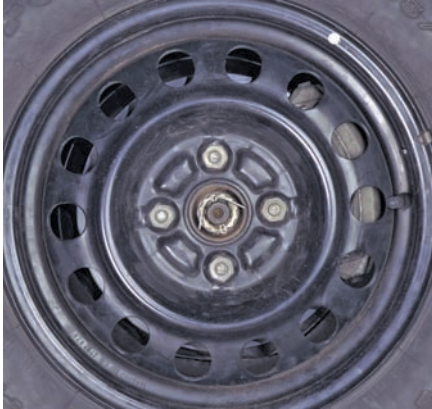
P37-1 Removing the axle from the car begins with the removal of the wheel cover and wheel hub cover. The hub nut should be loosened before raising the car and removing the wheel.
