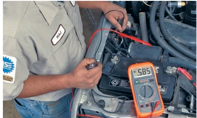
P15-12 Crank the engine and observe the reading on the meter. This is the voltage drop across the contacts inside the relay.
