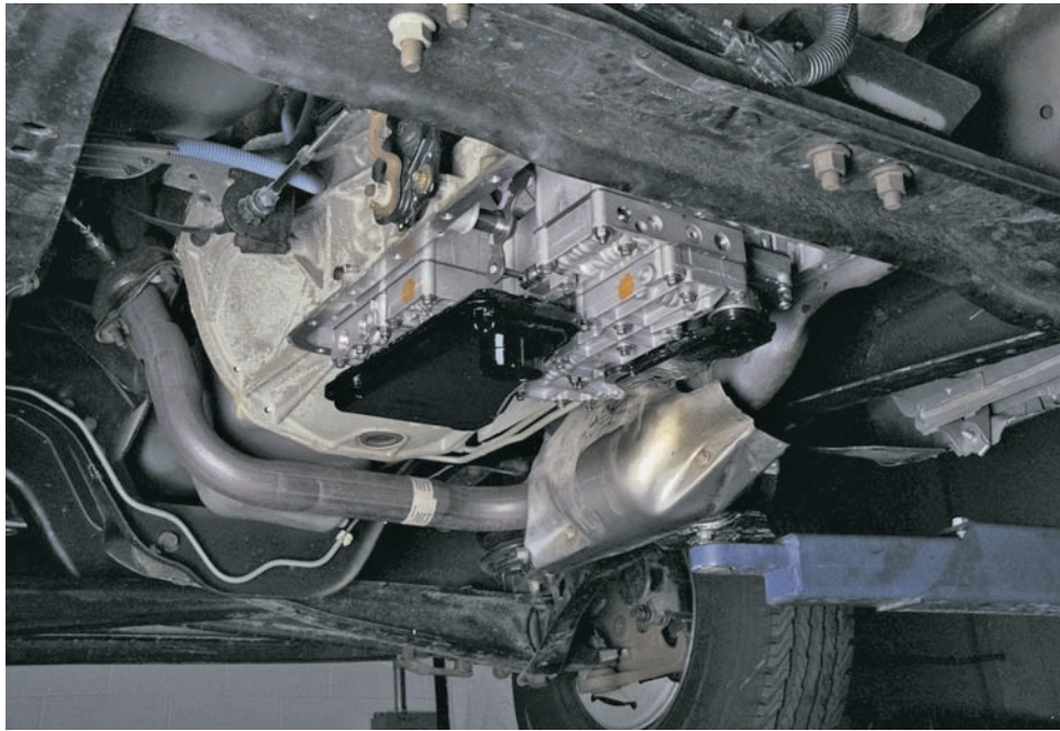
Figure 42-2 Transmission fluid filters are attached to the transmission case by screws, bolts, retaining clips, and/or by the pickup tube.
