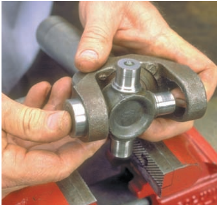
P39-4 Start one cup into the yoke's ear and over the cross's trunnion.
