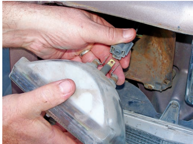
Figure 20-24 After unplugging the old bulb, check and clean the contacts in the connector before installing the new bulb.
