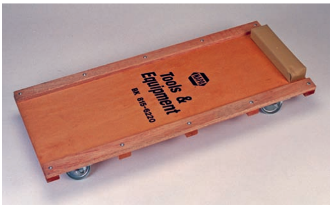
Figure 4-56 A creeper allows you to work comfortably and safely under a vehicle.
