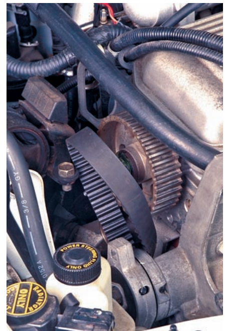
P10-6 Slide the belt off the crankshaft sprocket. Do not allow the crankshaft pulley to rotate while doing this.
