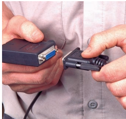
P24-5 Select the proper scan tool adapter for the vehicle's DLC.
