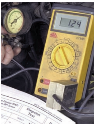
P25-7 Apply 10 in. Hg to the MAP sensor. Observe the voltage reading now and compare this to specifications.
