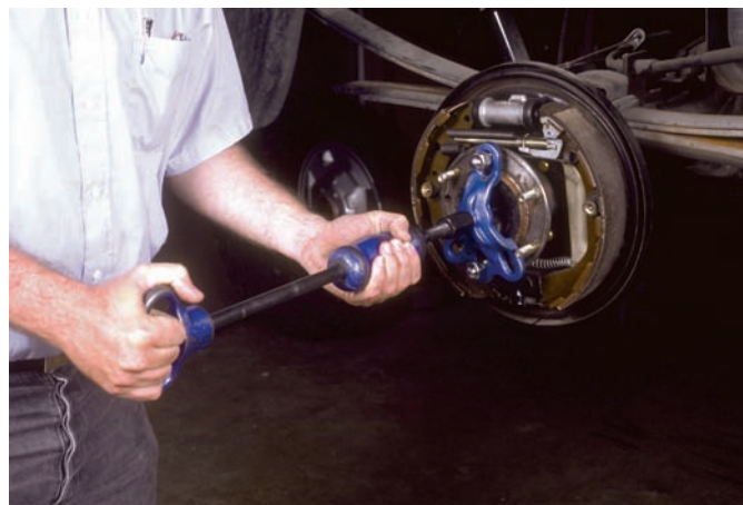
Figure 4-54 Using a slide hammer-type puller to remove a drive axle.
