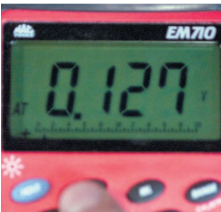
P26-7 Press the Min/Max button on the meter and observe the voltage. This reading will be the minimum voltage and should be about 0.1 volt.
