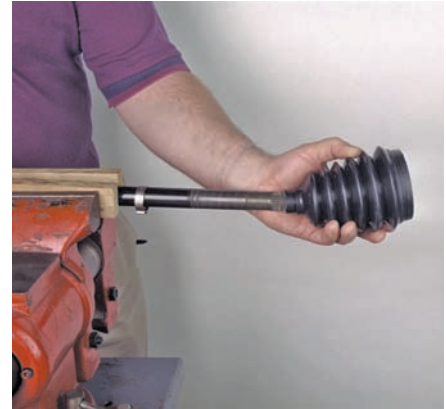
P37-12 Clean and inspect the joint, then wipe the axle shaft clean and install the new boot onto the shaft.
