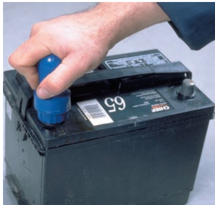
P5-14 Use a terminal cleaner brush to clean the battery posts.
