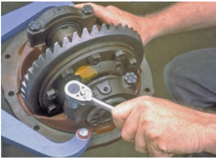
P41-4 Snugly tighten the top bearing cup bolts and finger tighten the lower bolts.
