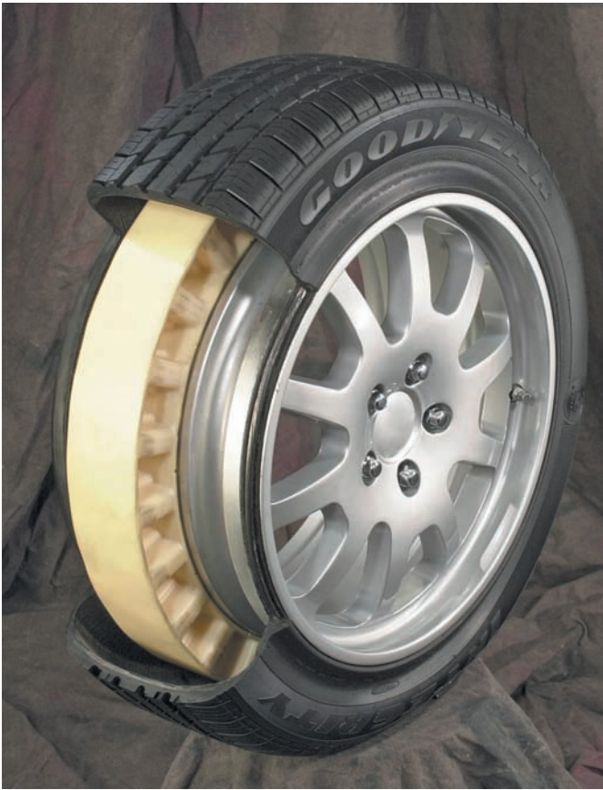
Figure 44-8 A cutaway of a run-flat tire with an insert for support in case the tire goes very flat. Courtesy of The Goodyear Tire & Rubber Company
