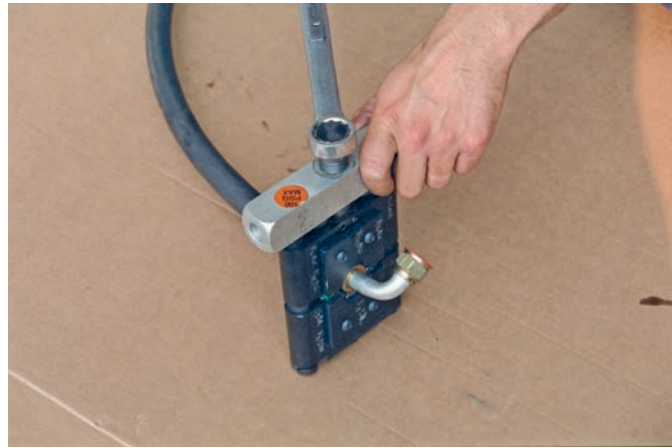
Figure 53-29 The ferrule is crimped with a special crimping tool.
