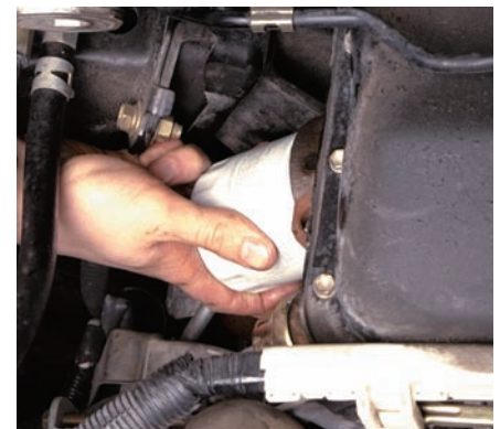
P3-9 Install the new filter and hand-tighten it. Oil filters should be tightened according to the directions given on the filter.
