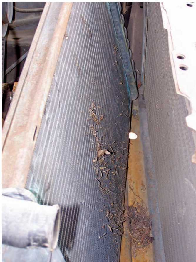
Figure 7-10 A buildup of dirt and bugs can restrict airflow through the radiator.
