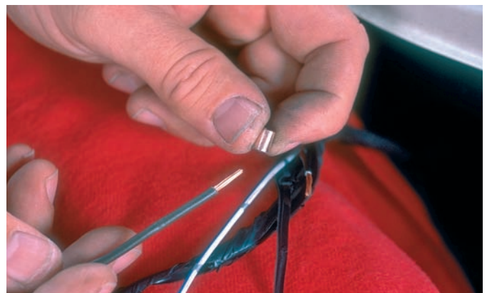
P13-6 Select the proper size splice clip to hold the splice.
