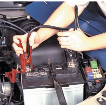
P6-7 Connect a battery charger to the car to allow the engine to crank at consistent and normal speeds needed for accurate test results.
