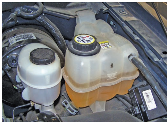
Figure 14-26 A coolant expansion tank.
