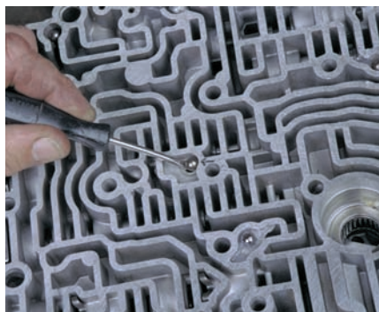
P43-8 Mark the location of and remove all of the check balls between the spacer plate and the valve body and between the channel plate and the spacer plate.
