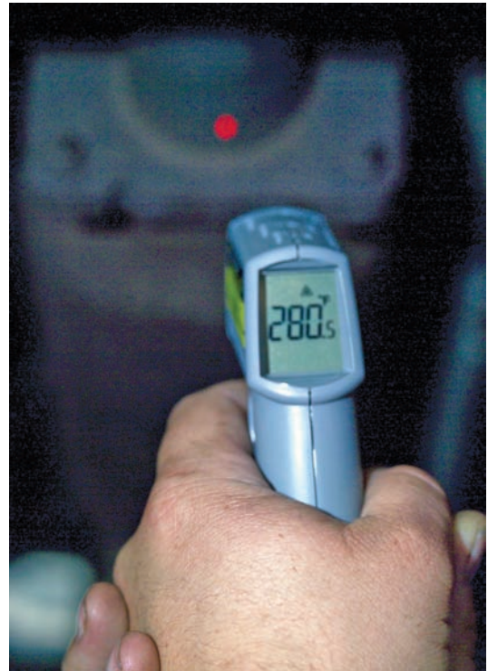
Figure 34-33 When doing the delta temperature test, check the temperature of the converter.
