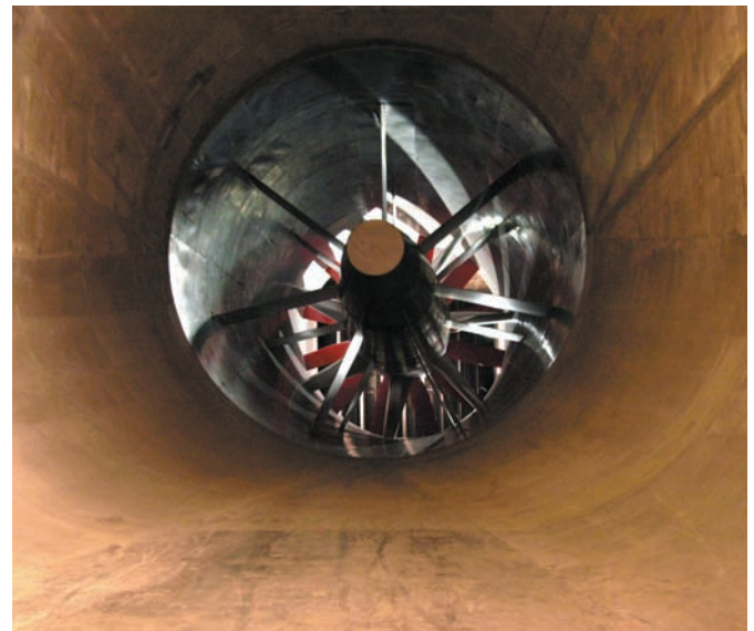
Figure 8-24 This wind tunnel can generate winds as high as 150 miles per hour. Courtesy of Chrysler LLC
