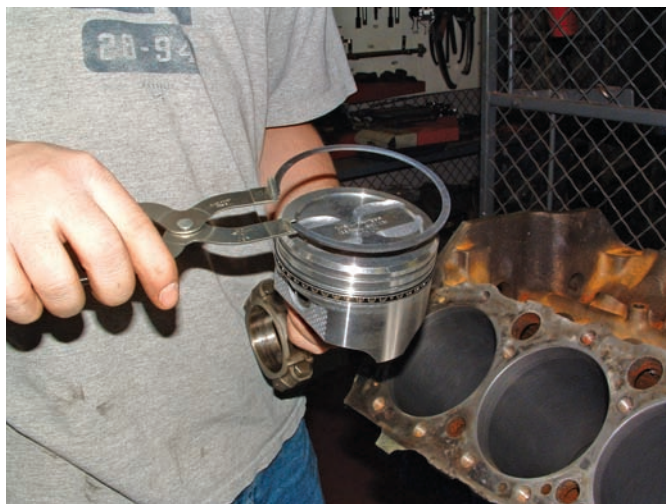
Figure 11-63 Use a ring expander to install the compression rings.
