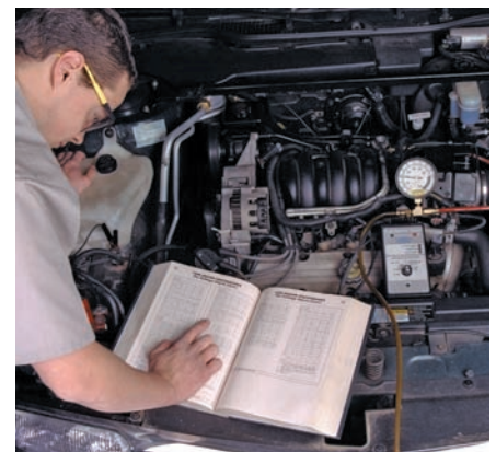
P31-9 Depress the switch on the tester to activate that injector and record the pressure drop. Continue the procedure for all injectors, then compare the results of each to specifications and to each other.
