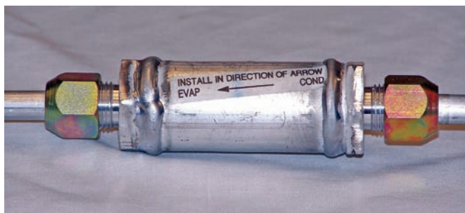
Figure 53-27 An inline filter.
