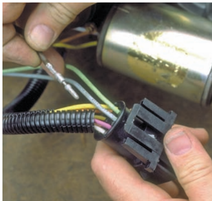
P44-4 Remove the wires from the electronic shift harness connector. Record the exact location of each disconnected wire.
