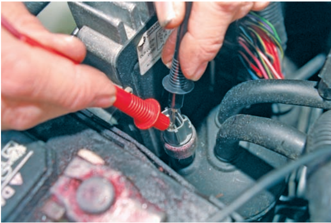
Figure 53-28 All sensors and switches can be checked with an ohmmeter.
