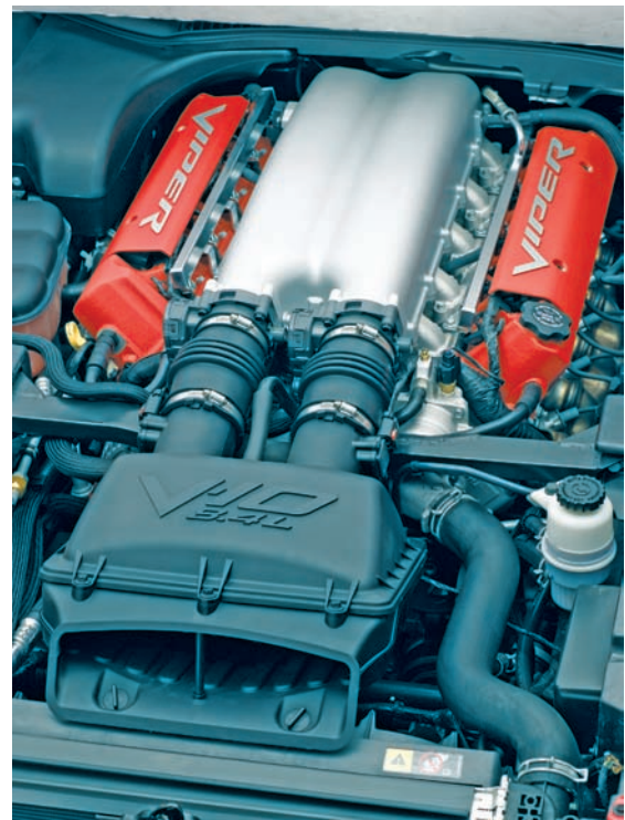
Figure 3-22 The intake system for a V-10 in a Dodge Viper. Courtesy of Chrysler LLC
