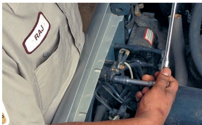
P15-13 The reading is higher than normal; therefore, the starter relay has high resistance and needs to be replaced.
