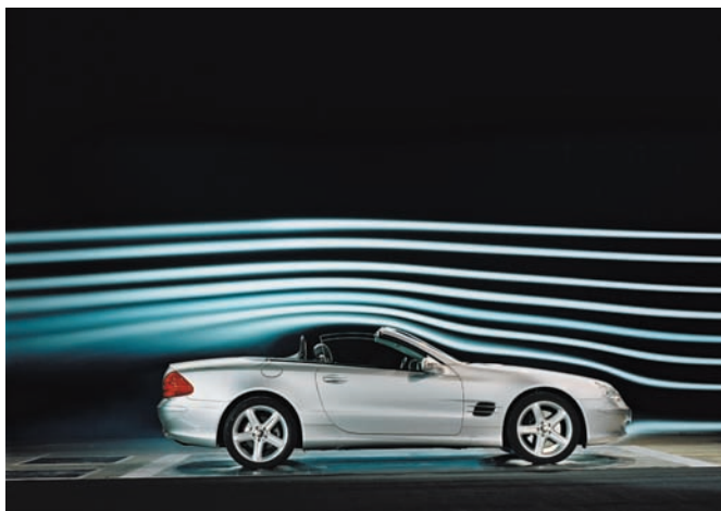
Figure 8-23 The movement of air as it goes over this car. Courtesy of Chrysler LLC
