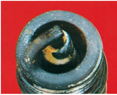
Figure 28-56 A splash-fouled spark plug. Courtesy of Federal-Mogul Corporation
