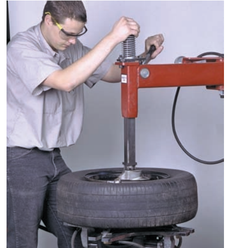
P46-3 Lower the machine's arm into position on the tire and wheel assembly.
