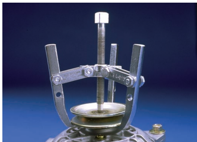
Figure 4-55 The jaws on this puller are reversible to allow for inside and outside pulls.
