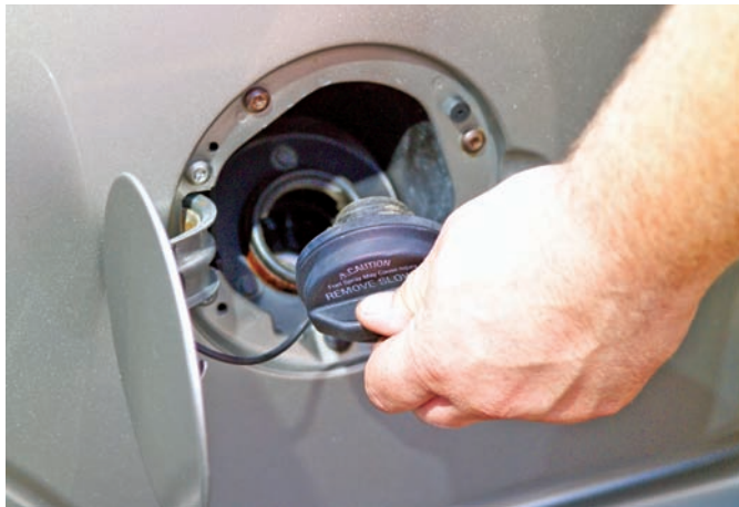
Figure 29-10 The gas cap for current vehicles is tethered to the vehicle and threaded into the filler tube.
