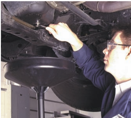
P3-4 Loosen the drain plug with the appropriate wrench. After the drain plug is loosened, quickly remove it so the oil can freely drain from the oil pan.
