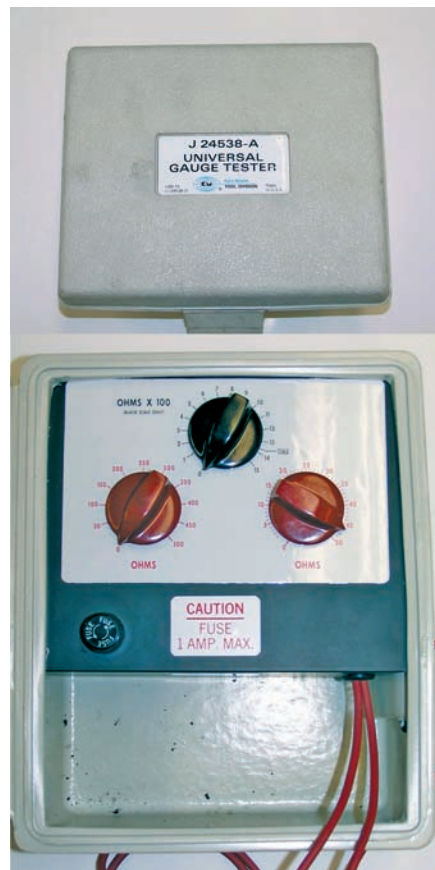
Figure 21-14 A universal gauge tester.
