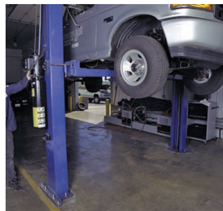
P29-6 Place the vehicle on the hoist and position the lift arms according to manufacturer's recommendations. Then raise the vehicle.
