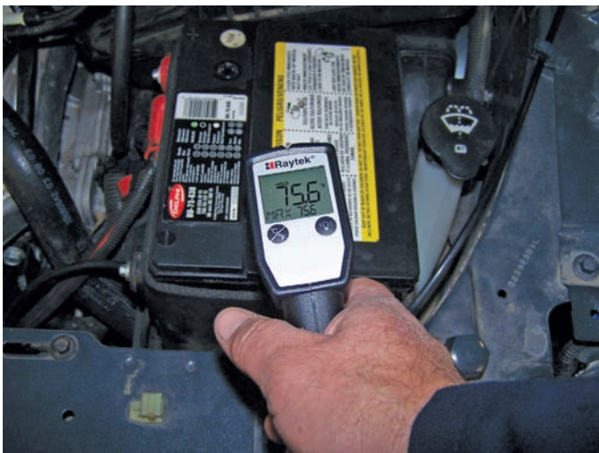
P14-3 Check the temperature of the battery; it should be around 70°F (21°C).
