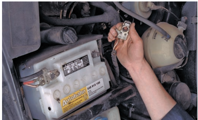
P32-4 As an extra precaution, many technicians disconnect the negative cable at the battery.
