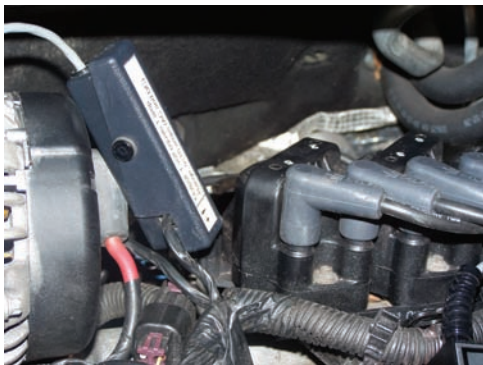
P27-5 Install the probe around the ignition feed at the ignition module.
