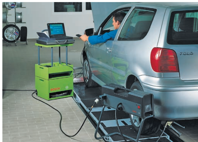
Figure 33-5 Emission levels are commonly checked with the vehicle running on a dyno. Courtesy of Robert Bosch GmbH, www.bosch-presse.de
