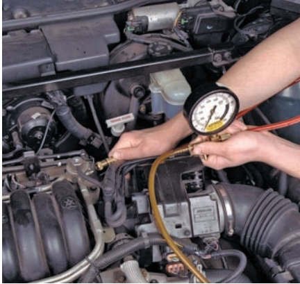
P31-1 Connect the fuel pressure gauge to the Schrader valve on the fuel rail, and then relieve the pressure in the system.
