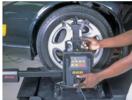
P50-4 Attach the wheel units. Make sure the wheel is raised before attaching an electronic wheel unit.
