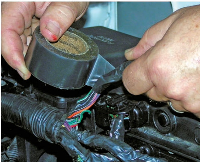
Figure 16-69 Tape all wire repairs to prevent corrosion and damage.
