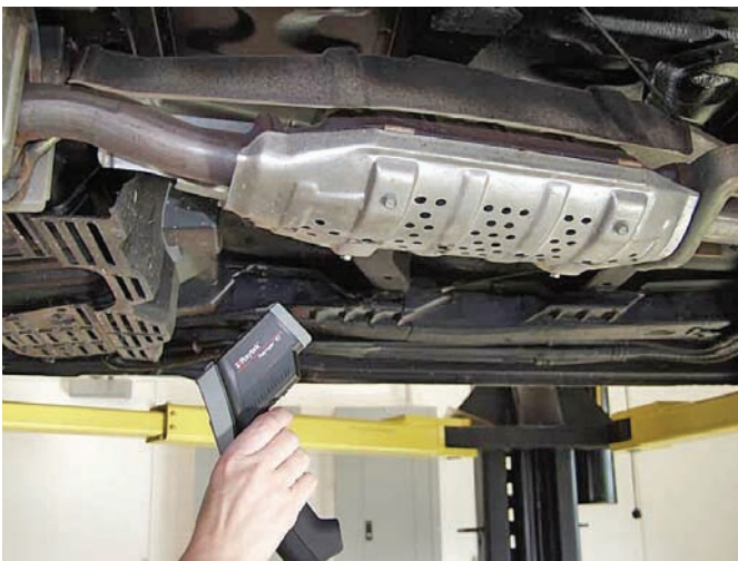
Figure 32-30 An infrared thermometer can be used to check the effectiveness of a catalytic converter.
