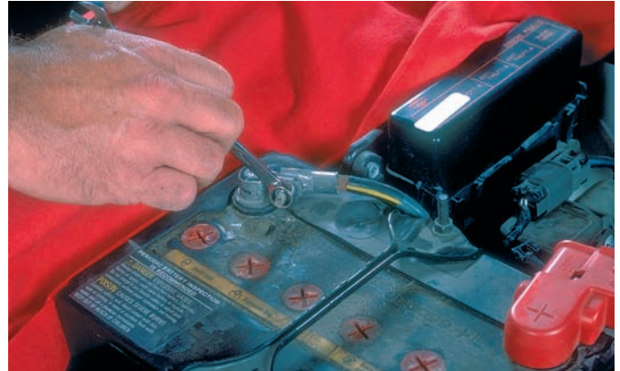
P13-2 Disconnect the fuse that powers the circuit being repaired. Note: If the circuit is not protected by a fuse, disconnect the ground lead of the battery.
