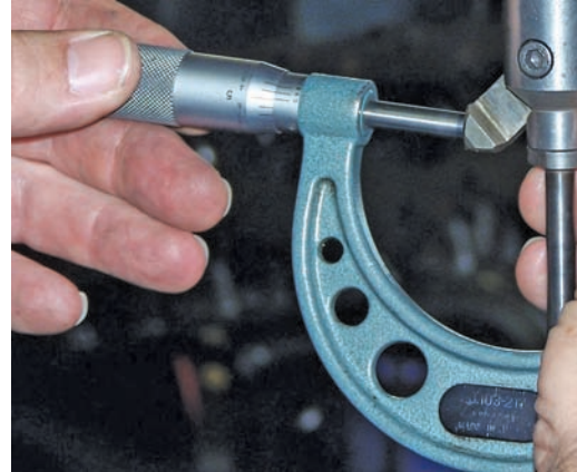
Figure 12-72 Using an outside micrometer to expand the cutter head to allow for an interference fit between the bore and the new valve seat.
