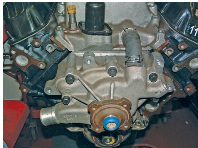
Figure 14-19 A water pump bolted to the front of an engine.
