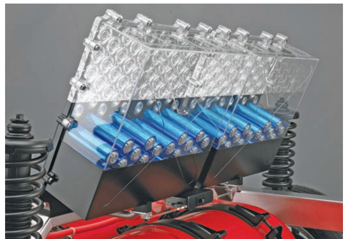
Figure 22-3 A super- or ultracapacitor assembly. Courtesy of American Honda Motor Company, Inc.
