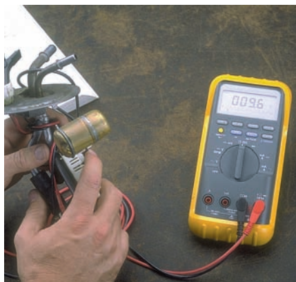
P19-8 Check the resistance value while holding the float against the full stop. Check the results with the specifications.
