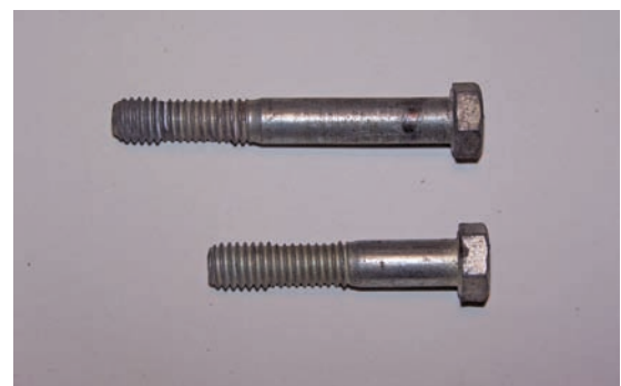
Figure 13-2 These bolts have been torqued beyond their yield. Note the soda bottle effect.
