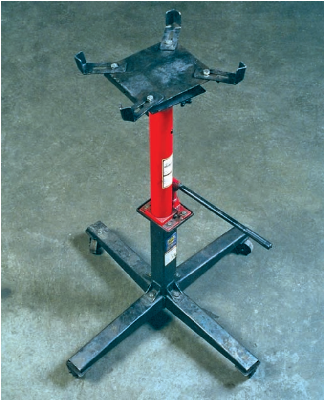
Figure 5-47 A typical transmission jack.
