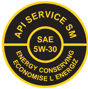
Figure 7-7 The SAE classification and the API rating are displayed in this way on a container of oil.
