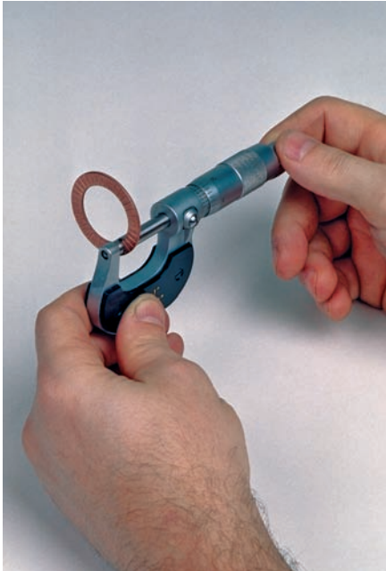
P9-7 If measured installed height is greater than the specifications, a valve shim must be placed under the spring to correct the difference.
