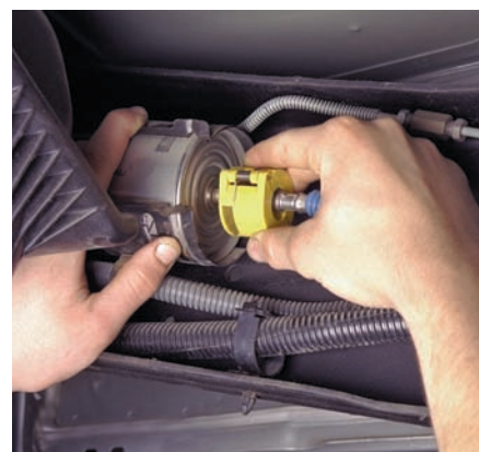
P29-9 Follow the recommended procedures for disconnecting the fuel outlet connector. Then remove the fuel filter.
