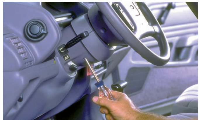
P18-4 Remove the shroud retaining screws and remove the lower shroud from the steering column.
