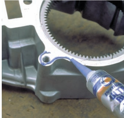
P45-2 Apply a thin bead of sealer around the ring gear housing.
