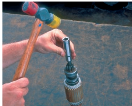
P16-11 Place a \frac{5}{8} -inch deep socket over the armature shaft until it contacts the retaining ring of the starter drive.
