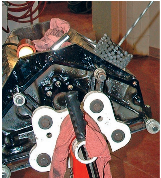
Figure 11-22 Using a resilient-based, hone-type brush, commonly called a ball hone.
