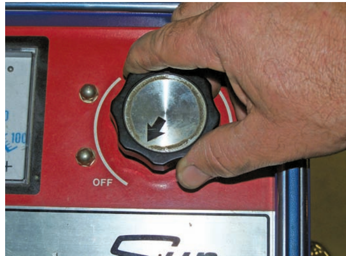
P14-8 After 15 seconds, read the voltage of the battery and turn the load control off. Then disconnect the tester's leads.
