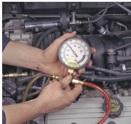
P30-7 Turn the ignition switch to the run position and observe the fuel pressure gauge. Compare the reading to specifications. A reading lower than normal indicates a faulty fuel pump or fuel delivery system.
