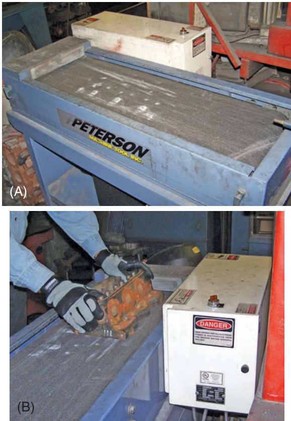
Figure 12-55 (A) A typical belt sander and (B) how it is used.
