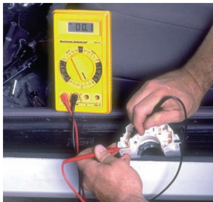
P18-15 With the switch in the high-beam position, there should be continuity across the high-beam circuit. Also check for continuity across the other circuits that should be open when the switch is in the high-beam position.
