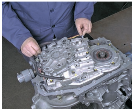
P43-41 Connect and install the wiring harness to the pressure switches, solenoids, and case connector. Then install the side covers and gaskets. Tighten the bolts to the specified torque.
