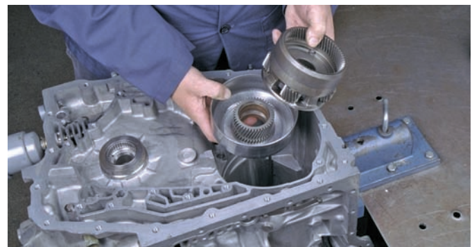
P43-17 Remove the reaction carrier, reaction sun gear/drum assembly, and forward band.
