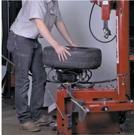
P46-2 Once both sides of the tire are unseated, place the tire and wheel onto the machine. Then depress the pedal that clamps the wheel to the tire machine.
