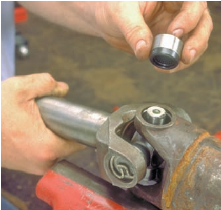
P38-1 Clamp the slip yoke in a vise and support the outer end of the drive shaft.
