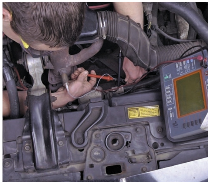
Figure 26-42 The correct way to connect a lab scope to an oxygen sensor.
