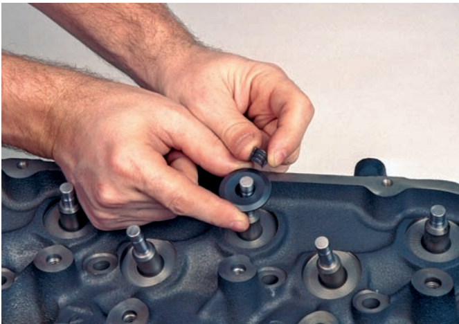
P9-3 Install the valve retainer and keepers. Without the spring, these must be held in place.
