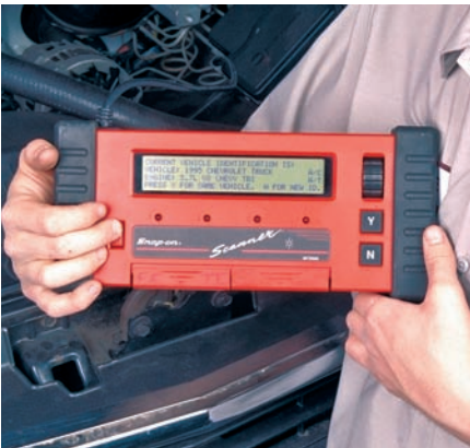
P24-4 Enter the vehicle's model year and VIN code into the scan tool.
