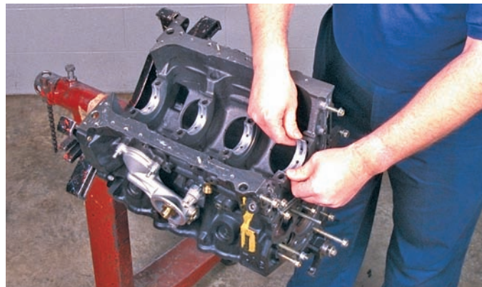
P7-2 Install main bearings into bores, being careful to properly seat them. Wipe the bearings with a clean lint-free rag.
