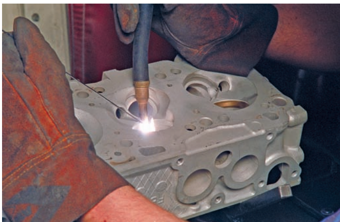
Figure 12-54 TIG welding an aluminum head.
