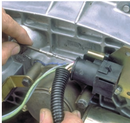
P45-17 Reinstall the wires into the connector and connect all electric sensors.
