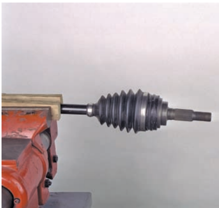
P37-7 The axle shaft should be mounted in a soft-jawed vise for work on the joint. Pieces of wood on either side of the axle work well to secure the axle without damaging it.
