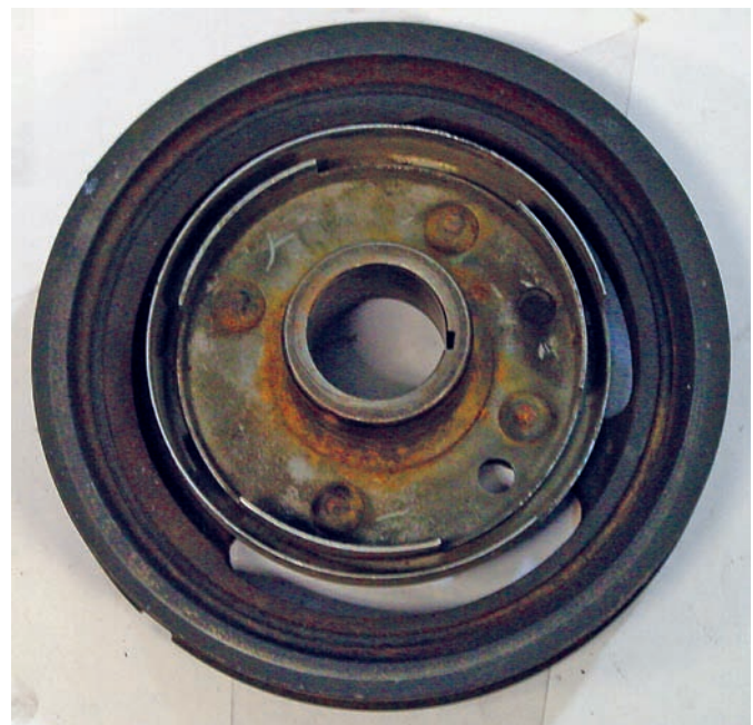
Figure 27-33 This crankshaft pulley for a six-cylinder engine has two sets of interrupter rings.
