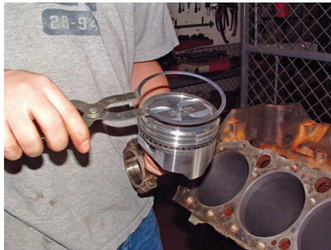
Figure 5-9 A piston ring expander.
