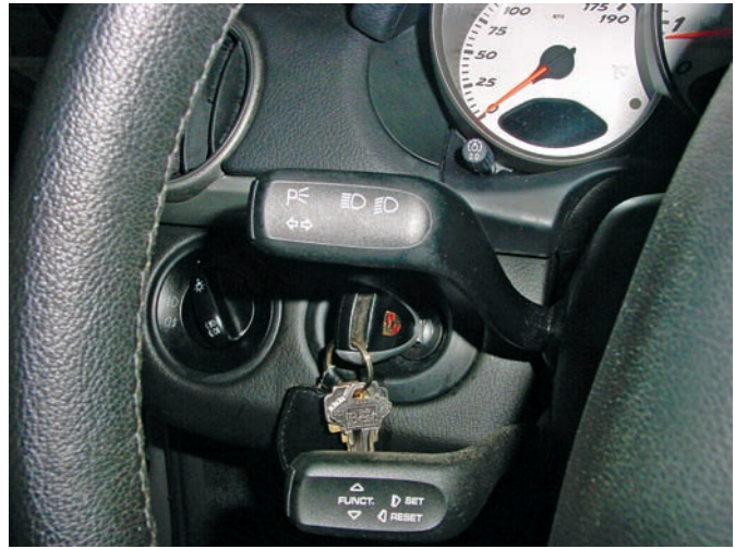
Figure 20-18 Most newer vehicles have the dimmer switch mounted on the steering column.
