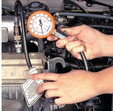
P6-11 Before removing the gauge from the cylinder, release the pressure from it using the release valve on the gauge.
