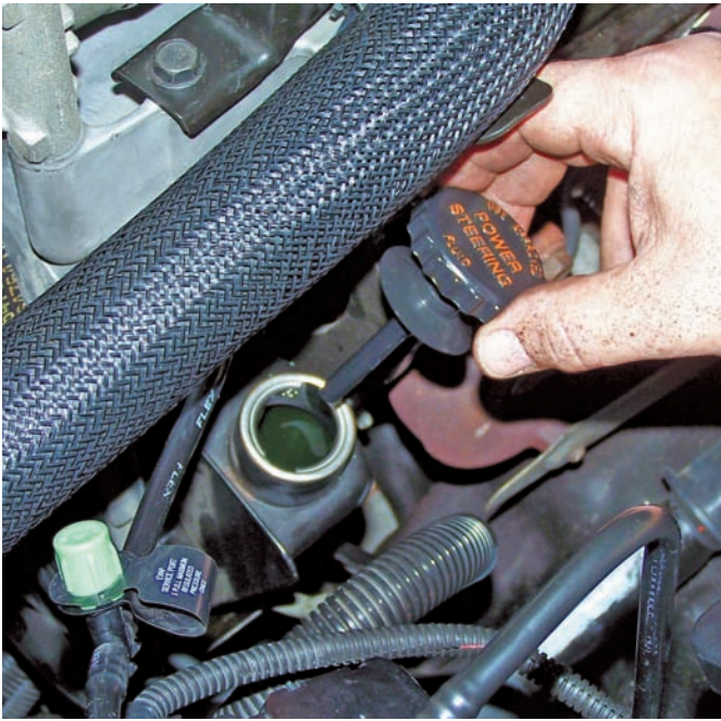
Figure 46-34 Check the fluid level with the dipstick attached to the cap.
