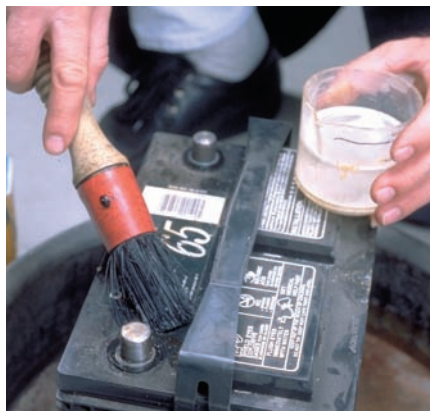
P5-8 Brush the baking soda solution over the battery case, but do not allow the solution to enter the cells of the battery.
