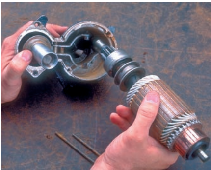
P16-10 Remove the armature. Note: On some units it may be necessary to remove the shift lever from the drive housing before removing the armature.
