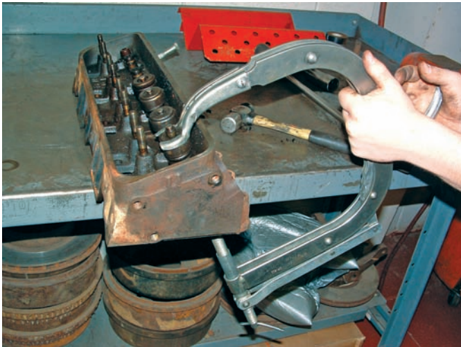
Figure 12-36 With a spring compressor, compress the springs just enough to remove the keepers.
