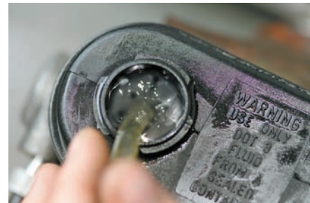
P51-6 Watch for bubbles to appear at the tube ends immersed in the fluid. Slowly release the cylinder piston and allow it to return to its original position. On quick take-up master cylinders, wait 15 seconds before pushing in the piston again. On other units, repeat the stroke as soon as the piston returns to its original position. Slow piston return is normal for some master cylinders.
