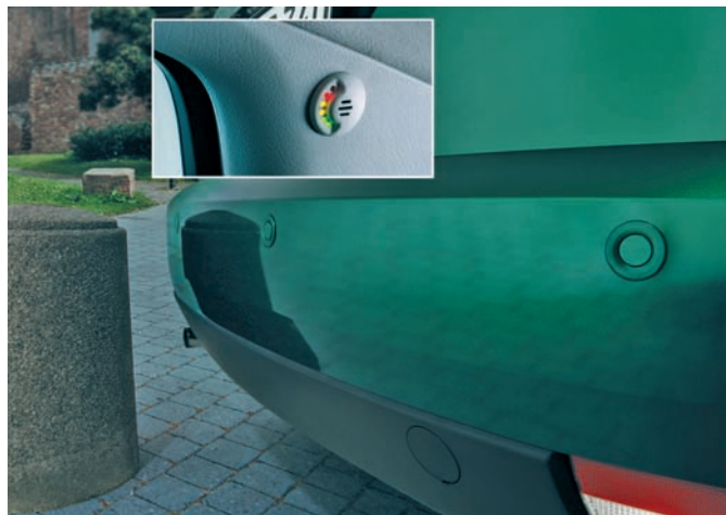
Figure 21-19 The sensors measuring the distance from the rear of the car to obstacles trigger the warning system (insert) inside the vehicle. Courtesy of Robert Bosch GmbH, www.bosch-presse.de
