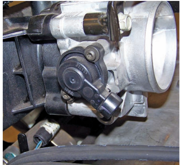
Figure 30-13 A TP sensor mounted to a throttle body.
