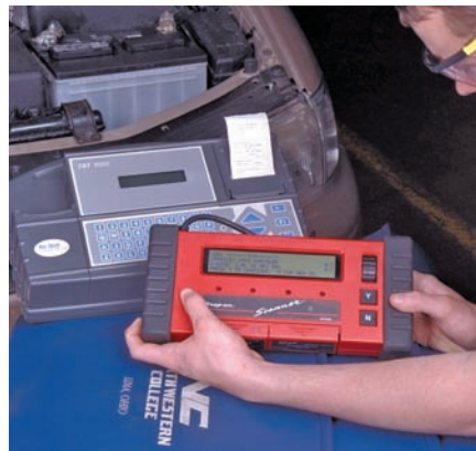
P24-8 Start the engine and obtain the input sensor and output actuator data on the scan tool. If a printer for the tool is available, print out the data report.
