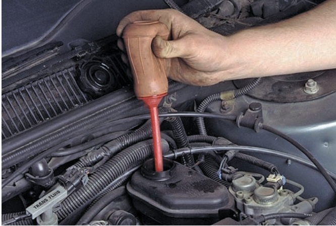
P52-1 Front brake pad replacement begins with removing brake fluid from the master cylinder reservoir.
