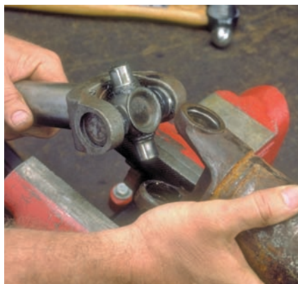
P38-8 Separate the joint by turning the shaft over in the vise and driving the cross and remaining bearing cup down through the yoke with a brass drift and hammer.
