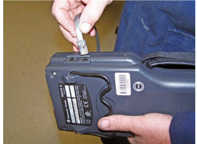
P20-2 Connect the scan tool to a PC that can link the scan tool to the flash software. Some scan tools will connect directly to an Internet site.
