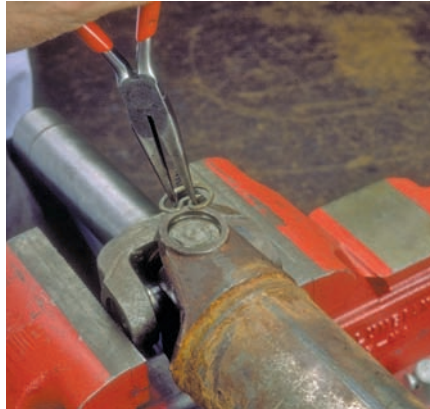
P38-2 Remove the lock rings on the tops of the bearing cups. Make index marks in the yoke so that the joint can be assembled with the correct phasing.
