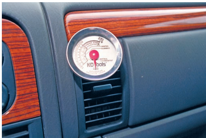
Figure 53-10 A thermometer is used to determine air discharge temperature into the passenger compartment.
