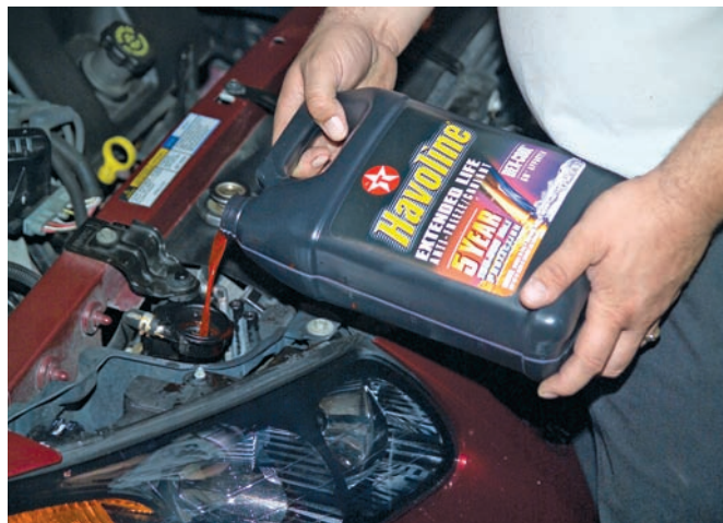
P11-7 Correct any leaks and top off the fluid level.
