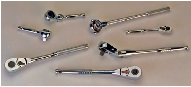
Figure 4-35 An assortment of ratchets.
