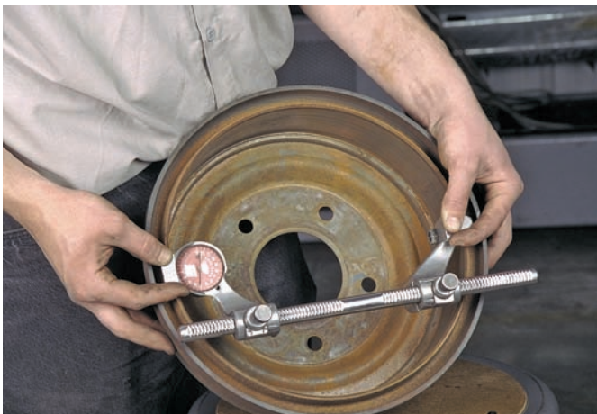
Figure 49-22 Measuring the inside diameter with a drum micrometer.
