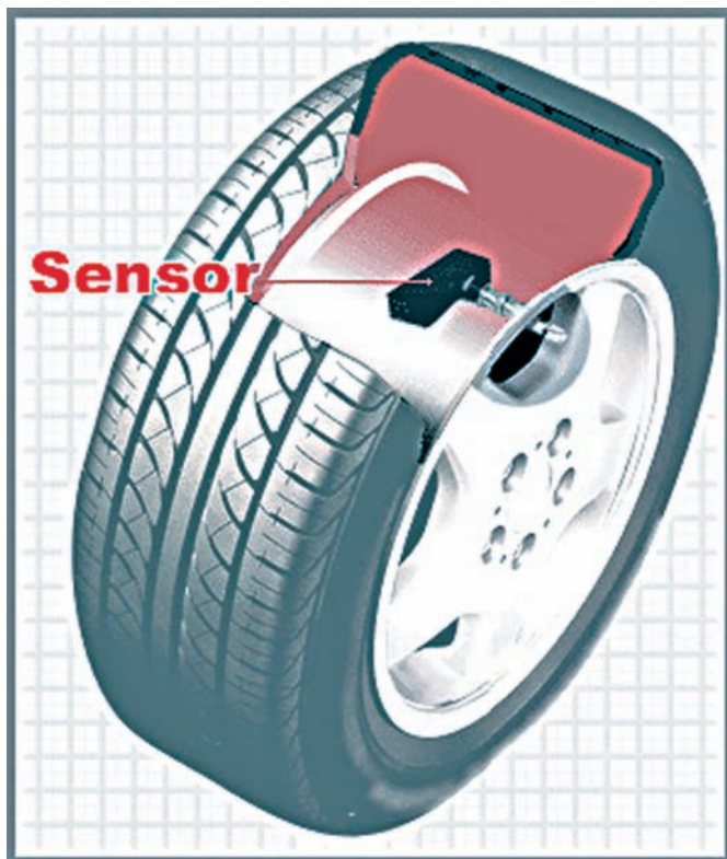
Figure 44-16 A tire pressure monitor and air valve assembly. Courtesy of Adaptive Activity Network BV, www.tiresmonitor.com
