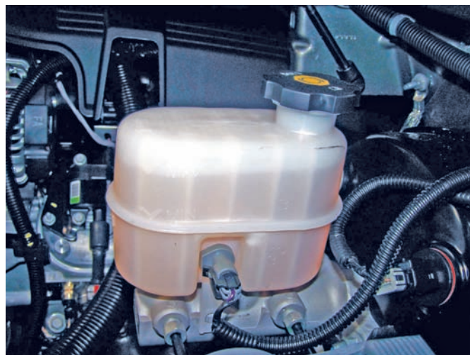
Figure 7-31 Translucent brake fluid reservoirs allow the fluid level to be observed from the outside.
