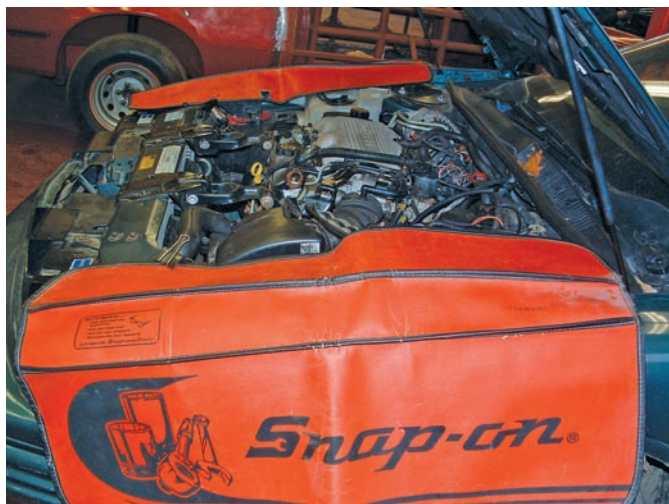
Figure 10-2 Before doing anything, put covers on the fenders.
