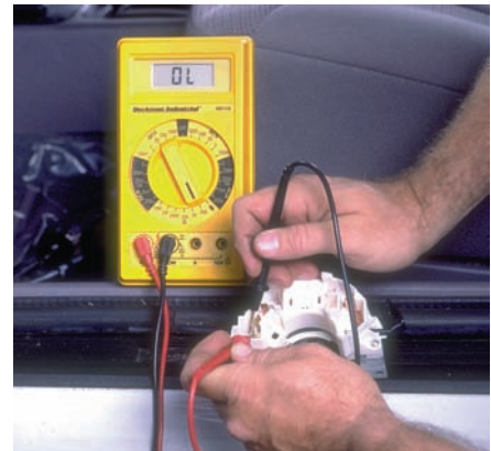
P18-13 When the switch is in the low-beam position, the circuit should be open between the high-beam terminals.
