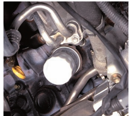
P3-15 Start the engine and allow it to reach normal operating temperature. While the engine is running, check the engine for oil leaks, especially around the oil filter and drain plug. If there is a leak, shut down the engine and correct the problem.
