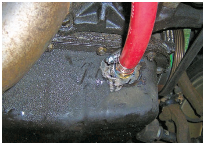
Figure 14-12 The presence of oil and dirt buildup around the oil pan indicates a leaky pan gasket.
