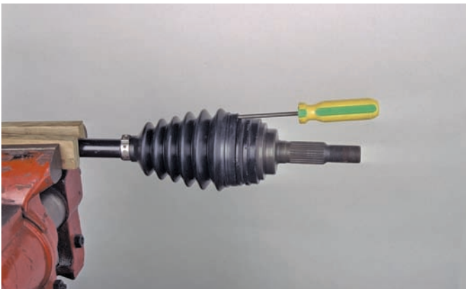
P37-15 Pull the boot over the joint and into its proper position. Use a dull screwdriver to lift an edge of the boot up to equalize the pressure inside the boot with the outside air.
