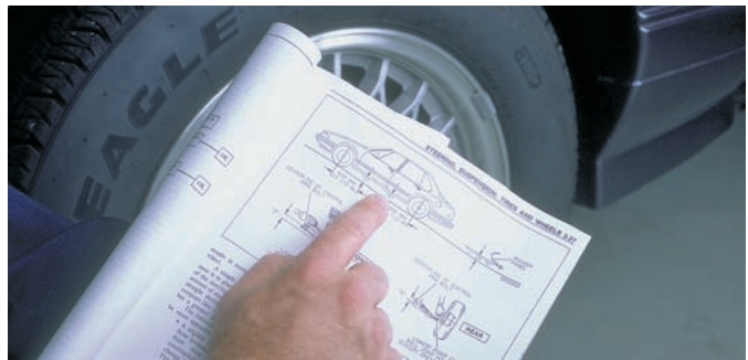
P47-4 Find the vehicle manufacturer's specified curb riding height measurement locations in the service manual.
