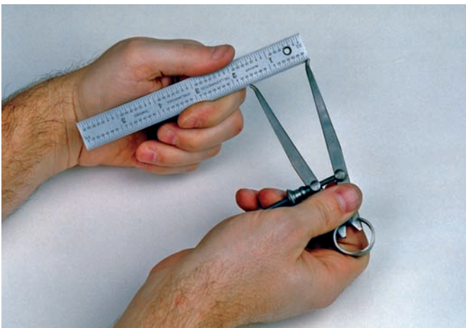
P9-5 Use a scale to determine the measurement expressed by the divider.
