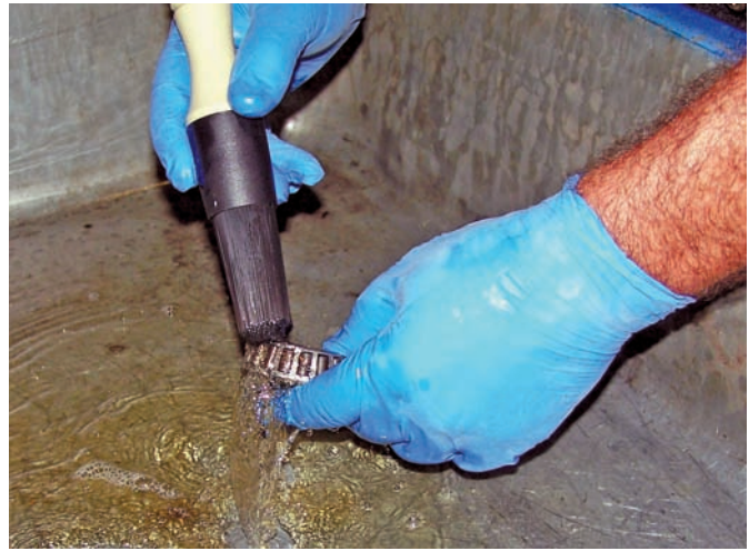
Figure 44-28 Thoroughly clean the bearings and races and then carefully inspect them before reusing them.
