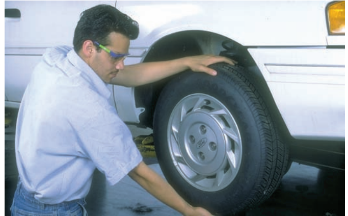
P48-2 Grasp the front tire at the top and bottom and rock the tire inward and outward while a coworker visually checks for movement in the front wheel bearing. If there is movement, adjust or replace the wheel bearing.
