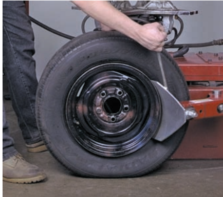
P46-1 Dismounting the tire from the wheel begins with releasing the air, removing the valve stem core, and unseating the tire from its rim. The machine does the unseating. The technician merely guides the operating lever.
