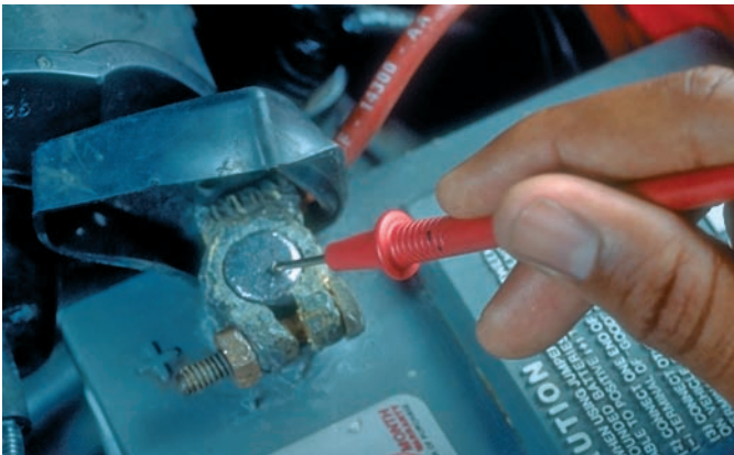
P12-3 To test the voltage drop of the entire headlamp system, connect the positive (red) lead to the battery positive terminal.
