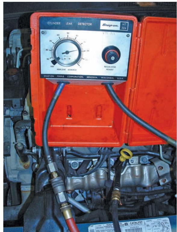
Figure 9-38 The reading on the tester is the percentage of air that leaked out during the test.
