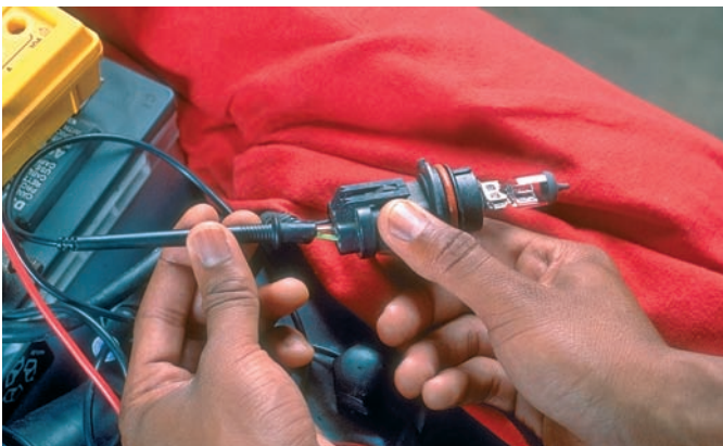
P12-4 Connect the negative (black) lead to the low beam terminal of the headlight socket. Make sure you are connected to the battery “+” or power feed wire of the headlight.
