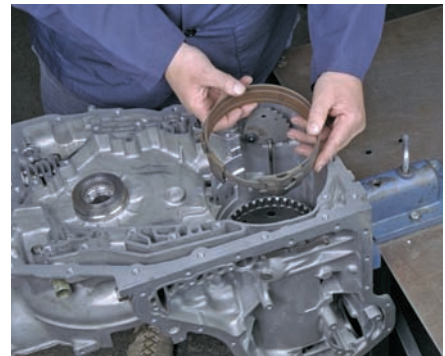
P43-33 Install the thrust washers. Using the correct tool, install the second clutch and input shaft clutch housings as an assembly. Install the reverse band.
