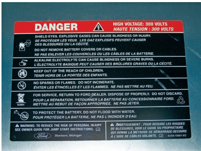
Figure 6-17 Most high-voltage components in a hybrid vehicle have “High Voltage” caution labels.
