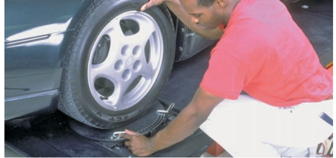
P50-2 Make sure the front tires are positioned properly on the turn tables.
