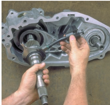
P44-14 Remove the mainshaft with the oil pump assembly.
