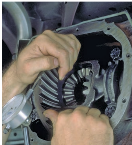
P40-8 Install and tighten the bearing caps to specifications.
