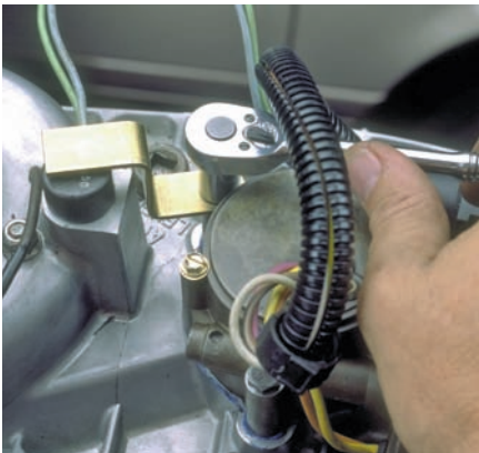
P45-16 Tighten the motor's retaining bolts to specifications.
