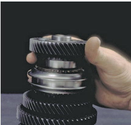
P36-4 Install fourth gear and its bearing. The bearing may need to be lightly pressed into position.
