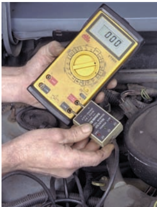
P25-4 Insert the voltage terminals of the MAP sensor tester into the test lead terminals on a DMM; make sure the polarity is correct.
