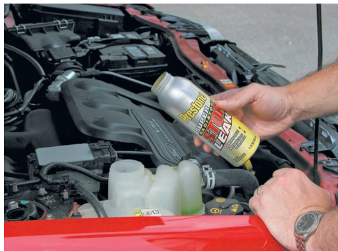
Figure 14-61 Stop leak being added to the cooling system. Courtesy of Honeywell International Inc.
