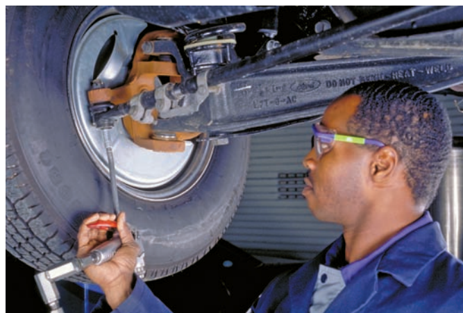
Figure 7-43 A grease gun forces lubrication into a joint through a zerk fitting.
