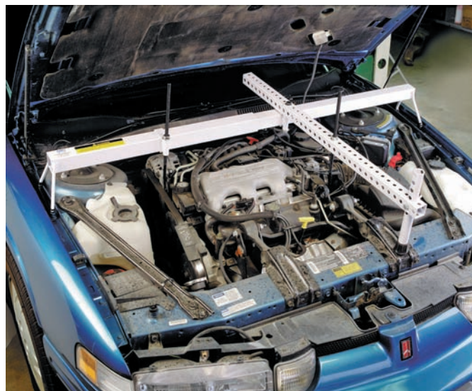
Figure 10-12 A transverse engine support bar provides the necessary support when removing an engine from a FWD vehicle. Courtesy of SPX Service Solutions
