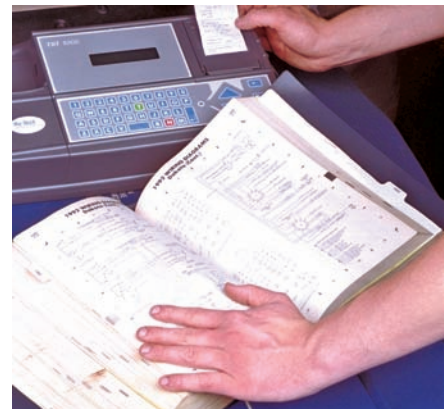
P24-9 Compare the input sensor and actuator data to the specifications given in the service manual. Mark all data that are not within specifications.
