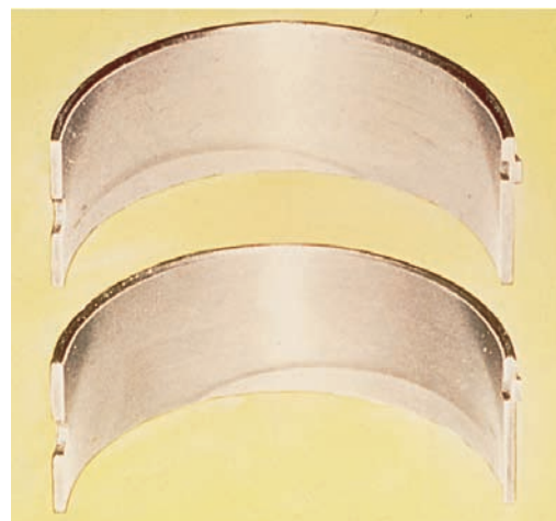
A sign of a bent and twisted rod
