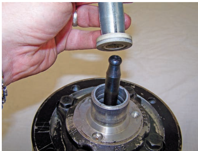
Figure 53-26 Install the protector over the threads of the compressor shaft. Place the new seal on the installer and install the seal with a gentle twisting motion.
