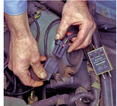
P25-3 Connect the remaining tester connector to the MAP sensor's electrical connector.
