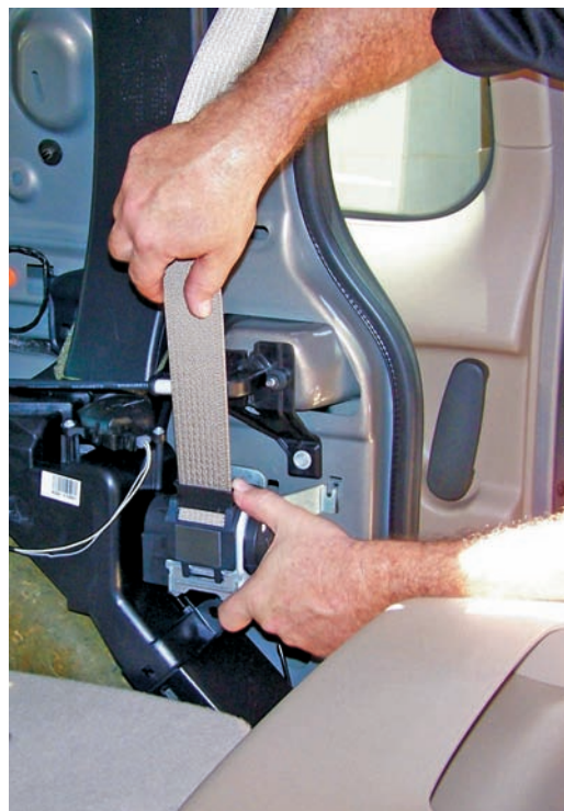
Figure 24-3 A seat belt retractor.
