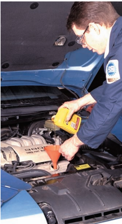
P3-13 Carefully pour the oil into the engine. The use of a funnel usually keeps oil from spilling on the engine.
