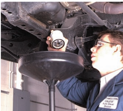
P3-7 Make sure the oil filter seal came off with the filter. Then place the filter into the drain pan so it can drain. After it has completely drained, discard the filter according to local regulations.
