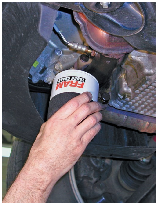
Figure 14-5 An oil filter being installed on an engine block. Courtesy of Honeywell International Inc.
