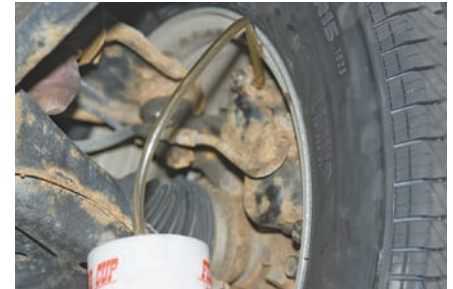
P51-12 After reinstalling the master cylinder, bleed the entire brake system on the vehicle.
