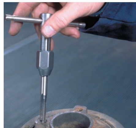
P1-6 Drive the tap back out of the hole by turning it counterclockwise.
