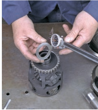
P43-19 Using the proper tool, remove the final drive assembly and selective thrust washers and bearings.
