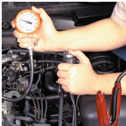
P6-8 Depress the remote starter button and observe the gauge's reading after the first engine revolution.
