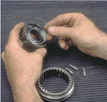
P36-1 Lightly oil the parts of the synchronizer.
