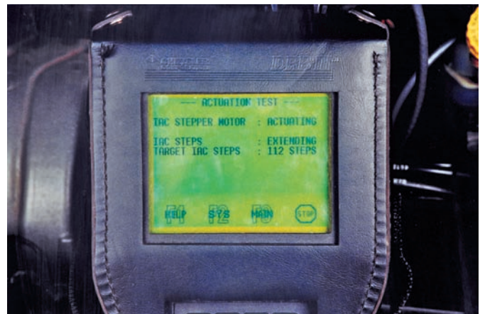
Figure 31-31 When operated in its high range, the IAC should move approximately 112 steps or counts.
