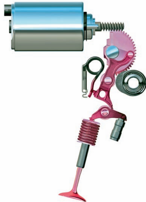
Figure 12-31 The position of the eccentric shaft to provide maximum lift in a Valvetronic system. Courtesy of BMW of North America, LLC
