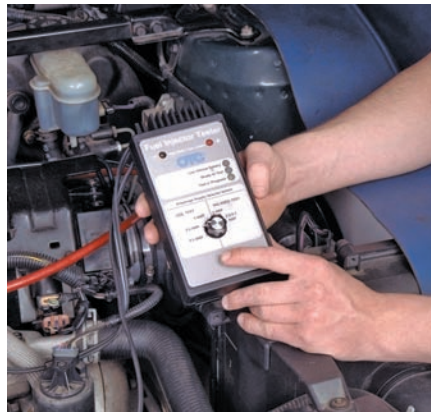
P31-5 Push the injector pulse tester switch and record the pressure on the pressure gauge. Subtract this reading from the measured system pressure. The answer is the pressure drop across that injector.
