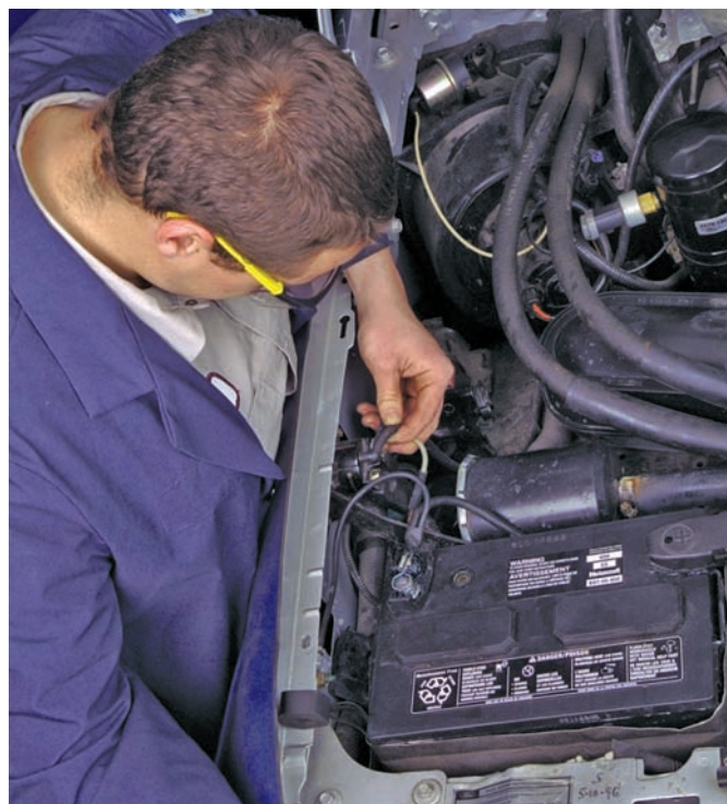
Figure 31-3 All underhood wiring should be carefully inspected.
