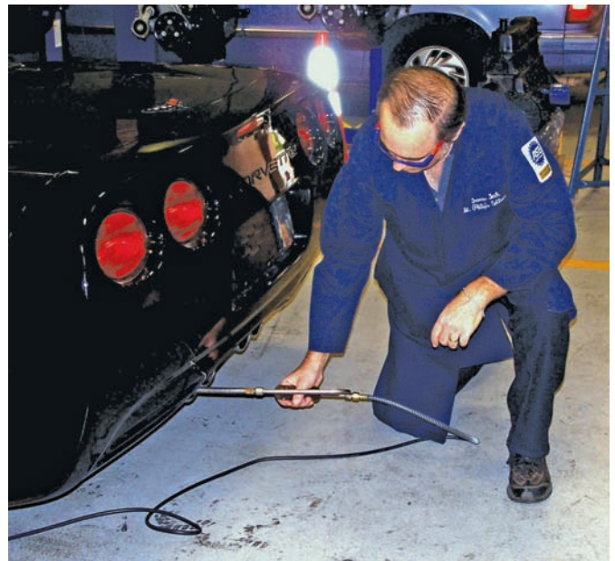
Figure 34-8 The analyzer's probe is inserted into the vehicle's tailpipe.
