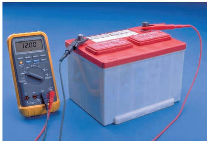
Figure 17-34 Measuring open circuit voltage across battery terminals using a voltmeter.
