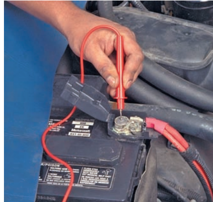
P15-2 Connect the meter's positive lead to the positive battery post. If at all possible, do not connect it to the battery clamp.
