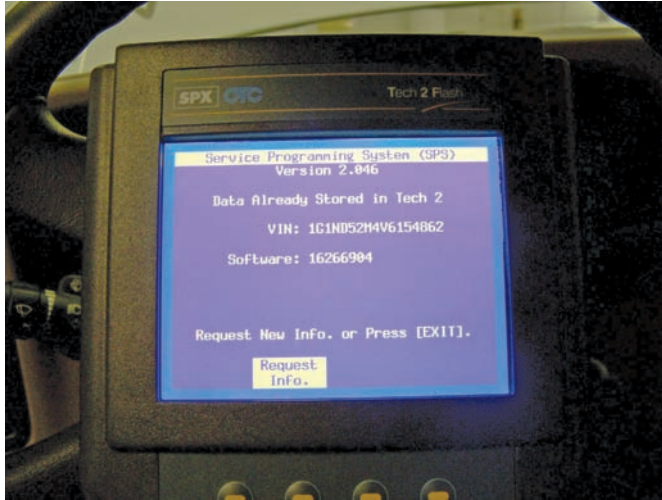
P20-1 Use the scan tool to retrieve the BCM's part number or the vehicle's VIN and record it.
