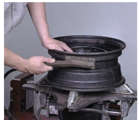
P46-6 Prepare the wheel for the mounting of the tire by using a wire brush to remove all dirt and rust from the sealing surface. Apply rubber compound to the bead area of the tire.
