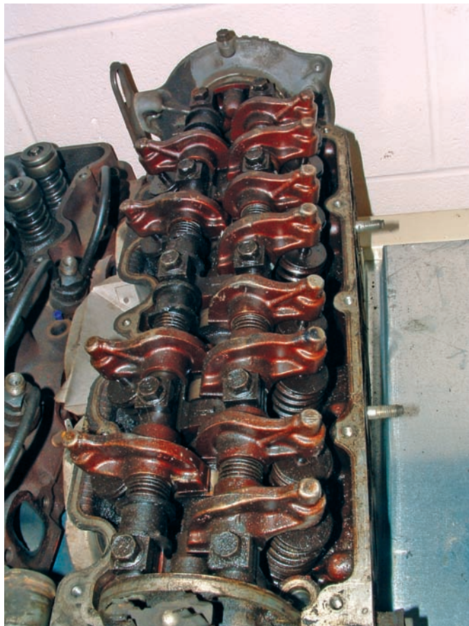
Figure 10-21 Remove the valve cover and disassemble the rocker arm components. Check the rocker area for sludge. Keep the rocker arms or rocker arm assemblies in the order they were installed.
