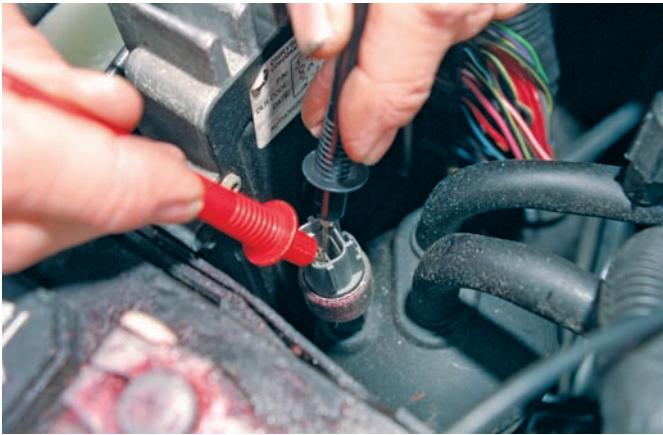
Figure 16-51 A temperature sensor (thermistor) can be checked with an ohmmeter.
