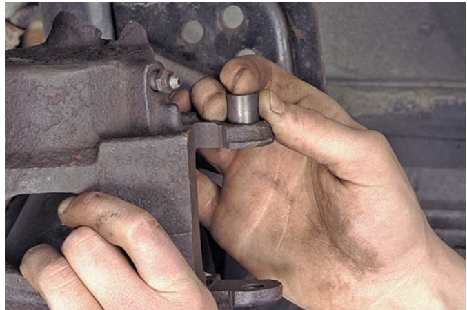
P52-10 Remove the clamp and install new locating pin insulators and sleeves, if necessary.
