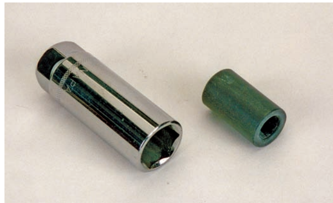
Figure 4-36 A chromed deep-well socket and an impact socket.
