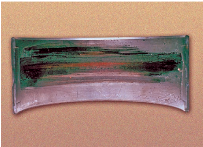
Figure 14-15 Damage to this main bearing was caused by a lack of oil. Courtesy of Dana Corporation
