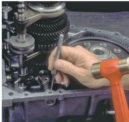
P35-5 Use a punch to drive the roll pin from the shift-lever shaft.
