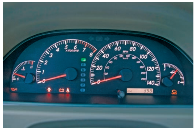
Figure 21-1 A simple but functional approach to the layout of the essential gauges in an instrument panel. Courtesy of Toyota Motor Sales, U.S.A., Inc.
