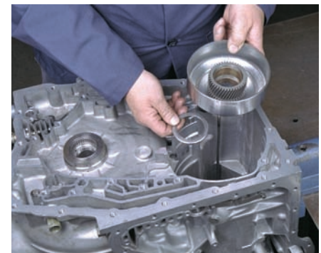
P43-24 Install the reaction sun gear to final drive ring gear thrust bearing. Then assemble the reaction sun gear and drum assembly onto the final drive ring gear.
