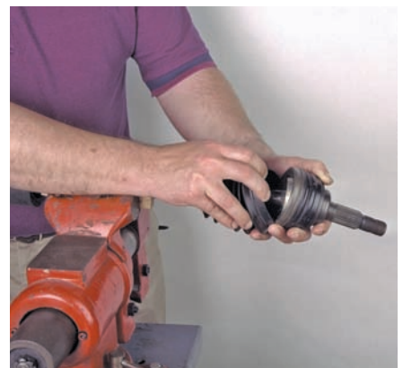
P37-9 Scribe a mark around the axle to indicate the boot's position on the shaft. Then move the boot off the joint.
