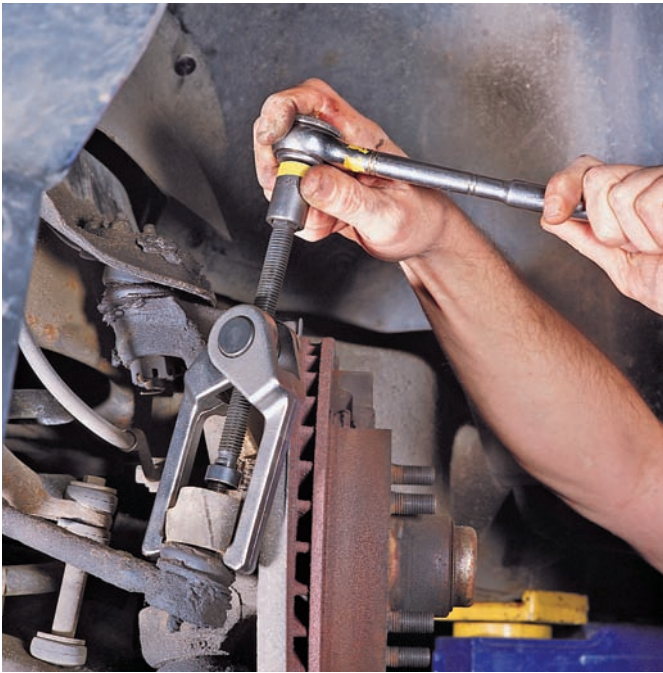
Figure 46-37 A tie-rod end-separating tool. Courtesy of Federal-Mogul Corporation
