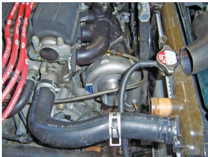
Figure 14-50 Nearly all radiator hoses have a part number painted on the outside of the hose. These should be used when replacing a hose.
