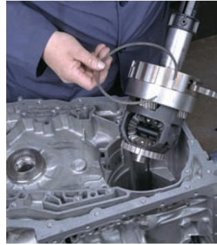
P43-20 Check the final drive end play and select the correct size thrust washers for the unit.
