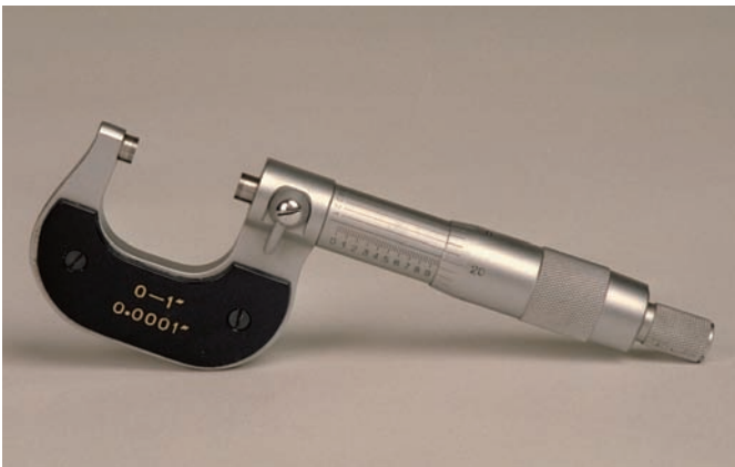
P2-3 The graduations on the sleeve each represent 0.025 inch. To read a measurement on a micrometer, begin by counting the visible lines on the sleeve and multiplying them by 0.025.
