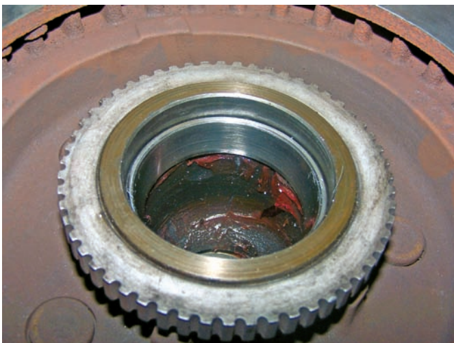
Figure 50-29 Check the wheel speed sensor's rotor when servicing a rotor.
