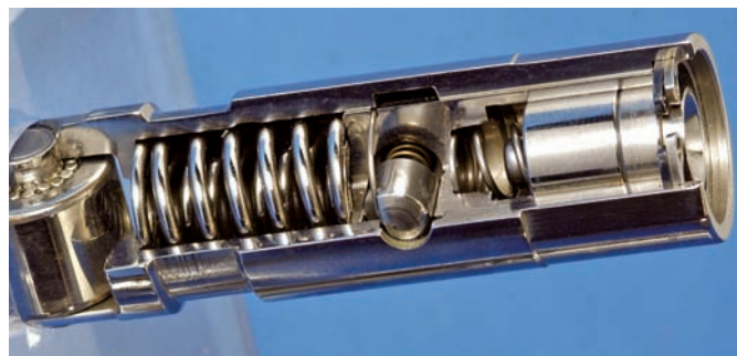
Figure 12-24 The lifter used in Chrysler's multidisplacement system. When the pin in the center is moved, the piston inside the lifter is disconnected from the lifter body. Courtesy of Chrysler LLC
