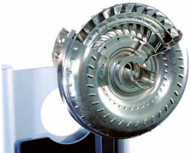
Figure 40-5 A cutaway of a modern torque converter. Courtesy of BMW of North America, LLC
