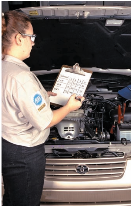
P6-13 After completing the test on all cylinders, compare them. If one or more cylinders is much lower than the others, continue testing those cylinders with the wet test.
