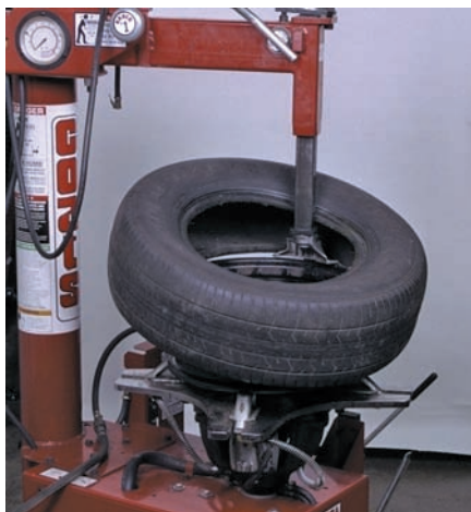
P46-5 After the tire is totally free from the rim, remove the tire.
