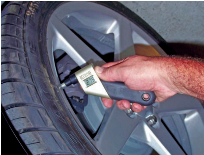
Figure 7-38 Check the tires and wheels for damage and proper inflation.
