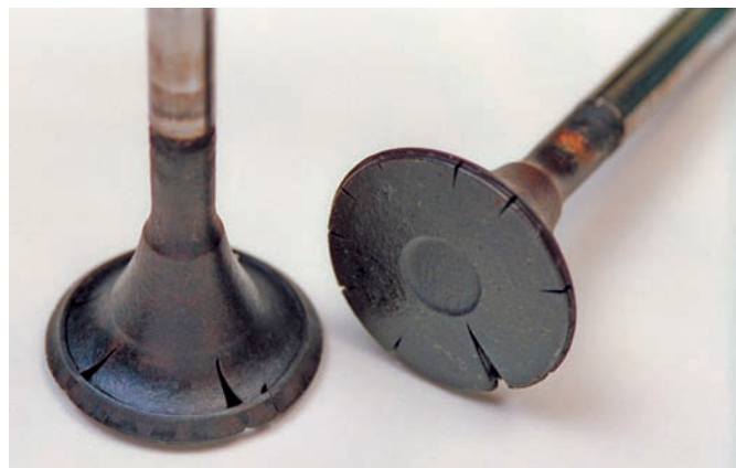
Figure 12-40 Severely burnt valves.
