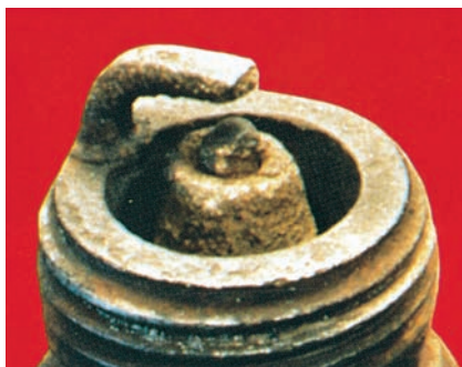
Figure 28-53 A worn spark plug. Courtesy of Federal-Mogul Corporation
