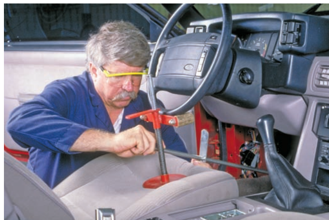
Figure 5-56 The technician is installing a brake pedal depressor; also note that a steering wheel lock is in place.
