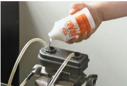
P51-4 Fill the reservoirs with fresh brake fluid until the level is above the ends of the tubes.
