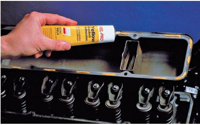
Figure 13-25 An adhesive is often used to hold a gasket in place during assembly. Courtesy of Federal-Mogul Corporation
