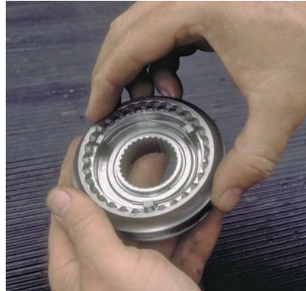
P36-2 Assemble the synchronizer assemblies, being careful to align the index marks made during disassembly.
