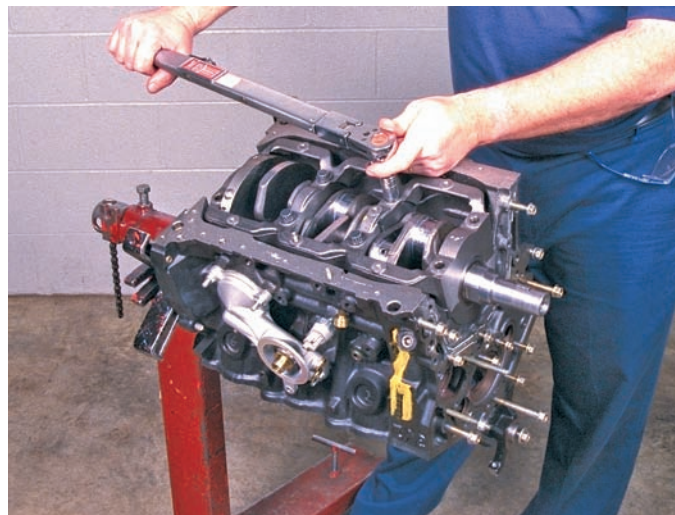
P7-7 Install the cap bolts and tighten them according to the manufacturer's recommendations.
