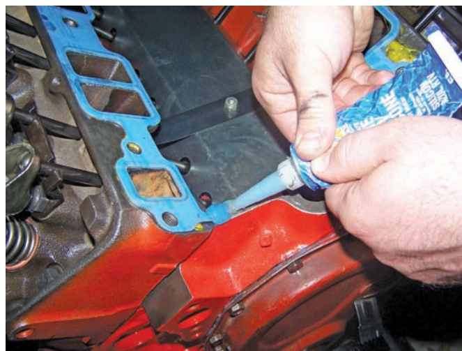
Figure 13-43 On some engines, after the intake manifold gaskets and seals are in place, a small bead of RTV should be applied at the point where the seals meet the gasket.
