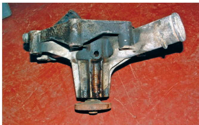
Figure 14-45 This pump shows signs of bad leaks.
