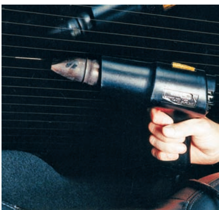
P21-7 Apply heat to the repair area for 2 minutes. Hold the heat gun 1 inch (25 mm) away from the repair.
