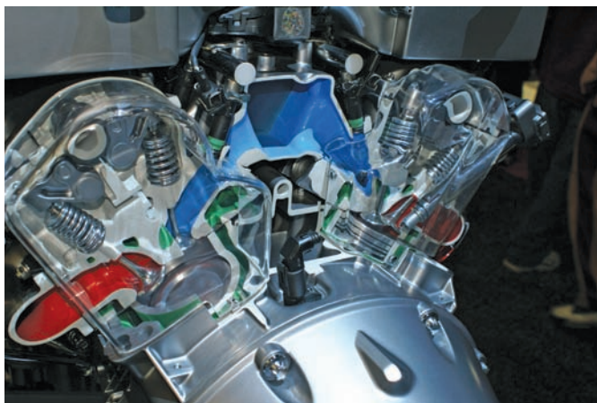
Figure 9-6 A cutaway of an engine showing the intake passages (blue) and valve and exhaust passage (red) and valve.
