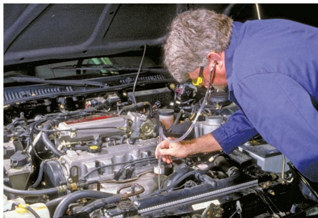
Figure 9-47 Using a stethoscope helps to identify the source of an abnormal noise.
