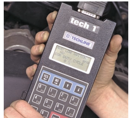
P33-9 Take the vehicle for a test drive with the scan tool still connected. The EGR solenoid should cycle to ON once the vehicle is at a cruising speed. If it does not, check the solenoid and associated circuits.
