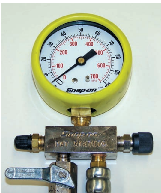
Figure 5-51 Pressure gauges are used to diagnose automatic transmissions and power steering systems.
