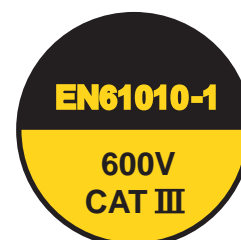
Figure 5-44 Only meters with this symbol should be used on the high-voltage systems in a hybrid vehicle.
