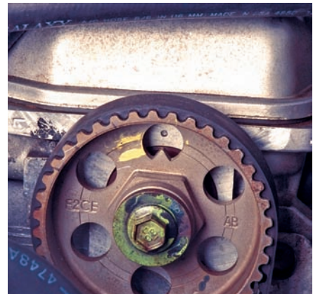
P10-12 Align the camshaft sprocket with the timing marks on the cylinder head. Then wrap the timing belt around the camshaft sprocket and allow the belt tensioner to put a slight amount of pressure on the belt.
