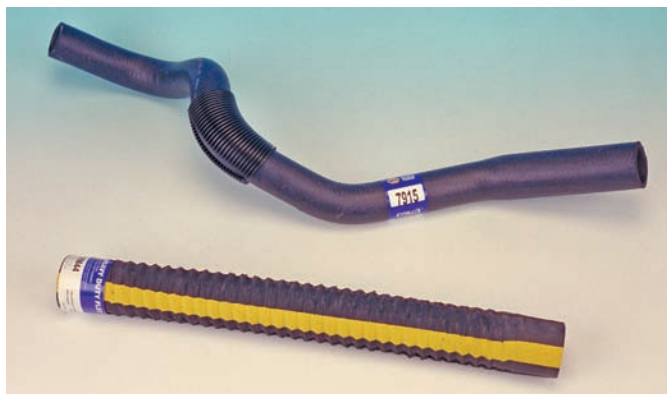
Figure 14-51 Aftermarket replacement hoses are either molded (top) or flex types (bottom).
