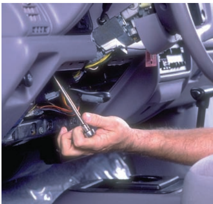
P18-5 Loosen the steering column attaching nuts. Do not remove the nuts.
