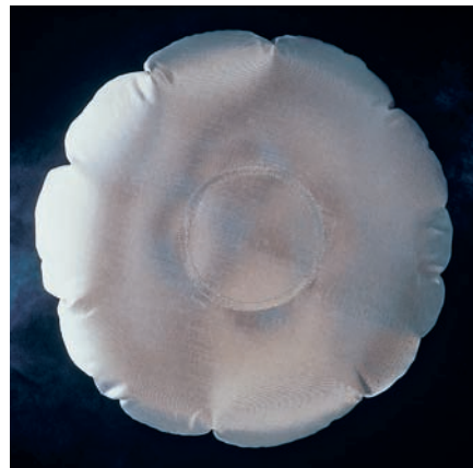
Figure 24-9 Various stages of air bag inflation. Courtesy of TRW, Incorporated
