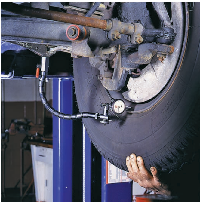
Figure 45-35 A typical mounting of a dial indicator for a radial check. Courtesy of Federal-Mogul Corporation
