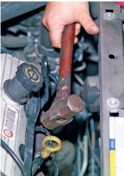
P28-6 Tap on the right exhaust manifold above the knock sensor with a hammer to simulate a knock. Watch the scan tool.
