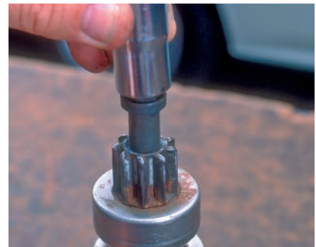
P16-12 Tap the end of the socket with a plastic-faced hammer to drive the retainer toward the armature. Move it only far enough to access the snapping.
