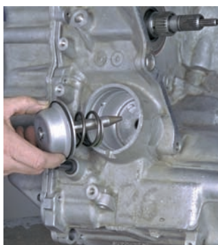
P43-43 Install the reverse servo cover, servo assembly, and retaining ring.
