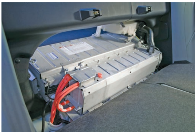
Figure 35-18 The battery pack in a Toyota Camry hybrid. Courtesy of Toyota Motor Sales, U.S.A., Inc.
