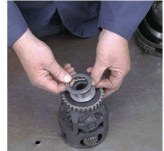
P43-21 Clean and inspect the transaxle case and components. Then position the correct thrust washers and bearings onto the final drive and install the unit. Use petroleum jelly to hold the bearings in place.
