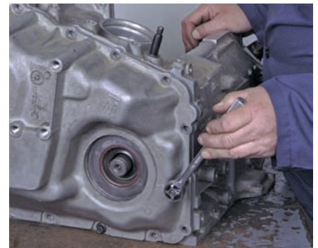
P43-6 Remove the side cover and gaskets. Disconnect the wiring harness to the pressure switches, solenoid, and case connector. Unplug solenoids and switches.
