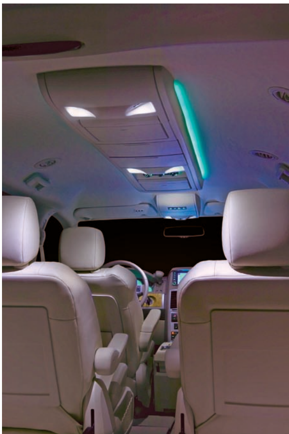
Figure 20-34 An example of using LEDs for interior lights. Courtesy of Chrysler LLC
