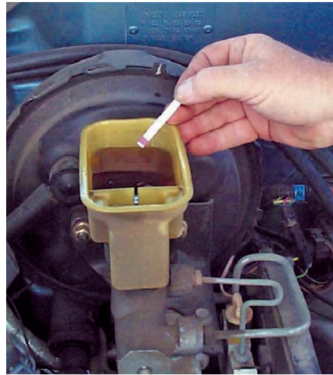
Figure 48-23 A test strip can be used to check for copper contaminants in the brake fluid. Courtesy of Phoenix Systems LLC
