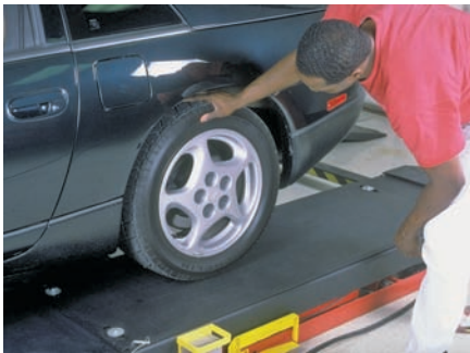
P50-3 Position the rear wheels on the slip plates.
