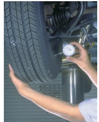
P48-6 Pull the bottom of the tire inward and be sure the dial indicator reading is zero. Adjust the dial indicator as required.
