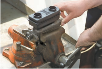
P51-1 Mount the master cylinder firmly in a vise, being careful not to apply excessive pressure to the casting. Position the master cylinder so the bore is horizontal.
