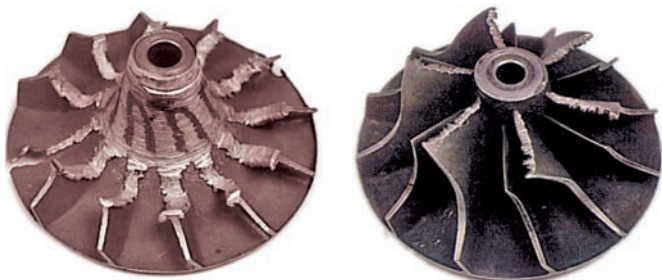
Figure 32-20 Damaged turbocharger wheels.
