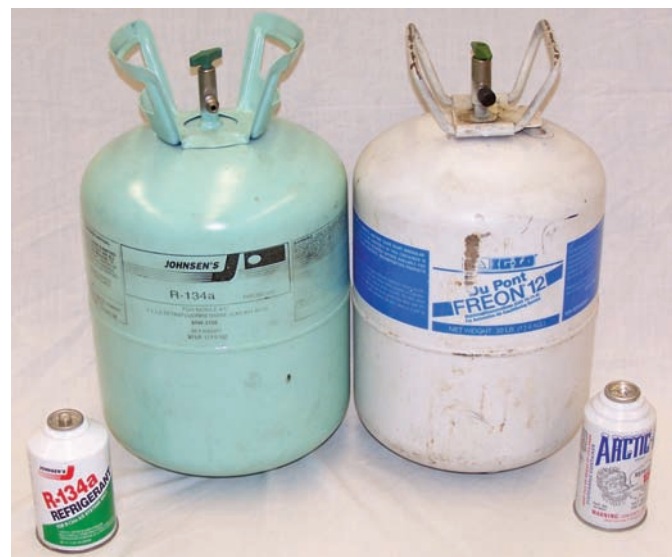
Figure 53-2 R-12 should be stored and sold in white containers, whereas R-134a should be stored in light blue containers.
