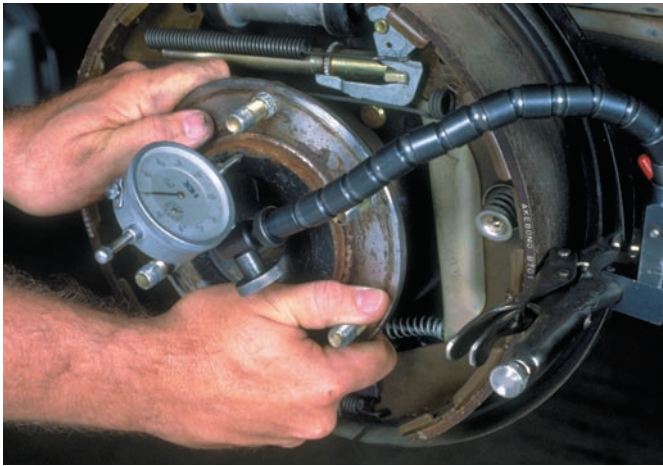
Figure 4-29 This dial indicator setup will measure the amount this axle can move in and out.
