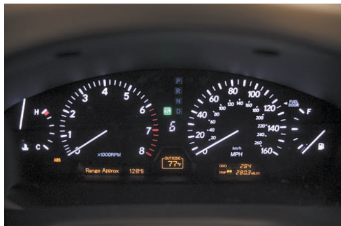
Figure 21-20 Information for the driver appears across the bottom of the instrument cluster. Courtesy of Toyota Motor Sales, U.S.A., Inc.
