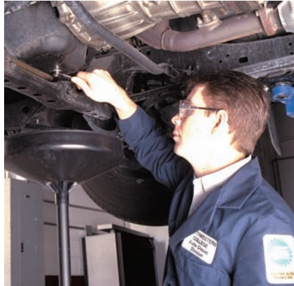
P3-11 Tighten the drain plug according to the manufacturer's recommendations. Overtightening can cause thread damage, whereas undertightening can cause an oil leak.
