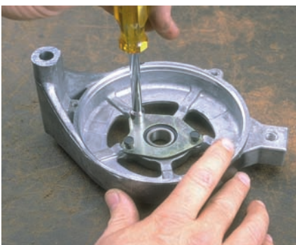
P17-16 Remove the three screws that hold the bearing retainer to the front housing.
