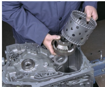
P43-26 Install the input carrier with its thrust bearing in the case. Then install the reverse reaction drum, making sure its spline engages with the input carrier.
