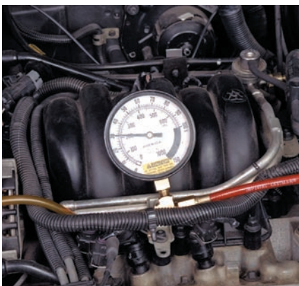
P31-7 Depress the injector pulse tester's switch and observe the fuel pressure. Again the difference between the system pressure and the pressure when an injector is activated is the pressure drop across the injector.
