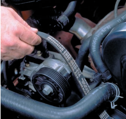
P4-9 Install the new belt over each of the drive pulleys. Often the manufacturer recommends a sequence for feeding the belt around the pulleys.
