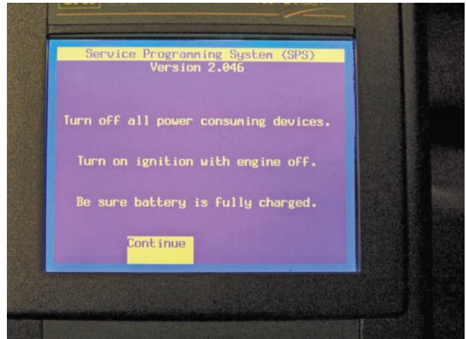
P20-9 Move through the menus on the scan tool until the desired flash screen is shown. Then follow all instructions given on the tool.
