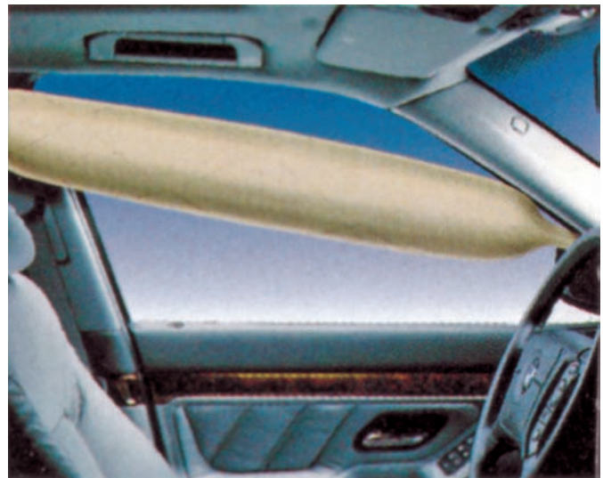
Figure 24-14 A side impact head air bag. Courtesy of BMW of North America, Inc.
