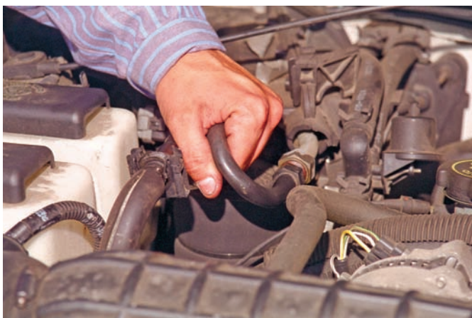
Figure 53-6 Feeling the temperature of the pressure lines in an A/C system is part of a basic visual inspection of the system.
