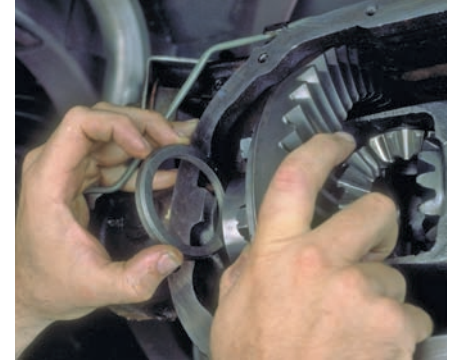
P40-3 Install service spacers that are the same thickness as the original preload shims between each bearing cup and the housing.
