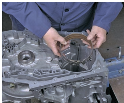
P43-23 Install the forward band into the case, making sure the band is aligned with the anchor pin.
