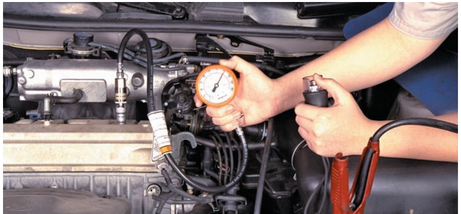
P6-16 If the reading increases with the presence of oil in the cylinder, the most likely cause of the original low readings was poor piston ring sealing. Using oil during a compression test is normally referred to as a wet test.
