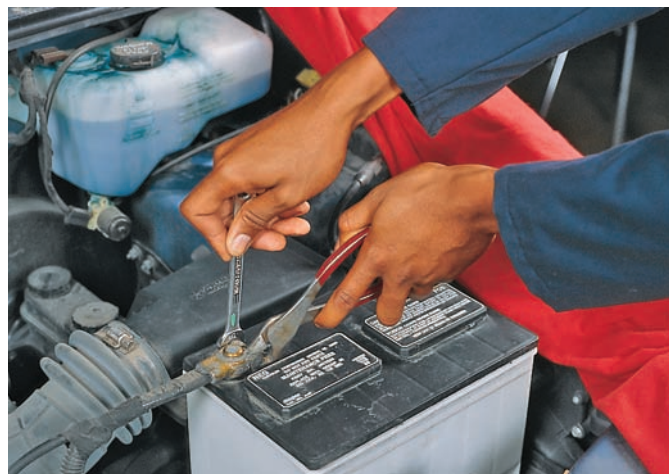
Figure 6-15 Before doing any electrical work or working around the battery, disconnect the negative lead of the battery.
