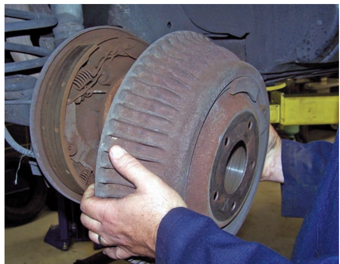
Figure 49-16 Pull the drum away from the axle flange or hub, being careful not to drop it.
