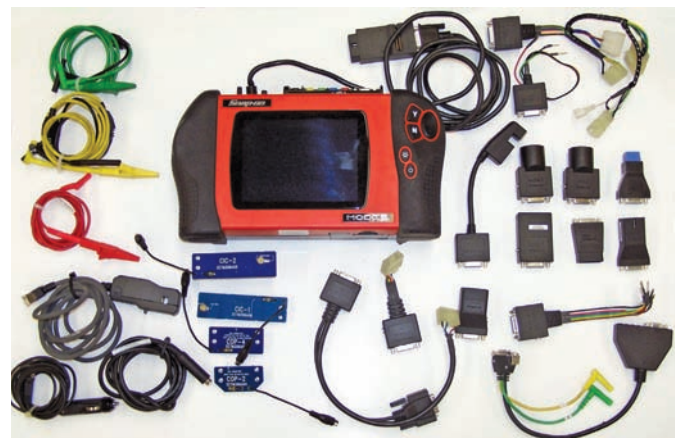
Figure 28-32 Examples of the various adapters and connectors needed to connect a lab scope or GMM to the different ignition systems.
