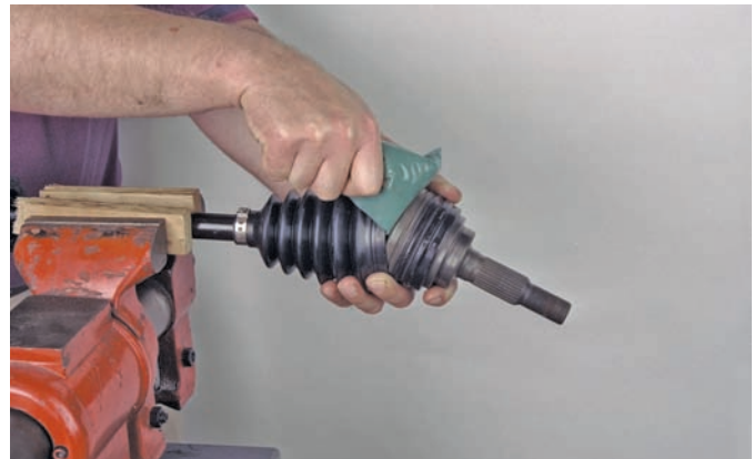
P37-14 Using a new circlip, reinstall the joint on the shaft. Pack joint grease into the joint and boot. The entire packet of grease that comes with a new boot needs to be forced into the boot and joint.
