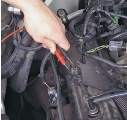
P33-1 Disconnect the connector to the EGR solenoid and connect the leads of an ohmmeter to the solenoid's terminals.
