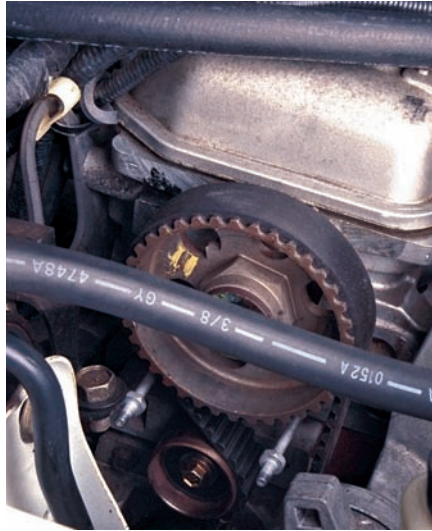
P10-2 Carefully remove the timing cover. Be careful not to distort or damage it while pulling it up. With the cover removed, check the immediate area around the belt for wires and other obstacles. If some are found, move them out of the way.
