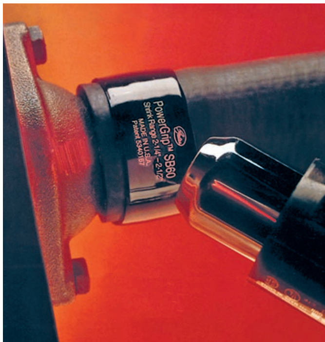
Figure 14-54 Thermoplastic clamps are tightened with a heat gun. Courtesy of Gates Corporation
