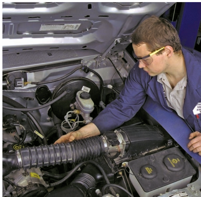
Figure 31-9 Carefully inspect the ductwork and hoses of the air induction system.
