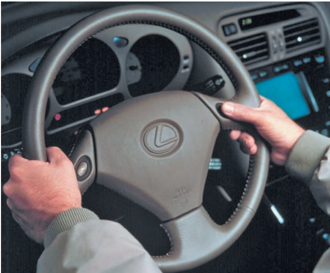
Figure 41-12 Fingertip controls for manually shifting Lexus' automatic/manual transmission. Courtesy of Toyota Motor Sales, U.S.A., Inc.
