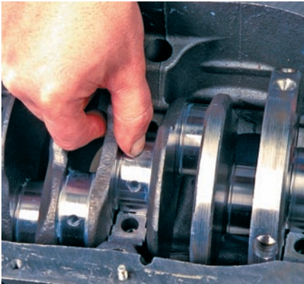
P7-10 Carefully scrape the Plastigage off the journal surface.
