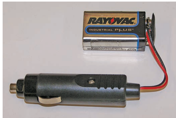
Figure 5-18 A simple 9-volt memory saver.
