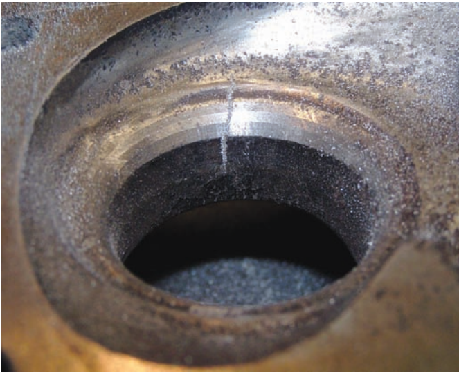
Figure 10-35 Examples of stress cracks.
