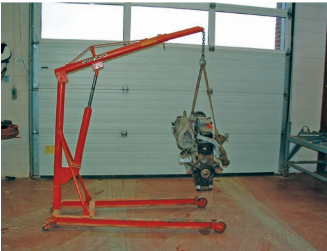
Figure 10-19 Once the engine is removed and is hanging on the engine hoist, lower it close to the floor so it can be safely moved to the work area.
