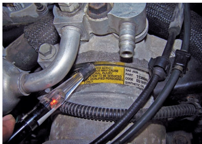
Figure 53-18 When the probe of the leak detector is near the area of a leak, its light will flash.
