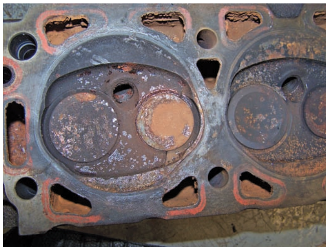
Figure 12-39 Lightweight aluminum heads are prone to cracking. This can lead to a recessed exhaust valve seat.
