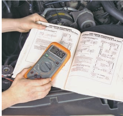
P33-2 Compare your readings to the specifications for the solenoid.
