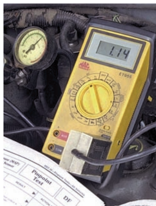
P25-8 Increase the vacuum to the MAP sensor so that it now has 15 in. Hg. Observe the voltage reading now and compare this to specifications.
