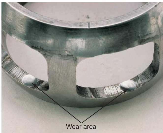
Figure 39-10 A worn cage or race can cause a clicking sound during a turn. Courtesy of Federal-Mogul Corporation
