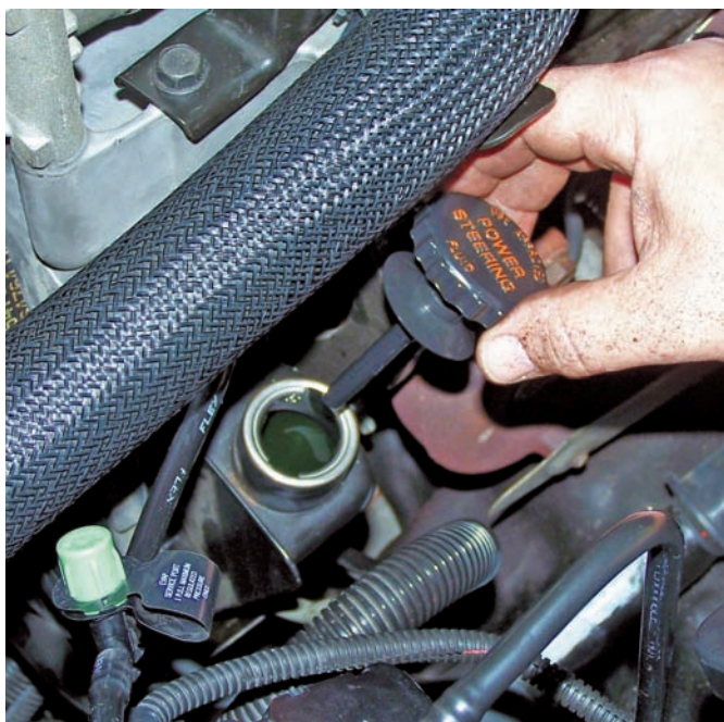
Figure 7-30 The filler cap on a power-steering pump normally has a dipstick to check the fluid level.
