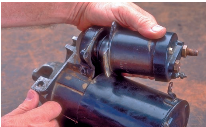
P16-6 Rotate the solenoid until the locking flange of the solenoid is free. Then remove the solenoid.
