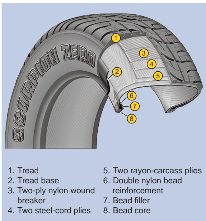
Figure 44-3 A typical tubeless tire. Courtesy of Pirelli Tire of North America, LLC
