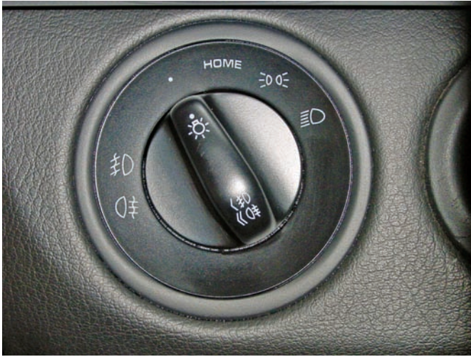
Figure 20-14 A headlight switch that also has positions for rear and front fog lights.
