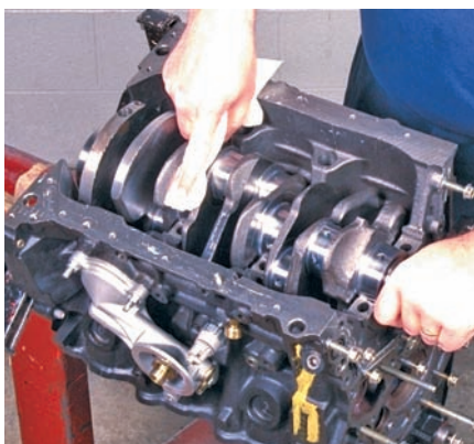
P7-4 Carefully install the crankshaft into the bearings. Try to keep the crankshaft from moving on the bearing surfaces.
