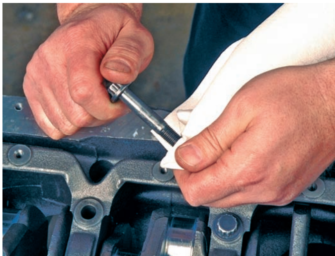
P7-6 Install the main caps in their proper locations and directions. Wipe the threads of the cap bolts with a clean rag.
