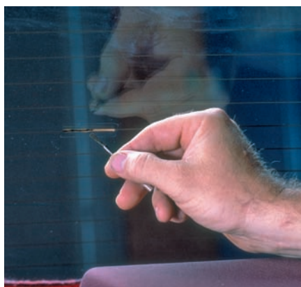
P21-8 Inspect the repair. If it is discolored, apply a coat of tincture of iodine to the repair. Allow to dry for 30 seconds, then wipe off the excess with a cloth.
