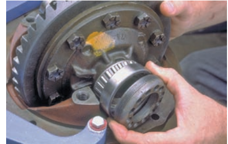
P41-3 Install the bearing cups and adjusting nuts onto the differential case.
