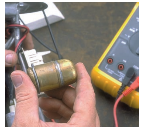
P19-9 Check the float to be sure it is not filled with fuel, distorted, or loose.
