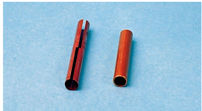
Figure 12-68 A thin-wall valve guide liner.
