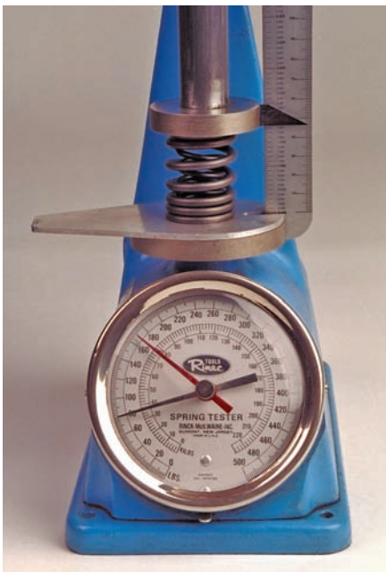
P9-10 The tension gauge will reflect the pressure of the spring when compressed to the installed or valve closed height. Compare this reading to the specifications.
