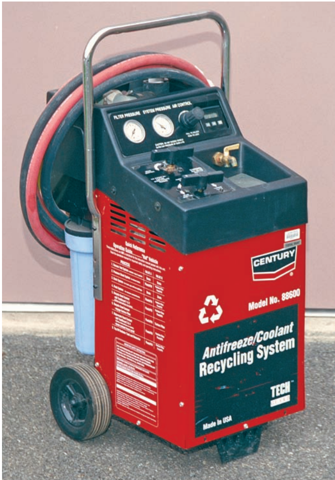
Figure 5-17 A coolant recycling machine that drains, back flushes, and fills the cooling system.
