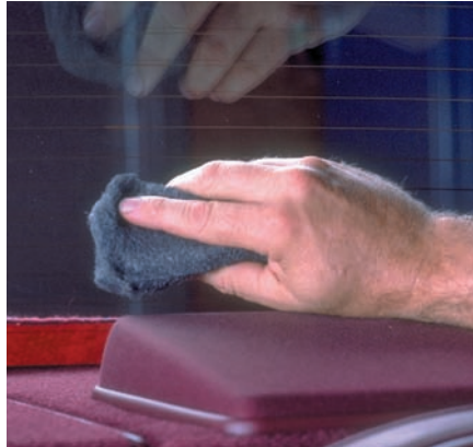
P21-2 Clean the grid line area to be repaired. Buff with fine steel wool. Wipe clean with a cloth dampened with alcohol. Clean an area about 1/4 inch (6 mm) on each side of the break.
