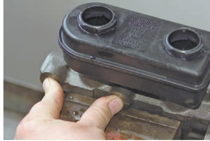
P51-8 Remove the tubes from the outlet ports and plug the openings with temporary plugs or your fingers. Keep the ports covered until you install the master cylinder on the vehicle.
