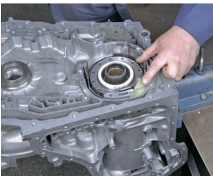
P43-34 Install the scavenging scoop and driven sprocket support with the second clutch thrust washer. Install the driven sprocket support and thrust washer between the sprockets and the channel plate.
