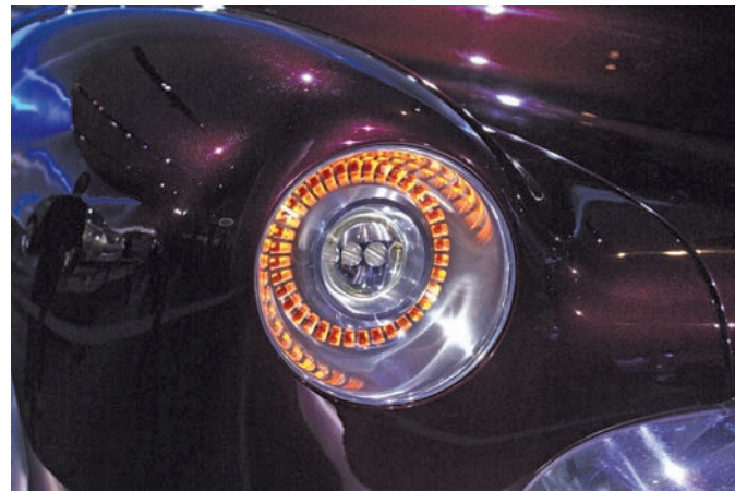
Figure 20-13 This headlight assembly combines a xenon bulb with LEDs. The number of LEDs that are energized depends on the driving conditions.
