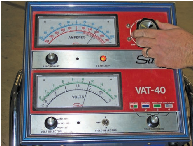
P14-7 Rotate the load control until the ammeter reads one-half of the battery's CCA rating, which in this case is 315 amps.
