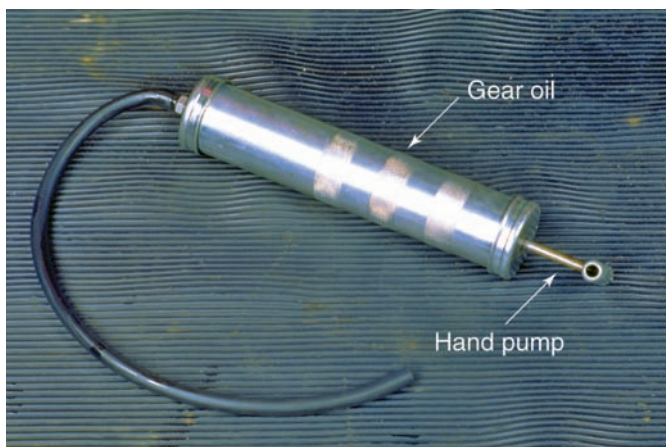
Figure 7-29 A hand-operated pump used to fill transmissions and drive axles with lubricant.
