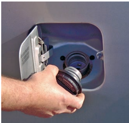
P29-2 Loosen the fuel tank filler cap to relieve any fuel tank vapor pressure.
