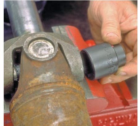
P38-3 Select a socket that has an inside diameter large enough for the bearing cup to fit into; usually a 1/4-inch socket works.
