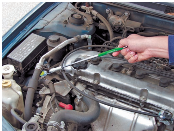
Figure 5-72 With a fluorescent tracer system, refrigerant leaks will glow brightly when inspected with a UV/Blue light as a luminous yellow-green. Courtesy of Tracer Products
