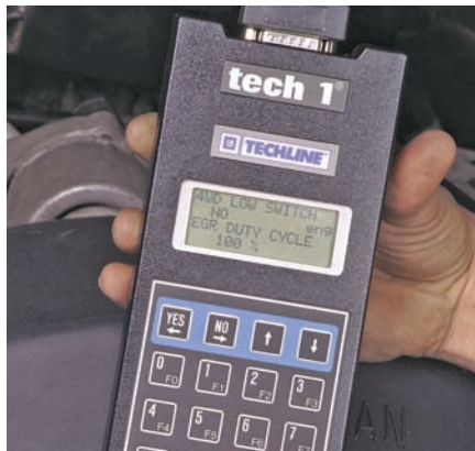
P33-8 Start the engine and obtain the EGR data on the scanner. The EGR valve should be off and remain off while the engine is idling.
