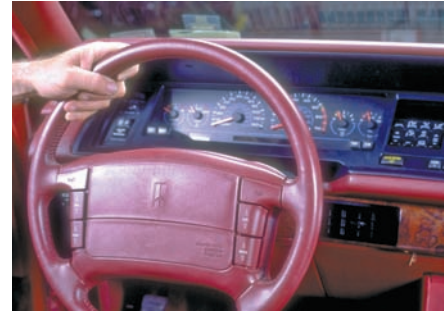
P22-3 Place the front wheels in the straight ahead position and turn the ignition switch to the LOCK position.
