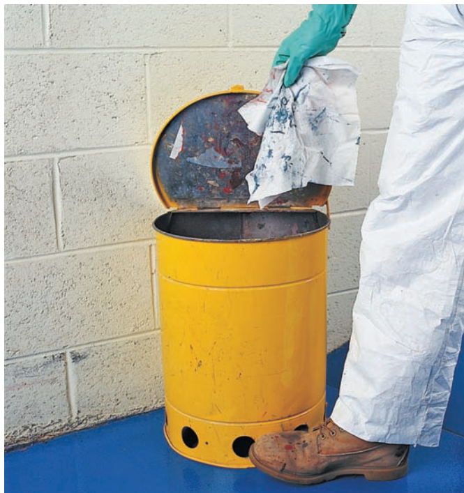
Figure 6-20 Dirty rags and towels should be kept in an approved container. Courtesy of the DuPont Company
