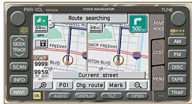
Figure 23-44 The screen of a typical navigational center. Courtesy of Toyota Motor Sales, U.S.A., Inc.
