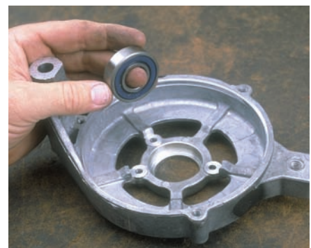
P17-18 Remove the front bearing from the housing. Test and inspect all parts. Replace any defective ones. Reassembly is the reverse of this procedure.
