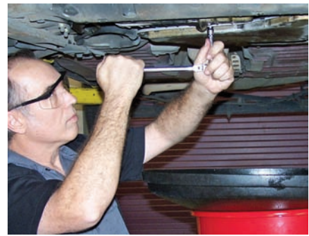
P42-3 Loosen all of the pan bolts except three at one end. This will allow some fluid to drain out.
