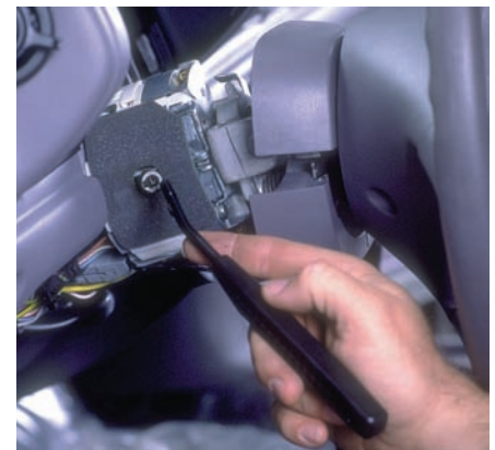
P18-7 Remove the turn signal lever by simply rotating the outer end of the lever. Then pull it straight out.
