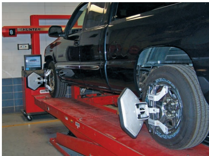
Figure 47-13 A wheel alignment machine that relies on high-imaging cameras and targets to gather measurements.
