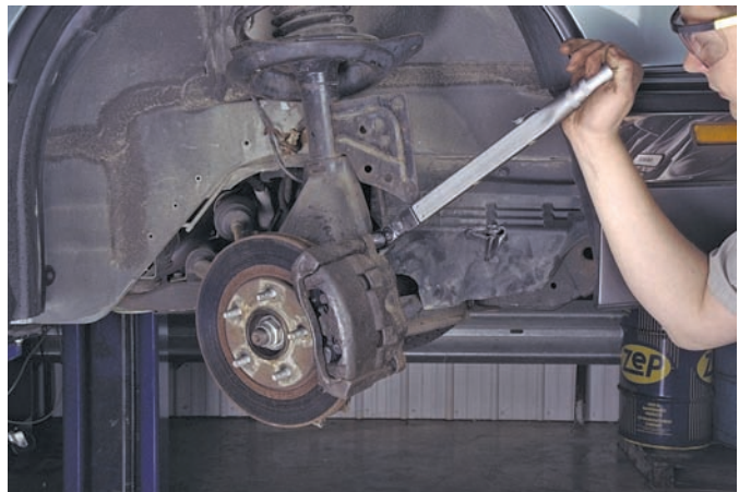
P52-12 Set caliper with pads over the rotor and install the locating pins. After the assembly is in the proper position, torque the pins according to specifications.
