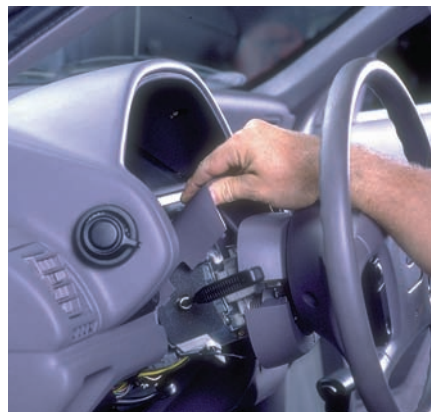
P18-6 Lower the steering column just enough to remove the upper shroud.
