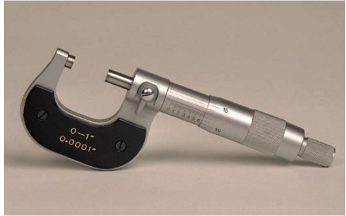
P2-2 Because the diameter of a valve stem is less than 1 inch, a 0-to-1-inch outside micrometer is used.
