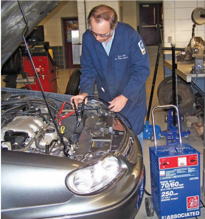
P14-1 To conduct this test, you need a VAT-40 or similar equipment. Before conducting the test, make sure the battery is fully charged.
