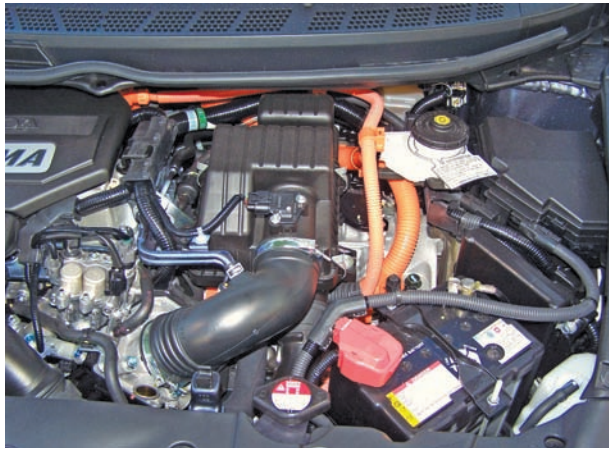
Figure 13-50 The high-voltage connectors and cables in a hybrid are colored orange for identification.
