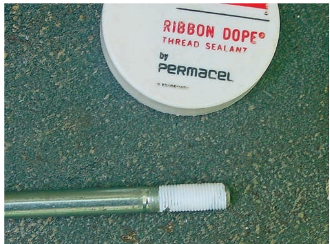
Figure 13-27 Bolts that pass through a liquid passage should be coated with Teflon or similar thread sealant.
