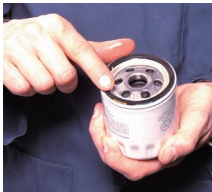
P3-8 Wipe off the oil filter sealing area on the engine block. Then apply a coat of clean engine oil onto the new filter's seal.
