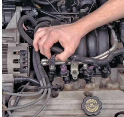
P31-2 Disconnect the number 1 injector and connect the injector pulse tester to the injector's terminals.
