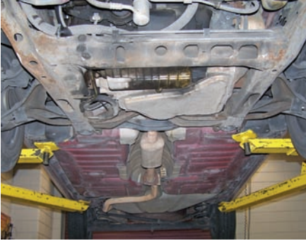
P42-1 Raise the vehicle to a good working height and safely positioned on the lift.
