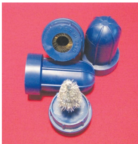
Figure 17-26 Combination external/internal wire brushes clean both terminals and inside cable connector surfaces.
