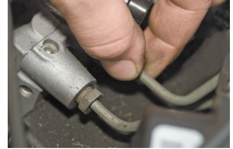
P51-9 Install the master cylinder on the vehicle. Attach the lines, but do not tighten the tube connections.
