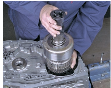
P43-15 Using the correct tool, remove the second clutch and input shaft clutch housings as an assembly. Remove the reverse band.
