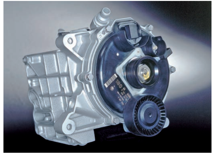
Figure 19-13 A water-cooled AC generator. Courtesy of BMW of North America, LLC
