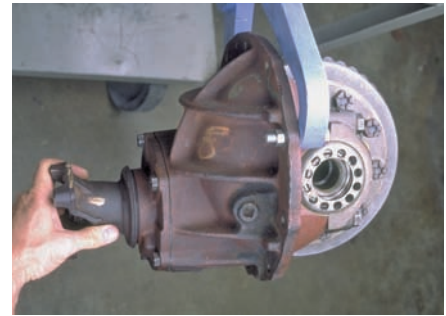
P41-6 Seat the bearings by rotating the pinion several times each time the adjusters are moved.
