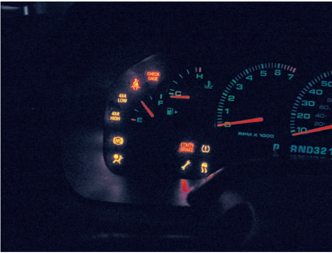
Figure 21-15 Most warning lights and indicators go through a bulb check when the ignition is first switched to the on position.
