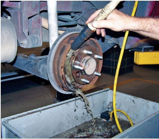
Figure 49-17 Before disassembling the brakes, use an OSHA-approved washer to make sure all asbestos dust is removed from the parts.
