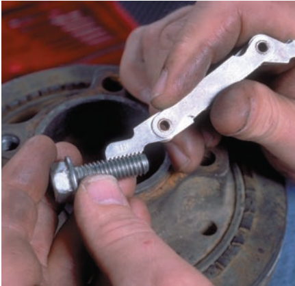
P1-1 Using a thread pitch gauge, determine the thread size of the fastener that should fit into the damaged internal threads.
