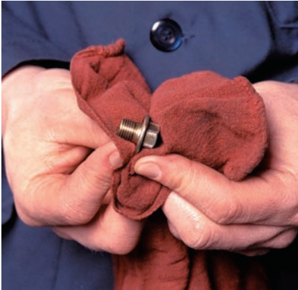
P3-10 Prior to installing the drain plug, wipe off its threads and sealing surface with a clean rag.
