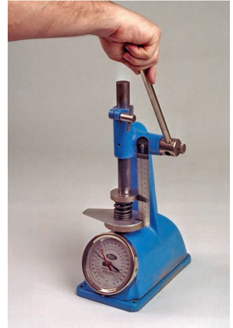
P9-9 Compress the spring into the installed height by pressing down on the tester's lever.
