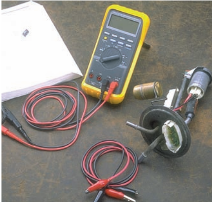
P19-1 The tools required to perform this task are a DMM, jumper wires, and a service manual.
