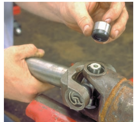
P39-9 Position the joint's cross in the drive shaft yoke and install the two remaining bearing cups.
