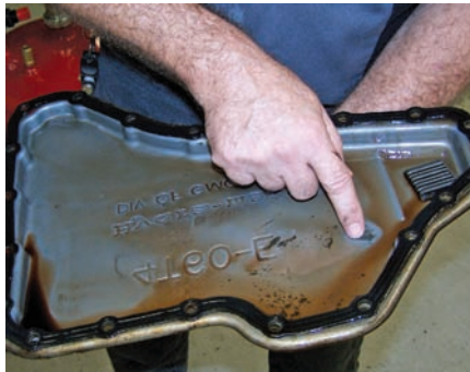
P42-5 Inspect the residue in the pan for indications of transmission problems. Then remove the old pan gasket and wipe the pan clean with a lint-free rag.
