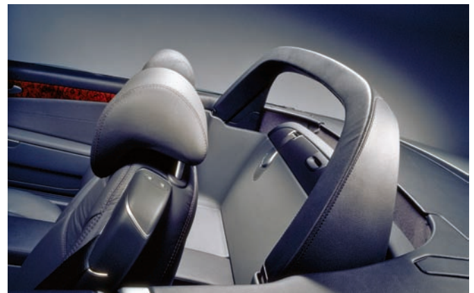
Figure 24-32 This roll bar pops out when the system anticipates a potential rollover. Courtesy of Chrysler LLC
