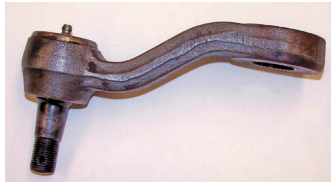
Figure 46-3 A typical pitman arm. It connects the steering column to the center link.
