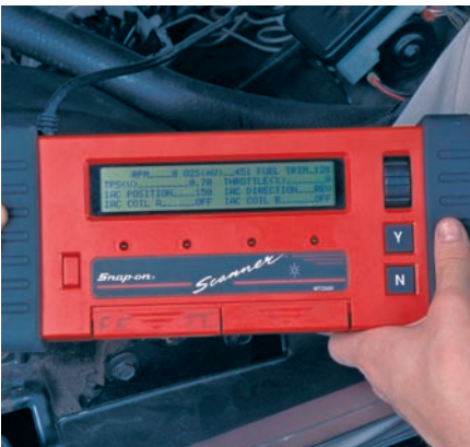
P24-7 Retrieve the DTCs with the scan tool. Interpret the codes by using the service manual.
