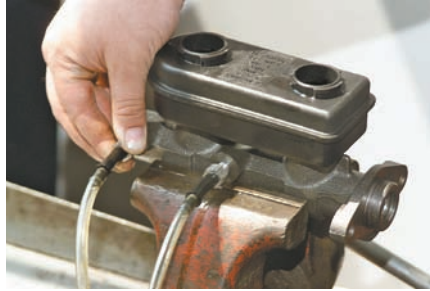
P51-2 Connect short lengths of tubing to the outlet ports, making sure the connections are tight.
