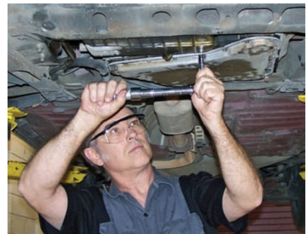
P42-9 Install the pan onto the transmission. Install and tighten the bolts to specifications. Then lower the vehicle and pour new fluid into the transmission. Run the engine to circulate the new fluid, then turn it off and raise the vehicle. Check for fluid leaks.
