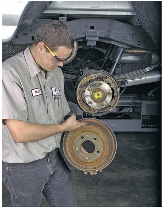
Figure 49-18 Carefully check the inside surface of the brake drum.
