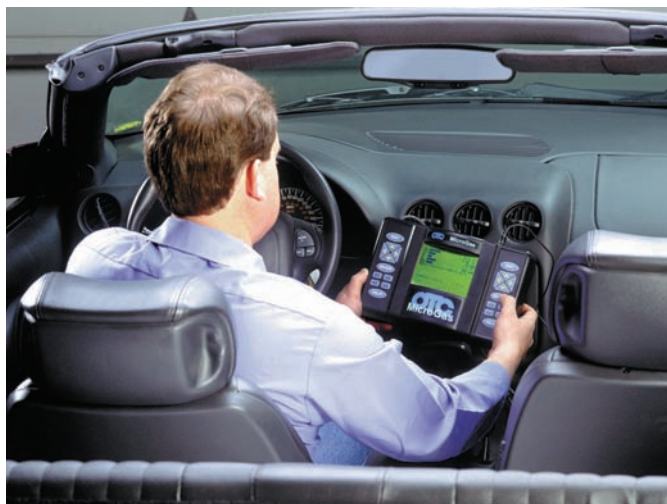
Figure 5-28 Using a scan tool during a road test. Courtesy of SPX Service Solutions
