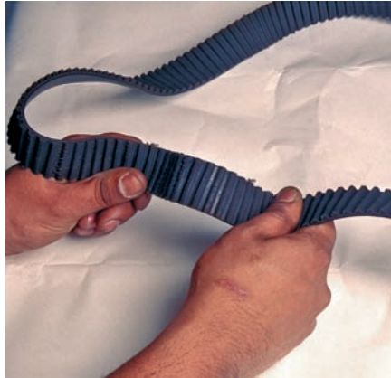
P10-8 After the belt has been removed, inspect it for cracks and other damage. Cracks will become more obvious if the belt is twisted slightly. Any defects in the belt indicate it must be replaced.
