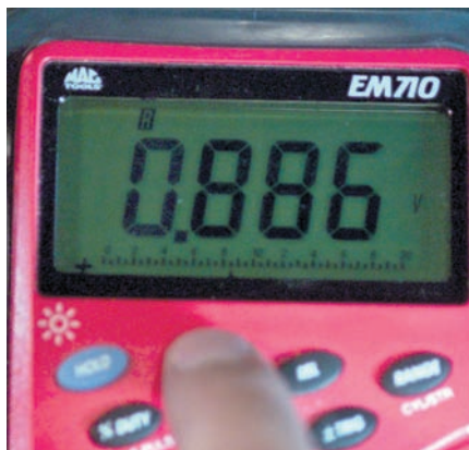
P26-8 Press the Min/Max button again to observe the maximum voltage reading. This should be about 0.9 volt.
