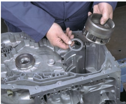
P43-25 Check the end play of the carrier in the reaction gear set. Then install the thrust washer and carrier assembly into the case. Rotate the carrier until the pinions engage with the reaction sun gear.
