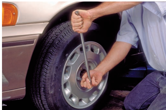
Figure 10-13 Use a large breaker bar to loosen the axle shaft hub nuts.
