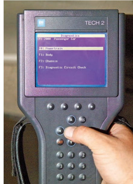
P28-3 Program the scan tool for the vehicle and system being tested.
