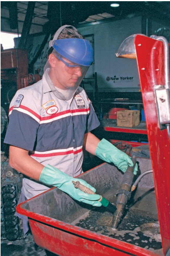
Figure 6-3 Polyurethane or vinyl gloves should be worn when handling strong and dangerous caustic chemicals.
