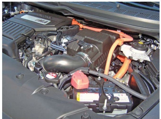
Figure 6-16 The high-voltage cables on this Civic hybrid are colored orange and are enclosed in orange casing.
