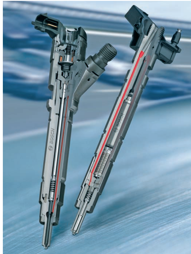
Figure 33-39 A solenoid-operated injector (left) and a piezo-inline injector (right); both are commonly used in diesel common rail systems. Courtesy of Robert Bosch GmbH, www.bosch-presse.de
