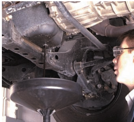
P3-5 Make sure the drain pan is positioned so it can catch all of the oil.
