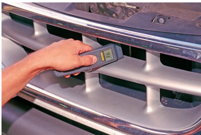
Figure 53-15 Measure the temperature of the air entering the condenser.
