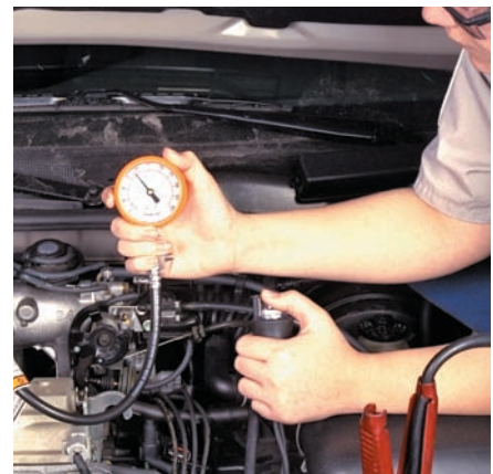
P6-9 Allow the engine to turn through four revolutions, and observe the reading after the fourth. The reading should increase with each revolution.
