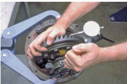
P41-10 Adjust the backlash by turning both adjusting nuts in equal amounts so that the preload adjustment remains unchanged.
