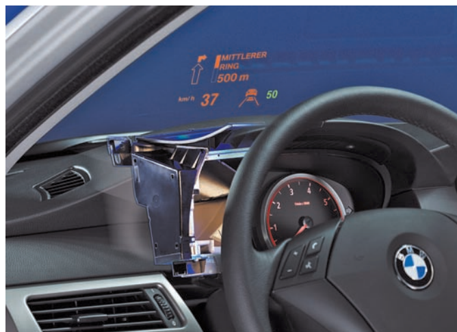
Figure 21-21 The heads-up display (HUD) can project the vehicle's speed onto the windshield, freeing the driver from looking down at the speedometer. Courtesy of Siemens VDO Automotive AG
