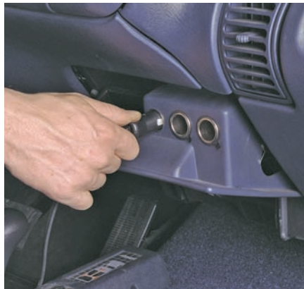
P33-5 Turn off the engine and connect the power cable of the scan tool to the vehicle.
