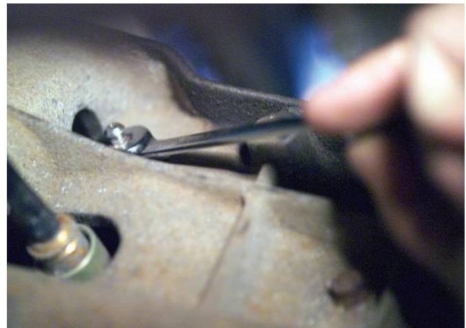
Figure 36-31 Make sure the bleeder screw is tight after the system has been bled.
