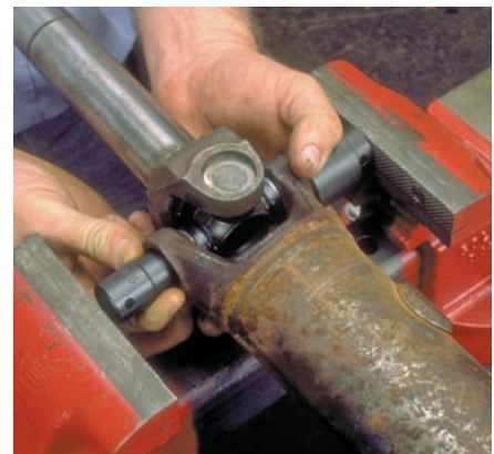
P38-6 Position the other socket to the center of the bearing cup opposite to the one in line with the large socket.
