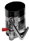
Figure 5-7 A piston ring compressor. Reproduced under license from Snap-on Incorporated. All of the marks are marks of their owners.
