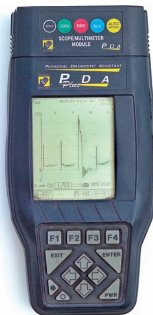
Figure 28-48 The scope pattern for a COP system with one faulty cylinder.
