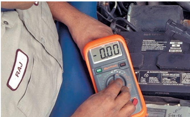
P15-4 Set the voltmeter to the scale that is close to, but greater than, battery voltage.
