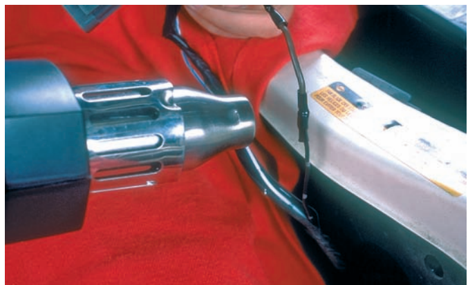
P13-12 Heat the tube with the hot air gun until it shrinks around the splice. Do not overheat the heat shrink tube.
