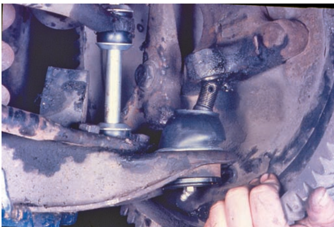
Figure 45-34 At times the steering knuckle must be disconnected from the lower and/or ball joint in order to remove a spring.
