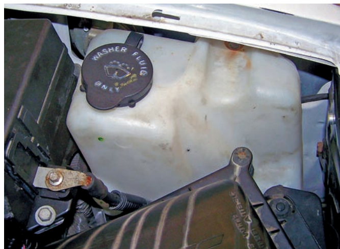
Figure 7-36 Check the level of the windshield washer fluid at the reservoir.
