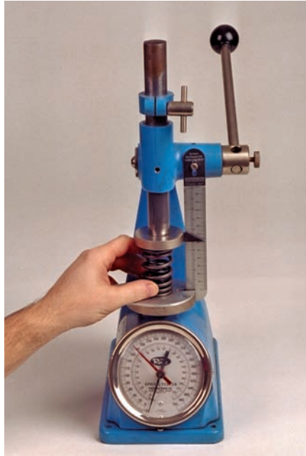
P9-8 Spring tension must be checked at the installed spring height; therefore, if a shim is to be used, insert it under the spring on the valve spring tension gauge.
