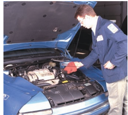
P3-16 After the engine has been turned off, recheck the oil level and correct it as necessary.
