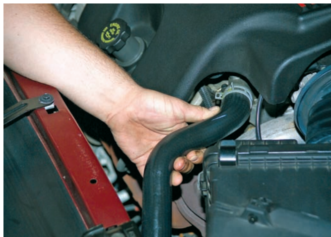
Figure 14-46 The operation of the water pump can be checked by squeezing the upper radiator hose while accelerating the engine. If a surge is felt in the hose, the pump is working.
