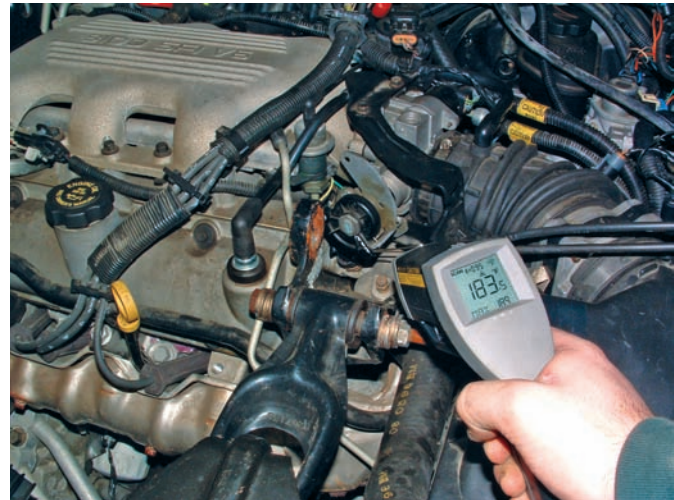
Figure 5-39 A hand-held digital infrared temperature gauge.
