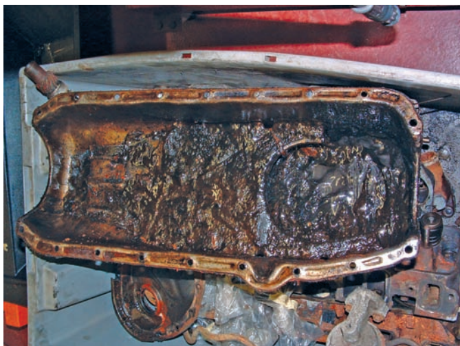
Figure 10-23 A major buildup of sludge on the bottom of this oil pan.
