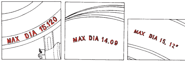
Figure 49-24 The drum's discard diameter is stamped on the drum.
