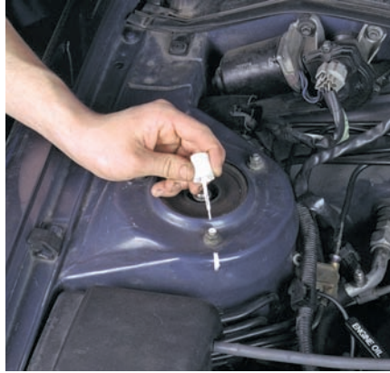
P49-2 Prior to loosening the strut chassis bolts, scribe alignment marks on the strut bolts and the chassis.
