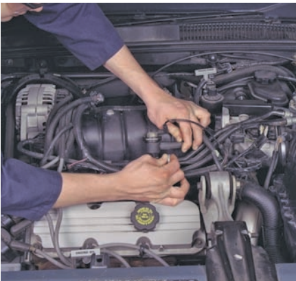
P30-3 The supply line into the fuel rail is a likely point of leakage. Check the area around the fitting to make sure no leaks have occurred.
