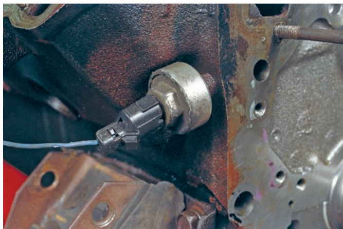
Figure 9-43 The oil pressure gauge is installed into the oil pressure sending unit's bore in the engine block.
