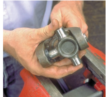
P39-6 Remove the shaft from the vise and push the cross toward the other side of the yoke.
