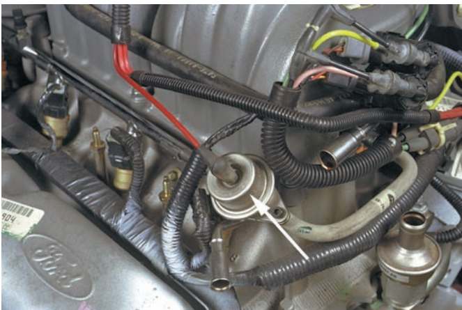
Figure 30-16 A typical fuel pressure regulator for a port injection system.
