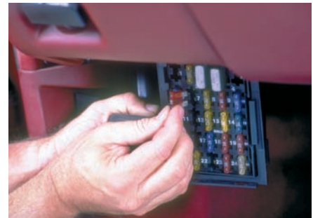
P22-6 Remove the SIR fuse from the fuse box. Wait 30 minutes to allow the reserve energy to dissipate.
