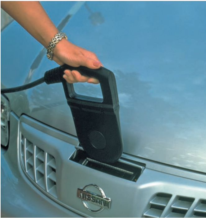
Figure 35-14 Recharging an electric vehicle with an inductive charge. Copyright, Nissan (2008). Nissan and the Nissan logo are registered trademarks of Nissan.
