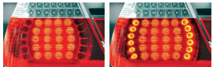
Figure 20-43 (Left) The normal illumination of the brake lights. (Right) The illumination during hard stops. Courtesy of BMW of North America, LLC
