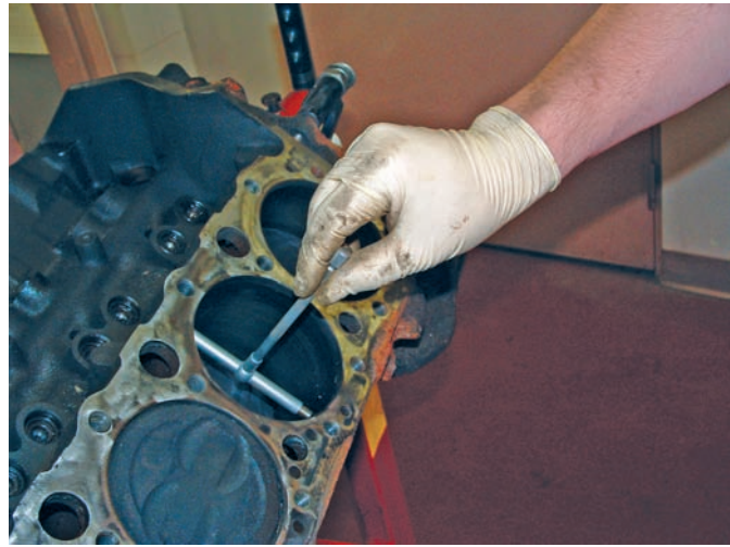
Figure 6-4 Many technicians wear thin, surgical-type latex or nitrile gloves whenever they are working on vehicles.
