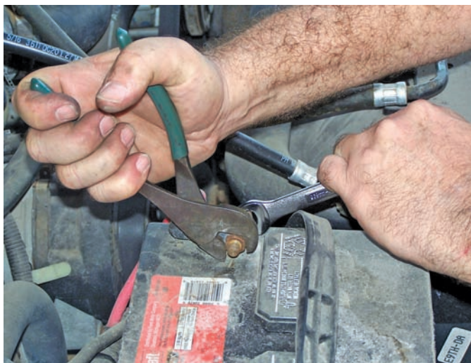
Figure 17-25 It is best to loosen a battery clamp with a box-end wrench and/or cable-clamp pliers.
