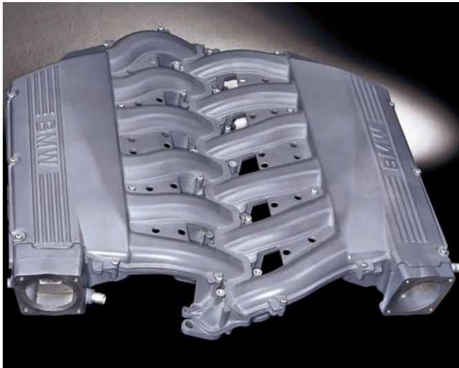
Figure 32-7 A die-cast aluminum intake manifold. Courtesy of BMW of North America, LLC
