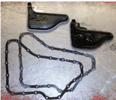
P42-7 Compare the replacement gasket and filter with the old ones to make sure the replacements are the right ones for this application.
