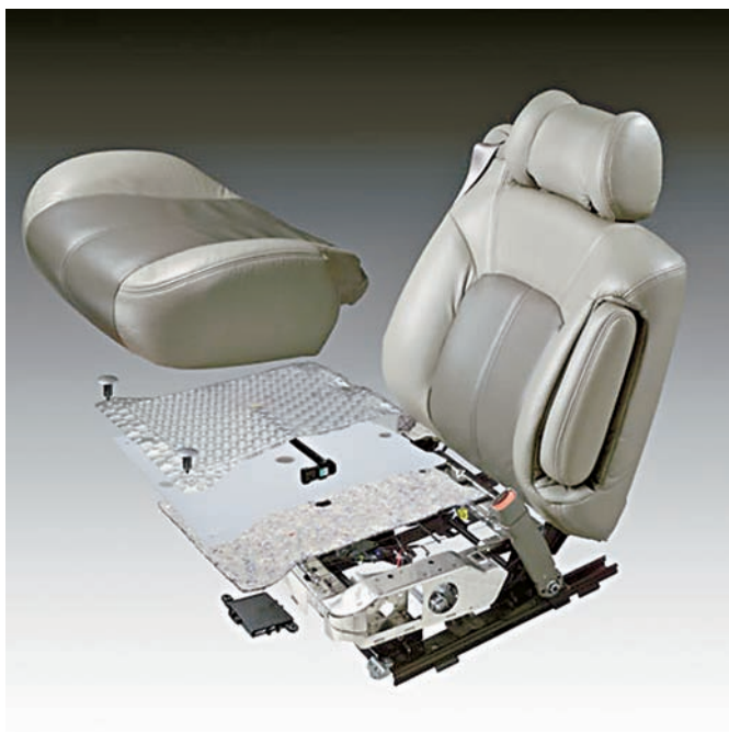
Figure 24-15 An occupant detection system with a seat belt tension sensor. Courtesy of Delphi Corporation
