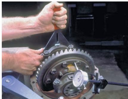
P41-8 Determine how much the preload needs to be adjusted and set the preload by turning the right adjusting nut.
