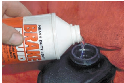
P51-11 When there are no air bubbles in the fluid, tighten the connections to the manufacturer's specifications. Make sure the master cylinder reservoirs are adequately filled with brake fluid.
