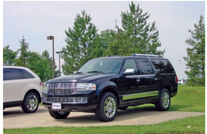
Figure 3-12 This Lincoln Navigator is an excellent example of a large SUV, and it is based on a truck chassis.
