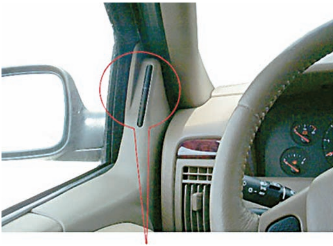
Figure 23-28 The infrared sensor for a smart window system. Courtesy of Delphi Corporation
