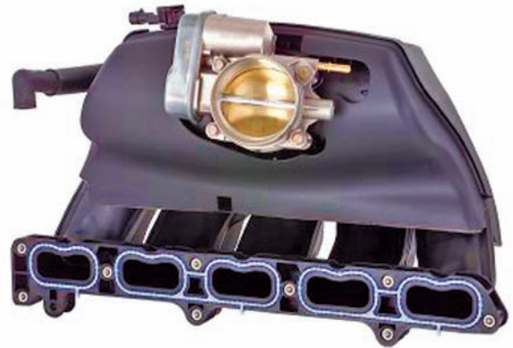
Figure 32-8 A plastic intake manifold for an inline five-cylinder engine. Courtesy of BMW of North America, LLC
