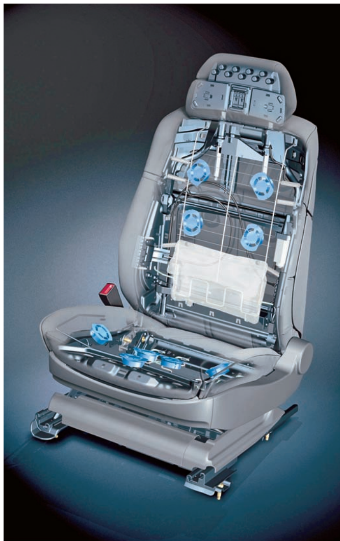
Figure 23-33 This seat features ventilation, heating, and multiple position adjustments, including the headrest and lumbar support; the small round things are fans. Courtesy of the BMW of North America, Inc.
