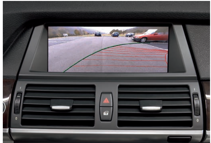
Figure 23-41 During self-parking, the driver must define the parking space on a screen in the instrument panel or the navigation display. Courtesy of BMW of North America, LLC
