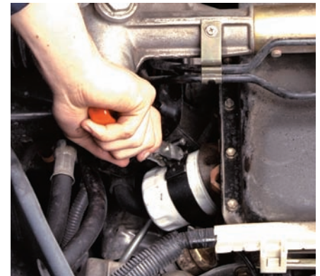
P3-6 While the oil is draining, use an oil filter wrench to loosen and remove the oil filter.
