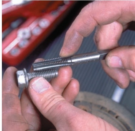
P1-2 Select the correct size and type of tap for the threads and bore to be repaired.
