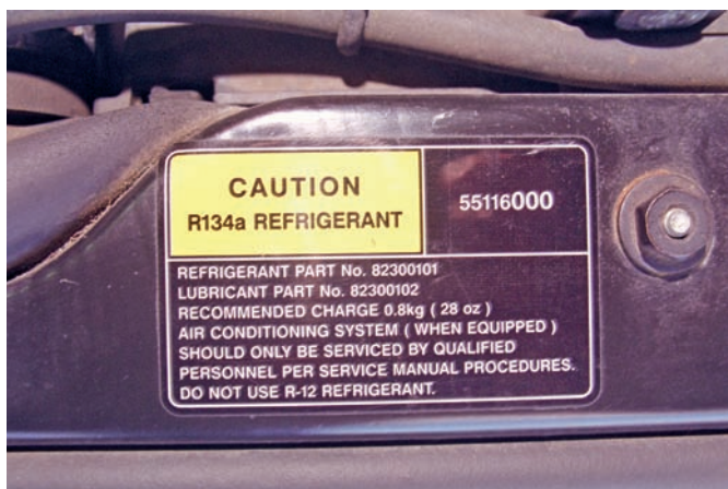
Figure 52-11 A typical decal informing the technician that the system uses R-134a.
