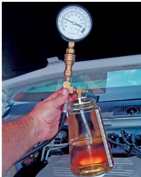
Figure 29-31 The setup for checking the fuel pump volume.
