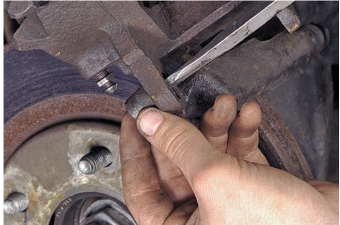
P52-8 Check the condition of the locating pin insulators and sleeves.
