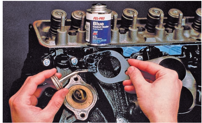
Figure 13-26 Applying gasket sealer with a brush. Courtesy of Federal-Mogul Corporation
