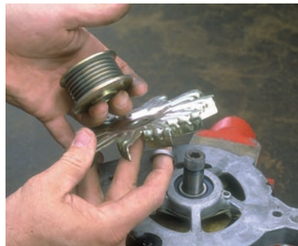
P17-14 Remove the pulley-attaching nut, flat washer, drive pulley, fan, and fan spacer from the rotor shaft.
