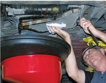
P42-4 Support the pan with one hand and remove the remaining bolts to remove the pan. Pour the fluid in the pan into the drain pan.
