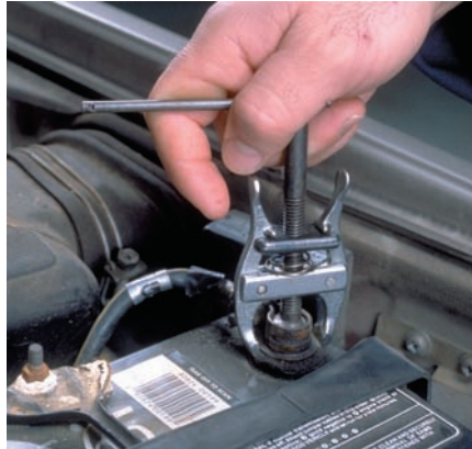
P5-2 Use a terminal clamp puller to remove the negative cable.
