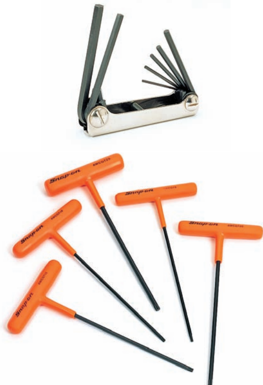
Figure 4-33 Top: A handy tool containing many different Allen wrenches. Bottom: Tee-handle Allen wrenches designed for better gripping and easier torque application. Reproduced under license from Snap-on Incorporated. All of the marks are marks of their owners.
