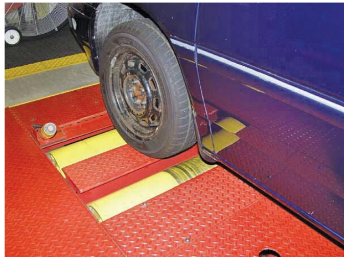
Figure 34-5 The wheels of this vehicle are ready to be dropped into the rollers of a chassis dynamometer.
