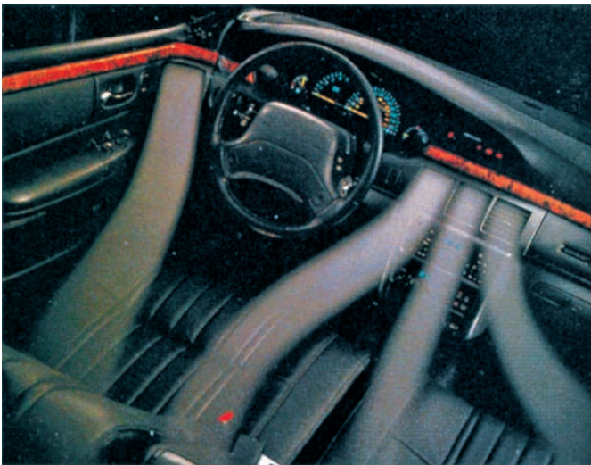
Figure 52-38 Air moving out from the dash vents to create comfort zones for the driver and passengers. Courtesy of Chrysler LLC
