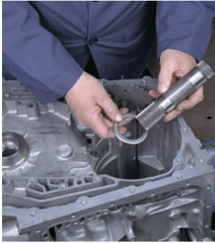
P43-18 Remove the reaction sun gear thrust bearing and final drive sun gear shaft.
