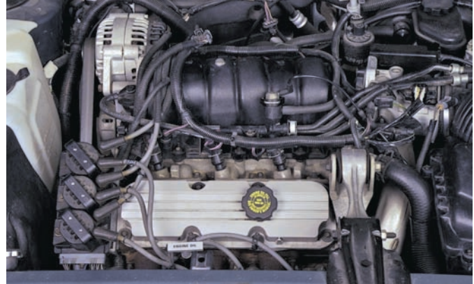
P30-2 Prior to testing the fuel pump, a careful visual inspection of the injectors, fuel rail, and fuel lines and hoses is necessary. Any sign of a fuel leak should be noted and the cause corrected immediately.
