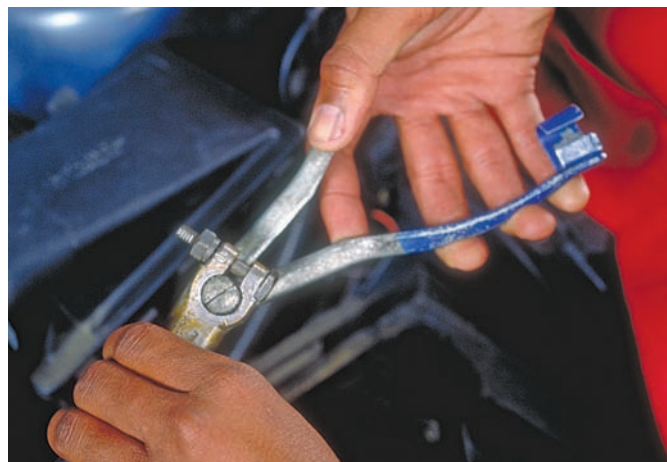
Figure 17-27 Before reinstalling the cable end onto the battery, use terminal end expanders to make sure the end does not need to be forced onto the battery post.
