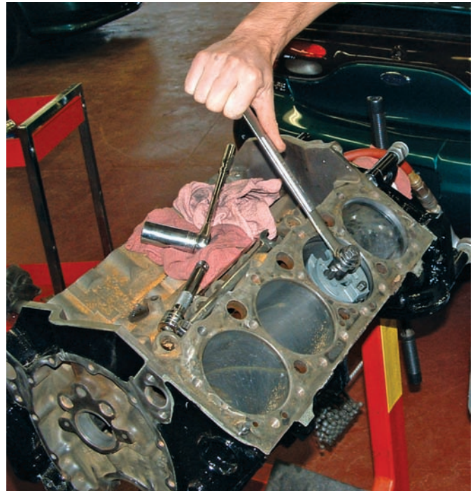
Figure 11-5 A ridge reamer should be used on all cylinders before removing the pistons.
