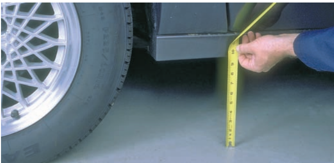
P47-5 Measure and record the right front curb riding height.
