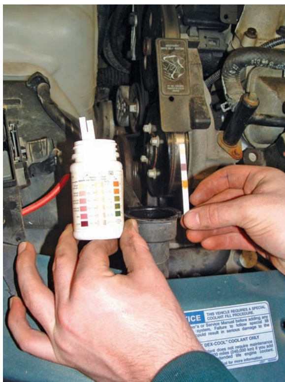
Figure 8-58 Litmus test strips can be used to check the condition of an engine's coolant.
