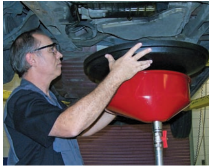
P42-2 Place a large-diameter oil drain pan under the transmission pan.
