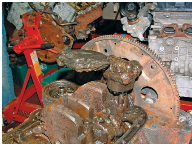
Figure 14-14 Sludge buildup on the lower parts of an engine.
