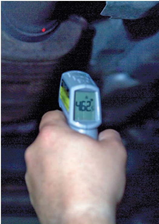
Figure 34-34 Compare the outlet temperature with the inlet to see how efficient the converter is.
