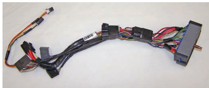
Figure 15-61 A typical partial wiring harness that connects to a connector on the fire wall.
