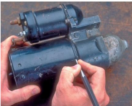
P16-3 Scribe reference marks at each end of the starter end housings and the frame.
