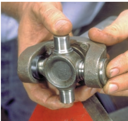
P39-7 Start a cup into the yoke's ear and over the trunnion.
