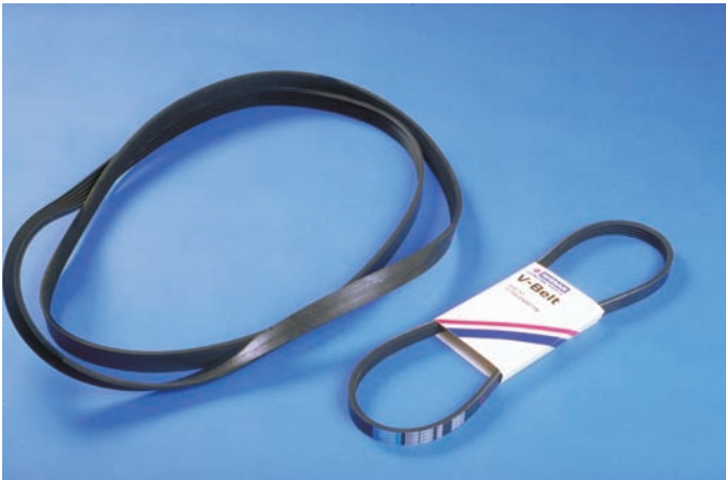
Figure 7-24 The size and part number of a new belt are given on the belt container. The size can be verified by physically comparing the old with the new belt.
