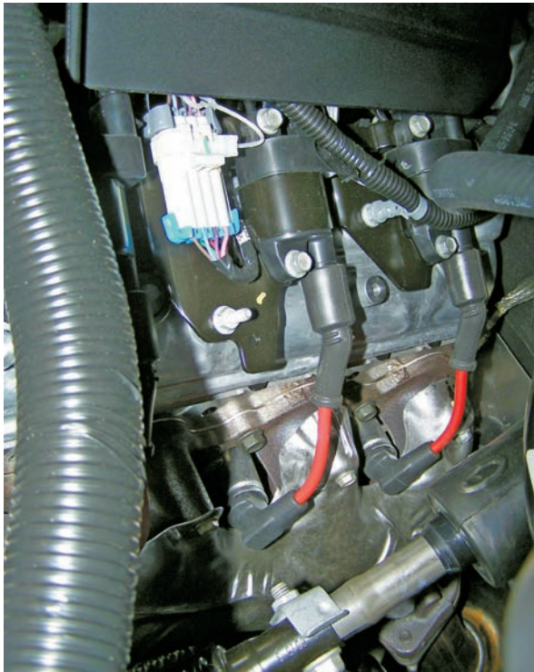
Figure 27-30 A coil-near-plug system.
