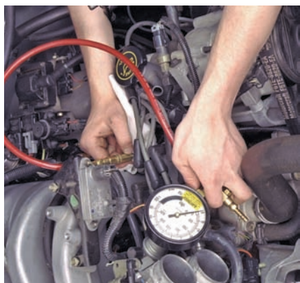
P29-4 Connect the fuel pressure gauge to the Schrader valve.
