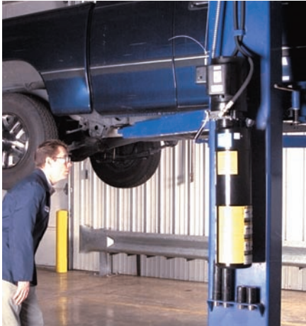
P3-1 Always make sure the vehicle is positioned safely on a lift or supported by jack stands before working under it. Before raising the vehicle, allow the engine to run awhile. After it is warm, turn off the engine.
