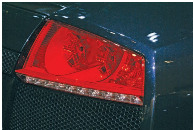
Figure 20-36 A stylish taillight assembly using LED technology.
