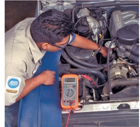
P15-3 Connect the negative lead to the battery connection at the starter.
