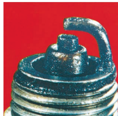
Figure 28-55 A wet- or oil-fouled spark plug. Courtesy of Federal-Mogul Corporation
