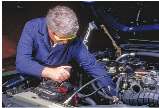
Figure 9-37 Rotate the engine so that the piston of the cylinder that will be tested is at TDC before checking leakage.
