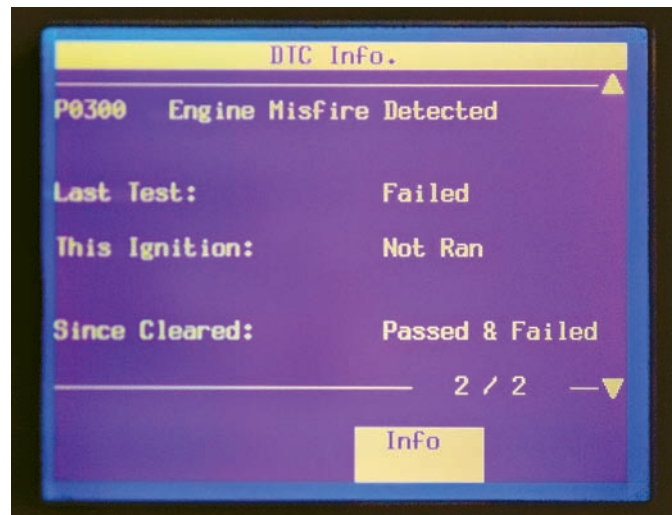
Figure 28-1 The PCM will store a DTC when it detects a misfire.
