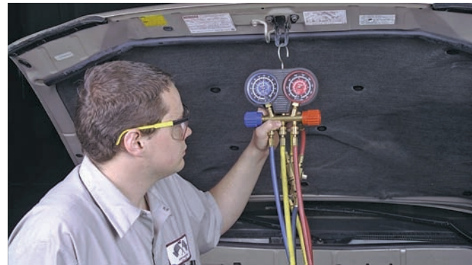
P53-5 Activate the reclaimer to discharge the system, then begin evacuation. Allow enough time for the machine to draw a good vacuum (at least 29 in. Hg) in the system. Observe the gauge set to determine when a vacuum is created.
