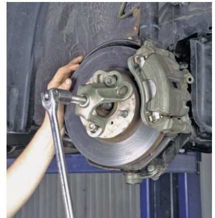
P37-6 A special tool is normally needed to separate the axle shaft from the hub allowing the axle to be removed from the car. Never hit the end of the axle with a hammer.
