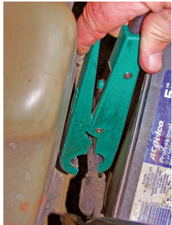
Figure 18-28 It is important to remember to move the inductive lead to the vehicle's system after checking the battery.
