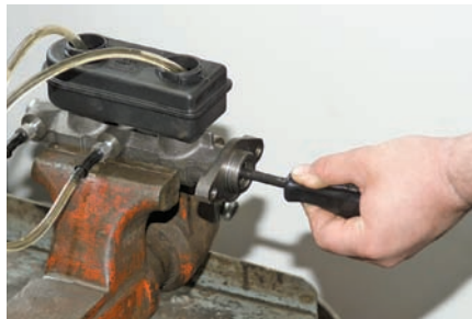
P51-5 Using a wooden dowel or the blunt end of a drift or punch, slowly push on the master cylinder pistons until both are completely bottomed out in their bore.
