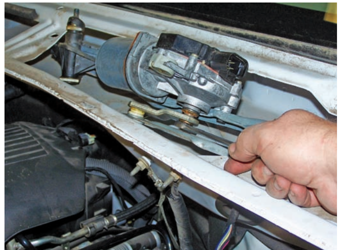
Figure 23-13 Disconnecting the wiper linkage arms at the wiper motor.
