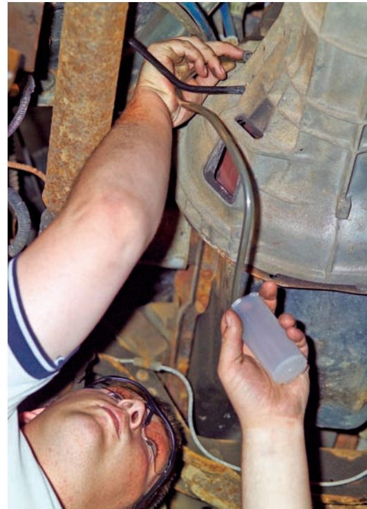
Figure 36-30 Attach a hose between the bleeder screw and a container before beginning to bleed the system.
