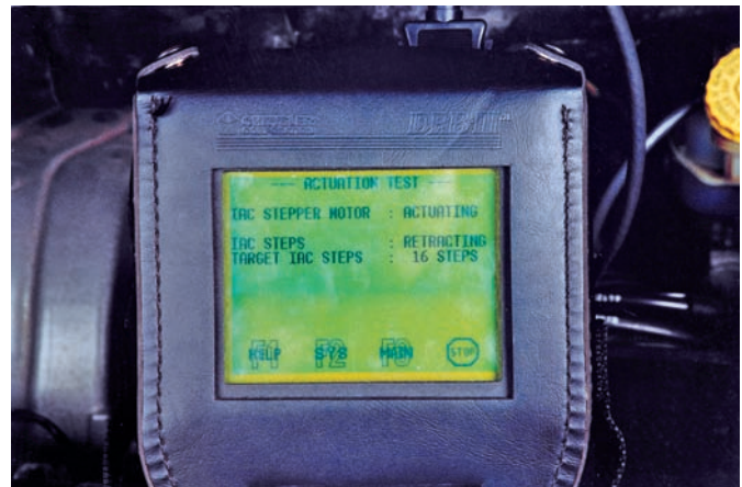
Figure 31-30 When the IAC is operated in its low range, the PCM will move the IAC in approximately 16 steps.
