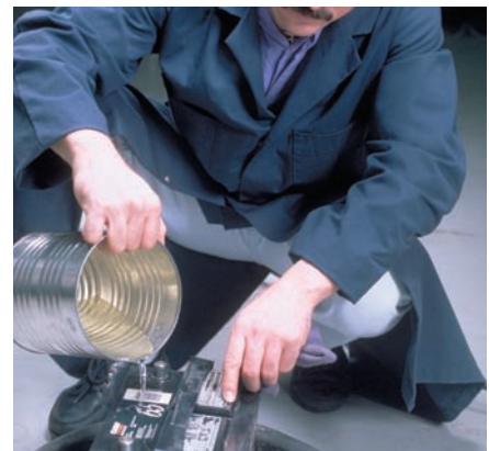
P5-9 Flush the baking soda off with water.
