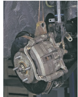
P49-7 Support the steering knuckle with wire and remove the strut assembly from the car.
