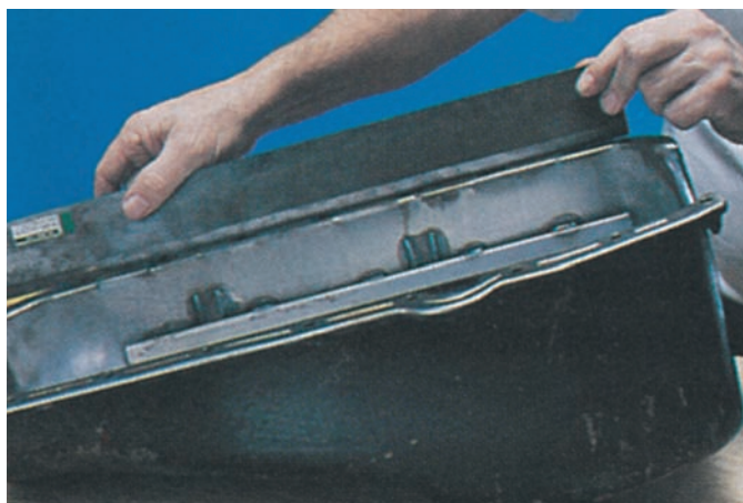
Figure 13-42 Checking the flatness of an oil pan flange. Courtesy of Detroit Gaskets
