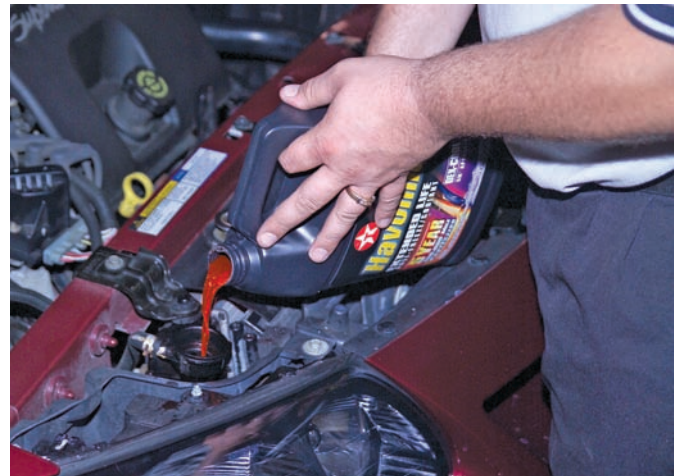
Figure 7-14 Ethylene glycol is the most commonly used antifreeze/coolant and is green in color. OAT coolant is orange and is often referred to by a brand name “DEX-COOL.”
