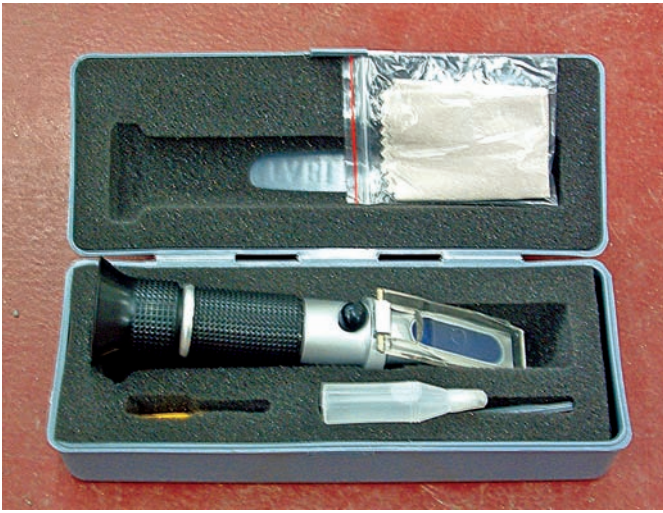
Figure 5-16 A refractometer checks the condition of the engine's coolant.
