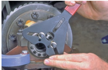
P41-5 Turn each adjuster until bearing free play is eliminated with little or no backlash present between the ring and pinion gears.
