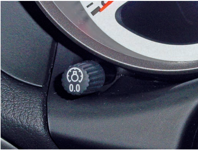
Figure 20-16 An instrument panel light control switch. This switch also resets the trip odometer.
