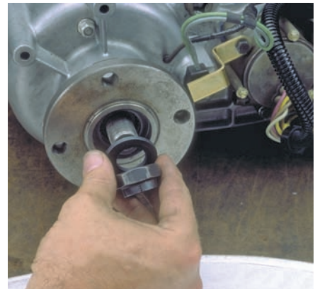
P45-18 Install the companion flanges' seal, washer, and nut. Then tighten the nut to specifications.
