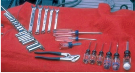
P22-1 Tools required to remove the air bag module: safety glasses, seat covers, screwdriver set, Torx driver set, battery terminal pullers, battery pliers, assorted wrenches, ratchet and socket set, and service manual.
