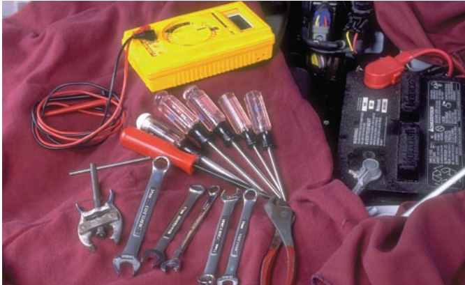
P18-1 The tools required to test and remove a multifunction switch are fender covers, battery terminal pliers and pullers, assorted wrenches, Torx driver set, and an ohmmeter.
