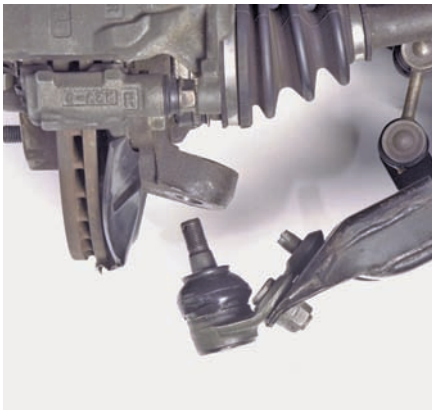
P37-4 The ball joint must be separated from the steering knuckle assembly. To do this, first remove the ball joint retaining bolt. Then pry down on the control arm until the ball joint is free.
