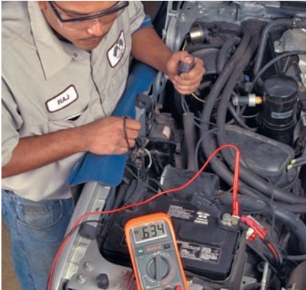
P15-8 Crank the engine and observe the reading on the meter. This is the voltage drop across the positive circuit from the battery to the output of the relay.
