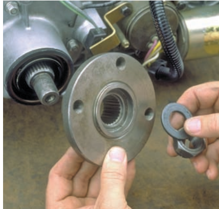
P44-2 Remove two output shaft yoke nuts, washers, rubber seals, and output yokes from the case.
