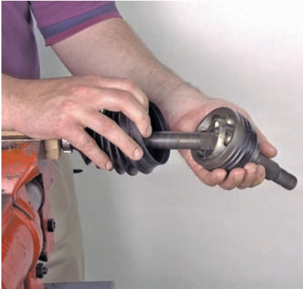
P37-10 Remove the circlip and separate the joint from the shaft.
