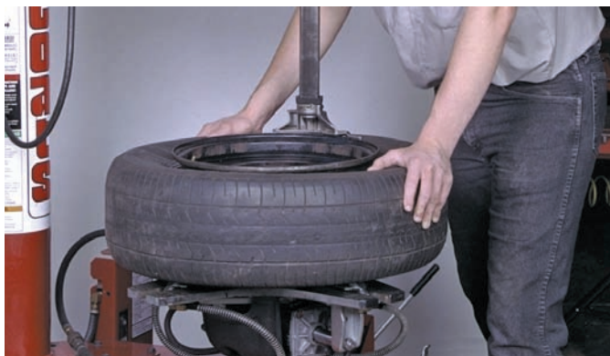
P46-7 Place the tire onto the wheel and lower the arm into place. As the machine rotates the wheel, the arm will force the tire over the rim. After the tire is completely over the rim, install the air ring over the tire. Activate it to seat the tire against the wheel.
