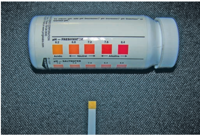
Figure 7-17 Matching the color of a test strip to the scale on its container will indicate the freeze protection level and the acidity of the coolant.
