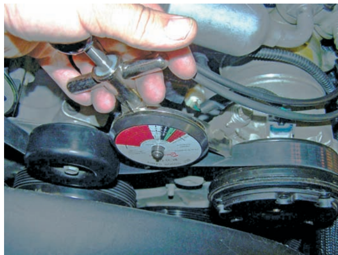
Figure 7-23 Check the tension of a drive belt with a belt tension gauge.
