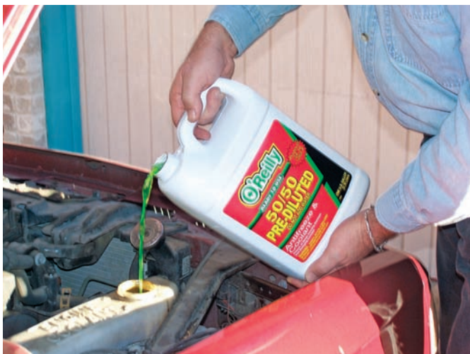
Figure 7-13 Topping off the cooling system with a 50/50 mixture of antifreeze and water.
