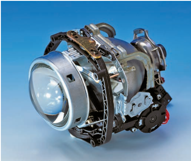
Figure 20-23 A headlamp assembly for an adaptive headlight system. Courtesy of Chrysler LLC
