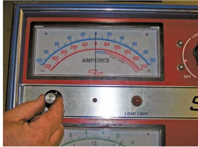
P14-6 Turn the "Zero Adjust" knob on the tester until the ammeter reads zero.
