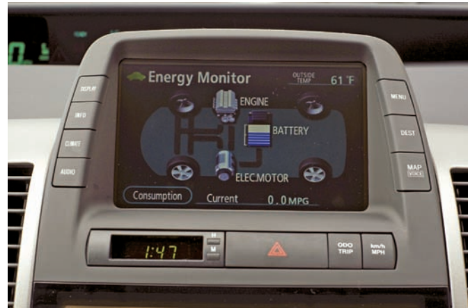
Figure 21-23 The energy monitor for a Toyota Prius. Courtesy of Toyota Motor Sales, U.S.A., Inc.
