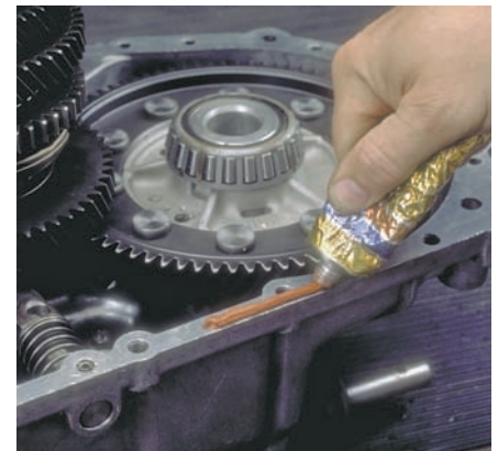
P36-15 Apply a thin bead of anaerobic sealant on the case's mating surface for the clutch housing.
