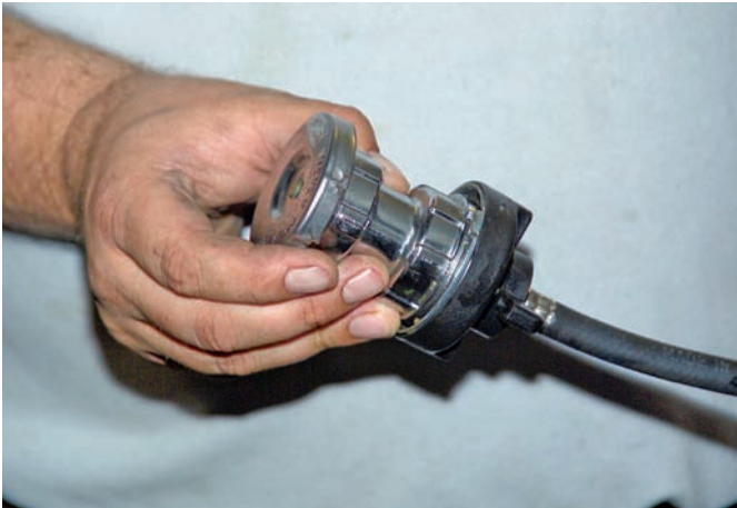
P11-5 Using the appropriate adapter, mount the pressure cap to the tester.
