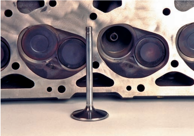
P9-1 Prior to installing the valve and fitting valve springs, all other head work should be completed.
