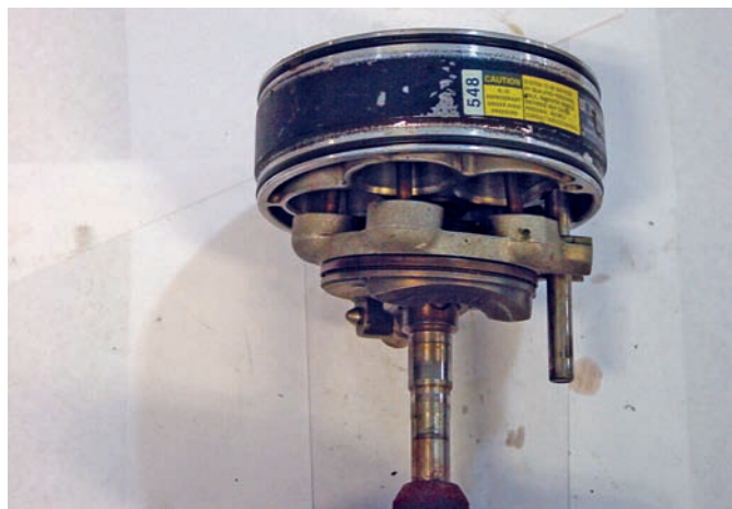
Figure 52-18 The pistons are driven by a short pushrod that connects the pistons to the wobble plate.
