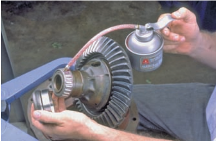
P41-1 Lubricate the differential bearings, cups, and adjusters.
