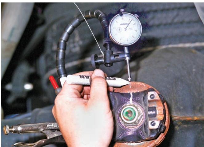
Figure 39-22 The setup for checking the runout of a companion flange.
