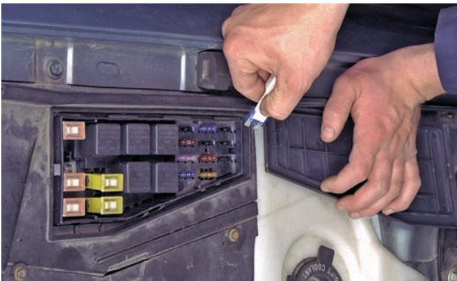
P32-3 Prior to loosening any fitting in the fuel system, the fuel pump fuse should be removed.
