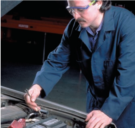
P5-1 Loosen the battery negative terminal clamp.
