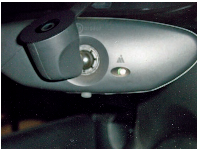
Figure 20-21 A photocell for an automatic lighting system.
