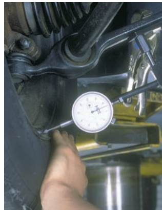
P48-5 With the tire held outward, read the dial indicator.
