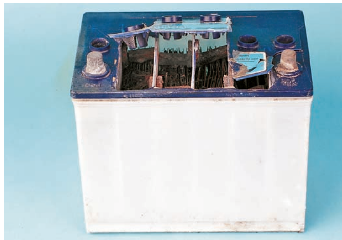
Figure 17-41 Careless use of a battery charger caused this battery to explode.
