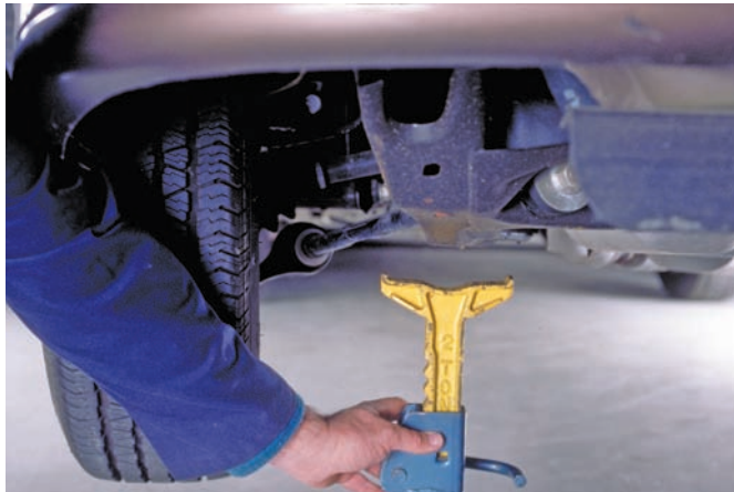
Figure 6-11 Jack stands should be used to support the vehicle after it has been raised by a jack.
