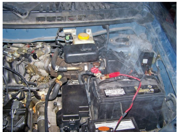
Figure 34-20 During a smoke test, smoke will be seen at all points of leakage. Be sure to inspect the entire system.
