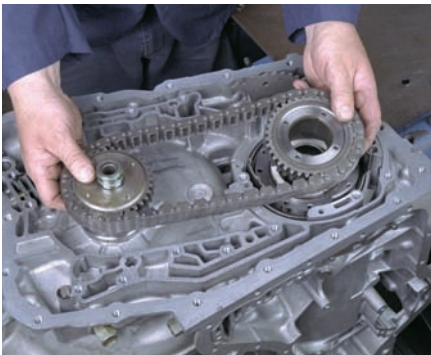
P43-13 Remove and discard the O-ring from the input shaft. Then remove the drive sprocket, driven sprocket, and chain as an assembly with the selective thrust washers.
