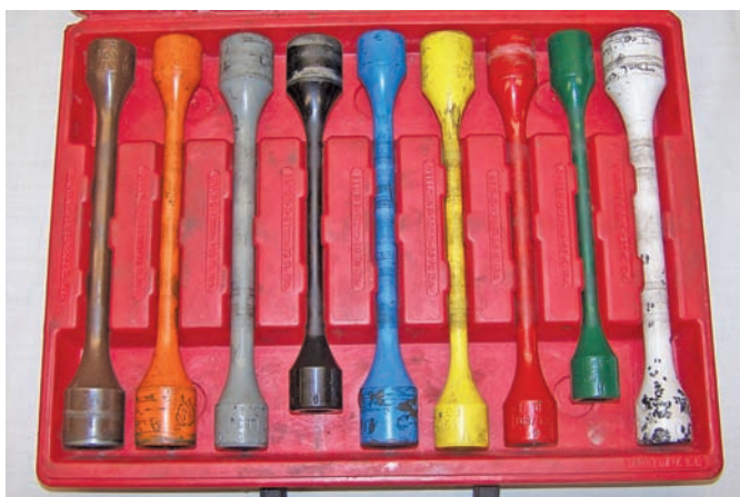
Figure 7-42 Torque sticks are color coded to indicate their torque setting.
