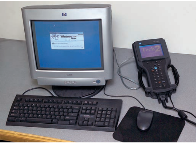
Figure 16-48 Many scan tools, DSOs, and GMMs allow for the transfer of captured information to a PC through a cable or wireless interface.
