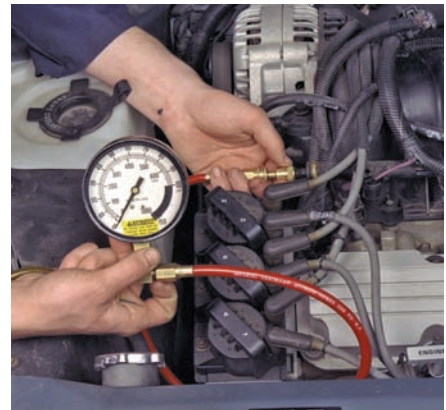
P30-5 To test fuel pressure, connect the appropriate pressure gauge to the fuel rail test fitting (Schrader valve).
