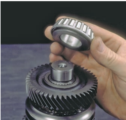
P35-13 Remove the bearing at the fourth-gear end of the mainshaft.
