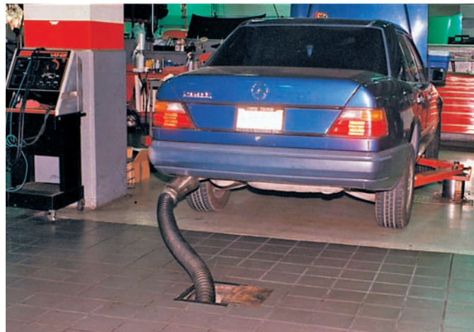
Figure 6-14 When running an engine in a shop; make sure the vehicle's exhaust is connected to the shop's exhaust ventilation system.
