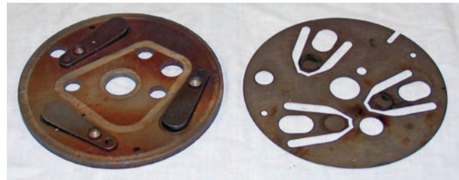
Figure 52-16 The reed valves for an A/C compressor.
