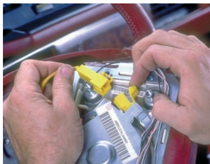
P22-11 Disconnect the electrical connectors.
