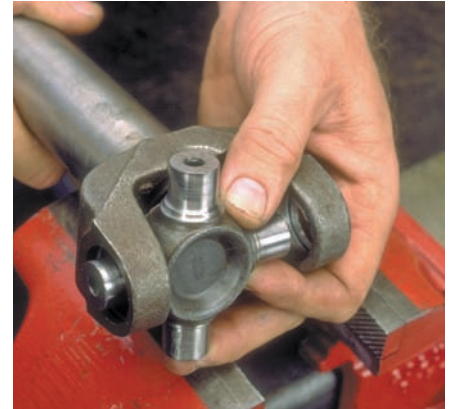
P39-3 Place the new spider inside the yoke and push it to one side.
