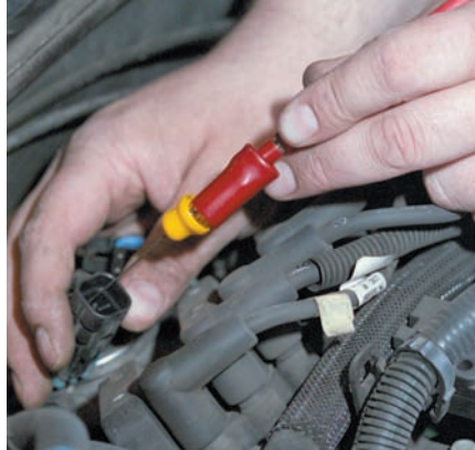
P26-2 Connect the positive lead of the meter to the power wire for the sensor's heater. Connect the meter's negative lead to a good ground.
