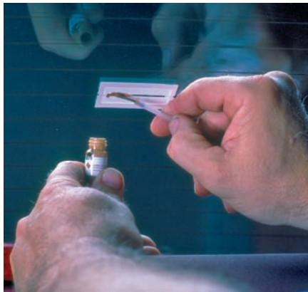
P21-5 Apply the grid repair material to the repair area using a small stick.
