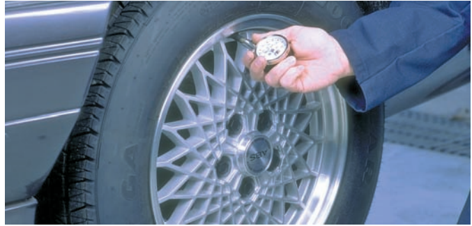
P47-2 Check the tires for normal inflation pressure.
