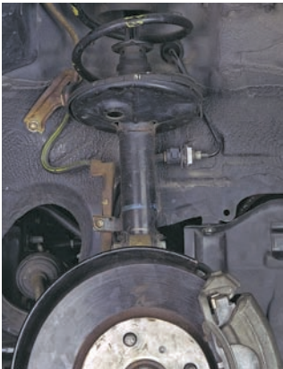
P49-4 Remove the wheel assembly. The strut is accessible from the wheel well after the wheel is removed.
