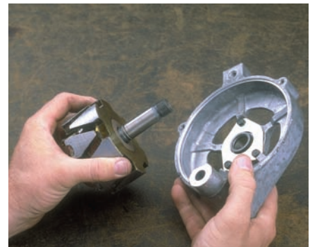
P17-15 Separate the front housing from the rotor. If the stop ring is damaged, remove it from the rotor. If not, leave it on the shaft.
