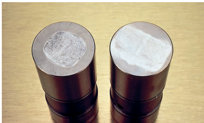
Figure 11-68 The possible wear patterns of a lifter that does not spin in its bore. Courtesy of TRW, Inc.
