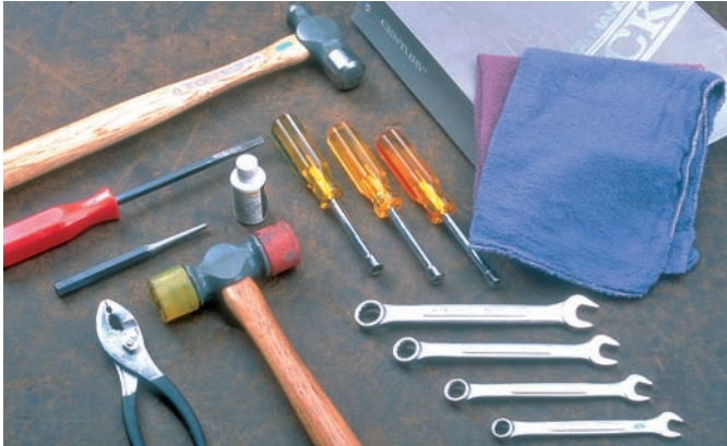
P16-1 Always have a clean and organized work area. The tools required for disassembling this starter are: rags, assorted wrenches, snapping pliers, flat blade screwdriver, ball-peen hammer, plastic head hammer, punch, scribe, safety glasses, and small press.
