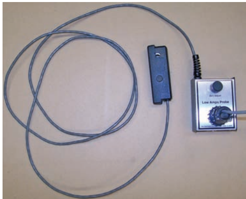
P27-3 To look at the primary circuit, connect a low-amp probe to the scope. Make sure it is compatible with the scope.
