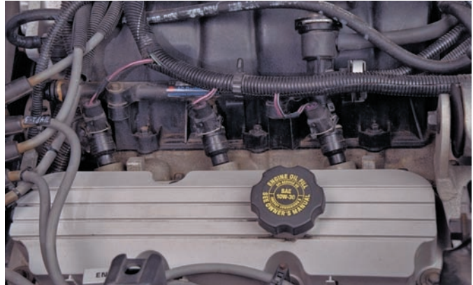
P32-2 The injectors are normally attached directly to a fuel rail and inserted into the intake manifold or cylinder head. They must be positively sealed because high-pressure fuel leaks can cause a serious safety hazard.
