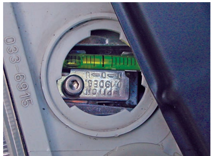
Figure 20-29 Some vehicles have a bubble level at the headlights to aid in alignment.
