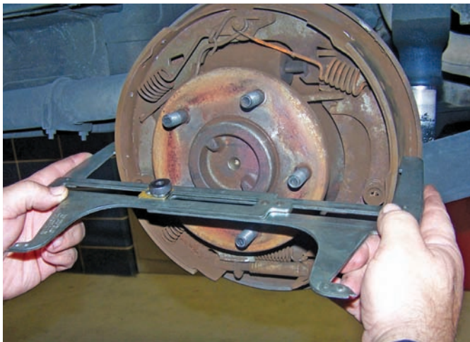
Figure 49-32 Using the other side of the brake gauge to set the brake shoes.
