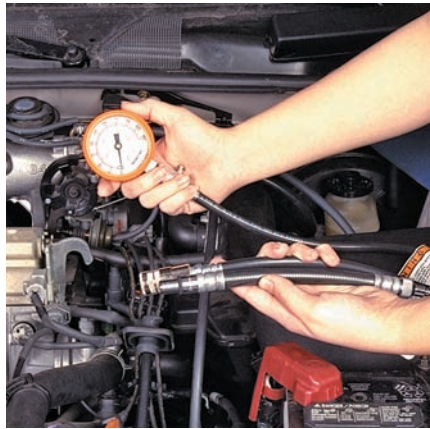
P6-5 Many types of compression gauges are available. The screw-in type tends to be the most accurate and easiest to use.
