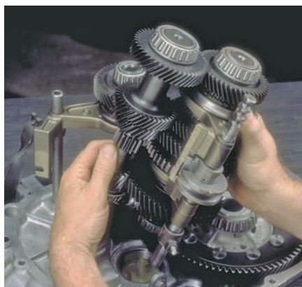
P35-8 Grasp the input and main shafts and lift them as an assembly from the case. Note the position of the shift forks as an aid when reinstalling them.
