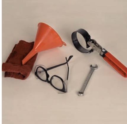
P3-2 The tools and other items needed to change the engine's oil and oil filter are rags, a funnel, an oil filter wrench, safety glasses, and a wrench for the drain plug.
