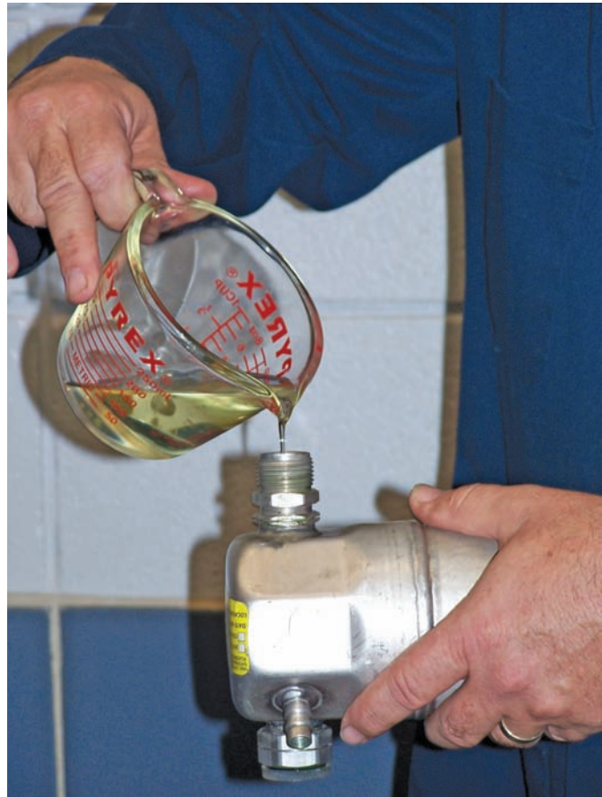
Figure 53-23 When a part is replaced, make sure to add the correct amount and type of refrigerant oil for that part to the system.
