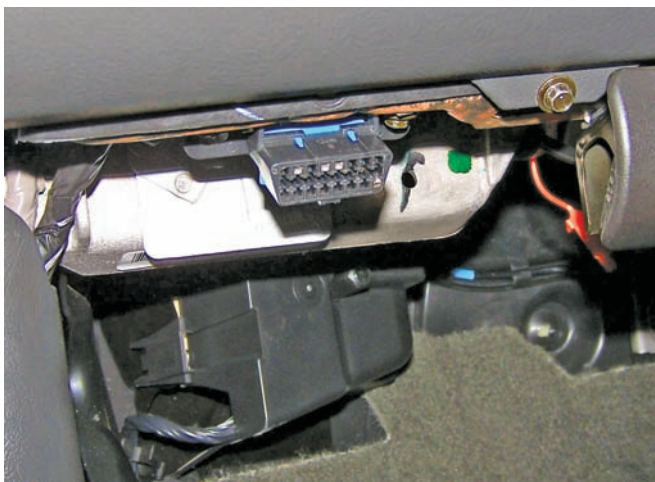
Figure 23-2 The DLC is used to access diagnostic trouble codes and serial data.
