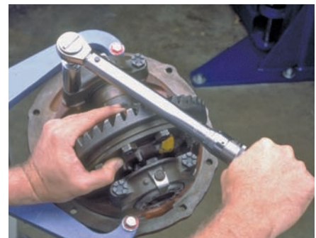
P41-12 Tighten the bearing cap bolts to the specified torque.
