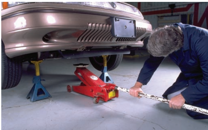
Figure 4-62 Whenever you have raised a vehicle with a floor jack, the vehicle should be supported with jack stands.
