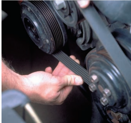
P4-1 Inspect the belt by looking at both sides.
