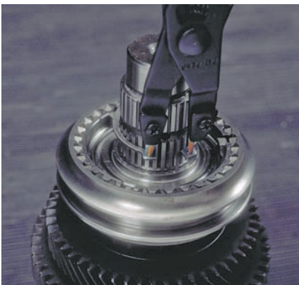
P35-16 Remove the third- and fourth-gear synchronizer retaining ring.
