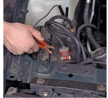
P31-3 Connect the injector pulse tester's power supply leads to the battery.
