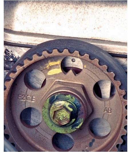
P10-3 Align the timing marks on the camshaft's sprocket with the mark on the cylinder head. If the marks are not obvious, use a paint stick or chalk to clearly mark them.
