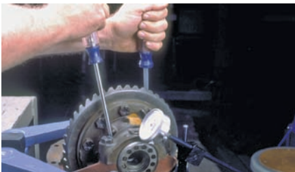
P41-7 Install a dial indicator and position the plunger against the drive side of the ring gear. Set the dial to zero. Using two screwdrivers, pry between the differential case and the housing. Observe the reading.
