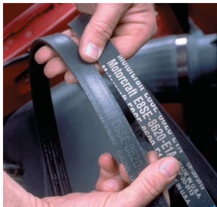
P4-7 Match the old belt up for size with the new replacement belt.
