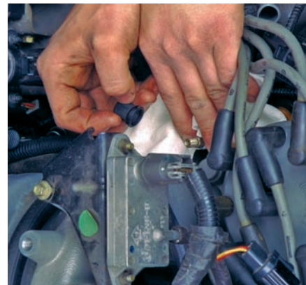
P29-3 Wrap a shop towel around the Schrader valve on the fuel rail and remove the dust cap from the valve.
