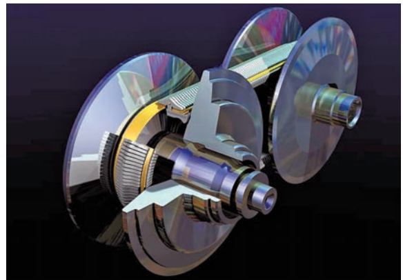
Figure 40-31 CVTs use pulleys that change size and are connected by a belt. Copyright, Nissan (2008). Nissan and the Nissan logo are registered trademarks of Nissan.
