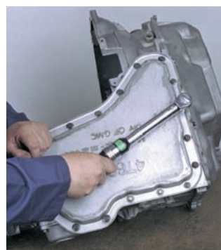
P43-45 Install the bottom oil pan, oil filter, modulator, and modulator valve.
