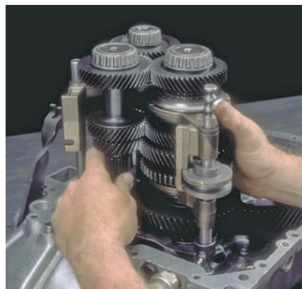
P36-8 Place the mainshaft control-shaft assembly on the mainshaft so that the shift forks engage in their respective slots in the synchronizer sleeves. Then install the mainshaft assembly.
