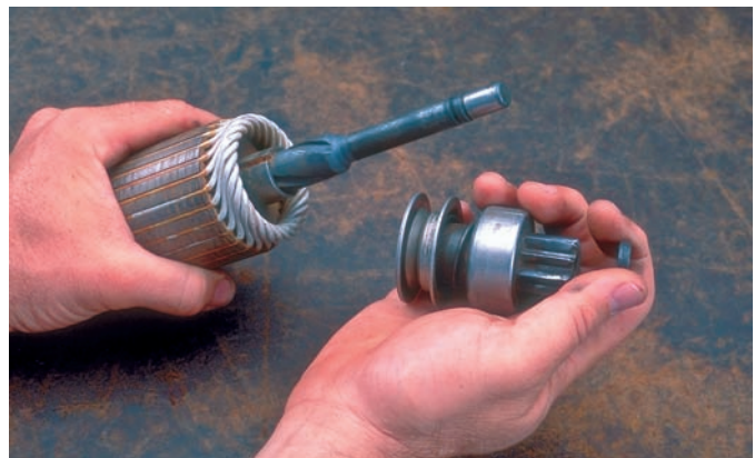
P16-14 Remove the retainer from the shaft and remove the clutch and spring from the shaft. Press out the drive housing bushing and the end-frame bushing.
