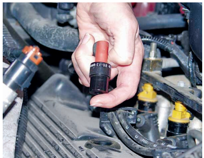
Figure 34-21 With the engine at idle, vacuum should be felt at the PCV valve.
