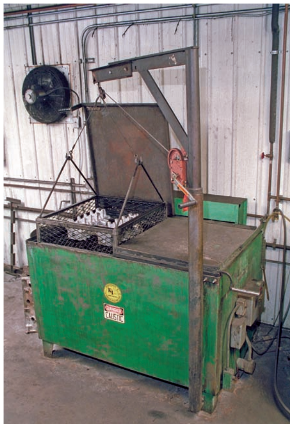
Figure 10-26 A hot soak (d.p) tank.
