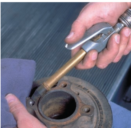
P1-7 Clean the metal chips left by the tap out of the hole.
