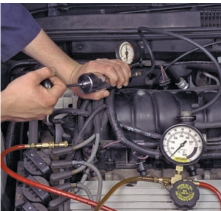
P30-6 Connect a hand-held vacuum pump to the fuel pressure regulator.
