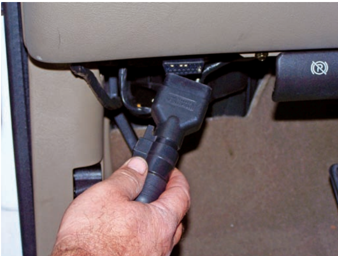
P20-8 Connect the scan tool to the DLC and turn the scan tool on.
