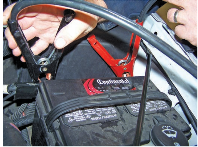
P20-7 Once downloading is complete, connect a battery charger to the vehicle's battery. Turn it on and maintain about 13.5 volts at the battery.
