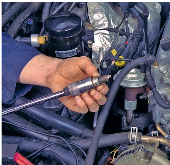
Figure 28-51 Use a spark plug socket to remove the plugs.
