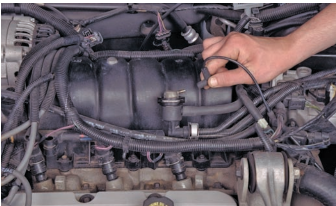
P32-5 To remove an injector, the fuel rail must be able to move away from the engine. The rail-holding brackets should be unbolted and the vacuum line to the pressure regulator disconnected.
