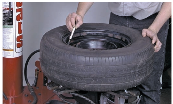
P46-8 Reinstall the valve stem core and inflate the tire to the recommended inflation.
