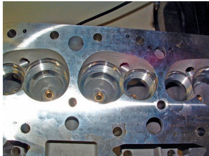
Figure 12-73 The valve to openings of this head has been bored and is ready for new seat inserts.
