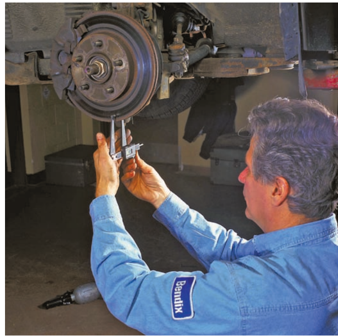
Figure 5-64 A digital caliper for measuring brake disc thickness. Courtesy of Honeywell International Inc.
