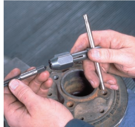
P1-3 Install the tap into a tap wrench.
