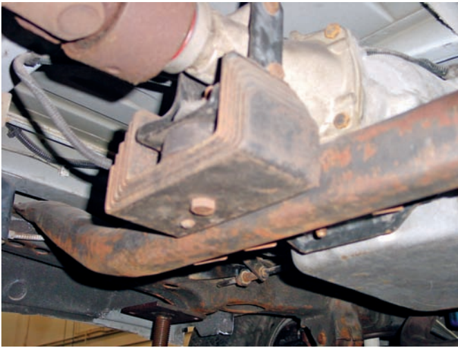
Figure 10-18 If the engine is removed with its transmission, remove the transmission mount and cross member.
