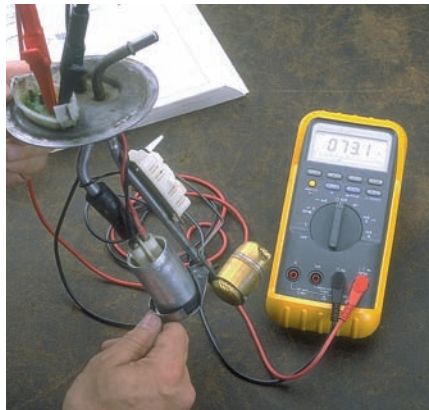
P19-5 Holding the sender unit in its normal position, place the float rod against the empty stop.
