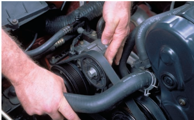
P4-4 To replace a worn belt, locate the tensioner or generator pulley.
