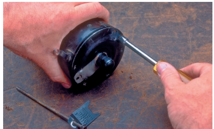
P16-7 Remove the through-bolts from the end frame.
