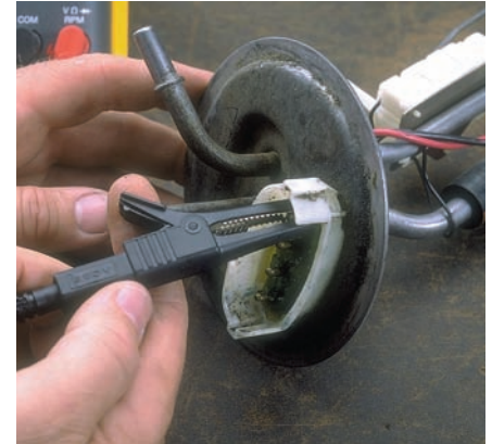
P19-3 Connect the DMM's negative test lead to the ground terminal of the sending unit.
