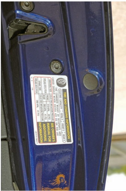
Figure 44-12 A tire placard on a door jamb. Courtesy of The Goodyear Tire & Rubber Company
