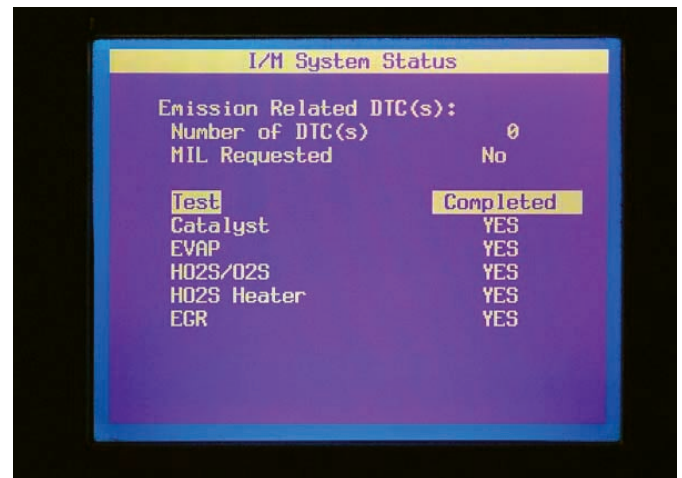
Figure 34-12 An I/M status screen on a scan tool showing the monitors have been completed.
