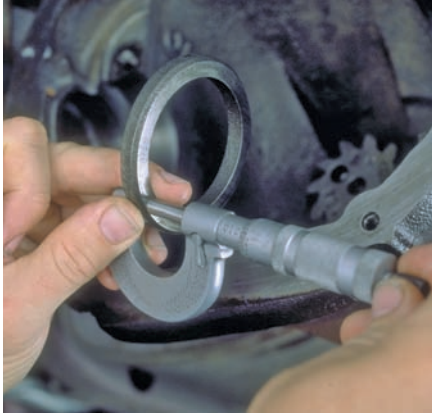
P40-1 Measure the thickness of the original side bearing preload shims.
