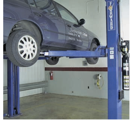
P49-3 With the top strut bolts or nuts removed, raise the car to a working height. It is important that the car be supported on its frame and not on its suspension components.
