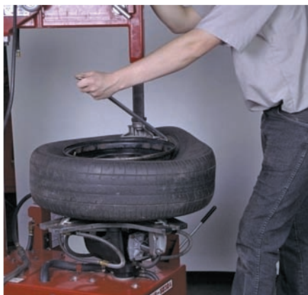
P46-4 Insert the tire iron between the upper bead of the tire and the wheel. Depress the pedal that causes the wheel to rotate. Do the same with the lower bead.
