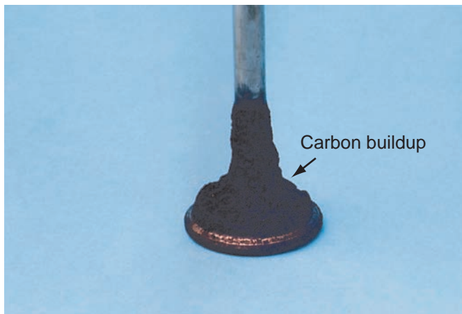
Figure 12-42 An oily soot or heavy carbon buildup on the back of the valves indicates bad valve seals.
