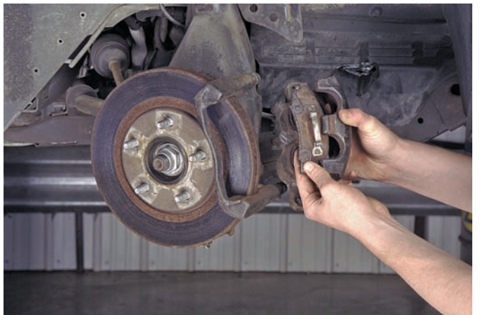
P52-6 Remove the brake pads from the caliper assembly.
