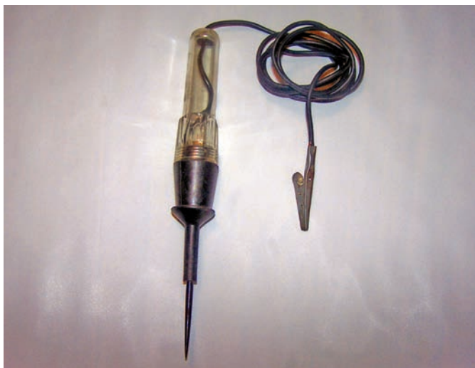
Figure 5-19 Typical circuit tester, commonly called a testlight.
