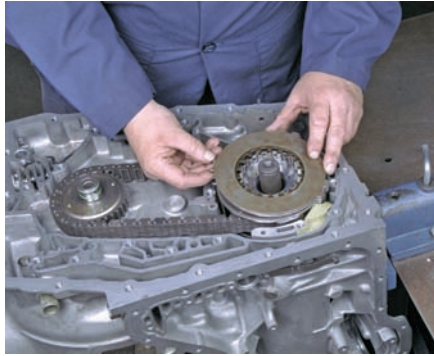
P43-37 Install the fourth clutch's thrust bearing, hub, and shaft. Then install the fourth clutch's plates and the apply plate. Install the input clutch accumulator and converter clutch piston assemblies. Install the oil pump drive shaft.
