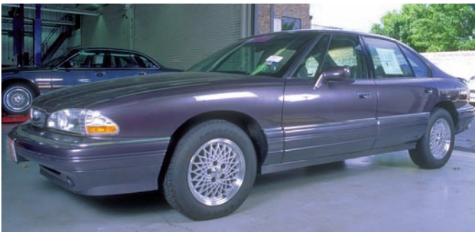
P47-3 Park the car on a level shop floor or alignment rack.
