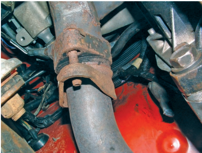
Figure 32-35 Leaking gaskets and seals are often found between the exhaust manifold and pipe.
