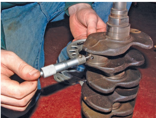
Figure 11-42 Measure the diameters of the crank journals with an outside micrometer.
