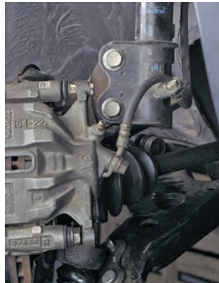
P49-5 Remove the bolt that fastens the brake line or hose to the strut assembly.
