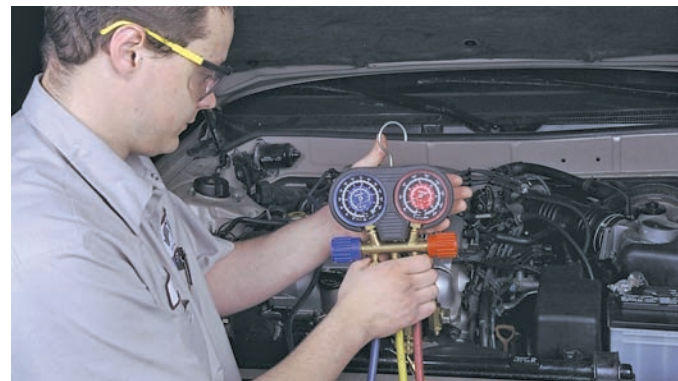
P53-7 After the system has been recharged, check the gauge readings while the system is in operation to make sure it is working properly.
