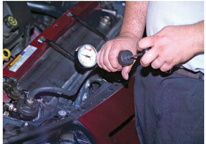
P11-4 Once the pressure is equal to the rating of the pressure cap, watch for a pressure decrease and look for leaks.
