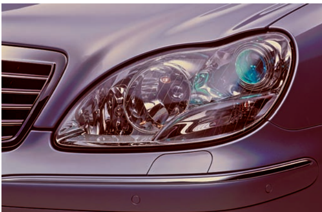
Figure 20-10 HID (xenon) headlamps are readily identifiable by their bluish light. Courtesy of Chrysler LLC
