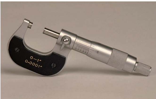
P2-5 A micrometer reading of 0.500 inch.
