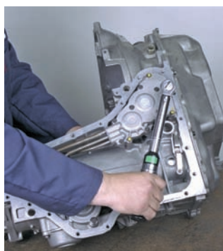
P43-44 Install the accumulator cover with governor feed and return pipes and the accumulator pistons, gaskets, retainers, and pipes into their bores.
