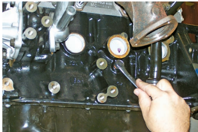
Figure 14-59 Most engines have drain plugs that allow for draining coolant out of the block.
