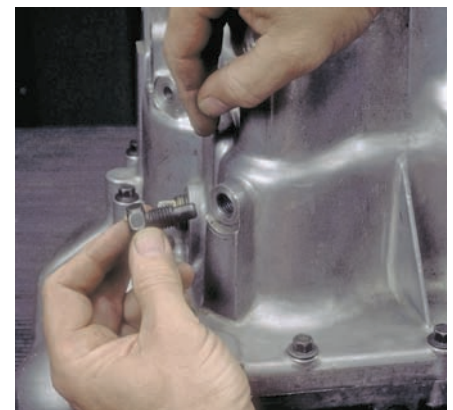
P36-18 Install and tighten the reverse-idler shaft retaining bolt.
