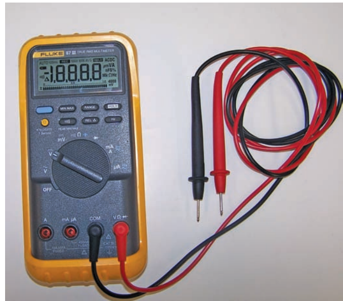
Figure 5-22 Typical multifunctional, low-impedance multimeter.
