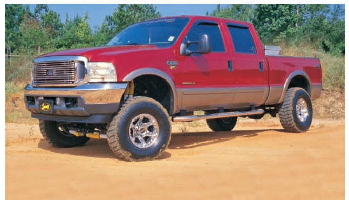
Figure 45-5 To provide more ground clearance, a lift kit that included ten-leaf rear springs was installed on this pickup. Courtesy of Superlift Suspension Systems
