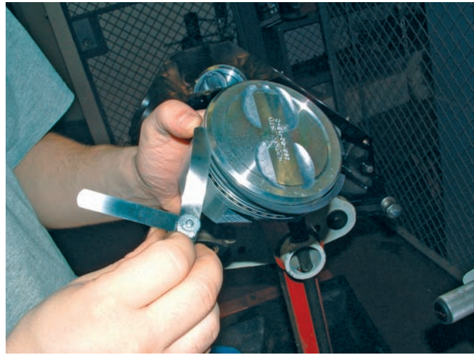
Figure 11-59 Ring side clearance should be checked on each piston.
