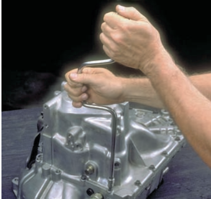
P35-1 Place the transaxle into a suitable work stand. Remove the reverse idler shaft retaining bolt and detent plunger retaining screw. Then loosen and remove all transaxle case-to-clutch housing attaching bolts.
