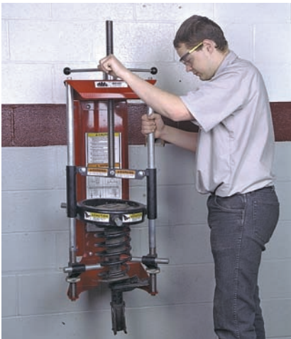
P49-8 Install the strut assembly into the proper type of spring compressor. Then compress the spring until it is possible to safely loosen the retaining bolts.
