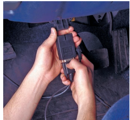
P24-6 Connect the scan tool to the DLC.
