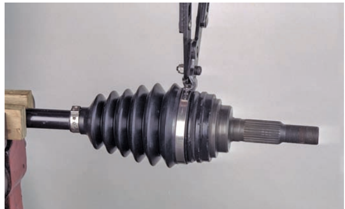
P37-16 Install the new large boot clamp and reinstall the axle into the car. Torque the hub nut after the wheels have been reinstalled and the car is sitting on the ground. Always follow the correct procedure for the clamp being installed.
