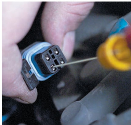
P26-5 Turn off the engine and move the positive meter lead to the sensor's signal wire. Keep the negative lead grounded.
