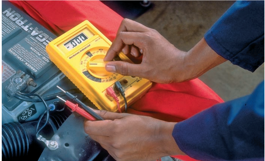
P12-2 Set the voltmeter on its lowest DC volt scale.
