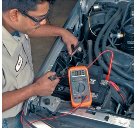
P15-9 There is still too much voltage drop; continue the test by moving the negative lead to the battery side of the relay.
