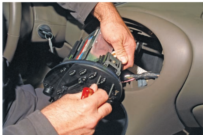
Figure 53-38 The control must be removed to test it and what it controls.
