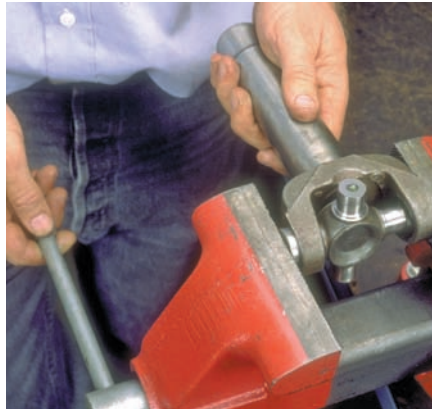
P39-5 Carefully place the assembly in a vise or U-joint bearing press and press the cup partially through the ear.
