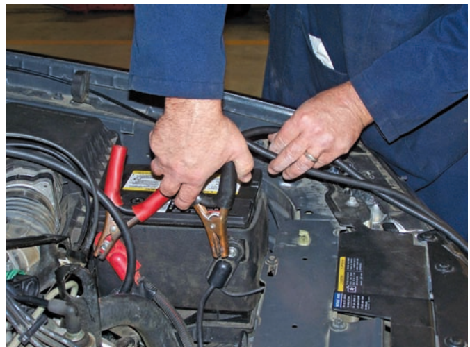
P14-4 Attach the tester's battery leads to the correct terminals on the battery.
