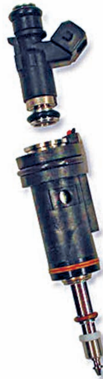
Figure 30-24 An injector for gasoline direct injection. Courtesy of Delphi Corporation
