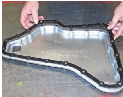
P42-8 Install the new filter and tighten the attaching bolts to specifications. Then lay the new gasket over the sealing surface of the pan.
