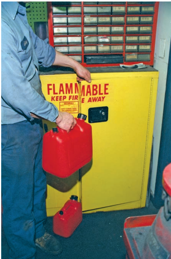
Figure 6-19 Store combustible materials in approved safety cabinets.
