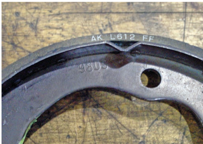
Figure 49-30 Identification codes, called the automotive friction material edge codes, are printed on the edges of drum brake linings.
