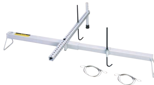
Figure 5-45 An engine support is used to hold the engine in place while the transaxle is removed on many FWD vehicles. Courtesy of SPX Service Solutions
