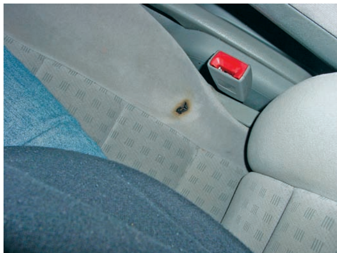
Figure 23-32 This heated seat became very hot because of a shorted heating coil.
