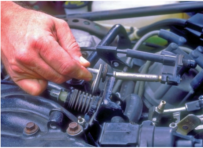
Figure 23-20 Check the linkage if the vehicle surges while cruise is activated.
