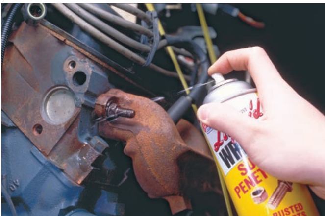
Figure 32-36 Before attempting to disassemble the exhaust system, spray all nuts and bolts with penetrating oil.
