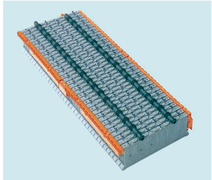
Figure 17-43 A high-voltage battery pack made with prismatic cells. Courtesy of Toyota Motor Sales, U.S.A., Inc.
