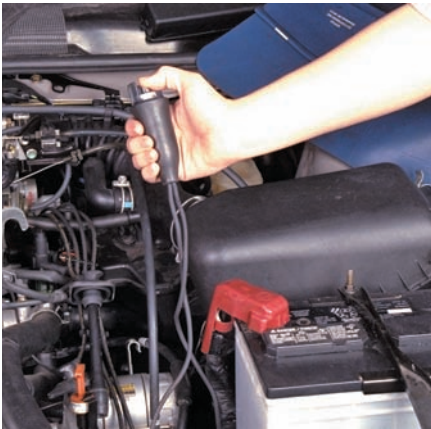
P6-4 Connect a remote starter button to the starter system.
