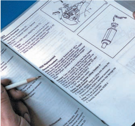
P26-1 Locate the oxygen sensor in a wiring diagram for the vehicle and identify what part of the sensor each wire is connected to.
