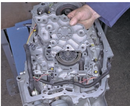
P43-7 Remove the pump assembly cover. Remove the servo pipe retainer bolt, retainer plate, bolts, and valve body.
