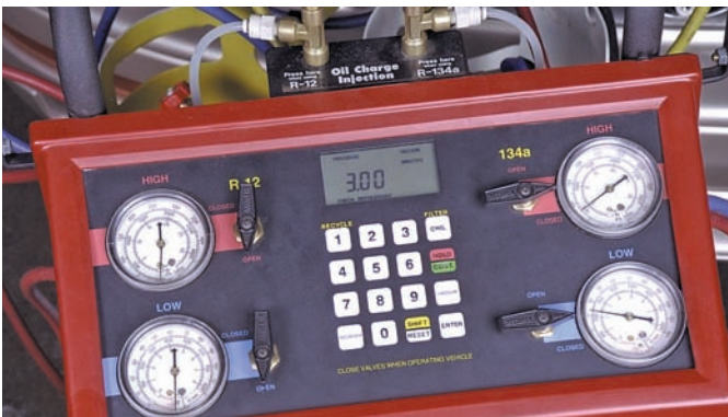
P53-6 Close the valves at the gauge set and disconnect the reclaiming machine. Connect the charging station and open the gauge set valves. Set the unit to deliver the required amount of refrigerant for that system.
