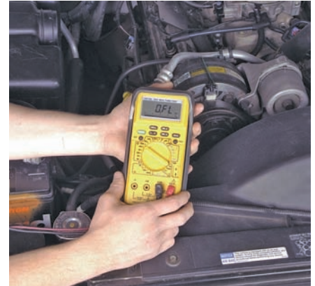
P33-3 Connect the ohmmeter leads to one of the solenoid's terminals and to ground. An infinite reading means the solenoid is not shorted to ground.
