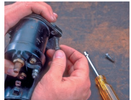
P16-5 Remove the two screws that attach the solenoid to the starter drive housing.
