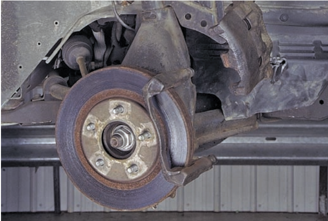
P52-7 Fasten a piece of wire to the car's frame and support the caliper with the wire.
