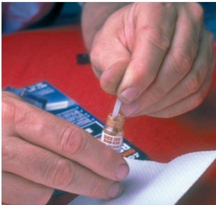
P21-4 Mix the hardener and silver plastic thoroughly. If the hardener has crystallized, immerse the packet in hot water.
