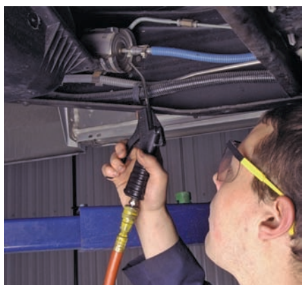
P29-7 Flush the fuel filter line connectors with water, and use compressed air to blow debris off and away from the connectors.
