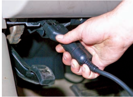
P28-2 Connect the scan tool with the correct adapter to the DLC.
