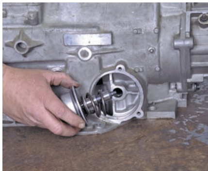
P43-5 Apply pressure to the 1-2 servo cover and remove the cover's retaining ring. Then remove the cover and servo assembly.
