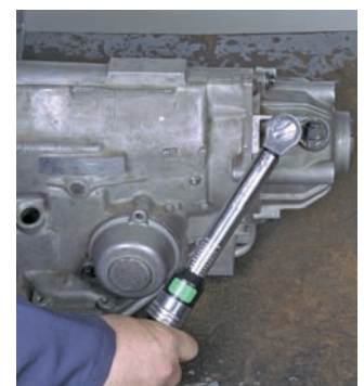
P43-46 Install the torque converter, speedometer sensor, and governor assembly.
