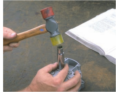
P17-12 Use a socket or a bearing driver to tap out the bearing from the housing.
