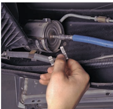
P29-8 Follow the recommended procedures for disconnecting the fuel inlet connector.
