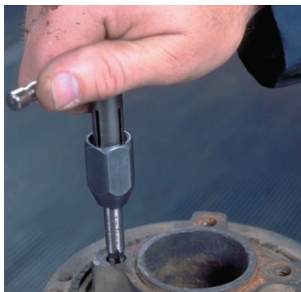
P1-5 Rotate the tap clockwise into the bore until the tap has run through the entire length of the threads. While doing this, periodically turn the tap backward to clean the threads. This prevents breaking the tap.
