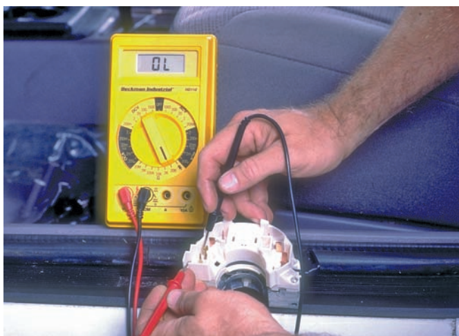
Figure 16-22 On some DMMs, an infinite reading is displayed as “OL.”
