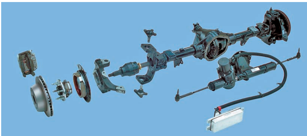
Figure 46-50 An exploded view of the Quadrasteer setup. Courtesy of the Delphi Corporation
