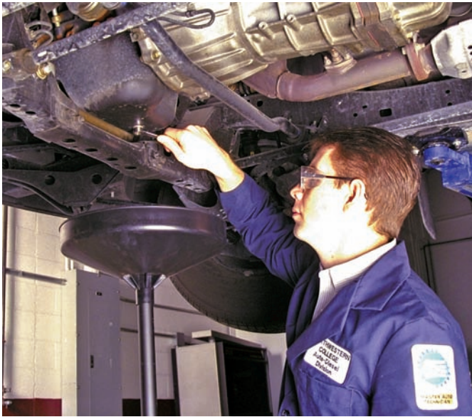
Figure 1-5 Regular preventive maintenance (PM) is important for keeping electronic control systems operating correctly. A common part of PM is changing the engine's oil and filter.
