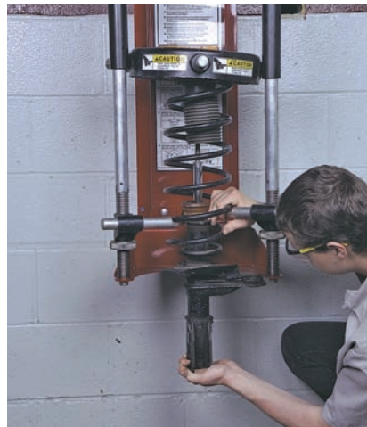
P49-9 Remove the old strut assembly from the spring and install the new strut. Compress the spring to allow for reassembly and tighten the retaining bolts.
