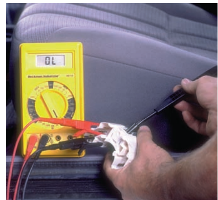
P18-16 When the dimmer switch is placed in the flash-to-pass position, there should be continuity across those designated terminals and an open across the others.
