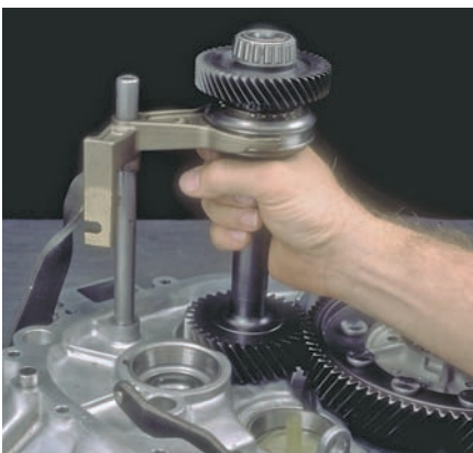
P36-7 Install the fifth-gear shaft assembly and fork shaft into the case.
