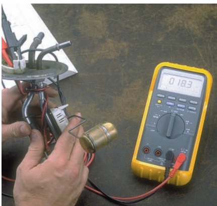
P19-7 Slowly move the float toward the full stop while observing the ohmmeter. The resistance change should be smooth and consistent.
