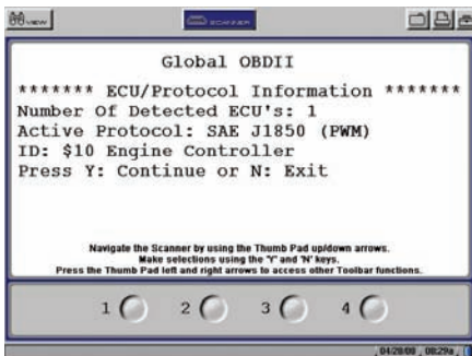
P23-4 The tool will display basic information about the control system.
