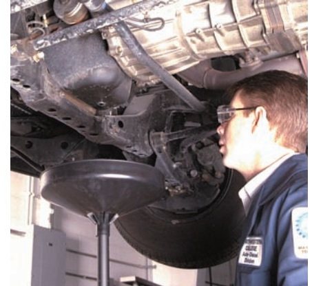
P3-3 Place the oil drain pan under the drain plug before beginning to drain the oil.
