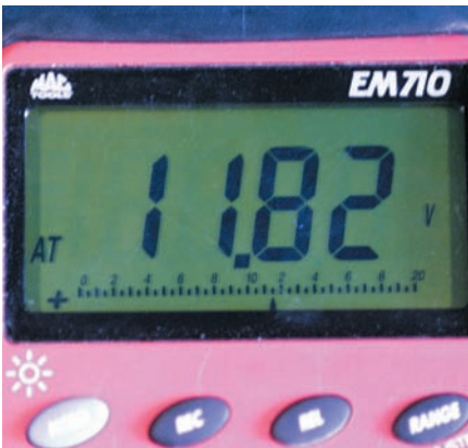
P26-4 Start the engine and observe the voltage reading as the engine initially starts.
