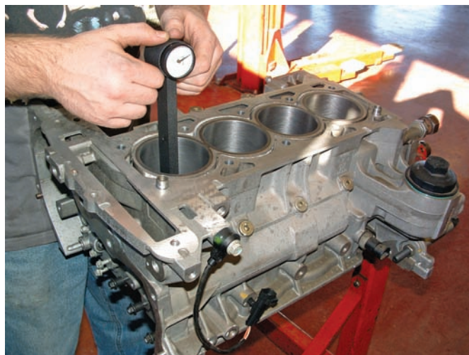
Figure 11-19 Cylinder bore is checked for out-of-roundness with a dial bore gauge.
