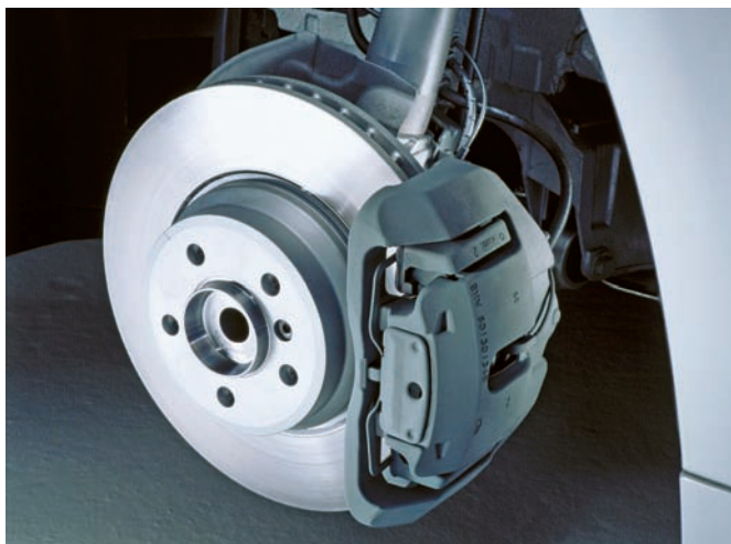
Figure 50-1 A typical disc brake assembly. Courtesy of BMW of North America, LLC
