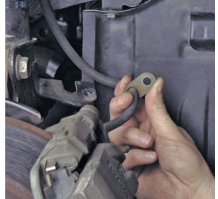
P37-3 The brake line holding clamp must be loosened from the suspension.
