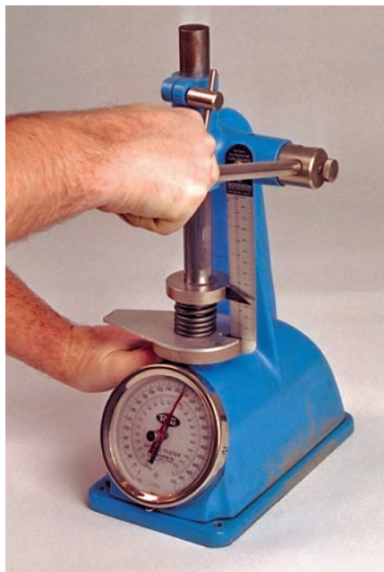
P9-11 Now compress the spring to the open height specification. Use the rule on the gauge or a scale to measure the compressed height.
