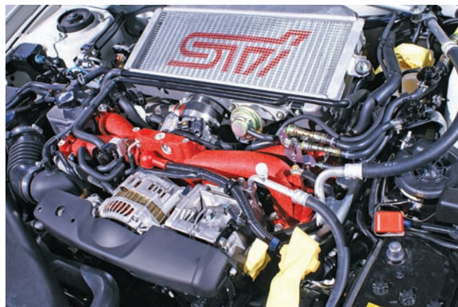
Figure 32-13 The intercooler for this engine is above the engine.
