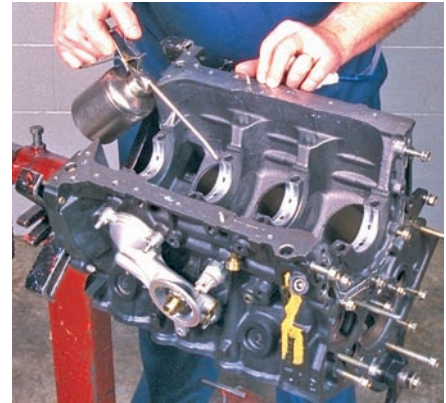
P7-12 If the clearance was within the specifications, remove the crankshaft and apply a good coat of fresh engine oil to the bearings.
