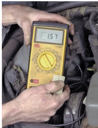
P25-5 Observe the MAP sensor barometric pressure voltage reading on the voltmeter. Compare this reading to the specifications.
