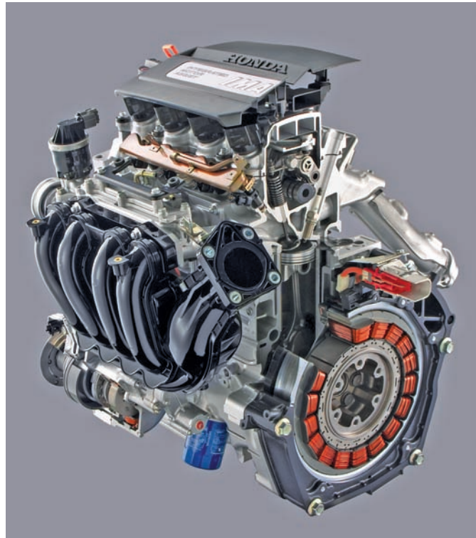
Figure 9-29 The Honda Civic Hybrid has a 1.3-liter gasoline engine and a 20-horsepower electric motor. Courtesy of American Honda Motor Co., Inc.
