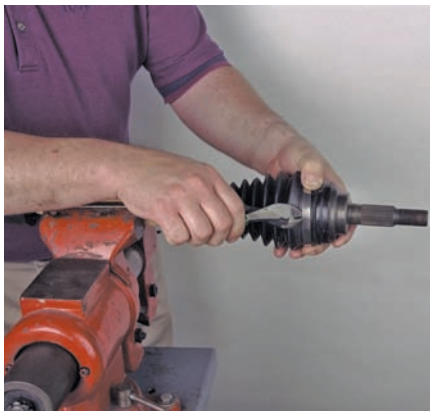
P37-8 Begin boot removal by cutting and discarding the boot clamps.
