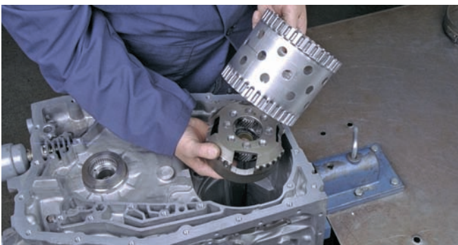
P43-16 Measure the end play of the input shaft clutch housing. Select the correct thickness of thrust washer and set it aside for reassembly. Remove the input clutch sprag assembly, the third clutch assembly, and the input sun gear. Then remove the reverse band, reverse reaction drum input carrier assembly and thrust washer.
