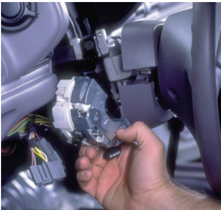
P18-11 Disengage the switch from the lock assembly.
