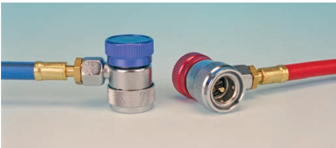
Figure 53-14 The test connectors with shutoff valves for an R-134a system.
