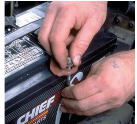
P5-15 Install the battery back into the tray. Also install the hold-down hardware.
