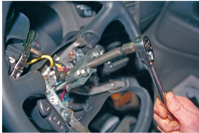
Figure 46-43 Use the correct puller to remove the steering wheel assembly.
