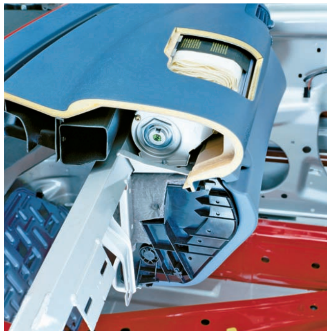
Figure 24-25 A cutaway view showing the complete passenger-side air bag module in the dash. Courtesy of Chrysler LLC
