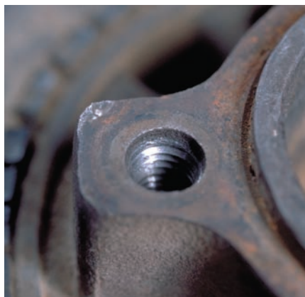
P1-8 Inspect the threads left by the tap to be sure they are acceptable.
