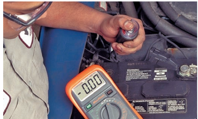
P15-5 Disable the ignition and fuel injection and/or connect a remote starter switch.
