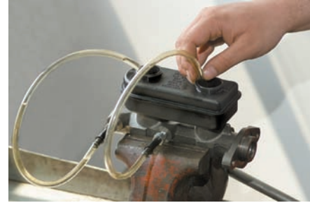
P51-3 Bend the tubing lines so that the ends are in each chamber of the master cylinder reservoir.
