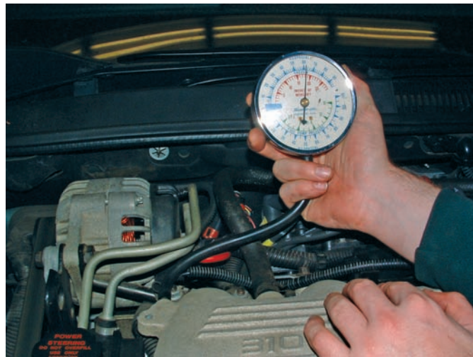
Figure 5-35 A vacuum/pressure tester used to measure engine vacuum.
