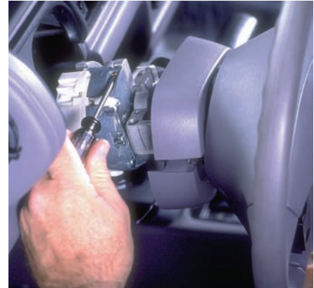
P18-10 Remove the screws that attach the switch to the lock cylinder assembly.
