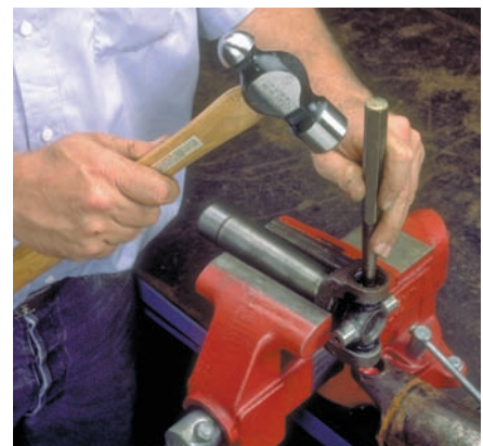
P38-9 Use a drift and hammer to drive the joint out of the other yokes.
