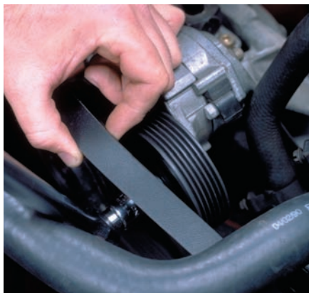
P4-6 Pry the tensioner or generator pulley inward to release the belt tension and remove the belt.
