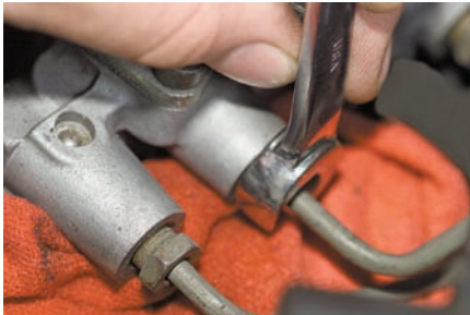
P51-10 Slowly depress the pedal several times to force out any air that might be trapped in the connections each time the pedal is depressed. Before releasing the pedal, tighten the nut slightly and loosen it before depressing the pedal each time. Soak up the fluid with a rag to avoid damaging the car finish.
