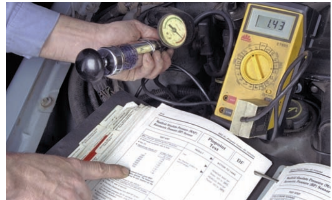
P25-6 Connect a hand-operated vacuum pump to the MAP sensor and apply 5 in. Hg to the sensor. Observe the sensor's voltage signal on the voltmeter. Compare the reading to specifications.
