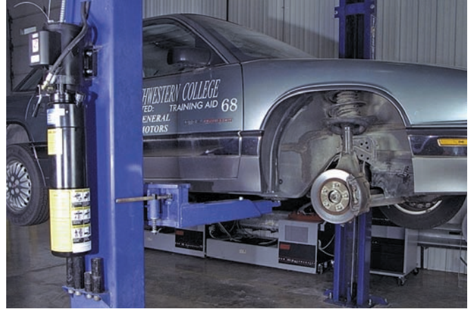
P52-2 Raise the car. Make sure it is safely positioned on the lift. Remove its wheel assemblies.
