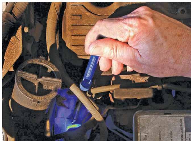
Figure 14-47 A common way to identify the source of an external leak is to use dye penetrant and a black light. Where the dyed coolant leaks, a bright or fluorescent green color will be seen. Courtesy of Tracer Products
