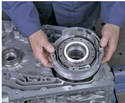
P43-14 Remove the driven sprocket support and thrust washer from between the sprockets and the channel plate. Remove the scavenging scoop and driven sprocket with the second clutch's thrust washer.
