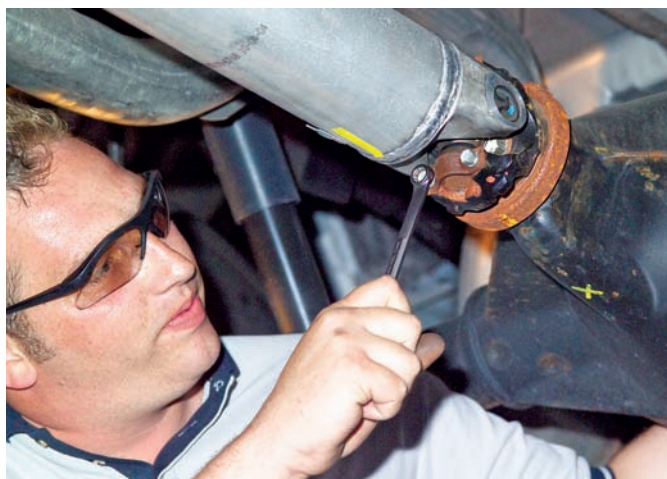
Figure 10-16 Mark the alignment of the rear U-joint and the pinion flange before removing the drive shaft.
