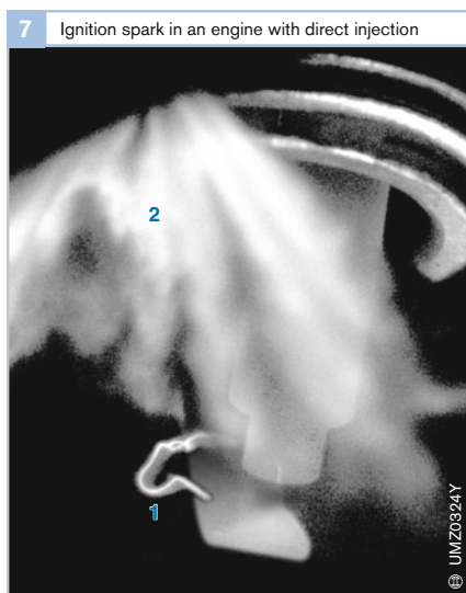
Fig. 7 Photograph of an ignition spark: taken in a transparent engine using a high-speed camera
