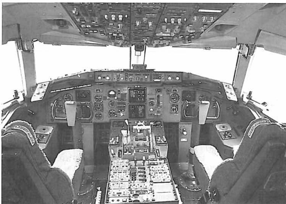
FIGURE 13.3 The flight deck of the Boeing 757 and 767 features digital control electronics, including an engine indicating system and a crew alerting system. All systems controls are within reach of either pilot. The system includes an inertial reference system making use of laser gyroscopes and an electronic attitude director indicator. A flight-management computer system integrates navigation, guidance, and performance data functions. When coupled with the automatic flight control system, the flight-management system provides accurate engine thrust settings and flight-path guidance during all phases of flight from immediately after takeoff to final approach and landing. (Courtesy of Boeing Airplane Co.)
