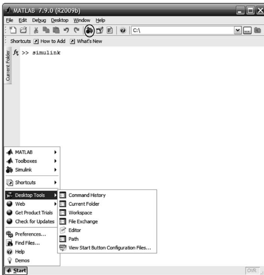
FIGURE C.1 MATLAB Window showing how to access Simulink. The Simulink Library Browser button is shown circled.
