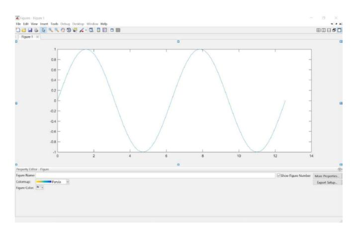
Click on one of the axes to get the following screen, you can give the plot a title, label the axes, change the limits of the axes, change the fonts ...
