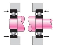
positioning or axially locating the shaft. Figure 11–20 shows a very common solution to this problem. The inner rings are backed up against the shaft shoulders and are held in position by round nuts threaded onto the shaft. The outer ring of the left-hand bearing is backed up against a housing shoulder and is held in position by a device that is not shown. The outer ring of the right-hand bearing floats in the housing.
