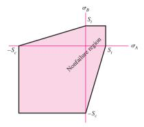
Since for the Coulomb-Mohr theory we do not need the torsional shear strength circle we can deduce it from Eq. (5–22). For pure shear  $\tau$ ,  $\sigma_1 = -\sigma_3 = \tau$ . The torsional yield strength occurs when  $\tau_{\text{max}} = S_{sy}$ . Substituting  $\sigma_1 = -\sigma_3 = S_{sy}$  into Eq. (5–22) and simplifying gives
