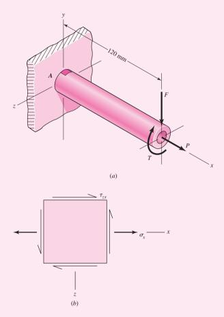
For accuracy, we choose the distortion-energy theory as the design basis. The von Mises stress from Eq. (5–15), is
