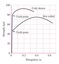
strength and hardness, and a decrease in ductility. In Fig. 2–12 the properties of a cold-drawn bar are compared with those of a hot-rolled bar of the same material.
