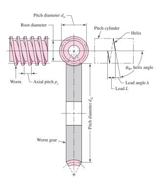
Since it is not related to the number of teeth, the worm may have any pitch diameter; this diameter should, however, be the same as the pitch diameter of the hob used to cut the worm-gear teeth. Generally, the pitch diameter of the worm should be selected so as to fall into the range
