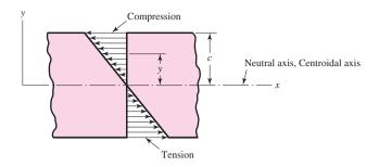
neutral axes of all cross sections, is called the *neutral plane*. Elements of the beam coincident with this plane have zero stress. The location of the neutral axis with respect to the cross section is coincident with the *centroidal axis* of the cross section.
