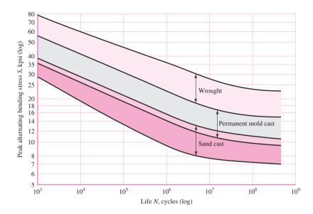
Soon we shall learn that *S-N* diagrams can be determined either for a test specimen or for an actual mechanical element. Even when the material of the test specimen and that of the mechanical element are identical, there will be significant differences between the diagrams for the two.
