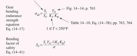
Remember to compare  $S_F$  with  $S_H^2$  when deciding whether bending or wear is the threat to function. For crowned gears compare  $S_F$  with  $S_H^3$ .
