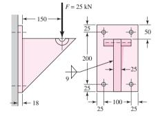
**9–48** The figure shows a welded steel bracket loaded by a static force *F*. Estimate the factor of safety if the allowable shear stress in the weld throat is 18 kpsi.
