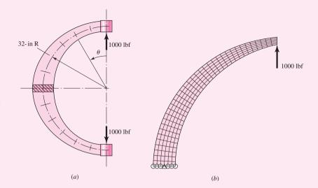
an amplitude of 2 in. The load is 1000 lbf. It follows that C = 1.2,  $G = 11.5(10^6)$  psi,  $E = 30(10^6)$  psi. The outer and inner radii are
