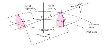
Thus, for a short period of time, there will be two teeth in contact, one in the vicinity of A and another near B. As the meshing proceeds, the pair near B must cease contact, leaving only a single pair of contacting teeth, until the procedure repeats itself.
