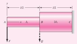
Since F is at A and in the direction of the desired deflection, the deflection at A from Eq. (4-31) is
