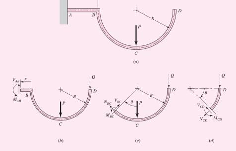
For section BC, with the variable of integration  $\theta$  defined as shown in Fig. 4–13c, summing moments about the break gives the moment equation for section BC.
