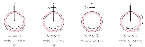
How the significant speed varies. (a) Common bearing case. (b) Load vector moves at the same speed as the journal. (c) Load vector moves at half journal speed, no load can be carried. (d) Journal and bushing move at same speed, load vector stationary, capacity halved.
