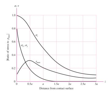
These equations are valid for either sphere, but the value used for Poisson's ratio must correspond with the sphere under consideration. The equations are even more complicated when stress states off the z axis are to be determined, because here the x and y coordinates must also be included. But these are not required for design purposes, because the maxima occur on the z axis.
