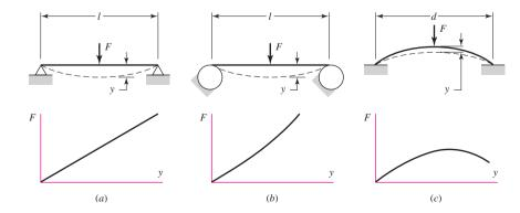
as shown by the graph. Any mechanical element having such a characteristic is called a *nonlinear softening spring*.
