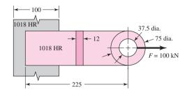
**9–35** The attachment shown carries a static bending load of 12 kN. The attachment length,  $l_1$ , is 225 mm. Specify the weldment (give the pattern, electrode number, type of weld, length of weld, and leg size).
