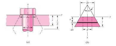
The pressure, however, falls off farther away from the bolt. Thus Ito suggests the use of Rotscher's pressure-cone method for stiffness calculations with a variable cone angle. This method is quite complicated, and so here we choose to use a simpler approach using a fixed cone angle.
