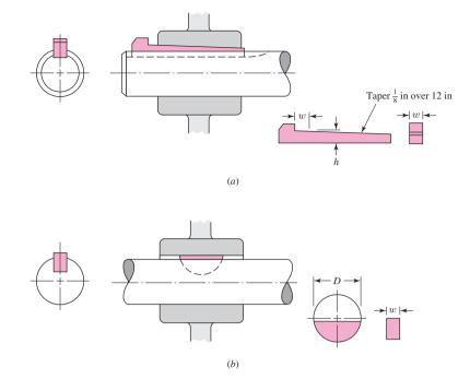
The gib-head key, in Fig. 7–17*a*, is tapered so that, when firmly driven, it acts to prevent relative axial motion. This also gives the advantage that the hub position can be adjusted for the best axial location. The head makes removal possible without access to the other end, but the projection may be hazardous.
