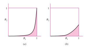
Curve shapes of the  $R_1R_2$  plot. In each case the shaded area is equal to 1 - R and is obtained by numerical integration. (a) Typical curve for asymptotic distributions; (b) curve shape obtained from lower truncated distributions such as the Weibull.
