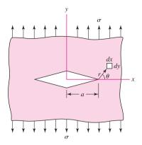
Consider a mode I crack of length 2a in the infinite plate of Fig. 5–24. By using complex stress functions, it has been shown that the stress field on a dx dy element in the vicinity of the crack tip is given by
