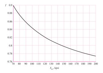
The process given for finding f can be repeated for various ultimate strengths. Figure 6–18 is a plot of f for  $70 \le S_{ut} \le 200$  kpsi. To be conservative, for  $S_{ut} < 70$  kpsi, let f = 0.9.
