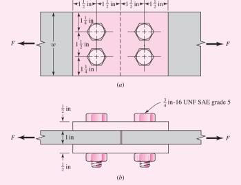
F/2 is transmitted by each of the splice plates, but since the areas of the splice plates are half those of the center bars, the stresses associated with the plates are the same. So for stresses associated with the plates, the force and areas used will be those of the center plates.
