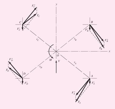
The primary shear load per bolt is
