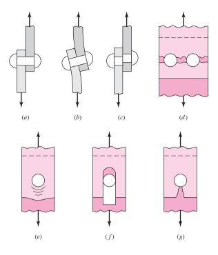
Rupture of one of the connected members or plates by pure tension is illustrated in Fig. 8–23*d*. The tensile stress is
