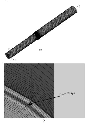
Resorting to another source,<sup>13</sup> the stress-concentration factor is found to be  $K_t = 3.00$ . The reaction at the right support is  $R_F = (8/20)600 = 240$  lbf. The bending moment at the start of the fillet is M = 240(11.52) = 2765 lbf · in = 2.765 kip · in. The analytical prediction of the maximum stress is thus
