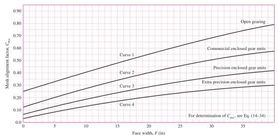
Figure 14–11 Mesh alignment factor  $C_{ma}$ . Curve-fit equations in Table 14–9. (ANSI/AGMA 2001-D04.)
