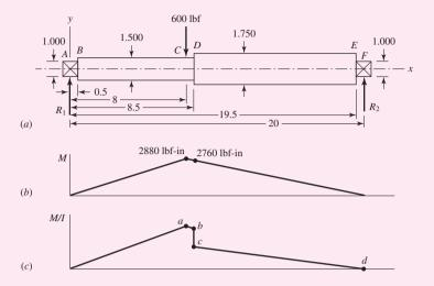
A plot of M/I is shown in Fig. 4–7c. The values at points b and c, and the step change are
