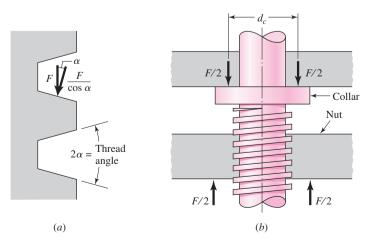
The axial stress  $\sigma$  in the body of the screw due to load F is
