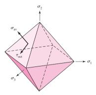
equal to the hydrostatic stress  $\sigma_{av}$ . There are eight surfaces symmetric to the principal directions that contain this stress. This forms an octahedron as shown in Fig. 5–10. The shear stresses on these surfaces are equal and are called the *octahedral shear stresses* (Fig. 5–10 has only one of the octahedral surfaces labeled). Through coordinate transformations the octahedral shear stress is given by<sup>5</sup>
