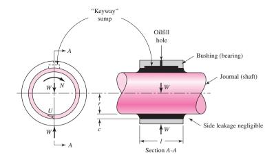
the radial clearance by c, and the length of the bearing by l, all dimensions being in inches. If the shaft rotates at N rev/s, then its surface velocity is  $U = 2\pi r N$  in/s. Since the shearing stress in the lubricant is equal to the velocity gradient times the viscosity, from Eq. (12–2) we have
