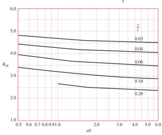
Approximate Stress-Concentration Factor  $K_t$  for Bending of a Round Bar or Tube with a Transverse Round Hole
