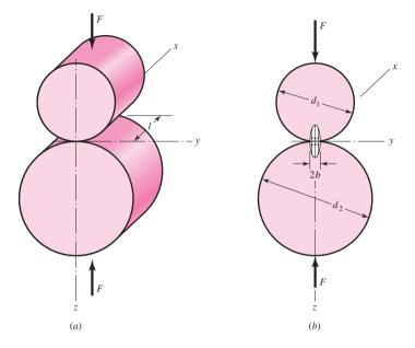
Equations (3–73) and (3–74) apply to a cylinder and a plane surface, such as a rail, by making  $d = \infty$  for the plane surface. The equations also apply to the contact of a cylinder and an internal cylindrical surface; in this case d is made negative for the internal surface.
