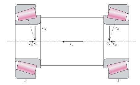
bearing and 0.75 for a steep angle bearing in the preliminary selection process. After a possible bearing is identified, the exact value of K for each bearing can be found in the bearing catalog.
