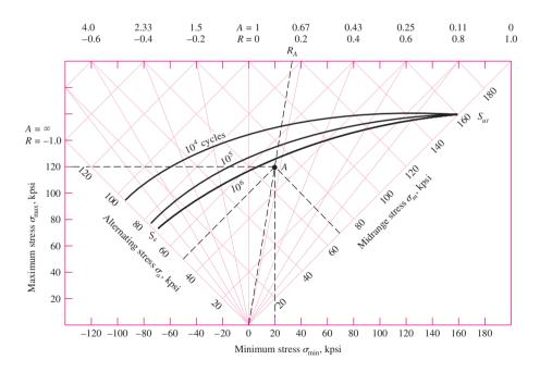
have been drawn too. Any stress state, such as the one at A, can be described by the minimum and maximum components, or by the midrange and alternating components. And safety is indicated whenever the point described by the stress components lies below the constant-life line.
