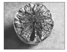
Impact failure of a lawn-mower blade driver hub. The blade impacted a surveying pipe marker.
