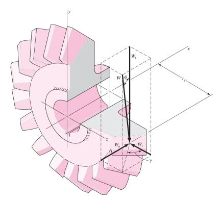
The three forces  $W_t$ ,  $W_r$ , and  $W_a$  are at right angles to each other and can be used to determine the bearing loads by using the methods of statics.
