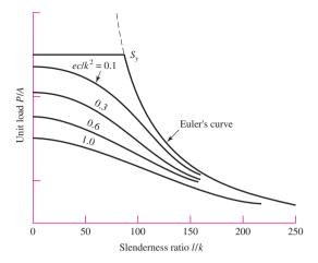
yield strength of 40 kpsi. Note how the P/A contours asymptotically approach the Euler curve as l/k increases.
