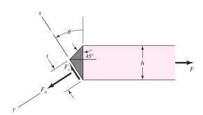
The average stress in a butt weld due to shear loading (Fig. 9–7b) is
