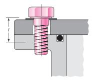
A section through a tension-loaded bolted joint is illustrated in Fig. 8–13. Notice the clearance space provided by the bolt holes. Notice, too, how the bolt threads extend into the body of the connection.
