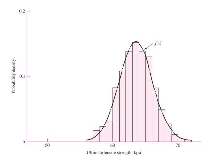
mean, standard deviation, and distribution type. Many tables display a single number, which is often the mean, minimum, or some percentile, such as the 99th percentile. Always read the foonotes to the table. If no qualification is made in a single-entry table, the table is subject to serious doubt.
