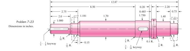
steel. At steady-state speed, the gear transmits a radial load of 230 lbf and a tangential load of 633 lbf at a pitch diameter of 8 in.
