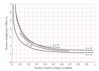
in fatigue or in wear. However, the graph does show that the rope will have a long life if the ratio  $p/S_u$  is less than 0.001. Substitution of this ratio in Eq. (17–42) gives
