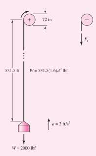
From Fig. 17–21, use  $p/S_u = 0.0014$ . Fatigue tension  $F_f$  from Eq. (17–47) is given by
