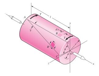
The last assumption depends upon the axisymmetry of the member, so it does not hold true for noncircular cross sections. Consequently, Eqs. (3–35) through (3–37) apply *only* to circular sections. For a solid round section,
