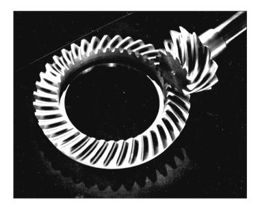
It is frequently desirable, as in the case of automotive differential applications, to have gearing similar to bevel gears but with the shafts offset. Such gears are called *hypoid gears*, because their pitch surfaces are hyperboloids of revolution. The tooth action between such gears is a combination of rolling and sliding along a straight line and has much in common with that of worm gears. Figure 15–3 shows a pair of hypoid gears in mesh.
