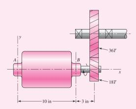
Free-body diagram of motor shaft of Ex. 13–9.
