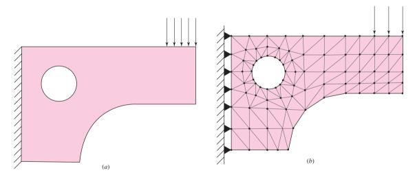
**Figure 19–2**Structural problem. (*a*) Idealized model; (*b*) finite-element model.
