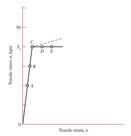
For materials that strain-strengthen, the critical location in the notch has a higher  $S_y$ . The shank area is at a stress level a little below 40 kpsi, is carrying load, and is very near its failure-by-general-yielding condition. This is the reason designers do not apply  $K_t$  in *static loading* of a *ductile material* loaded elastically, instead setting  $K_t = 1$ .
