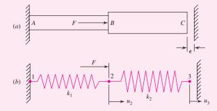
reactions, the internal forces in the members, and the deflection of point B. Let E=10 Mpsi and assume that end C hits the wall. Check the validity of the assumption.
