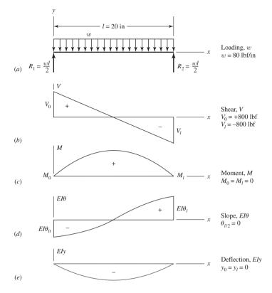
The nomenclature and conventions are illustrated by the beam of Fig. 4–2. Here, a beam of length l=20 in is loaded by the uniform load w=80 lbf per inch of beam length. The x axis is positive to the right, and the y axis positive upward. All quantities—loading, shear, moment, slope, and deflection—have the same sense as y; they are positive if upward, negative if downward.
