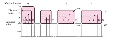
dimensions directly, it is necessary to resort to tabulations. The 02 series is used here as an example of what is available. See Table 11–2.
