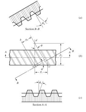
Figure 13–22 represents a portion of the top view of a helical rack. Lines ab and cd are the centerlines of two adjacent helical teeth taken on the same pitch plane. The angle  $\psi$  is the *helix angle*. The distance ac is the *transverse circular pitch*  $p_t$  in the plane of rotation (usually called the *circular pitch*). The distance ae is the *normal circular pitch*  $p_n$  and is related to the transverse circular pitch as follows:
