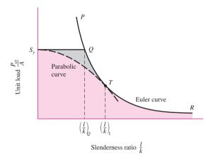
compression member. Thus it would appear that any compression member having an l/k value less than  $(l/k)_Q$  should be treated as a pure compression member while all others are to be treated as Euler columns. Unfortunately, this is not true.
