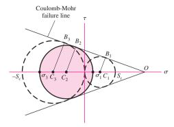
where  $B_1C_1 = S_t/2$ ,  $B_2C_2 = (\sigma_1 - \sigma_3)/2$ , and  $B_3C_3 = S_c/2$ , are the radii of the right, center, and left circles, respectively. The distance from the origin to  $C_1$  is  $S_t/2$ , to  $C_3$  is  $S_c/2$ , and to  $C_2$  (in the *positive*  $\sigma$  direction) is  $(\sigma_1 + \sigma_3)/2$ . Thus
