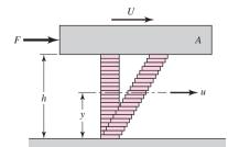
where  $\mu$  is the constant of proportionality and defines *absolute viscosity*, also called *dynamic viscosity*. The derivative du/dy is the rate of change of velocity with distance and may be called the rate of shear, or the velocity gradient. The viscosity  $\mu$  is thus a measure of the internal frictional resistance of the fluid. For most lubricating fluids, the rate of shear is constant, and du/dy = U/h. Thus, from Eq. (12–1),
