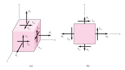
Note that double subscripts are necessary for the shear. The first subscript indicates the direction of the surface normal whereas the second subscript is the direction of the shear stress.
