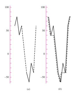
hidden cycle is applied but once. If the all-positive stress cycle is applied alternately with the all-negative stress cycle, the hidden cycle is applied 100 times.
