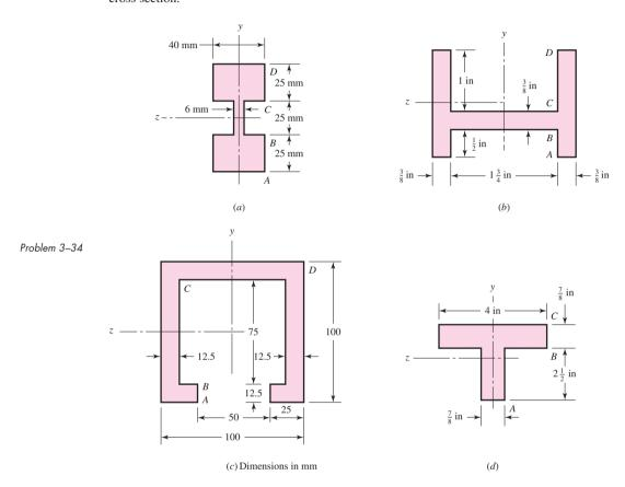
**3–35 to** For the beam illustrated in the figure, find the locations and magnitudes of the maximum tensile bending stress due to *M* and the maximum shear stress due to *V*.
