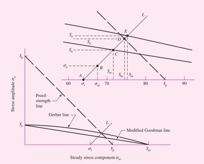
of the load line L with the respective failure lines at points C, D, and E defines a set of strengths  $S_a$  and  $S_m$  at each intersection. Point B represents the stress state  $\sigma_a$ ,  $\sigma_m$ . Point A is the preload stress  $\sigma_i$ . Therefore the load line begins at A and makes an angle having a unit slope. This angle is  $45^{\circ}$  only when both stress axes have the same scale.
