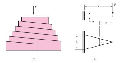
which is proportional to the distance x if I/c is a constant. But there is no reason why I/c need be a constant. For example, one might design such a spring as that shown in Fig. 10–13b, in which the thickness h is constant but the width b is permitted to vary. Since, for a rectangular section,  $I/c = bh^2/6$ , we have, from Eq. (a),
