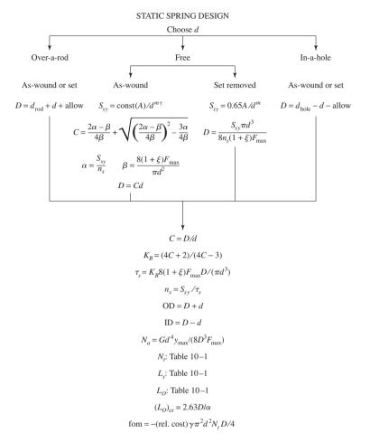
Print or display: d, D, C, OD, ID,  $N_a$ ,  $N_r$ ,  $L_s$ ,  $L_O$ ,  $(L_O)_{\rm cr}$ ,  $n_s$ , fom Build a table, conduct design assessment by inspection Eliminate infeasible designs by showing active constraints Choose among satisfactory designs using the figure of merit  $^{\dagger}$  const is found from Table 10–6.
