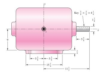
Problem 13–35 NEMA No. 364 frame; dimensions in inches. The z axis is directed out of the paper.
