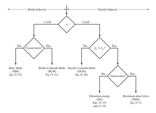
namely, Coulomb Mohr, or modified Mohr. Figure 5–21 provides a summary flowchart for the selection of an effective procedure for analyzing or predicting failures from static loading for brittle or ductile behavior. Note that the maximum-normal-stress theory is excluded from Fig. 5–21 as the other theories better represent the experimental data.
