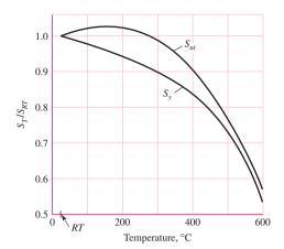
only a small amount until a certain temperature is reached. At that point it falls off rapidly. The yield strength, however, decreases continuously as the environmental temperature is increased. There is a substantial increase in ductility, as might be expected, at the higher temperatures.
