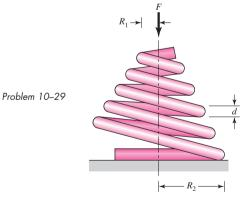
A helical coil compression spring is needed for food service machinery. The load varies from a minimum of 4 lbf to a maximum of 18 lbf. The spring rate k is to be 9.5 lbf/in. The outside diameter of the spring cannot exceed  $2\frac{1}{2}$  in. The springmaker has available suitable dies for drawing 0.080-, 0.0915-, 0.1055-, and 0.1205-in-diameter wire. Using a fatigue design factor  $n_f$  of 1.5, and the Gerber-Zimmerli fatigue-failure criterion, design a suitable spring.
