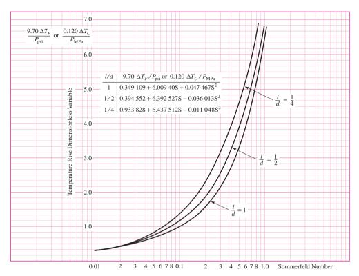
Figures 12–18, 12–19, and 12–20 combined to reduce iterative table look-up. (Source: Chart based on work of Raimondi and Boyd boundary condition (2), i.e., no negative lubricant pressure developed. Chart is for full journal bearing using single lubricant pass, side flow emerges with temperature rise  $\Delta T/2$ , thru flow emerges with temperature rise  $\Delta T$ , and entire flow is supplied at datum sump temperature.)
