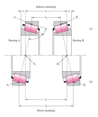
load will induce a thrust reaction within the bearing because of the taper. To avoid the separation of the races and the rollers, this thrust must be resisted by an equal and opposite force. One way of generating this force is to always use at least two tapered roller bearings on a shaft. Two bearings can be mounted with the cone backs facing each other, in a configuration called *direct mounting*, or with the cone fronts facing each other, in what is called *indirect mounting*.
