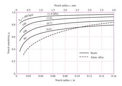
Notch-sensitivity curves for materials in reversed torsion. For larger notch radii, use the values of  $q_{\rm shear}$  corresponding to r=0.16 in (4 mm).
