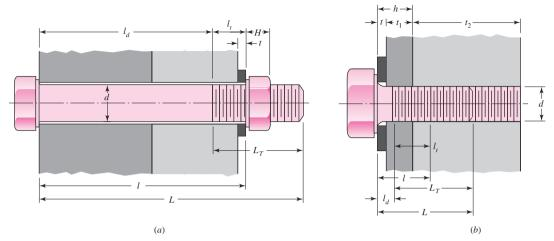
Given fastener diameter d and pitch p in mm or number of threads per inch
