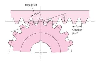
Internal gear and pinion.
