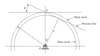
Next, on each gear draw a circle tangent to the pressure line. These circles are the *base circles*. Since they are tangent to the pressure line, the pressure angle determines their size. As shown in Fig. 13–10, the radius of the base circle is
