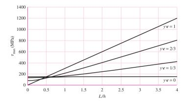
surface where the transverse shear is zero, or if L/h is small enough, it is on the neutral axis where the bending stress is zero.
