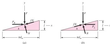
In Fig. 8–5 a square-threaded power screw with single thread having a mean diameter  $d_m$ , a pitch p, a lead angle  $\lambda$ , and a helix angle  $\psi$  is loaded by the axial compressive force F. We wish to find an expression for the torque required to raise this load, and another expression for the torque required to lower the load.
