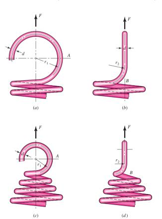
Note: Radius  $r_1$  is in the plane of the end coil for curved beam bending stress. Radius  $r_2$  is at a right angle to the end coil for torsional shear stress.
