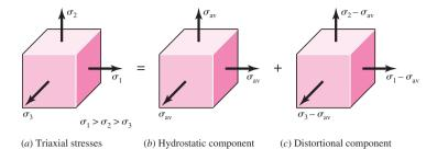
(a) Element with triaxial stresses; this element undergoes both volume change and angular distortion. (b) Element under hydrostatic normal stresses undergoes only volume change. (c) Element has angular distortion without volume change.
