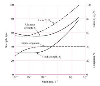
the strengths increase, as shown in Fig. 2–8. In fact, at very high strain rates the yield strength seems to approach the ultimate strength as a limit. But note that the curves show little change in the elongation. This means that the ductility remains about the same. Also, in view of the sharp increase in yield strength, a mild steel could be expected to behave elastically throughout practically its entire strength range under impact conditions.
