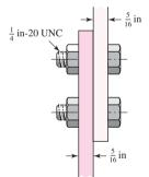
**8–71** A beam is made up by bolting together two cold-drawn bars of AISI 1018 steel as a lap joint, as shown in the figure. The bolts used are ISO 5.8. Ignoring any twisting, determine the factor of safety of the connection.
