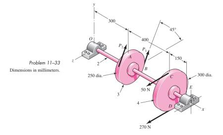
11–34 A gear-reduction unit uses the countershaft depicted in the figure. Find the two bearing reactions. The bearings are to be angular-contact ball bearings, having a desired life of 50 kh when used at 300 rev/min. Use 1.2 for the application factor and a reliability goal for the bearing pair of 0.96. Select the bearings from Table 11–2.
