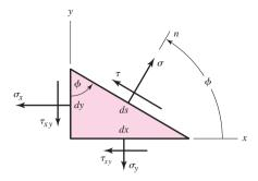
Differentiating Eq. (3–8) with respect to  $\phi$  and setting the result equal to zero maximizes  $\sigma$  and gives
