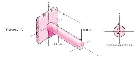
significance of the transverse shear stress in combination with bending by performing the following steps.
