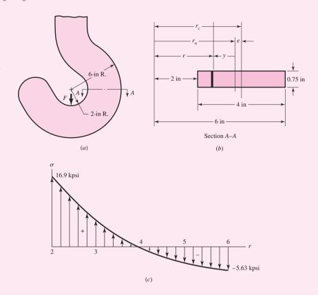
Note in the hook example, the symmetrical rectangular cross section causes the maximum tensile stress to be 3 times greater than the maximum compressive stress. If we wanted to design the hook to use material more effectively we would use more material at the inner radius and less material at the outer radius. For this reason, trapezoidal, T, or unsymmetric I, cross sections are commonly used. Sections most frequently encountered in the stress analysis of curved beams are shown in Table 3–4.
