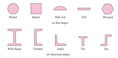
Hot rolling is usually used to create a bar of material of a particular shape and dimension. Figure 2–11 shows some of the various shapes that are commonly produced by the hot-rolling process. All of them are available in many different sizes as well as in different materials. The materials most available in the hot-rolled bar sizes are steel, aluminum, magnesium, and copper alloys.
