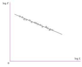
In selecting a bearing for a given application, it is necessary to relate the desired load and life requirements to the published catalog load rating corresponding to the catalog rating life. From Eq. (11–1) we can write
