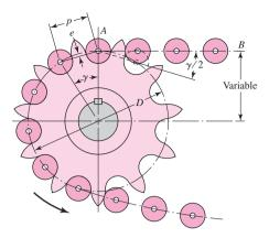
rollers and the sprocket teeth and also wear in the chain joint. Since the life of a properly selected drive is a function of the wear and the surface fatigue strength of the rollers, it is important to reduce the angle of articulation as much as possible.
