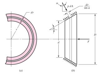
cone angle is too small, say, less than about  $8^{\circ}$ , then the force required to disengage the clutch may be quite large. And the wedging effect lessens rapidly when larger cone angles are used. Depending upon the characteristics of the friction materials, a good compromise can usually be found using cone angles between 10 and  $15^{\circ}$ .
