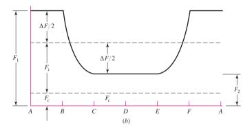
Figure 17–12 illustrates the variation of flexible flat-belt tensions at some cardinal points during a belt pass.
