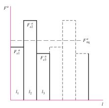
a load level of  $F_1$  is selected and run to the failure criterion, then the area under the  $F_1$ - $L_1$  trace is numerically equal to K. The same is true for a load level  $F_2$ ; that is, the area under the  $F_2$ - $L_2$  trace is numerically equal to K. The linear damage theory says that in the case of load level  $F_1$ , the area from L=0 to  $L=L_A$  does damage measured by  $F_1^aL_A=D$ .
