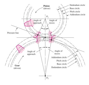
To draw a tooth, we must know the tooth thickness. From Eq. (13–4), the circular pitch is
