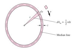
where  $L_m$  is the *length of the section median line*. These equations presume the buckling of the tube is prevented by ribs, stiffeners, bulkheads, and so on, and that the stresses are below the proportional limit.
