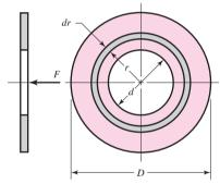
single-plate disk clutch; a multiple-disk clutch-brake is shown in Fig. 16–15. Let us now determine the capacity of such a clutch or brake in terms of the material and geometry.
