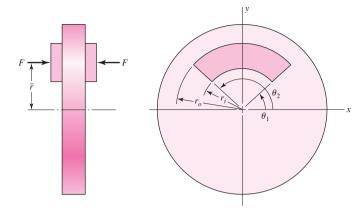
of a rotating disk. Depicted in Fig. 16–19 is the geometry of an annular-pad brake contact area. The governing axial wear equation is Eq. (12–27), p. 663,
