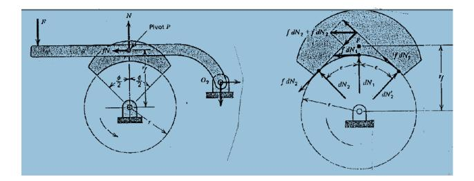
Integrating over the symmetrical shoe surface, the intersection point of the normal and friction forces  $r_f$ :
