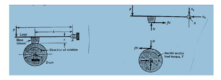
Taking moment about pivot A for the shoe and lever:  $\sum M_{A} = 0 \qquad \Rightarrow \qquad Fc + fNa - bN = 0 \qquad (1)$ Taking moment about O of the drum:  $\sum M_{o} = 0 \qquad \Rightarrow \qquad T = fNr \qquad (2)$ Solving (1) for N and substituting in (2):  $\Rightarrow \qquad N = \frac{Fc}{(b - fa)}$
