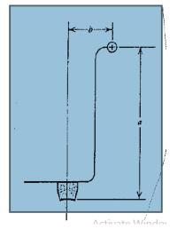
To determine the pressure *p* of lining on the drum caused by applying the force *F* on the left shoe which is deformed (as shown by dashed line)  $\delta =$ Radial deflection
