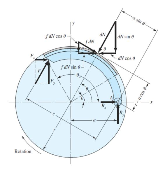
It is required to find the friction torque and the reactions at the hinge of the shoe.
