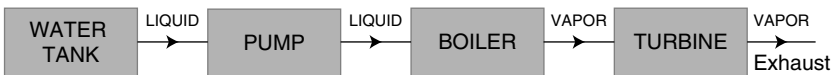
Figure 3.5 In the open-cycle Rankine, exhaust vapor is released directly into the environment. A large water tank is required.
