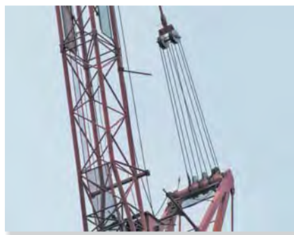
The cable is wrapped around the pulleys on this crane in order to reduce the required force needed to hoist a load. (© R.C. Hibbeler)
