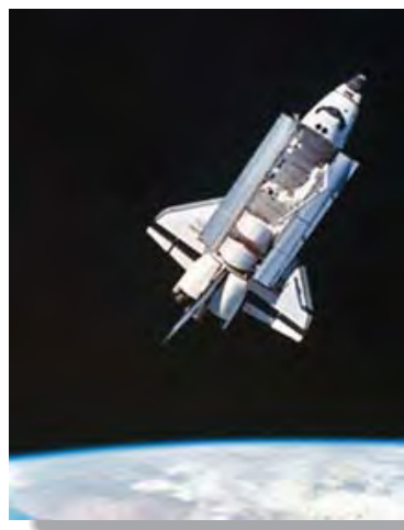
The dynamics of the space shuttle while it orbits the earth can be predicted only if its moments and products of inertia are known relative to its mass center. (©Ablestock/Getty Images)
