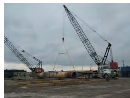
The crane must do work in order to hoist the weight of the pipe. (© R.C. Hibbeler)
