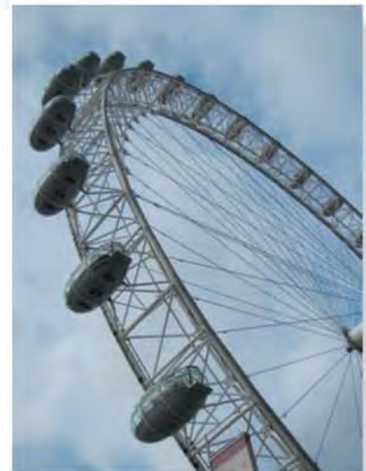
Riders on this Ferris wheel are subjected to curvilinear translation, since the gondolas move in a circular path, yet it always remains in the upright position. (© R.C. Hibbeler)
