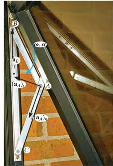
The mechanism for a window is shown. Here CA rotates about a fixed axis through C , and AB undergoes general plane motion. Since point A moves along a curved path it has two components of acceleration, whereas point B moves along a straight track and the direction of its acceleration is specified. (© R.C.Hibbeler)
