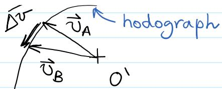
Instantaneous Acceleration  $\vec{a}_{inst} = \lim_{\Delta t \rightarrow 0} \frac{\Delta \vec{v}}{\Delta t} = \frac{d\vec{v}}{dt}$
