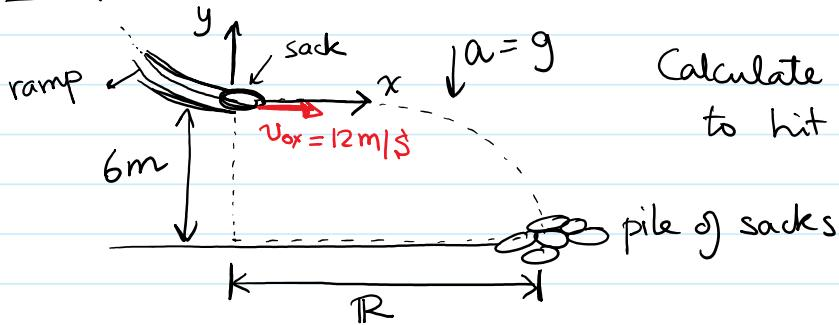
Calculate the time needed to hit the floor and the Range  $R$
