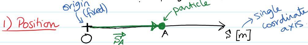
A vector quantity representing the location of a particle at any instant with respect to the point of origin \$O\$.
