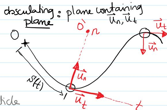
$t$ -axis: tangent to the curve, +ve  $\rightarrow$  increasing  $S$
