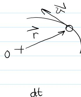
$d\vec{r}$  is tangent to the curve  $\Rightarrow \vec{v}$  is tangent to the curve
