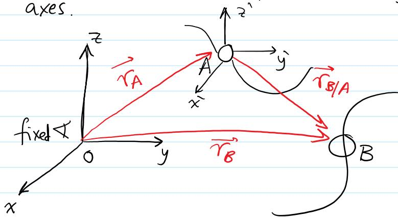
1) Position  $\vec{r}_A, \vec{r}_B$  Absolute positions wrt the fixed frame
