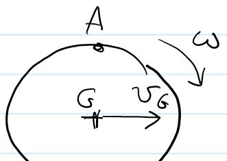
$$T_2 = \frac{1}{2} m v_G^2 + \frac{1}{2} I_G \omega_2^2$$
