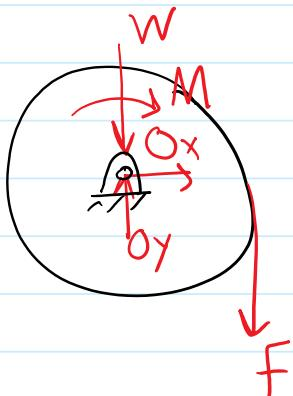
$$\begin{aligned} U_{1 \rightarrow 2} &= U_M + U_F \\ &= M\theta + FS \\ &= 5\theta + 10(r\theta) \end{aligned}$$
