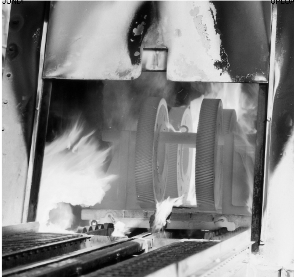
Figure 5.1 Furnace for heat treating steel using the carburization process. (Courtesy of Cincinnati Steel Treating).
