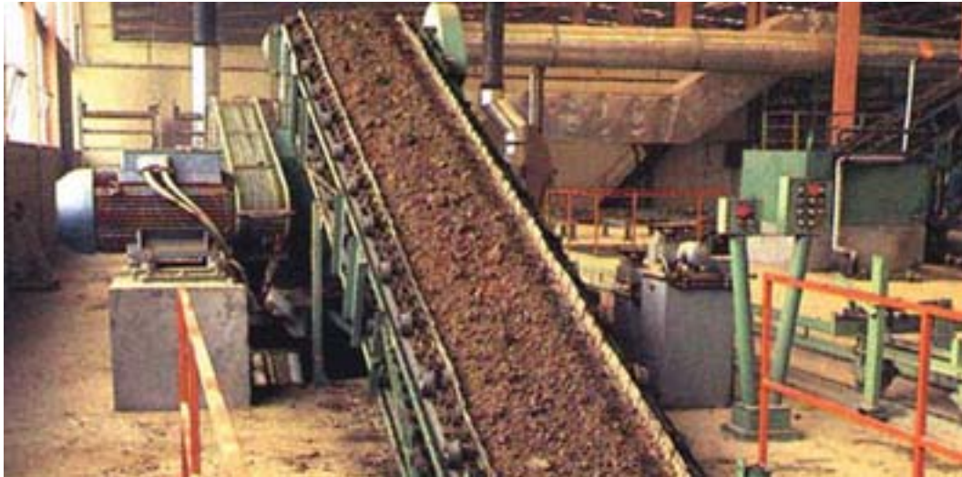
Material being moved via-belt conveyor.
