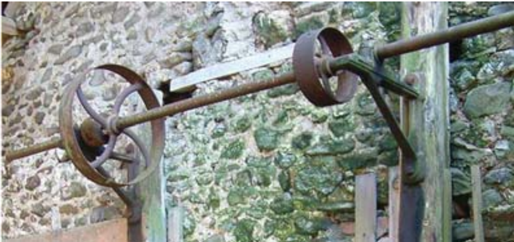
When loads are applied on the above two pulleys, the shaft is subject to torsional vibration
