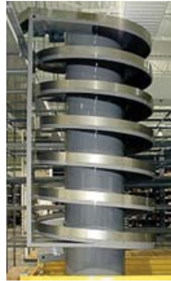
A spiral elevator conveyor for material handling.
