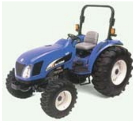
Tractors are specially made to move on rough terrain and exert high power at low speeds.
