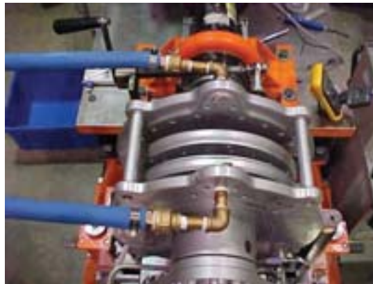
Dynamometers measure the power of the engines.
