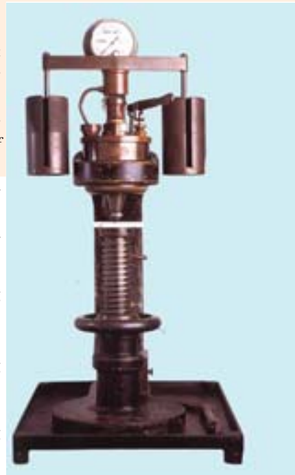
This Brinell hardness testing machine is used to test the hardness of the metal.
