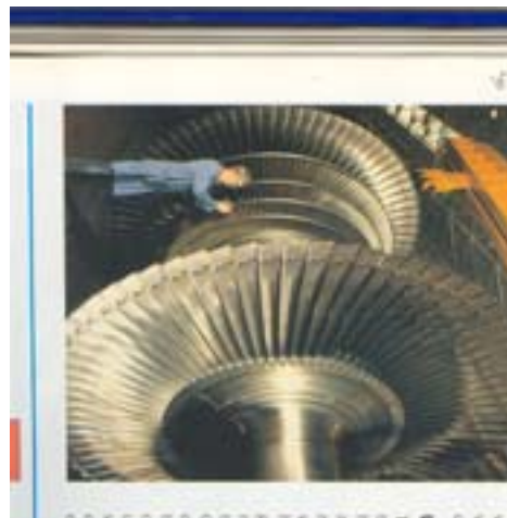
A steam turbine used in thermal power stations.
