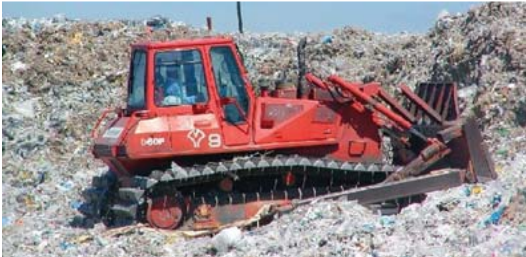
The chain-belt at the bottom of a bulldozer provides powerful grip, spreads weight and force on the ground, and allows to exert high force on the objects to be moved.
