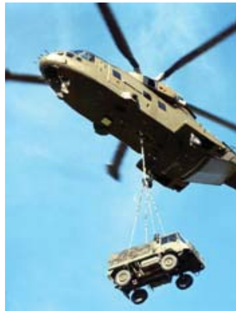
Blades of the helicopter propeller push the air downwards and the resultant reaction gives helicopter the necessary lifting power.
