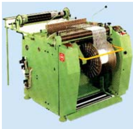
Warping machine uses many mechanisms.
