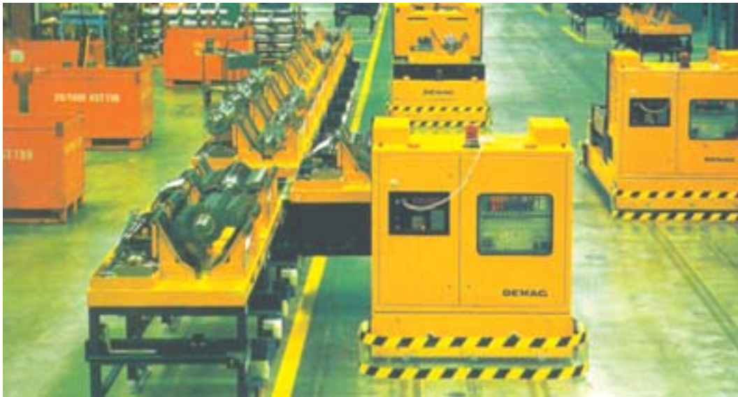
Automated Guided Vehicles, AGVs, operate in many factories. They ferry goods and materials along carefully marked routes. Many AGVs are guided by signals from electrical loops buried under factory floors.
