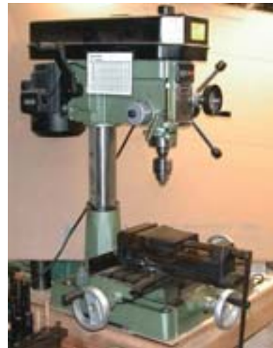
A drill press has a pointed tool which is used for boring holes in hard materials usually by rotating abrasion or repeated blows.
