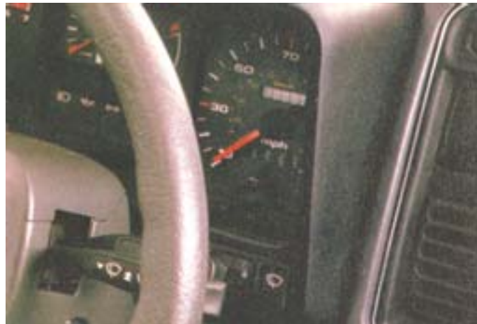
The speedometer is an instrument which shows how fast a car is moving. It works with a magnet that spins around as the car moves.
