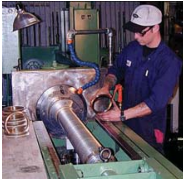
Broaching machine. Broaching is a process of machining through holes of any cross sectional shape, straight and helical slots, external surfaces of various shapes, external and internal toothed gears, splines, keyways and rifling.
