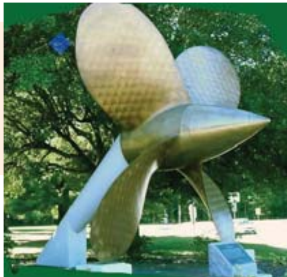
Ship's propeller shown as a separate part. A ship's propeller is located at backside (stern) of the ship below the water surface.
