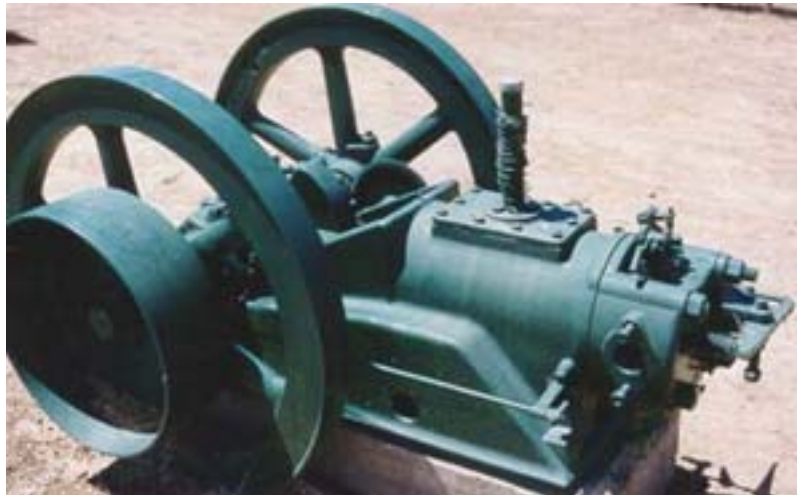
Flywheel of a pump run by a diesel engine.
