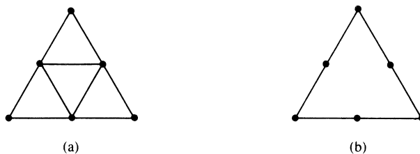
Figure 8–4 Basic triangular element: (a) four-CST and (b) one-LST
