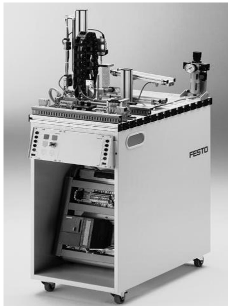
Figure 5.2 Testing Station with Trolley, Control Console and PLC Board
