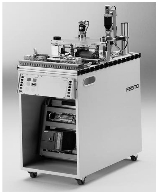
Figure 6.2 Processing Station with Trolley, Control Console and PLC Board
