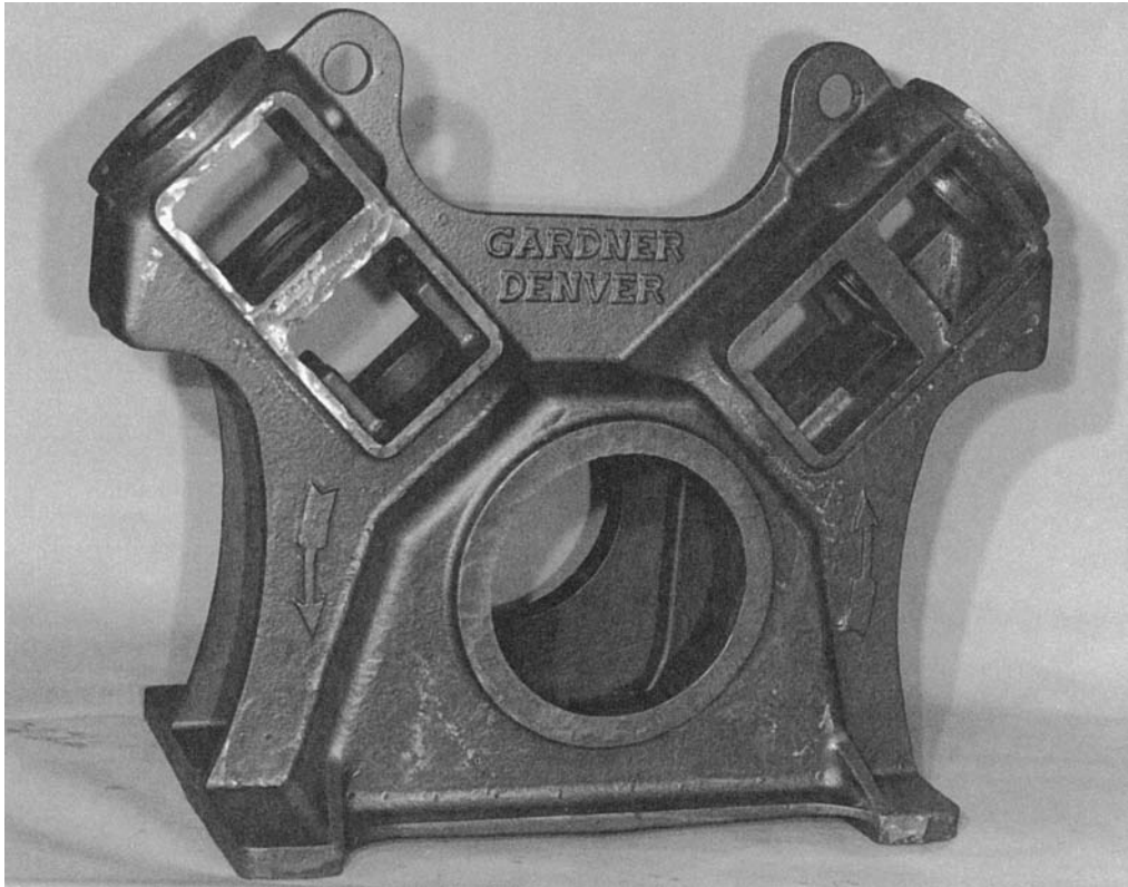
FIGURE 11.1 A large sand casting weighing more than 680 kg (1500 lb) for an air compressor frame. (Courtesy of Elkhart Foundry, photo by Paragon Inc., Elkhart, Indiana.)
