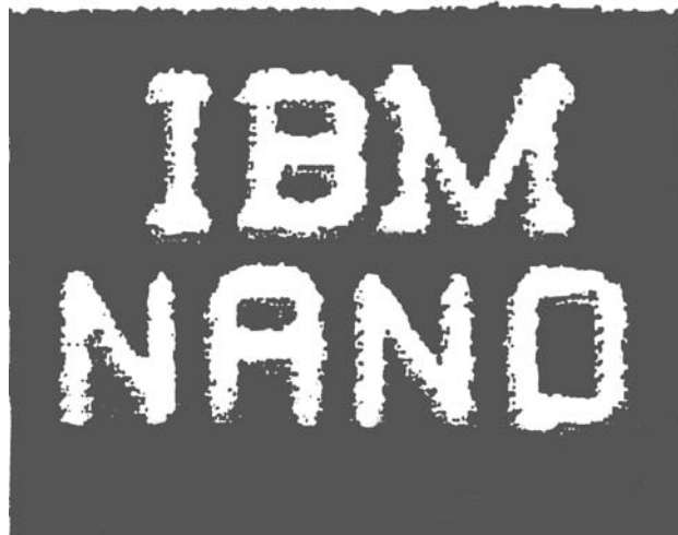
FIGURE 37.3 An atomic force microscope image of silicon dioxide letters on a silicon substrate. The oxide lines of the letters are about 20 nm wide. (Image courtesy of IBM Corporation.)
