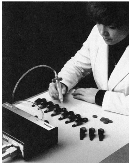
FIGURE 31.13 Adhesive is dispensed by a manually controlled dispenser to bond parts during assembly. (Courtesy of EFD, Inc., East Providence, Rhode Island.)
