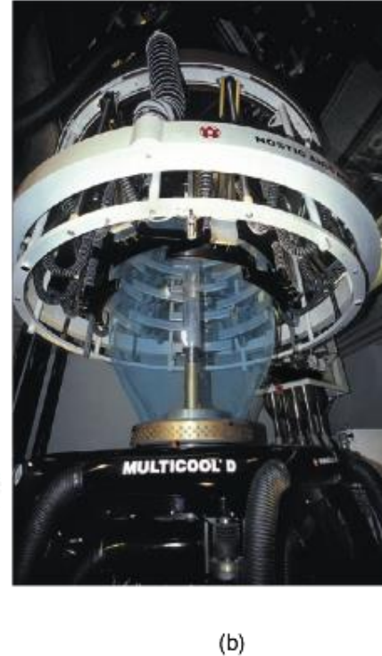
FIGURE 10.25 (a) Schematic illustration of production of thin film and plastic bags from a tube produced by an extruder, and then blown by air. (b) A blown-film operation. Source: Courtesy of Windmoeller & Hoelscher Corp.
