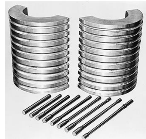
Figure 16-19 (Top) Roll-forging machine in operation. (Right) Rolls from a roll-forging machine and the various stages in roll forging a part. (Courtesy of Ajax Manufacturing Company, Euclid, OH)
