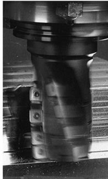
FIGURE 24-8 Solid end mills are often coated. Insert tooling end mills come in a variety of sizes and are mounted on taper shanks.
