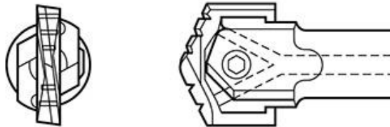
Spade drill with oil holes
