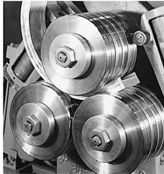
Figure 17-28 (Left) Schematic of the roll-bending process; (right) the roll bending of an I-beam section. Note how the material is continuously subjected to three-point bending. (Courtesy of Buffalo Forge Company, Buffalo, NY.)
