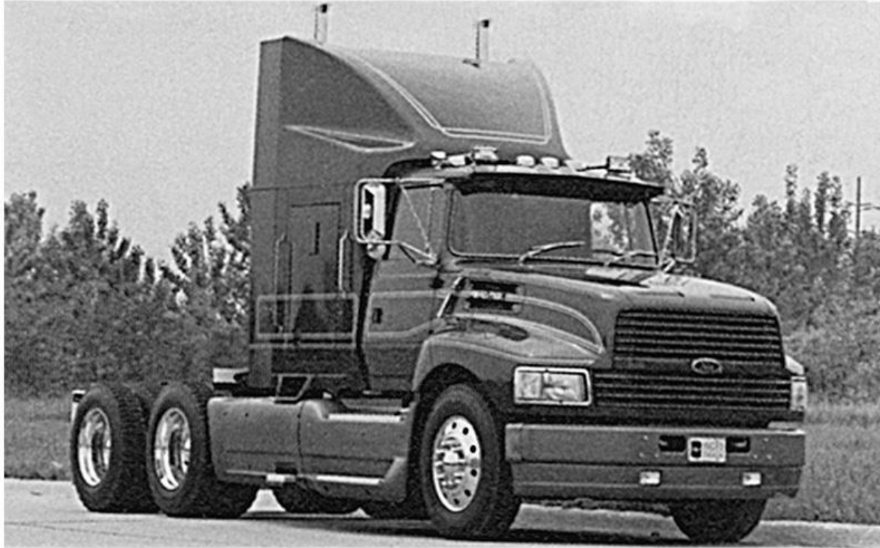
Figure 14-24 Aerodynamic styling and smooth surfaces characterize the hood and fender of Ford Motor Company's AeroMax truck. This one-piece panel was produced as a resin-transfer molding by Rockwell International. ( Courtesy of ASM International, Metals Park, OH. )
