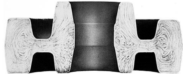
Figure 15-4 Flow structure of a hot-forged gear blank. Note how flow is parallel to all critical surfaces. (Courtesy of Bethlehem Steel Corporation, Bethlehem, PA.)
