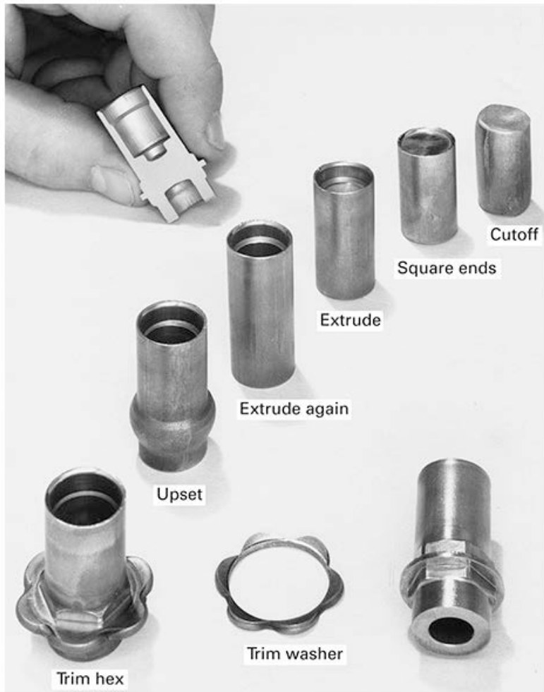
Figure 16-46 Cold-forming sequence involving cutoff, squaring, two extrusions, an upset, and a trimming operation. Also shown are the finished part and the trimmed scrap. (Courtesy of National Machinery Co., Tiffin, OH.)
