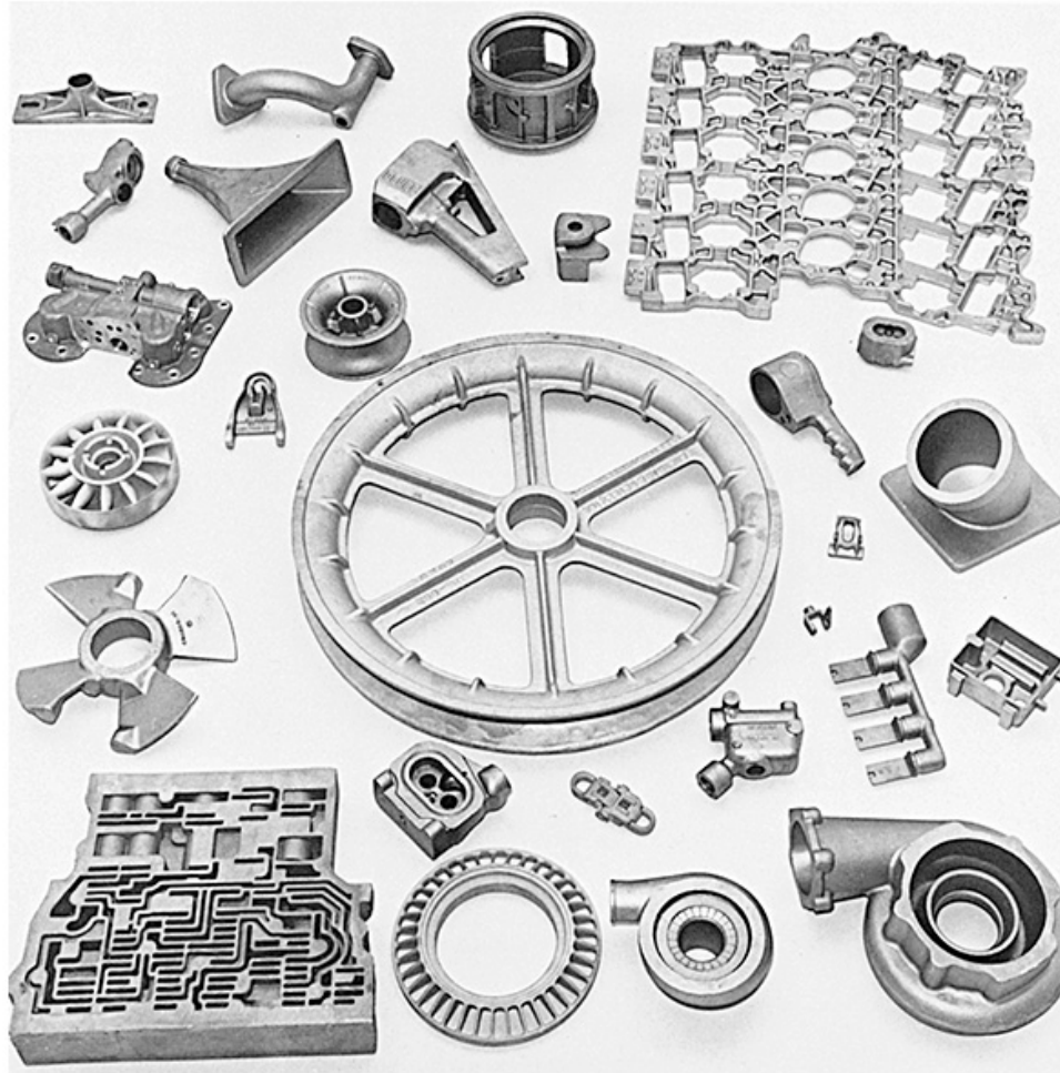
Figure 12-17 A variety of sand cast aluminum parts. (Courtesy of Bodine Aluminum Inc., St. Louis, MO)
