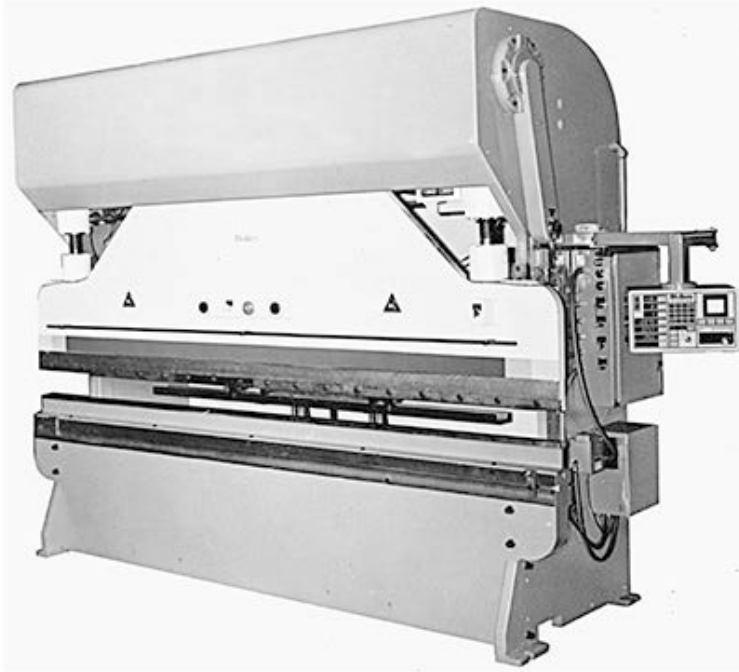
Figure 17-21 (Left) Press brake with CNC gauging system. (Courtesy of DiAcro Division, Acrotech Inc., Lake City, MN.) (Right) Close-up view of press brake dies forming corrugations. (Courtesy of Cincinnati Incorporated, Cincinnati, OH.)
