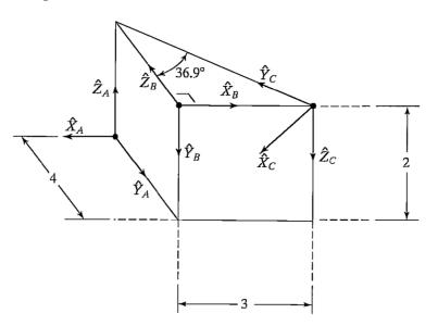
4 The figure shows a schematic of a typical industrial robot with all angles multiples of  $\pm \frac{\pi}{4}$  and the dimensions labeled. Frame 0 is attached to the ground and Frame 6 is attached to the end-effector to which a camera is fixed and pointing in the  $-y_6$  direction.
