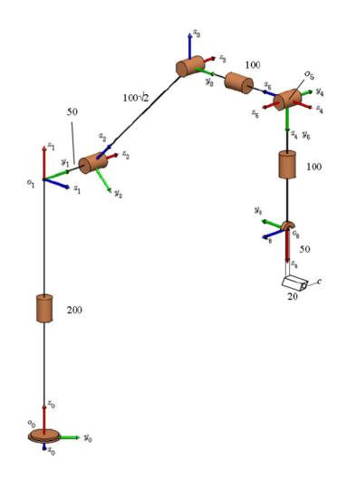
**5** For the robot vehicle shown in the Figure, find  ${}^{0}_{4}T$
