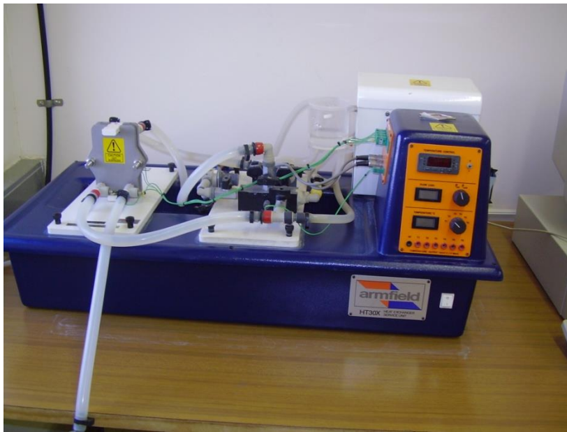
Figure 1 shows the experimental heat exchanger.
