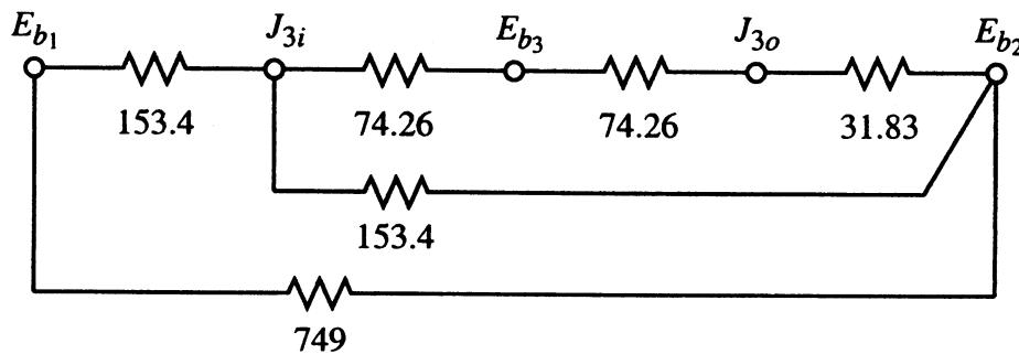
$$\frac{1}{R_l} = \frac{1}{153.4} + \frac{1}{74.26 + 74.26 + 31.83} \quad R_l = 82.89 \quad \frac{1}{R} = 5.5671 \times 10^{-3}$$
