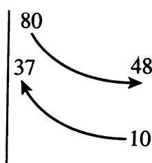
$$c_a = 1005 \quad \rho_a = \frac{1.013 \times 10^5}{(287)(283)} = 1.247 \text{ kg/m}^3$$
