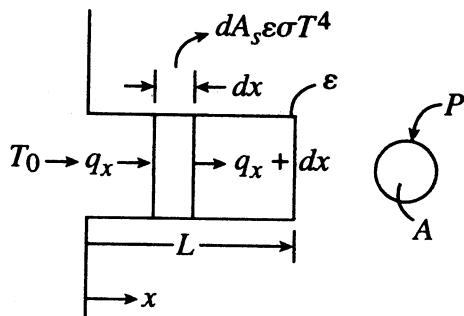
$$q_x = q_{x+dx} + dA_s \varepsilon \sigma T^4 \quad -kA \frac{dT}{dx} = -kA \left( \frac{dT}{dx} + \frac{d^2T}{dx^2} dx \right) + P dx \varepsilon \sigma T^4$$
