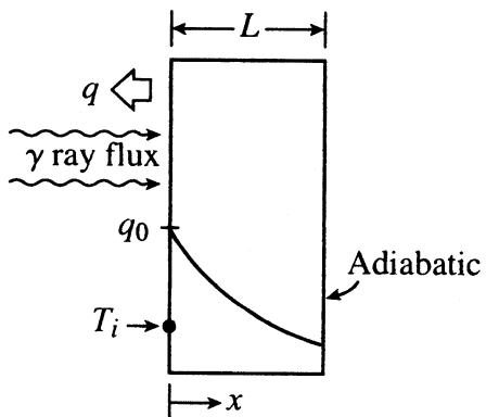
$$\dot{q} = \dot{q}_0 e^{-ax} \quad \frac{d^2T}{dx^2} = \frac{-\dot{q}_0}{k} e^{-ax}$$
