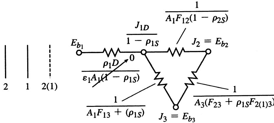
$$T_1 = 823 \text{ K} \quad \epsilon_1 = 0.6 \quad T_3 = 283 \text{ K} \quad \rho_{1D} = 0 \quad \rho_{1S} = 0.4$$
