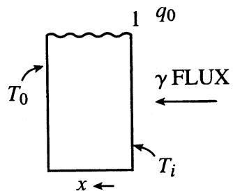
$$\dot{q}_x = \dot{q}_0 e^{-ax} \quad \frac{d^2T}{dx^2} = \frac{-\dot{q}_0 e^{-ax}}{k}$$
