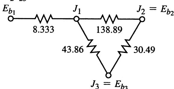
$$q = \frac{3543 - 459}{8.333 + \frac{1}{\frac{1}{43.86} + \frac{1}{138.89 + 30.49}}} = 71.44 \text{ W} = \frac{E_{b_1} - J_1}{8.333} \quad J_1 = 2948 \text{ W/m}^2$$
