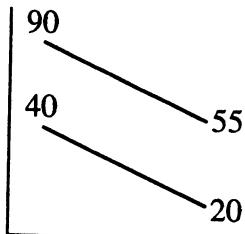
$$\Delta T_m = \frac{50 - 35}{\ln\left(\frac{50}{35}\right)} = 42.06^\circ\text{C} \quad q = UA\Delta T_m \quad A = \frac{59,000}{(340)(42.06)} = 4.11 \text{ m}^2$$
