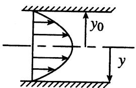
$$\begin{aligned} 2yp - 2yp - 2yp = -2\tau dx = -2\left(\mu \frac{du}{dy}\right)dx \\ ydp = \mu dx \frac{du}{dy} \\ u = \frac{1}{2\mu} \frac{dp}{dx} y^2 + c \quad \text{at } y = y_0 \quad u = 0 \quad c = -\frac{1}{2\mu} \frac{dp}{dx} y_0^2 \\ u = \frac{1}{2\mu} \frac{dp}{dx} (y^2 - y_0^2) \\ \text{at } y = 0 \quad u = u_0 \quad u_0 = \frac{1}{2\mu} \frac{dp}{dx} (-y_0^2) \\ \frac{u}{u_0} = \left(1 - \frac{y^2}{y_0^2}\right) \end{aligned}$$
