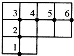
$$\Delta x = \Delta y = 0.5 \text{ m} \quad \text{All internal nodes } k = 1.4$$
