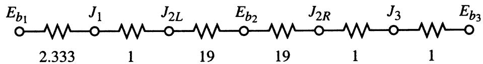
(b)  $q = \frac{37,194 - 1451}{42.333} = 844.3 \text{ W/m}^2 \quad \text{a reduction of 90\%}$
