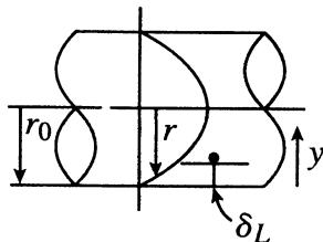
$$\frac{u}{u_c} = \left( 1 - \frac{r}{r_0} \right)^{1/7} \quad f = \frac{0.316}{\text{Re}_r^{1/4}} \quad u_m = \frac{49}{60} u_c = 0.816 u_c$$
