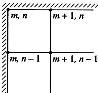
$$T_{m, n-1} + T_{m+1, n} - 2T_{m, n} = \bar{q}_{m, n}$$
