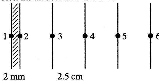
Because polyethylene is so thin it can be neglected in comparison to other material
