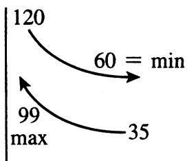
$$q_{\text{max}} = m_w c_w \Delta T_w = \frac{230}{3600} (4180)(99 - 35) = 17,090 \text{ W}$$
