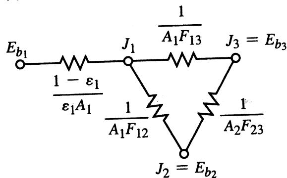
$$\frac{X}{D} = 1.0 \quad \frac{Y}{D} = 1.5 \quad F_{13} = 0.25 \quad F_{12} = 0.75$$
