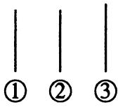
$$T_1 = 1073 \text{ K} \quad T_3 = 308 \text{ K} \quad \epsilon_1 = 0.5 \quad \epsilon_3 = 0.8 \quad \rho_{2D} = 0.4$$
