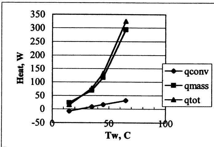
$$q = hA(T_w - T_\infty) + h_D A(C_w - C_\infty)h_{fg} = q_{\text{conv}} + q_{\text{mass}}$$
