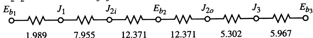
$$\frac{q}{L} = \frac{E_{b_1} - E_{b_3}}{\sum R} = \frac{75,146 - 1097}{45.953} = 1611 \text{ W/m} \quad \text{a reduction of 65%}$$
