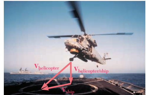
Photo 11.4 The pilot of a helicopter landing on a moving carrier must take into account the relative motion of the ship.
