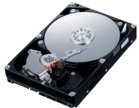
Photo 16.2 The hard disk and pick-up arm of a computer hard drive undergo fixed-axis rotation.
