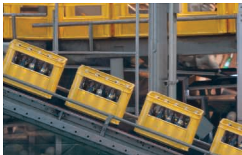
Photo 8.2 The coefficient of static friction between a crate and the inclined conveyor belt must be sufficiently large to enable the crate to be transported without slipping.
