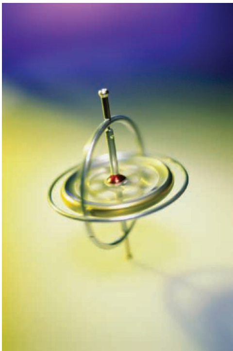
Photo 18.5 A gyroscope can be used for measuring orientation and is capable of maintaining the same absolute direction in space.
