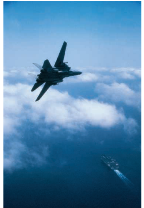
Photo 12.3 A fighter jet making a sharp turn has a large normal component of acceleration, often equal to several g . As a result, the pilot experiences a large normal force, which in extreme cases, can cause blackouts.
