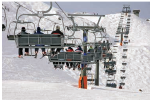
Photo 13.1 The power used to operate a chair lift at a ski resort is the product of the force applied and the speed of the lift.
