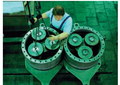
Photo 15.4 Planetary gear systems are used in applications requiring a large reduction ratio and a high torque-to-weight ratio. The small gears undergo general plane motion.
