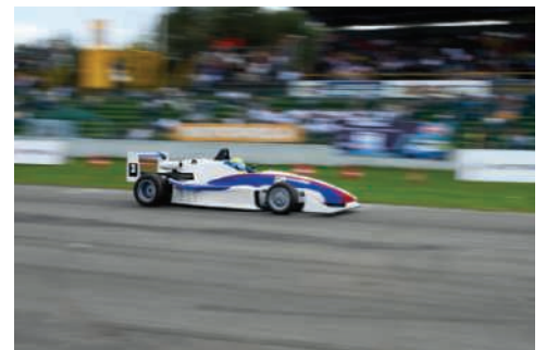
Photo 12.1 When the racecar accelerates forward, the rear tires have a friction force acting on them in the direction the car is moving.
