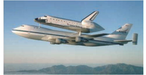
Photo 5.5 To predict the flight characteristics of the modified Boeing 747 when used to transport a space shuttle, engineers had to determine the center of gravity of each craft.
