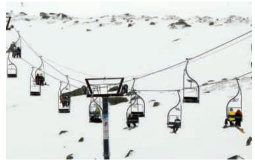
Photo 7.3 The weight of the chairlift cables is negligible compared to the weights of the chairs and skiers, so we can use the methods of this section to determine the force at any point in the cable.
