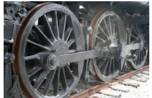
Photo 15.1 The horizontal linkage of a locomotive undergoes curvilinear translation.
