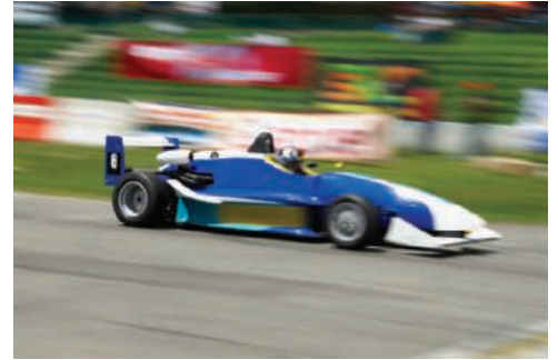
Photo 15.5 If the tires of this car are rolling without sliding, the instantaneous center of rotation of each tire is the point of contact between the road and the tire.
