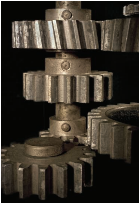
Photo 15.2 For the central gear rotating about a fixed axis, the angular velocity and angular acceleration of that gear are vectors directed along the vertical axis of rotation.
