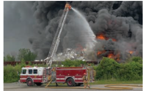
Photo 15.8 You can obtain the angular velocity of a fire truck ladder rotating about its fixed base by adding the angular velocities that correspond to simultaneous rotations about two different axes.
