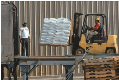
Photo 16.3 The forklift and moving load can be analyzed as a system of two connected rigid bodies in plane motion.
