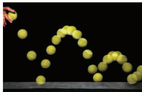
Photo 13.5 The height the tennis ball bounces decreases after each impact because it has a coefficient of restitution less than one and energy is lost with each bounce.
