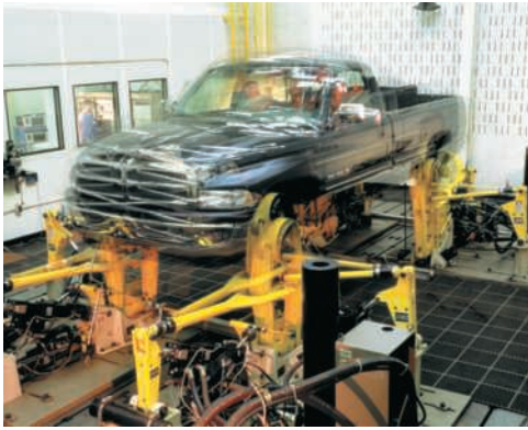
Photo 19.3 This truck is experiencing damped vibration in the vehicle dynamics test.
