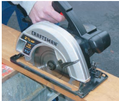
Photo 7.1 The design of the shaft of a circular saw must account for the internal forces resulting from the forces applied to the teeth of the blade. At a given point in the shaft, these internal forces are equivalent to a force-couple system consisting of axial and shearing forces and couples representing the bending and torsional moments.
