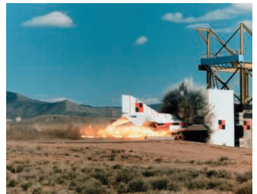
Photo 13.4 This impact test between an F-4 Phantom and a rigid reinforced target was to determine the impact force as a function of time.
