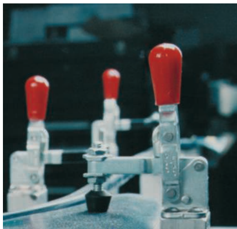
Photo 10.3 The clamping force of the toggle clamp shown can be expressed as a function of the force applied to the handle by first establishing the geometric relations among the members of the clamp and then applying the method of virtual work.
