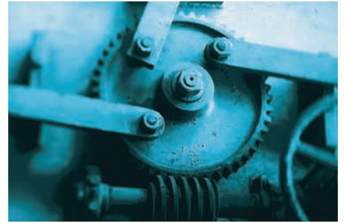
Photo 15.6 The central gear rotates about a fixed axis and is pin-connected to three bars in general plane motion.
