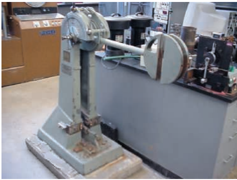
Photo 17.2 A Charpy impact test is used to determine the amount of energy absorbed by a material during impact. To determine the amount of energy absorbed, the final gravitational potential energy of the arm is subtracted from its initial gravitational potential energy.
