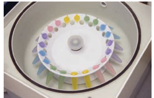
Photo 12.4 The forces on the specimens used in a high speed centrifuge can be described in terms of radial and transverse components. UPLOADED BY AHMAD T JUNDI
