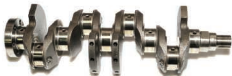
Photo 9.2 The rotational behavior of this crankshaft depends upon its mass moment of inertia with respect to its axis of rotation, as you will see in a dynamics course.
