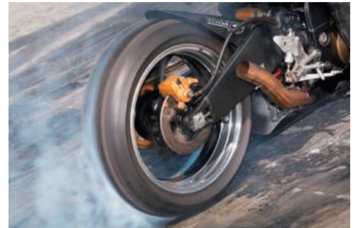
Photo 17.1 The work done by friction reduces the kinetic energy of the wheel.
