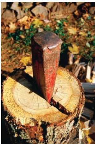
Photo 8.3 Wedges are used as shown to split tree trunks because the normal forces exerted by a wedge on the wood are much larger than the force required to insert the wedge.
