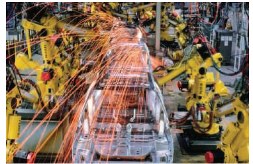
Photo 18.1 The design of a robotic welder for an automobile assembly line requires a three-dimensional study of both kinematics and kinetics.
