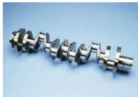
Photo 18.4 The rotating automobile crankshaft causes static and dynamic reactions on its bearings. The crankshaft can be designed to minimize dynamic imbalances and reduce these reaction forces.
