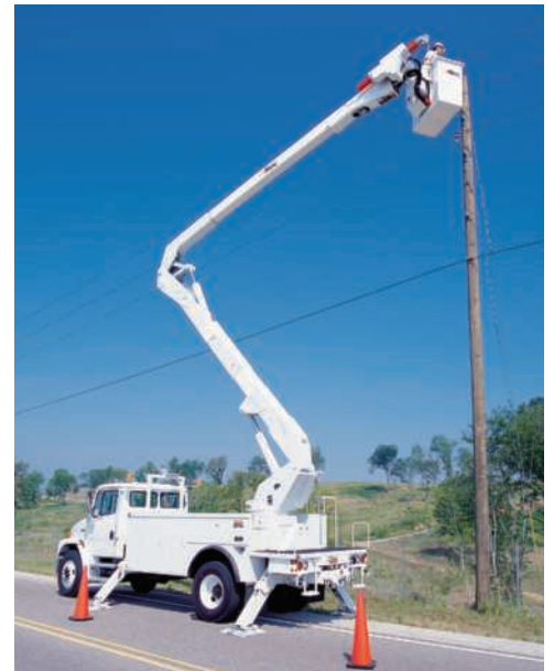
Photo 10.2 The method of virtual work is useful for determining the forces exerted by the hydraulic cylinders positioning the bucket lift. The reason is that a simple relation exists among the displacements of the points of application of the forces acting on the members of the lift.
