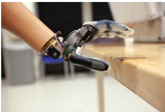
Photo 6.6 Frames and machines contain multi-force members. Frames are fully constrained structures, whereas machines like this prosthetic hand are movable and designed to transmit or modify forces.
