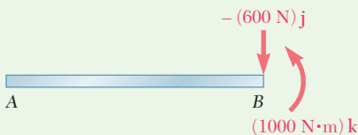
Fig. 2 Finding force-couple system at B equivalent to that determined in part a.
