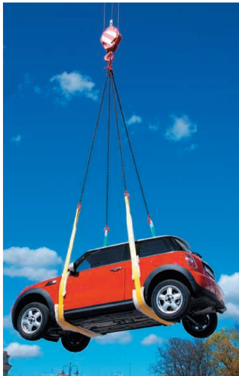
Photo 2.4 Although we cannot determine the tension in the four cables supporting the car by using the three equations (2.34), we can obtain a relation among the tensions by analyzing the equilibrium of the hook.
