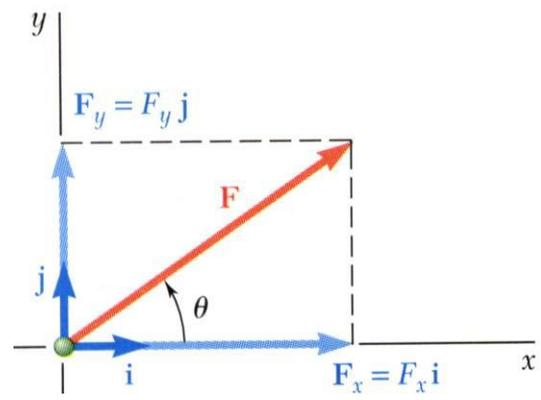
$F_x$  and  $F_y$  are referred to as the *scalar components* of  $\vec{F}$
