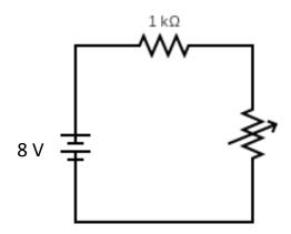
After building this electrical circuit in which the electromotive force is equal to 8 volts, we change the value of the variable resistance according to the values mentioned above in the data, to find out the current values at each different value of the resistance, This enables us to calculate the value of the internal resistance in two ways.
