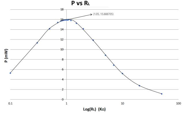
And now if we apply the condition of maximum power transfer to the load resistance of the same circuit we get: RL = R + rin, We calculate the other value of the internal resistance and then the rate.
