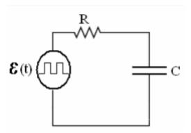
During the positive half period of the square wave, the charge in the straightforward RC circuit accumulates on the capacitor plates according to the following formula:
