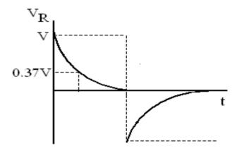
A positive charge will build up on one of the capacitor plates when it is linked to a power source, and a similar negative charge will build up on the other. The charge build-up causes an electric field to develop between the capacitor plates. The capacitor is charged throughout this procedure. and the capacitor will discharge and each of its plates will turn neutral.
