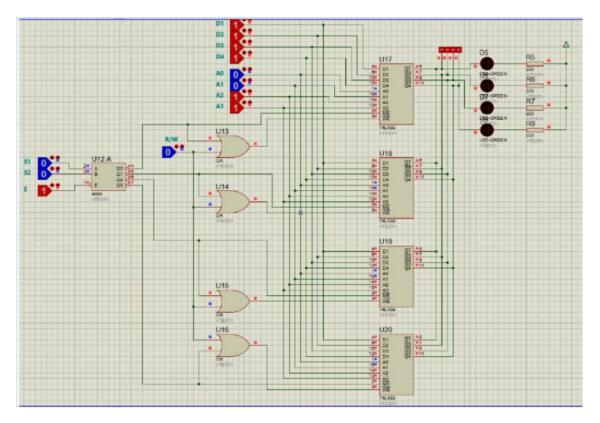
First, we need to design four separate 4x4 RAMs. Each RAM will have 4 address lines, A0-A3, four data lines, D0-D3, and an active low write line (WR\*).
