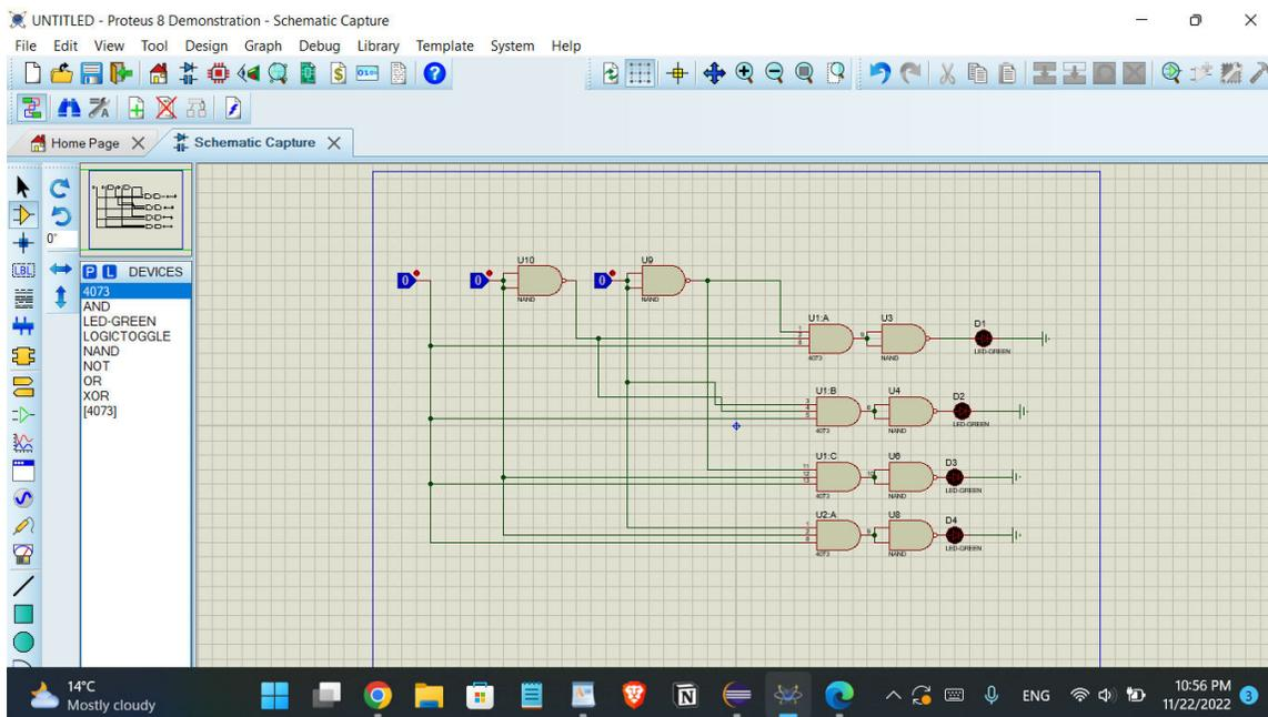
f) Use the 2x4 decoder to implement a 2 inputs function that acts like an equivalence gate
