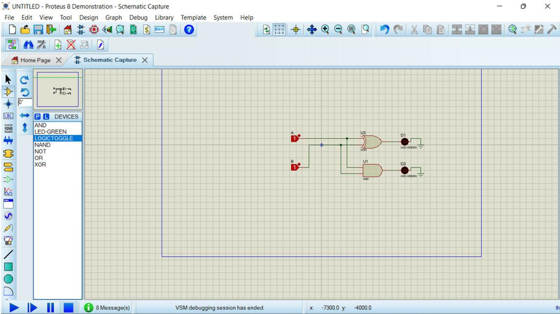
b) Build the bellow circuit using universal gates
