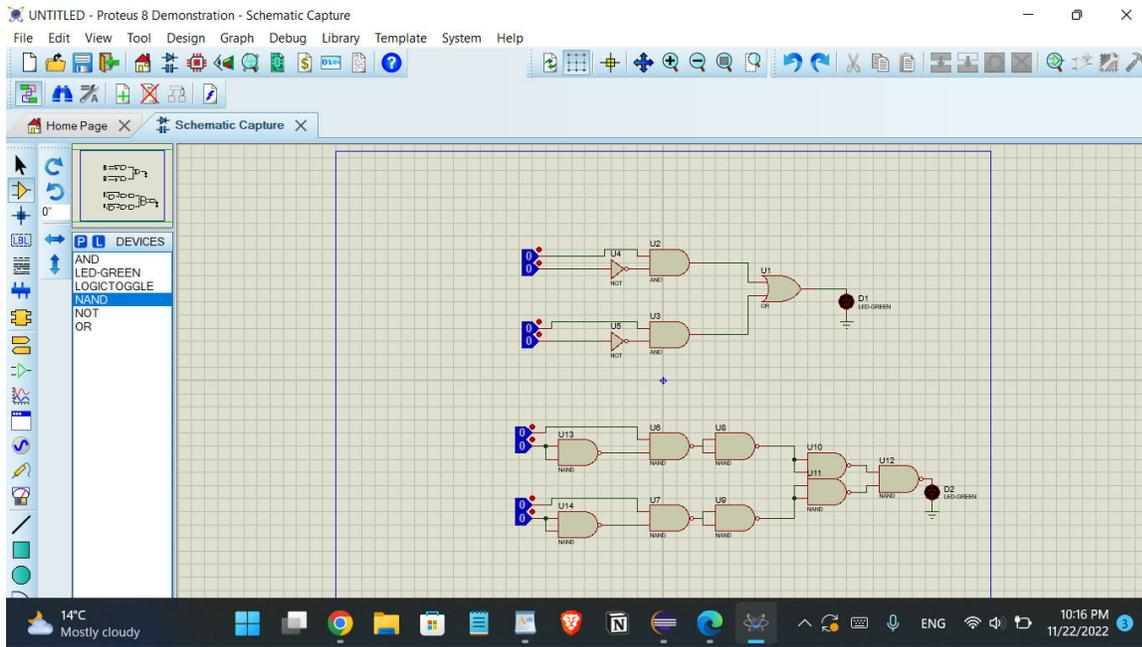
c) Build a 3x8 Decoder (active low) using basic gates.
