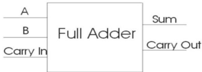
Figure (3): Full-Adder Functional Diagram.
