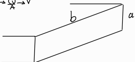
$$D_h = \frac{4 \times \text{Cross sectional area}}{\text{Perimeter}} = \frac{2ab}{a+b}$$
