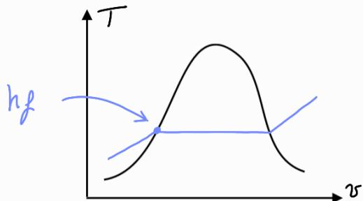
The expansion valve changes the pressure and temperature but enthalpy is constant so:  $h_{inlet} = h_{tank} = 503.69 \text{ kJ/kg}$
