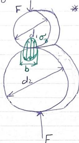
► Gear involute is treated as cylinder with radius equals to radius of curvature of involute at contact point
