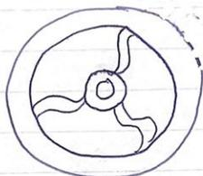
$$m_B = \frac{b_R}{h_t} = \frac{\text{Rim thickness}}{\text{height of tooth}}$$
