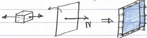
Shear Force. → It Does a shear stress
