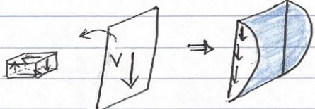
Bending Moment. → It Does a stress (Bending Stress)
